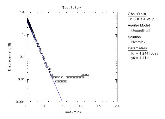
**Figure C-20.** Graphical Representation of Raw Data Obtained from Slug Test of 3BS1-GW3p, Hvorslev Solution
