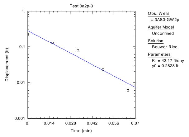
**Figure C-7.** Graphical Representation of Raw Data Obtained from Slug Test of 3AS3-GW2p, Bouwer-Rice Solution
