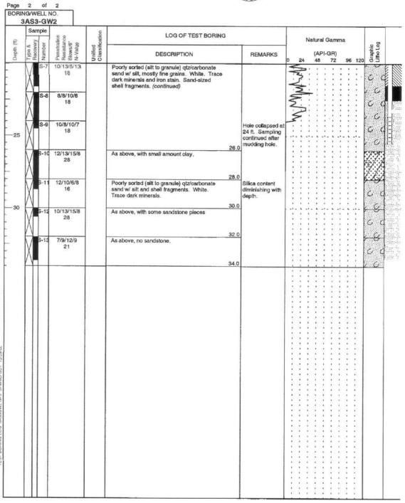
Figure B-19. Test Boring Log for Well 3AS3-GW2 (Sheet 2 of 2)
