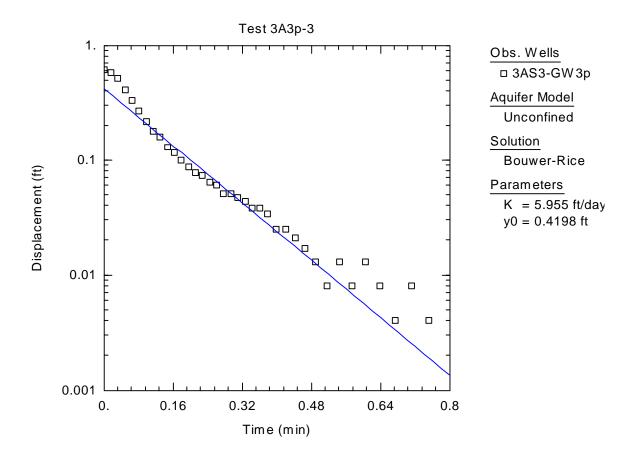
**Figure C-11.** Graphical Representation of Raw Data Obtained from Slug Test of 3AS3-GW3p, Bouwer-Rice Solution
