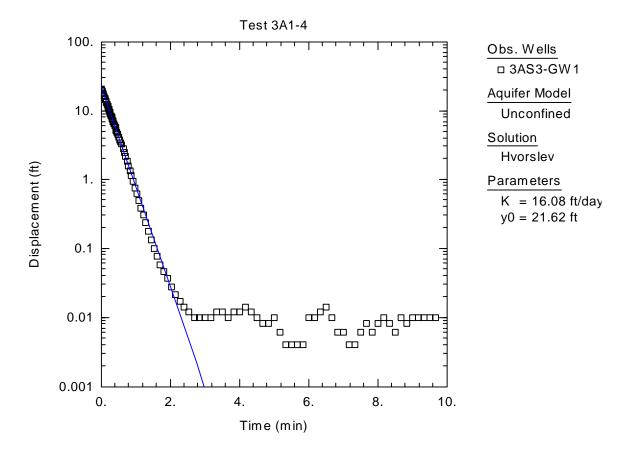
**Figure C-2.** Graphical Representation of Raw Data Obtained from Slug Test of 3AS3-GW1, Hvorslev Solution
