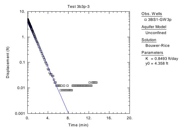
**Figure C-19.** Graphical Representation of Raw Data Obtained from Slug Test of 3BS1-GW3p, Bouwer-Rice Solution
