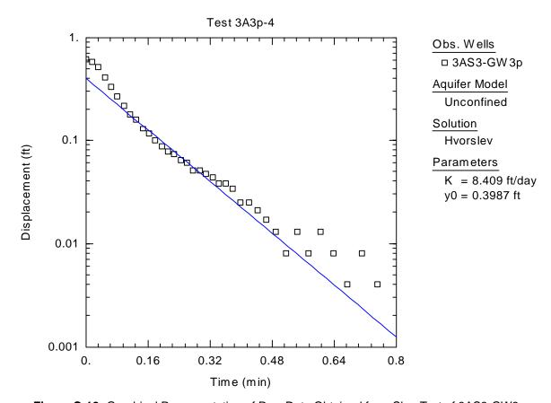
**Figure C-12.** Graphical Representation of Raw Data Obtained from Slug Test of 3AS3-GW3p, Hvorslev Solution
