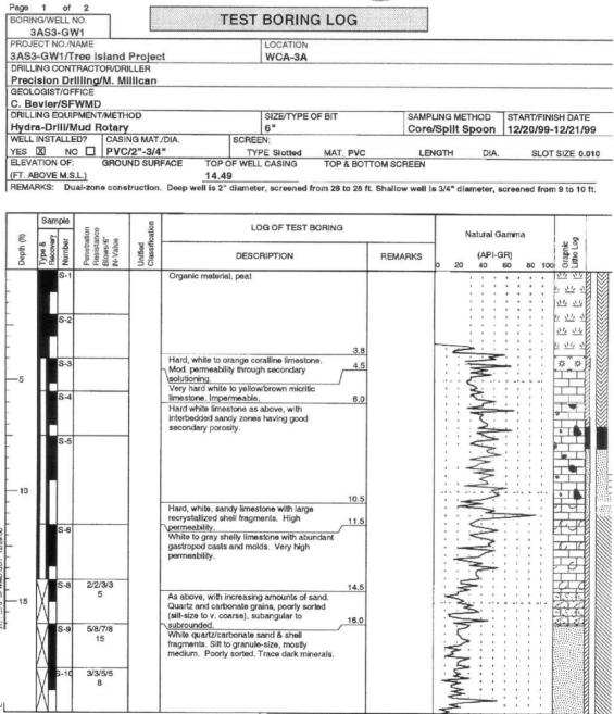
Figure B-16. Test Boring Log for Well 3AS3-GW1 (Sheet 1 of 2)
