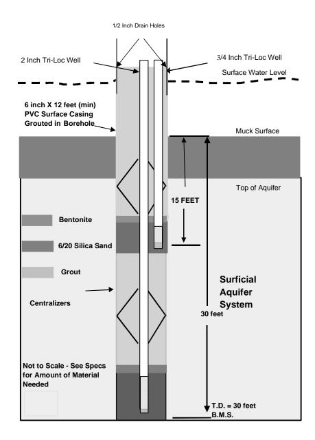
Figure A-10. 30/15-ft Dual Completion Monitor Well
