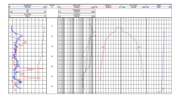
Figure B-39. Geophysical Logs for Well 3BS1-GW4
