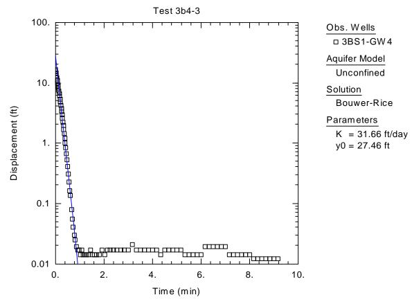
**Figure C-21.** Graphical Representation of Raw Data Obtained from Slug Test of 3BS1-GW4, Bouwer-Rice Solution
