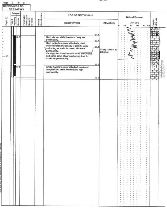
Figure B-29. Test Boring Log for Well 3BS1-GW3 (Sheet 2 of 2)
