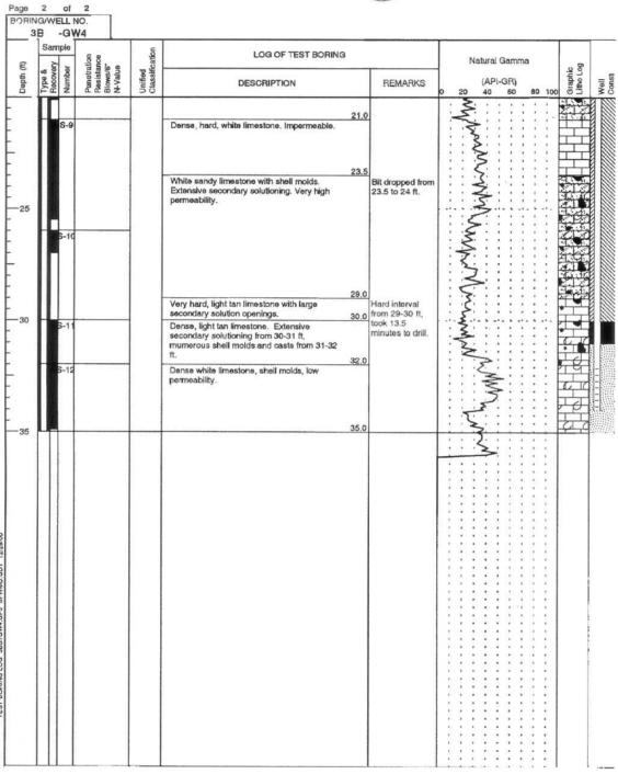
Figure B-31. Test Boring Log for Well 3BS1-GW4 (Sheet 2 of 2)
