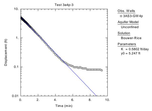
**Figure C-15.** Graphical Representation of Raw Data Obtained from Slug Test of 3AS3-GW4p, Bouwer-Rice Solution
