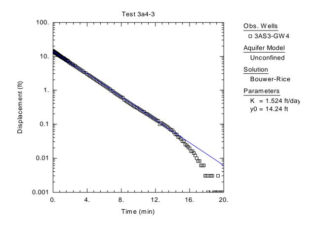
**Figure C-13.** Graphical Representation of Raw Data Obtained from Slug Test of 3AS3-GW4, Bouwer-Rice Solution
