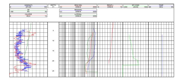
Figure B-38. Geophysical Logs for Well 3BS1-GW3
