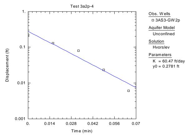
**Figure C-8.** Graphical Representation of Raw Data Obtained from Slug Test of 3AS3-GW2p, Hvorslev Solution
