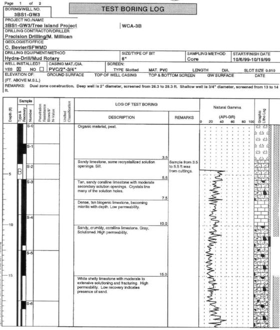
Figure B-28. Test Boring Log for Well 3BS1-GW3 (Sheet 1 of 2)
