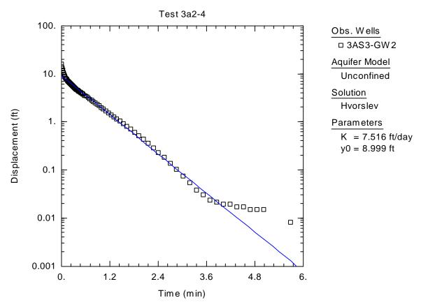
**Figure C-6.** Graphical Representation of Raw Data Obtained from Slug Test of 3AS3-GW2, Hvorslev Solution
