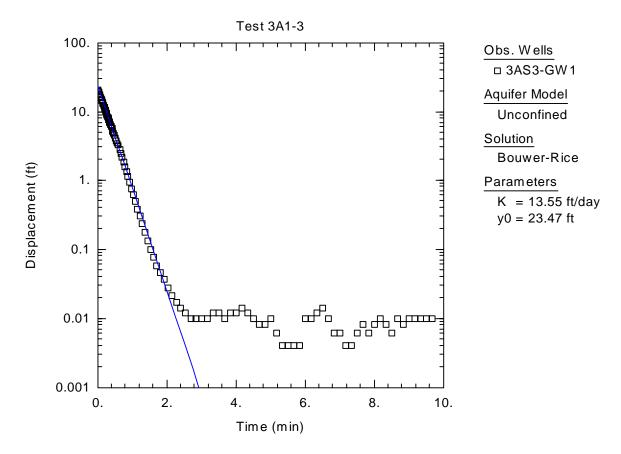
**Figure C-1.** Graphical Representation of Raw Data Obtained from Slug Test of 3AS3-GW1, Bouwer-Rice Solution
