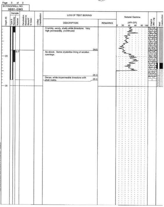
Figure B-27. Test Boring Log for Well 3BS1-GW2 (Sheet 2 of 2)
