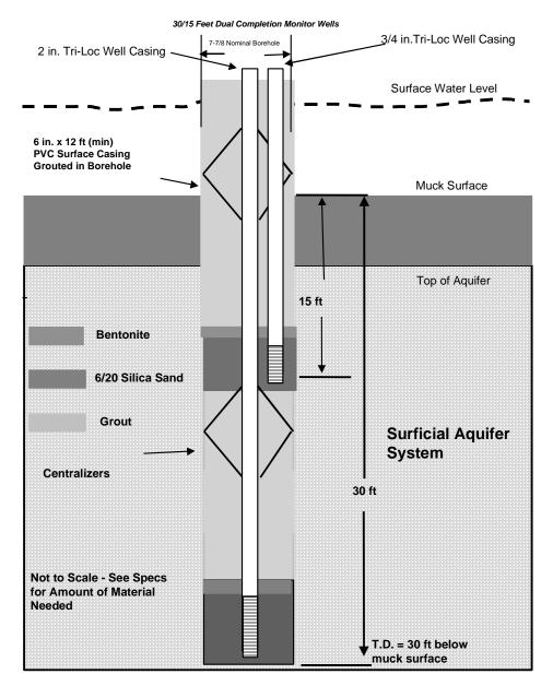
Figure 4. General Schematic of Dual Zone Monitor Well
