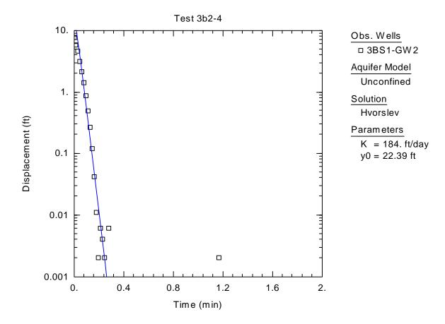
**Figure C-18.** Graphical Representation of Raw Data Obtained from Slug Test of 3BS1-GW2, Hvorslev Solution
