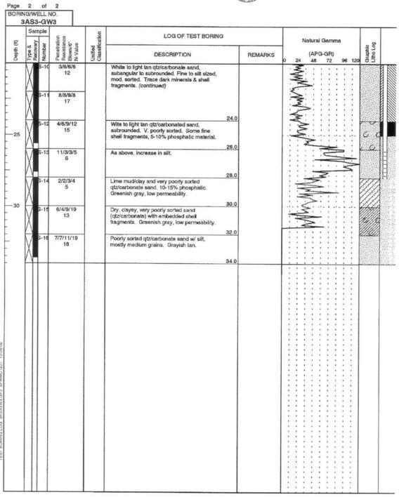
Figure B-21. Test Boring Log for Well 3AS3-GW3 (Sheet 2 of 2)
