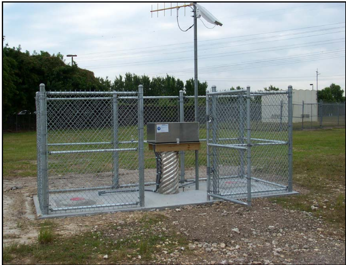
Figure 9. Instrumented groundwater monitor station.
