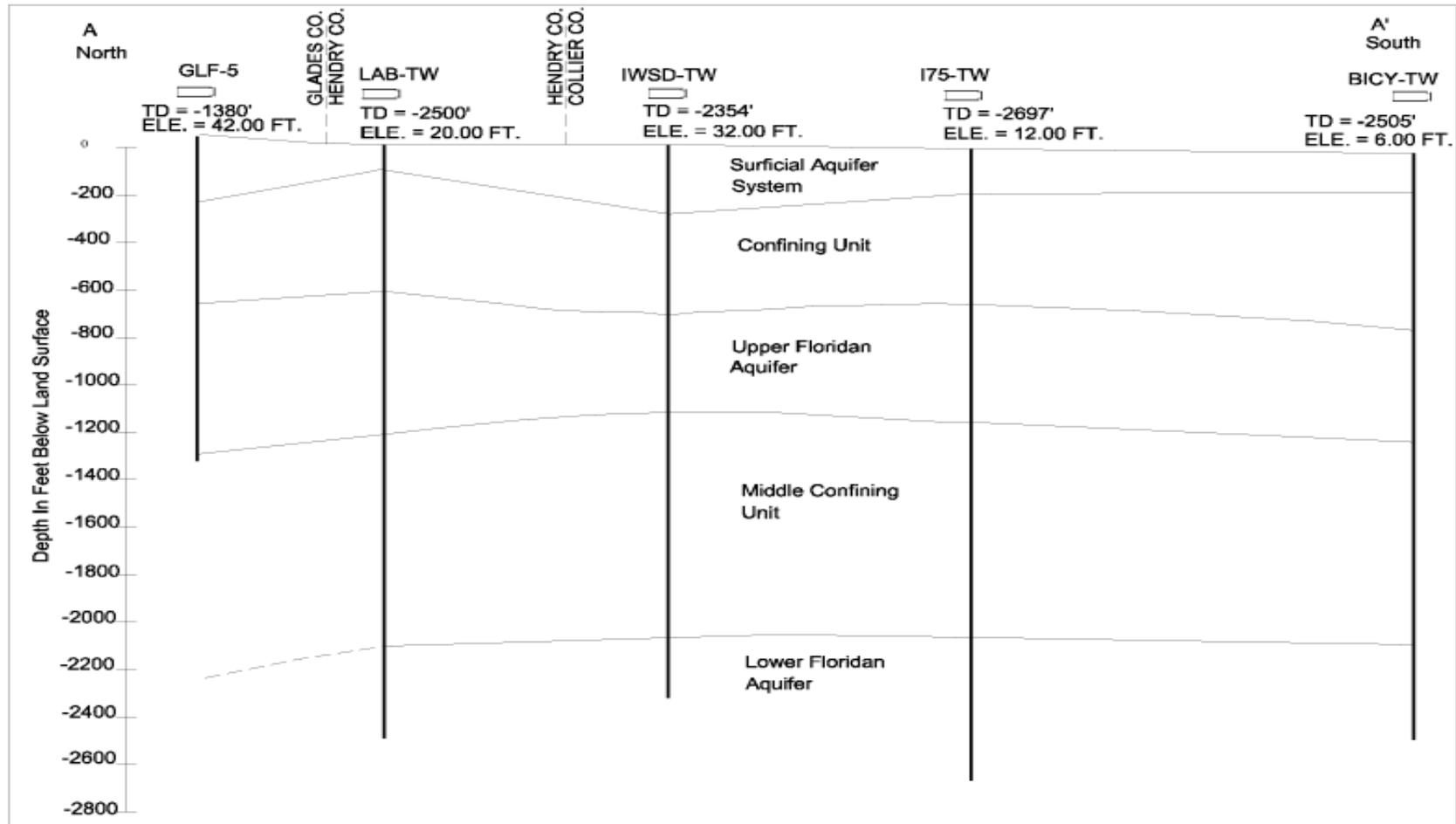
Figure 2. Hydrostratigraphic Cross-Section from A-A' through Southwestern Florida (Line of Cross-Section Shown in Figure 1.)
