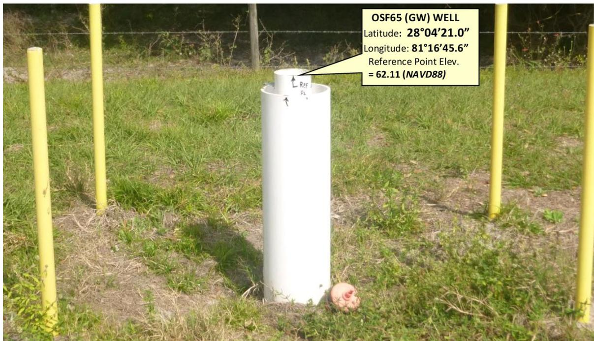
Figure 4. Completed wellhead, showing measuring point elevation for depth-to-water measurements for OSF-65.
