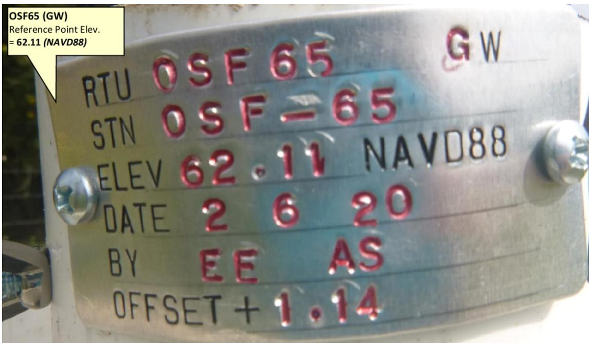
Figure 6. Close-up of brass tag and reference location for OSF-65.
