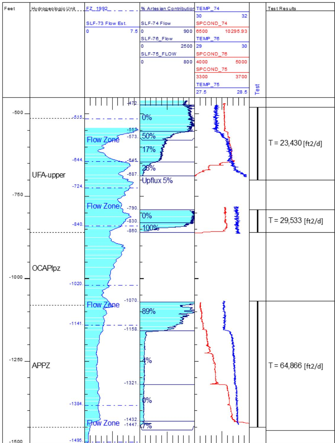
Figure 13. Comparison of flowmeter logs from SLF-73 (1990) and SLF-74, SLF-75, and SLF-76 (2016).
