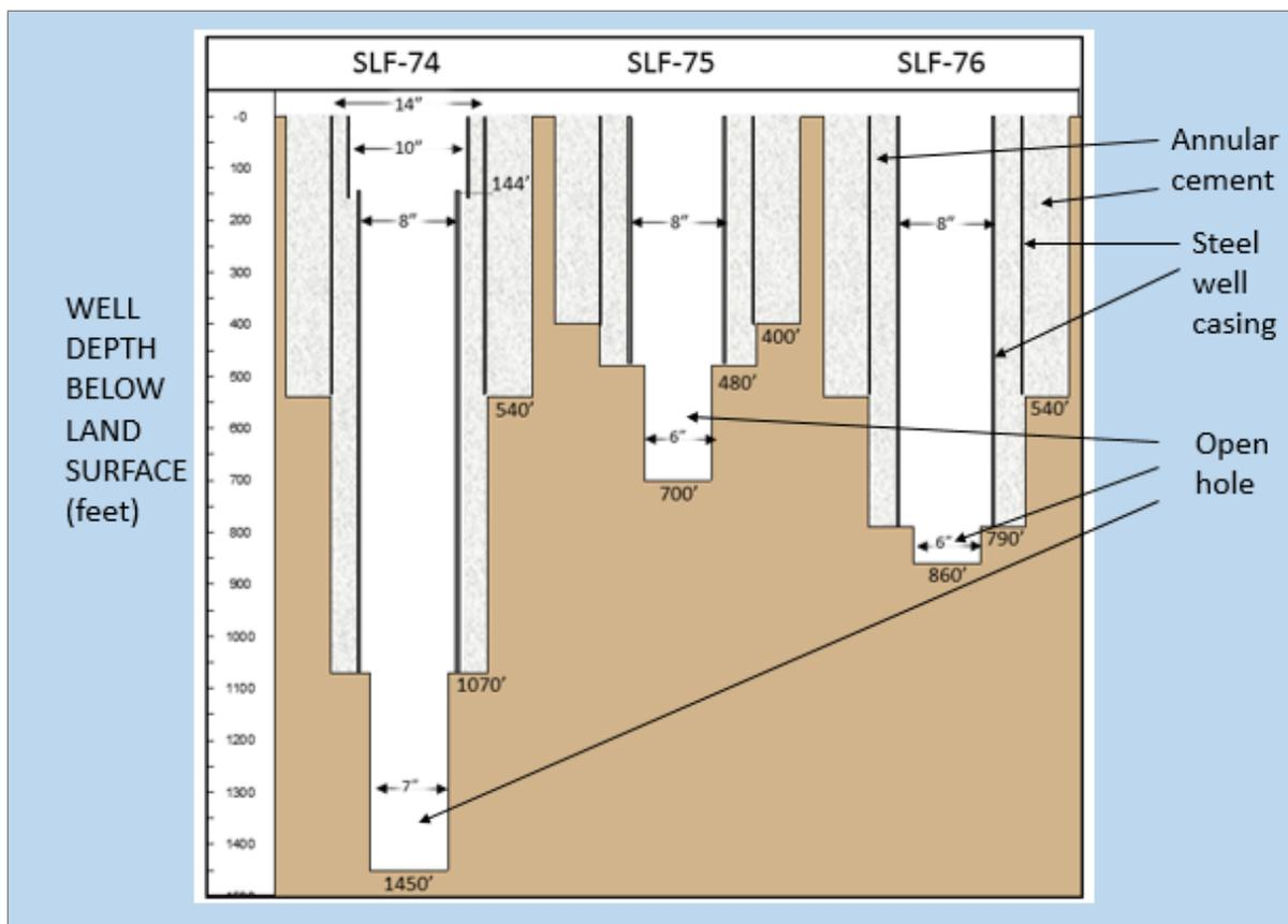
Figure 3. Well completion diagram for production wells SLF-74, SLF-75, and SLF-76.
