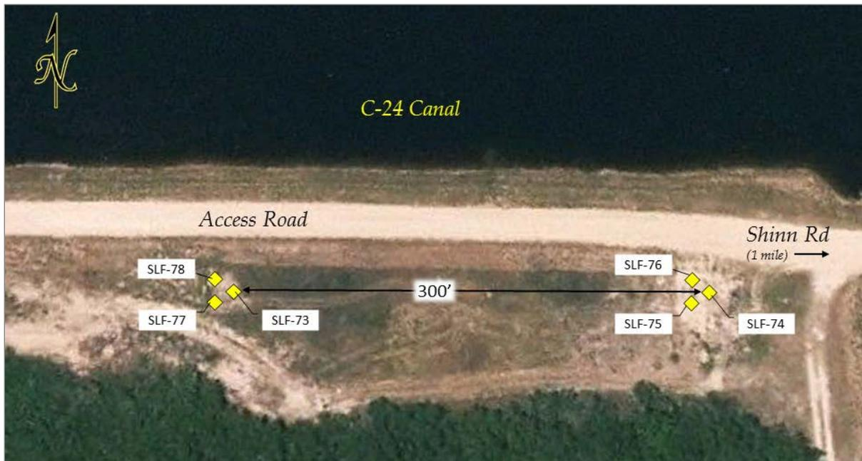
Figure 2. Location of monitor and production wells at the C-24 Canal test site.
