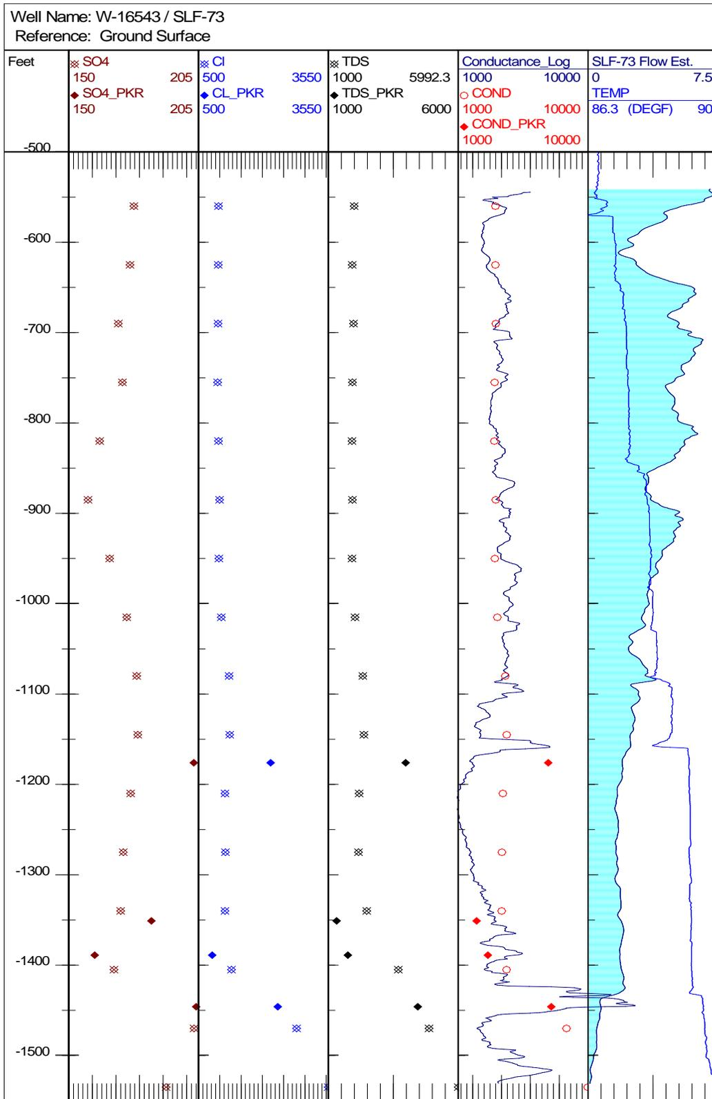
Figure 9. Comparison of drill-stem and packer test results with geophysical logs from pilot hole drilling at well SLF-73.
