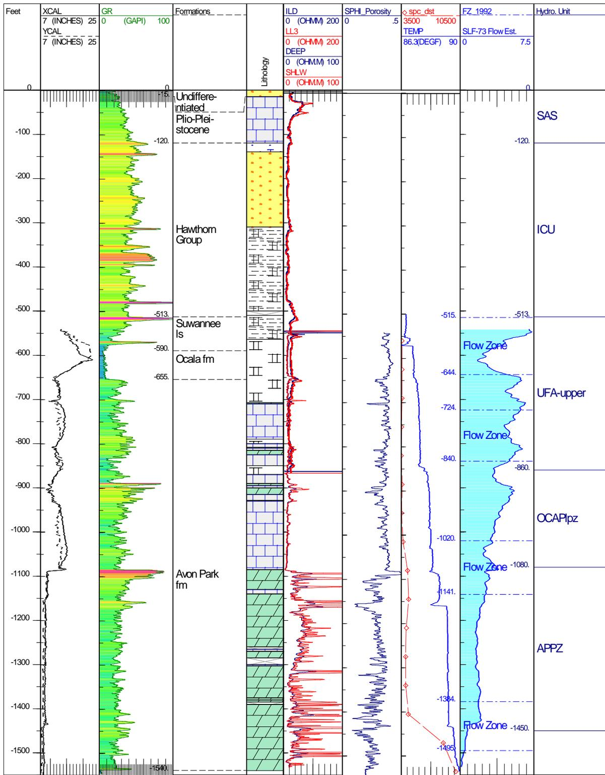
Figure 8. Borehole geophysical logs and delineation of lithologic and hydrogeologic units at the C-24 Canal site.
