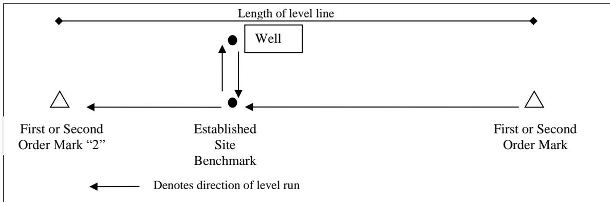
The FGCS maximum allowable misclosure for this type of run is 0.03' multiplied by the square root of the length of the line in miles.
