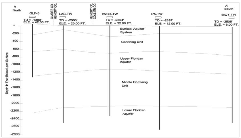
Figure 2. Hydrostratographic Cross-Section from A-A' through Southwestern Florida (Line of Cross-Section Shown in Figure 1.)
