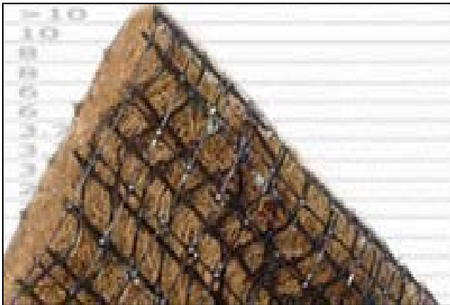
Figure H3. Turf reinforcement mat (from NRCS 2 , 2007)
