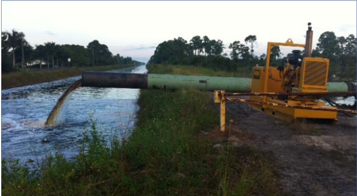
24" Pump from Corbett to M-O Canal extension
