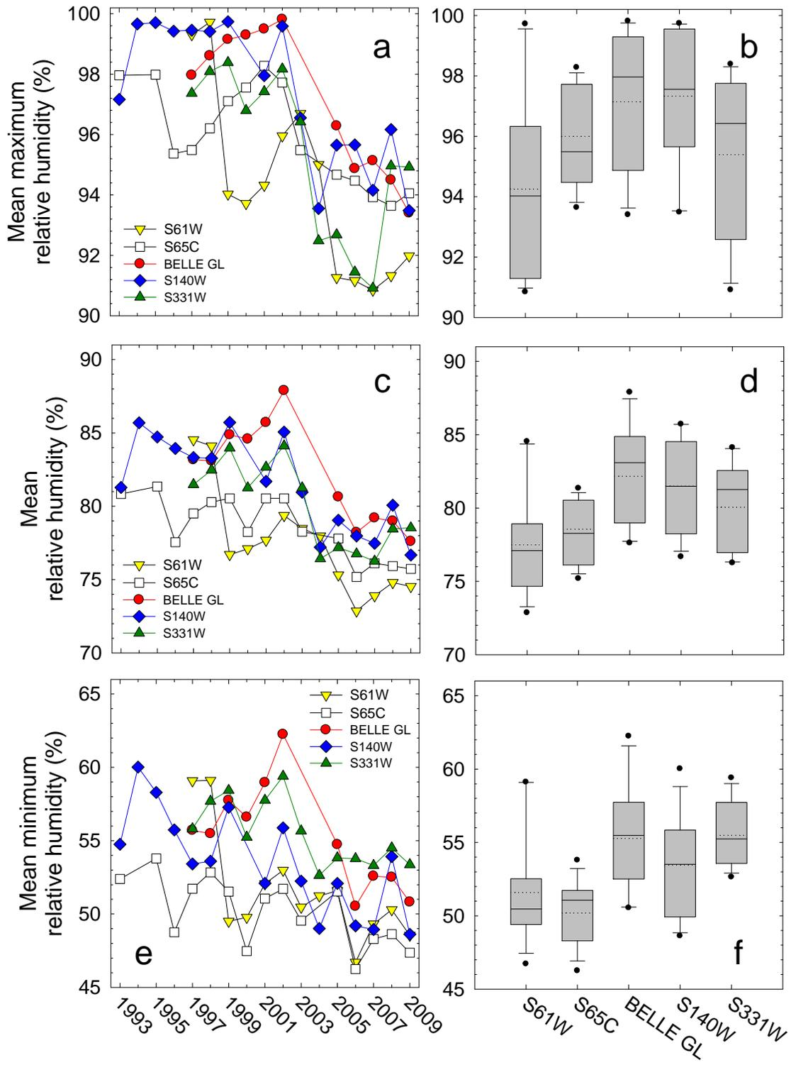
Figure 7. Mean daily maximum (a) daily mean (c) and mean daily minimum (e) relative humidity at five sites. Box plots compare mean daily maximum (b) daily mean (d) and mean daily minimum (f) relative humidity between sites. Dashed lines represent the means of the data and the solid lines represent the medians of the data for each site.
