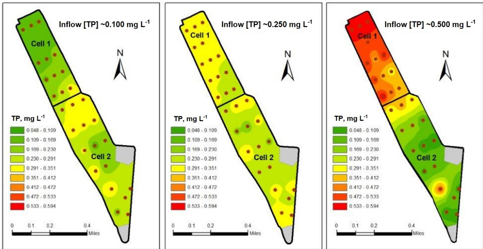
**Figure 2.** Spatial distribution of total phosphorus (TP) concentrations in the Taylor Creek STA on December 6, 2012, December 20, 2012 and September 17, 2010 at measured inflow TP concentrations of 0.101, 0.242 and 0.561  $\text{mg L}^{-1}$ , respectively.
