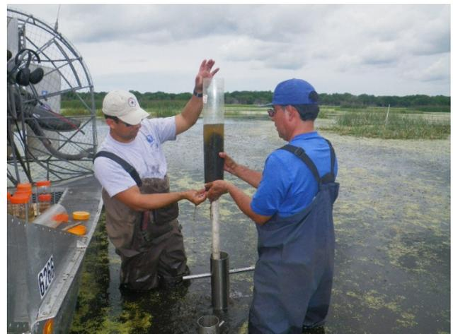
**Figure 5.** A photo of sediment collection in the field (photo by SFWMD).
