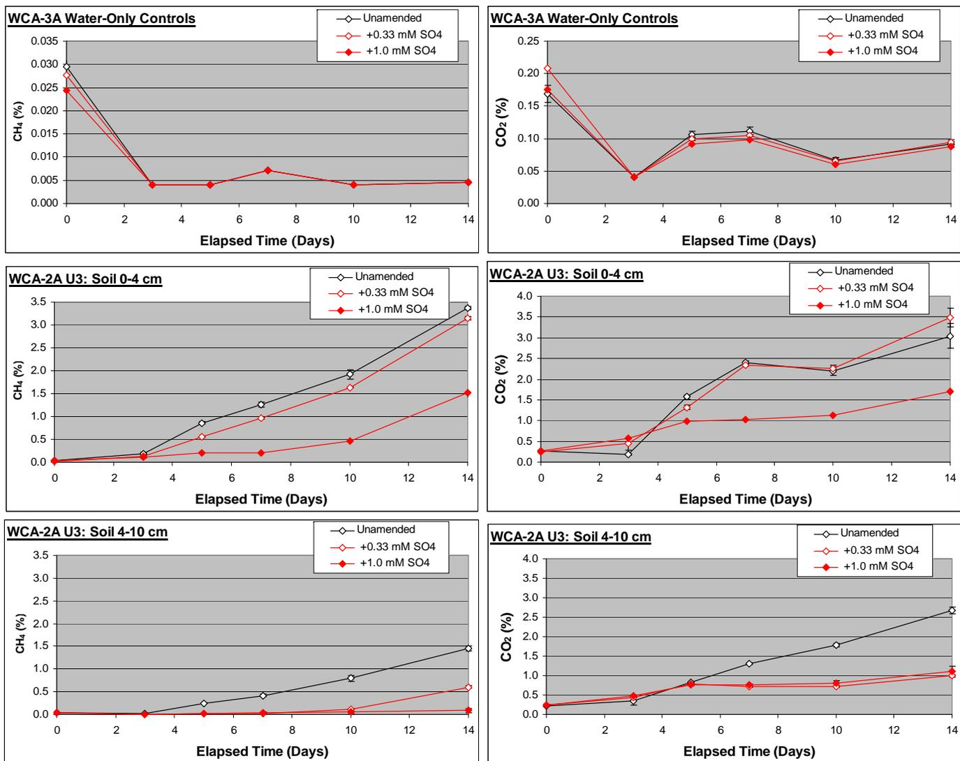
**Figure 32.** Time course of methane (CH<sub>4</sub>) and carbon dioxide (CO<sub>2</sub>) mean (n=3 ± 1 S.E.) concentrations in the headspace during anaerobic incubations of soil slurries from two horizons (0-4 and 4-10 cm) in WCA-2A U3. Each soil-less (water only) and soil slurry vessel received either 0.33 or 1.0 mM sulfate, or was not amended. Note the different Y-axis scales.
