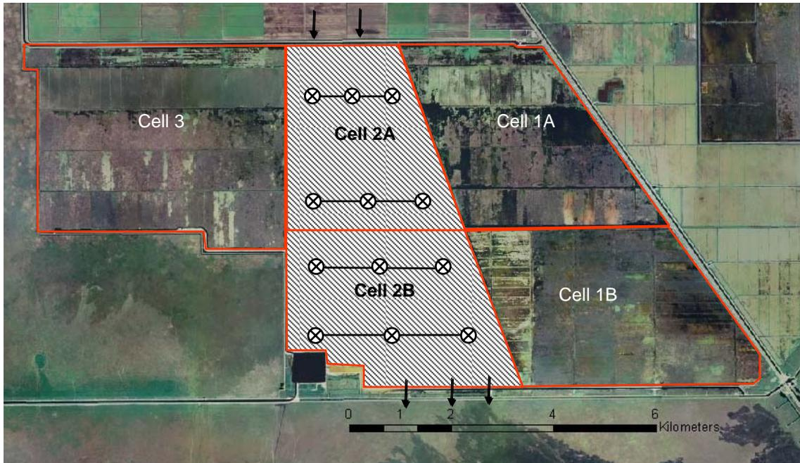
**Figure 9.** Transects selected for surface water, porewater, and sediment characterization in the STA-3/4 central flow path.
