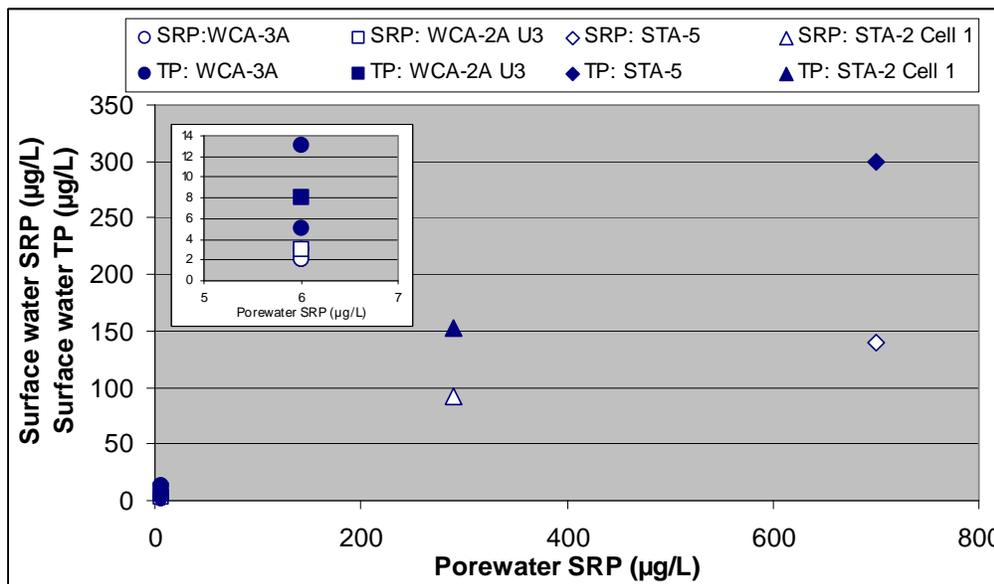
**Figure 41.** The relationship between porewater soluble reactive phosphorus (SRP) concentration, and surface water SRP and total phosphorus (TP) concentrations for the wetland soils where cores were retrieved for anaerobic incubations in the lab. Each data represent the mean of three replicate samples collected at each site.
