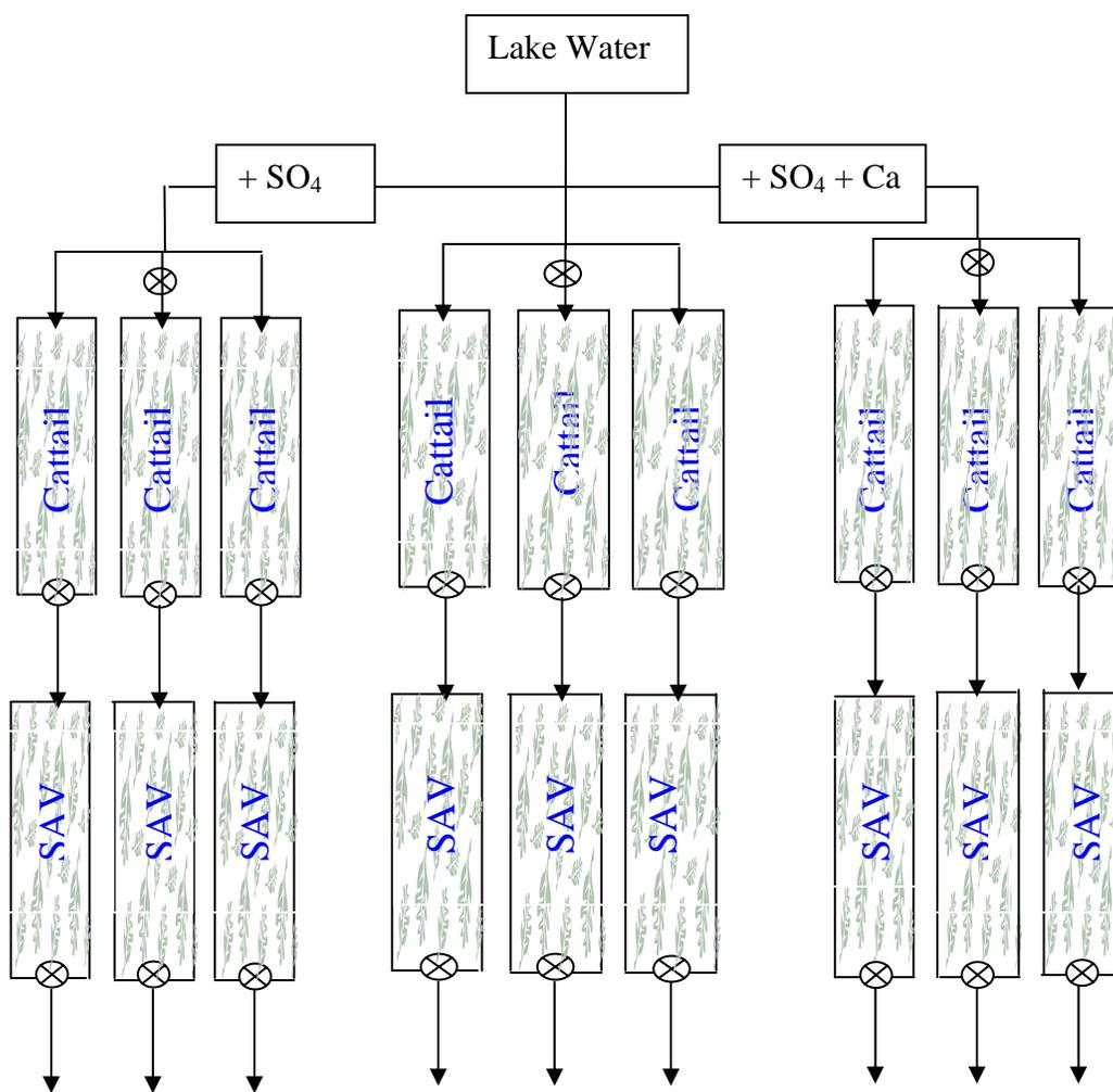
**Figure 12.** Port Mayaca two tanks-in-series flow-through mesocosms for testing effects of sulfate and calcium on phosphorus removal.
