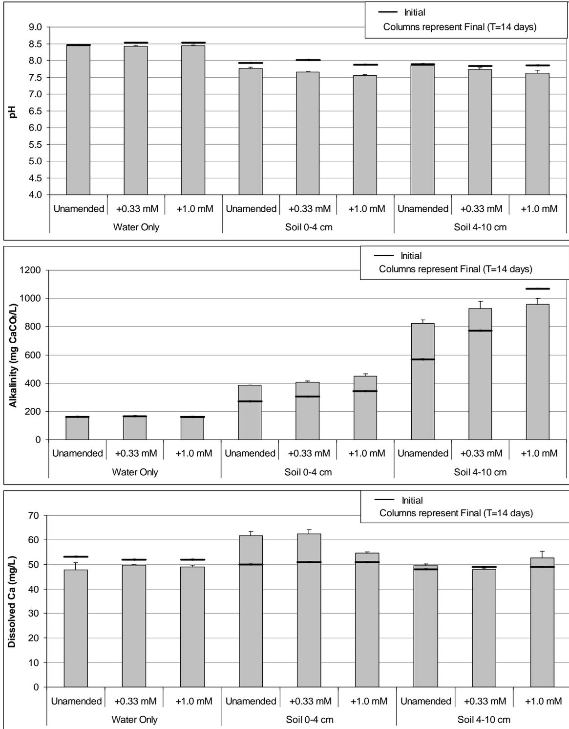
**Figure 22.** pH (top panel), alkalinity (middle panel), and dissolved calcium (Ca) (bottom panel) concentrations before and after a 14-day anaerobic incubation of soils from WCA-2A U3 with sulfate-amended (0.33 mM or 1.0 mM) and unamended WCA-3A surface water. Each data point represents the mean ( $n=3$ )  $\pm$  1 S.E. except for T=0 where a composite of two replicates were analyzed.
