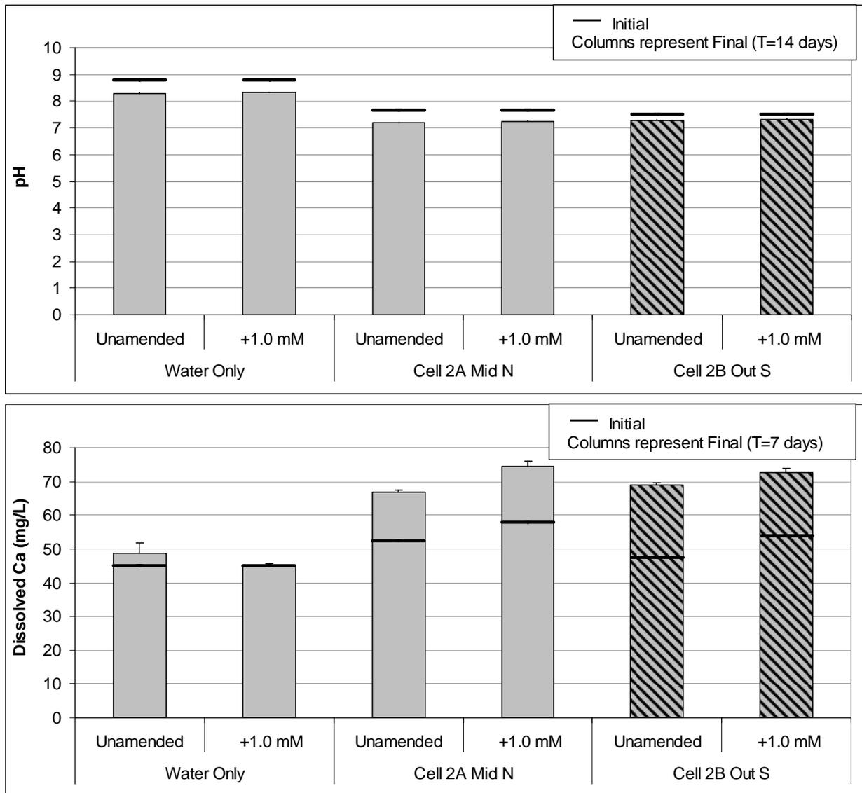
**Figure 26.** pH (top panel) and dissolved calcium (Ca) (bottom panel) concentrations before and after a 7-day anaerobic incubation of Cell 2A Mid N and Cell 2B Out S soils from STA-5 with sulfate-amended (1.0 mM) and unamended STA-5 Out surface water. Only the 0-4 cm soil layer from each location was incubated. Each data point represents the mean (n=3) ± 1 S.E. except for T=0 where a composite of two replicates were analyzed.
