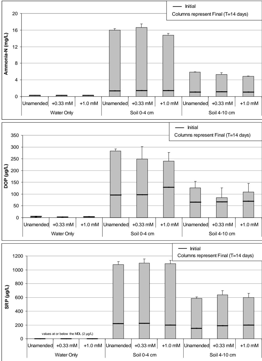
**Figure 28.** Ammonia-N (top panel), dissolved organic phosphorus (DOP) (middle panel), and soluble reactive phosphorus (SRP) (bottom panel) concentrations before and after a 14-day anaerobic incubation of soils from STA-2 Cell 1 with sulfate-amended (0.33 mM or 1.0 mM) and unamended WCA-3A surface water. Each data point represents the mean (n=3) ± 1 S.E. except for T=0 where a composite of two replicates were analyzed.
