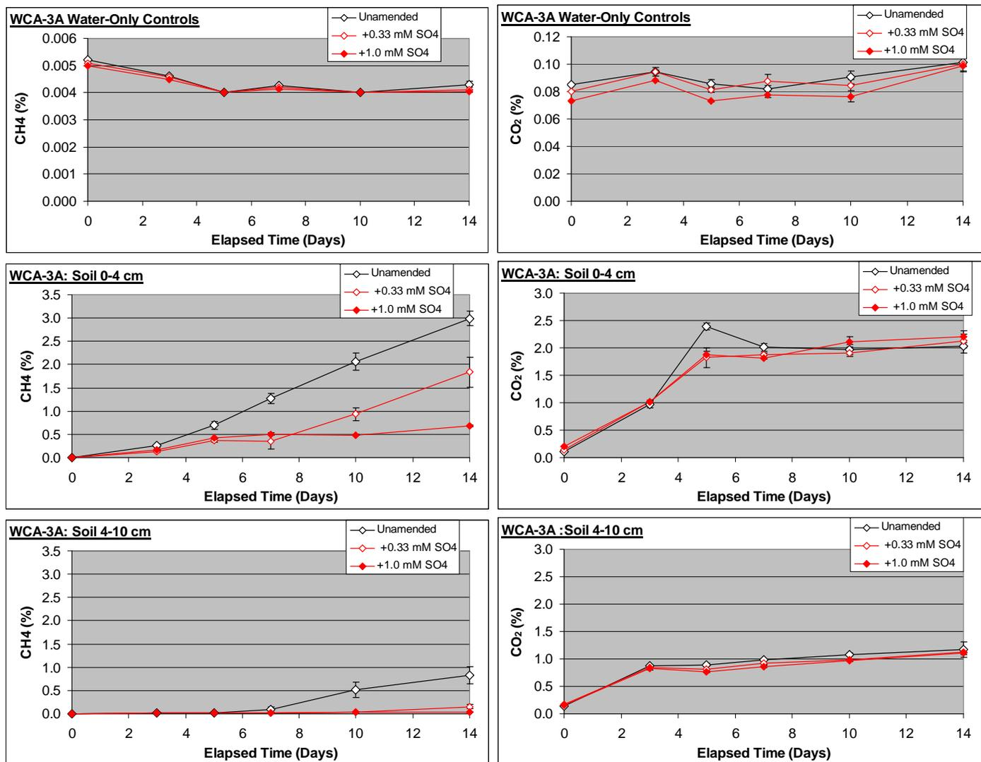
**Figure 31.** Time course of methane (CH<sub>4</sub>) and carbon dioxide (CO<sub>2</sub>) mean (n=3 ± 1 S.E.) concentrations in the headspace during anaerobic incubations of soil slurries from two horizons (0-4 and 4-10 cm) in WCA-3A. Each soil-less (water only) and soil slurry vessel received either 0.33 or 1.0 mM sulfate, or was not amended. Note the different Y-axis scales.
