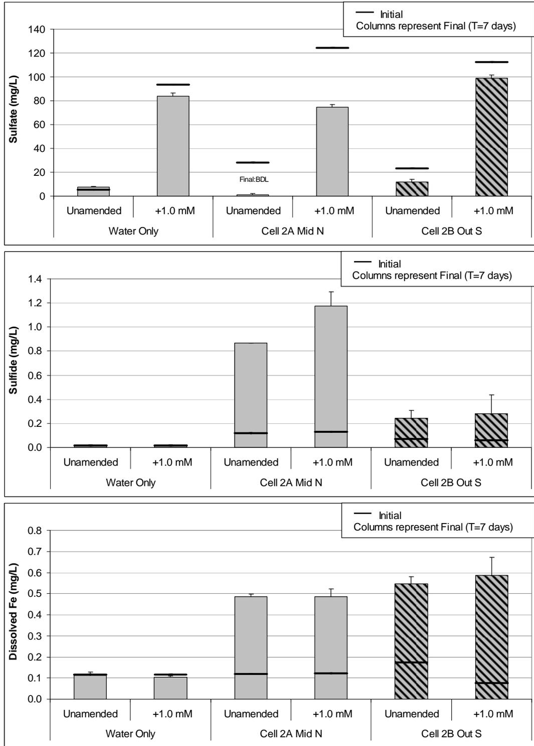
**Figure 25.** Sulfate (top panel), sulfide (middle panel), and dissolved iron (Fe) (bottom panel) concentrations before and after a 7-day anaerobic incubation of Cell 2A Mid N and Cell 2B Out S soils from STA-5 with sulfate-amended (1.0 mM) and unamended STA-5 Out surface water. Only the 0-4 cm soil layer from each location was incubated. Each data point represents the mean ( $n=3$ )  $\pm$  1 S.E. except for T=0 where a composite of two replicates were analyzed.
