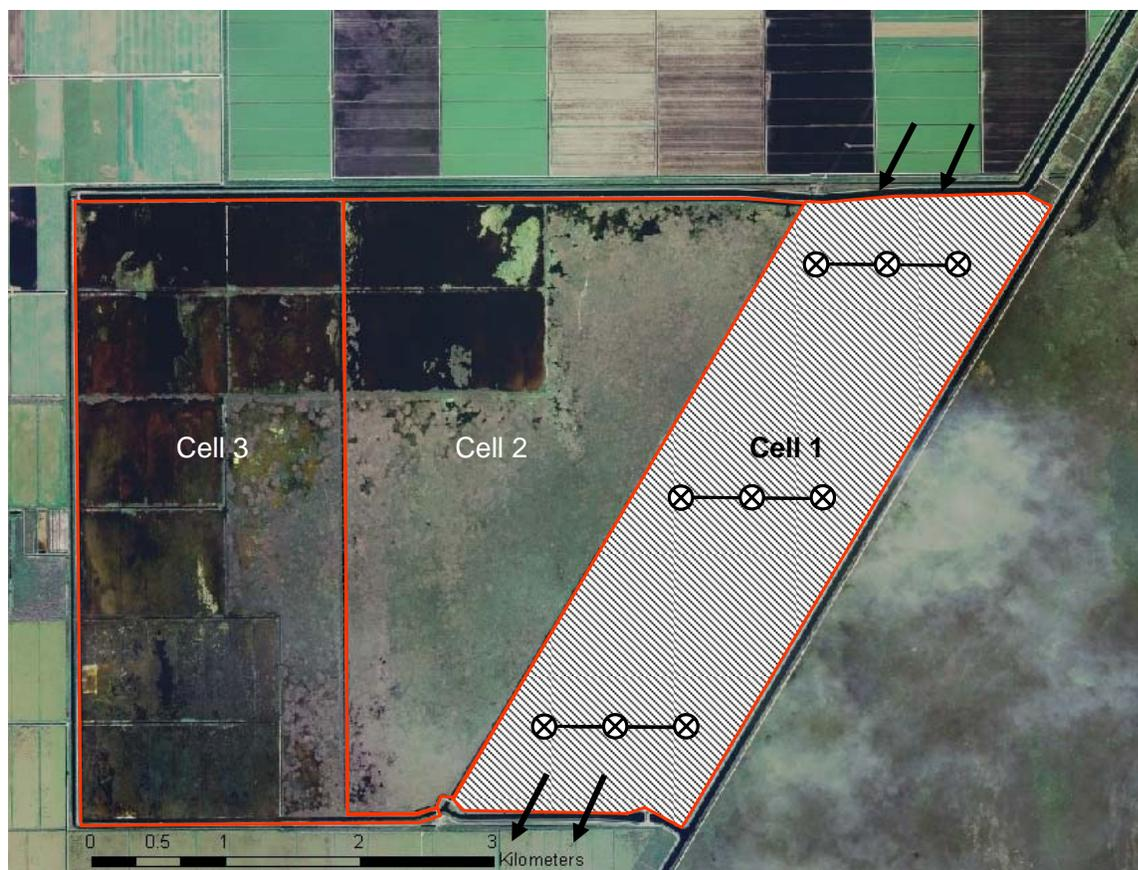
**Figure 8.** Transect locations for surface water, porewater, and sediment characterization in STA-2 Cell 1.
