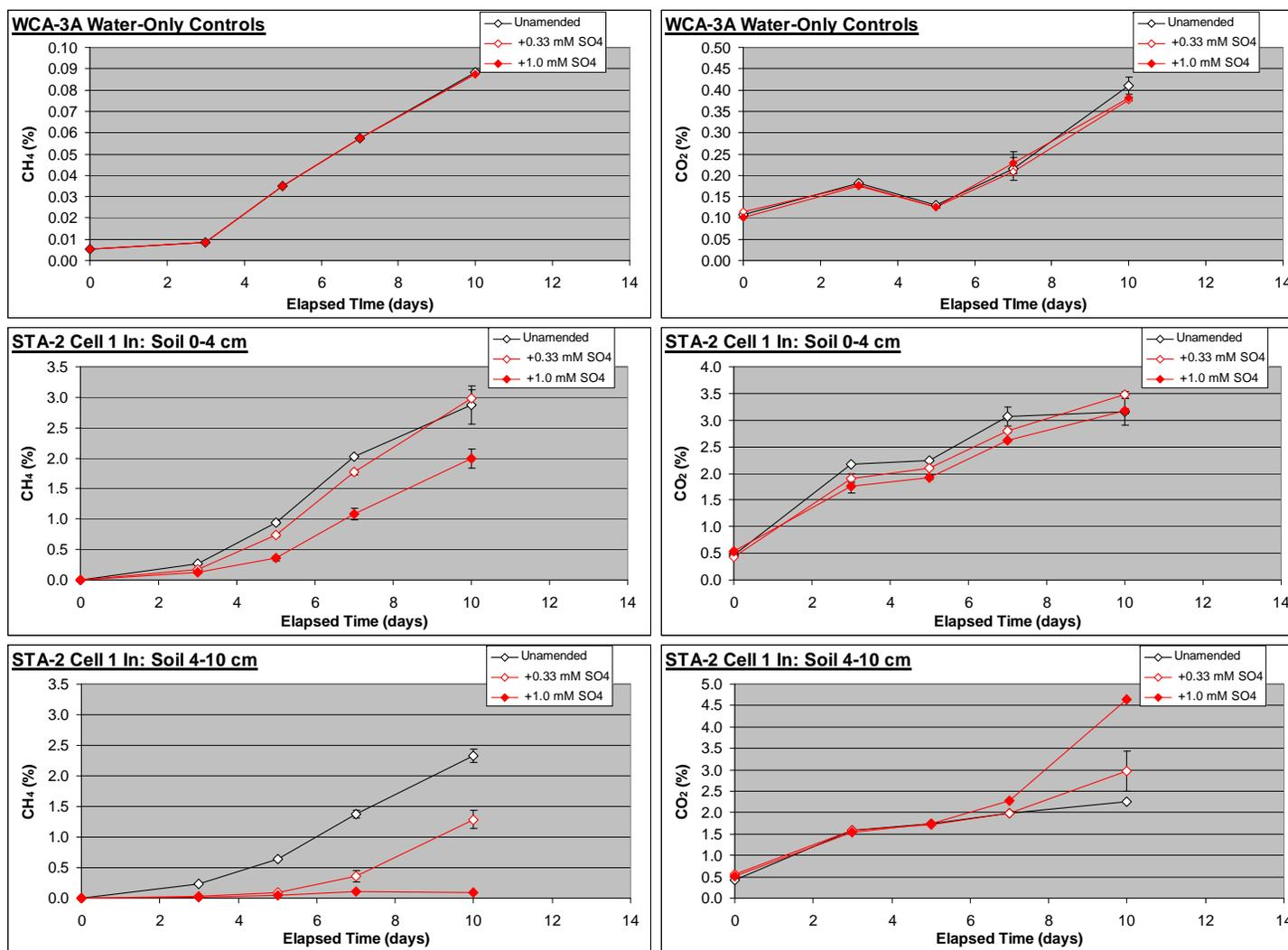
**Figure 33.** Time course of methane (CH<sub>4</sub>) and carbon dioxide (CO<sub>2</sub>) mean ( $n=3 \pm 1$  S.E.) concentrations in the headspace during anaerobic incubations of soil slurries from two horizons (0-4 and 4-10 cm) in STA-2 Cell 1 In. Each soil-less (water only) and soil slurry vessel received either 0.33 or 1.0 mM sulfate, or was not amended. The sampling period covered only 10 instead of 14 days due to a technical difficulty. Note the different Y-axis scales.
