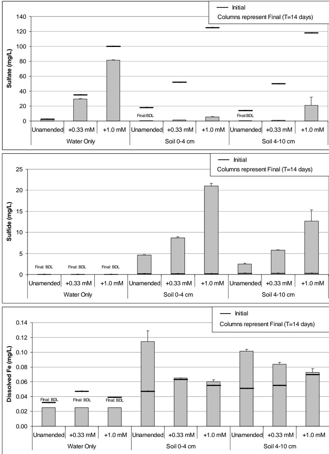
**Figure 29.** Sulfate (top panel), sulfide (middle panel), and dissolved iron (Fe) (bottom panel) concentrations before and after a 14-day anaerobic incubation of soils from STA-2 Cell 1 with sulfate-amended (0.33 mM or 1.0 mM) and unamended WCA-3A surface water. Each data point represents the mean ( $n=3$ )  $\pm$  1 S.E. except for T=0 where a composite of two replicates were analyzed.
