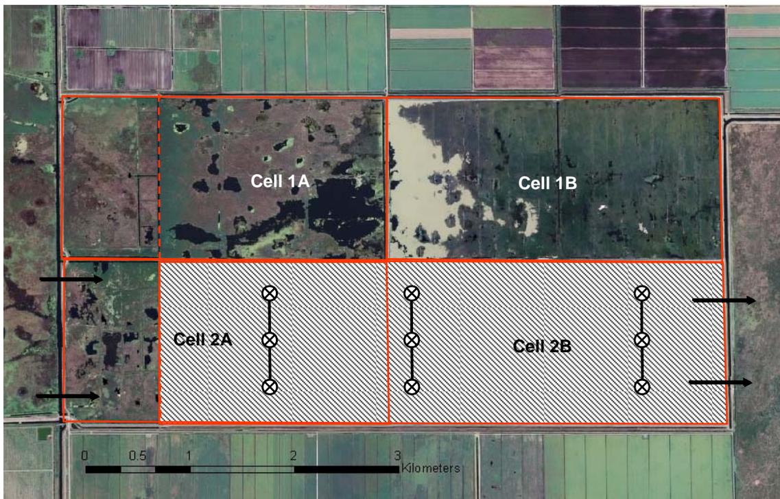
**Figure 10.** Transect locations for surface water, porewater, and sediment characterization in the STA-5 central flow path.
