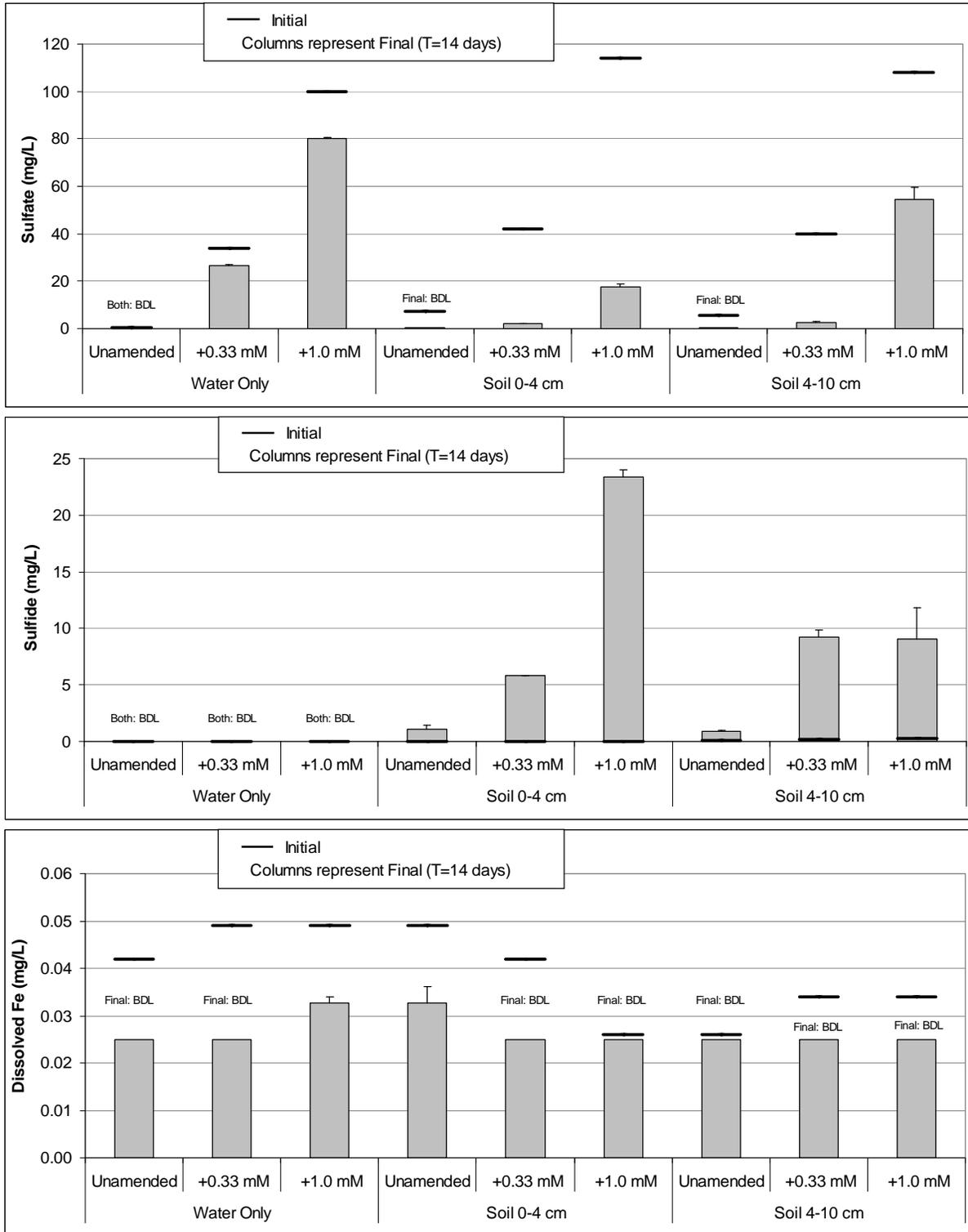
**Figure 21.** Sulfate (top panel), sulfide (middle panel), and dissolved iron (Fe) (bottom panel) concentrations before and after a 14-day anaerobic incubation of soils from WCA-2A U3 with sulfate-amended (0.33 mM or 1.0 mM) and unamended WCA-3A surface water. Each data point represents the mean ( $n=3$ )  $\pm$  1 S.E. except for T=0 where a composite of two replicates were analyzed.
