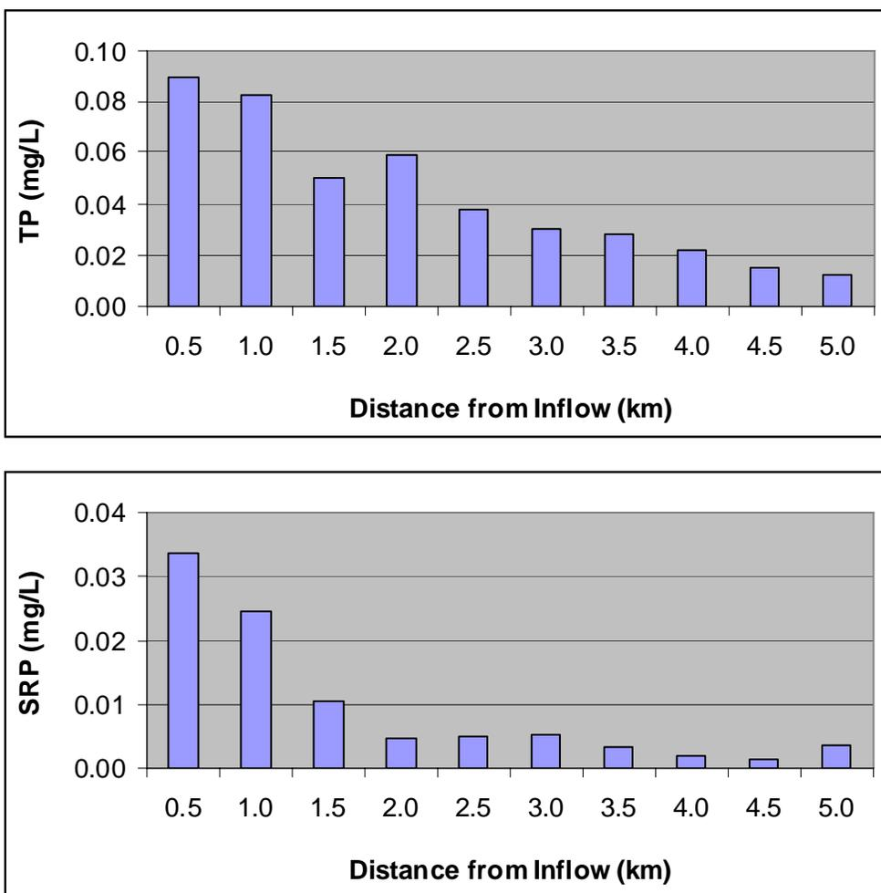
**Figure 6.** Total (TP) and soluble reactive phosphorus (SRP) concentration gradients along the flow-path in STA-2 Cell 1. The values represent the mean of two sampling events (6/21/07 and 9/28/07).
