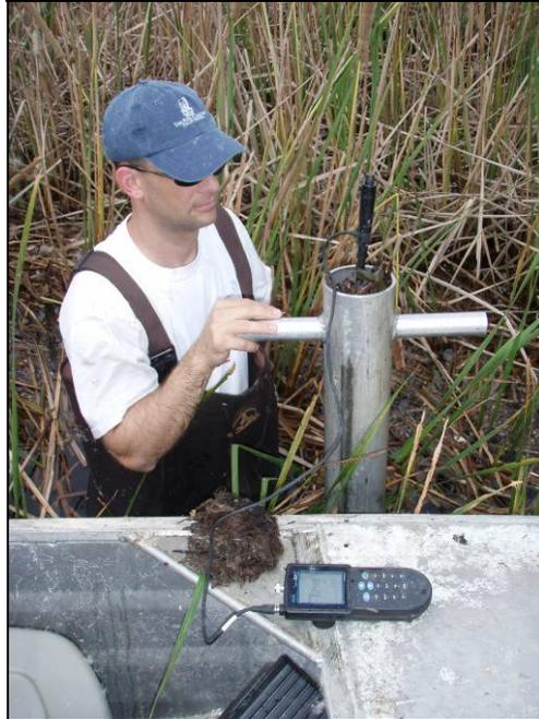
**Figure 7.** Measuring redox potential in a soil core from the inflow region of STA-2 Cell 1 on June 2, 2009.
