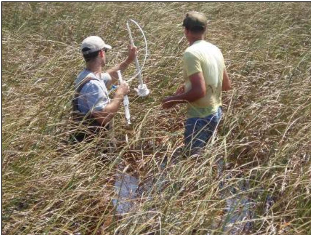
**Figure 8.** Deployment of the “sipper” for sampling pore waters at the ridge location in WCA-3A on September 19, 2008.
