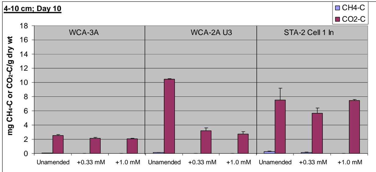
**Figure 34.** The mass of methane (CH<sub>4</sub>) and carbon dioxide (CO<sub>2</sub>) mineralized per initial dry weight of soil in the 0-4 cm (top panel) and 4-10 cm (bottom panel) soil layers of WCA-3A, WCA-2A U3, and STA-2 Cell 1 In after 10 days of anaerobic incubation. Each soil layer was either unamended or amended with 0.33 mM (32 mg/L) or 1.0 mM (96 mg/L) sulfate. Each column represents the mean (n=3) and 1 S.E.
