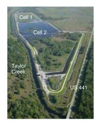
cells are controlled by individual gated structures located at the southerly end of each cell.
