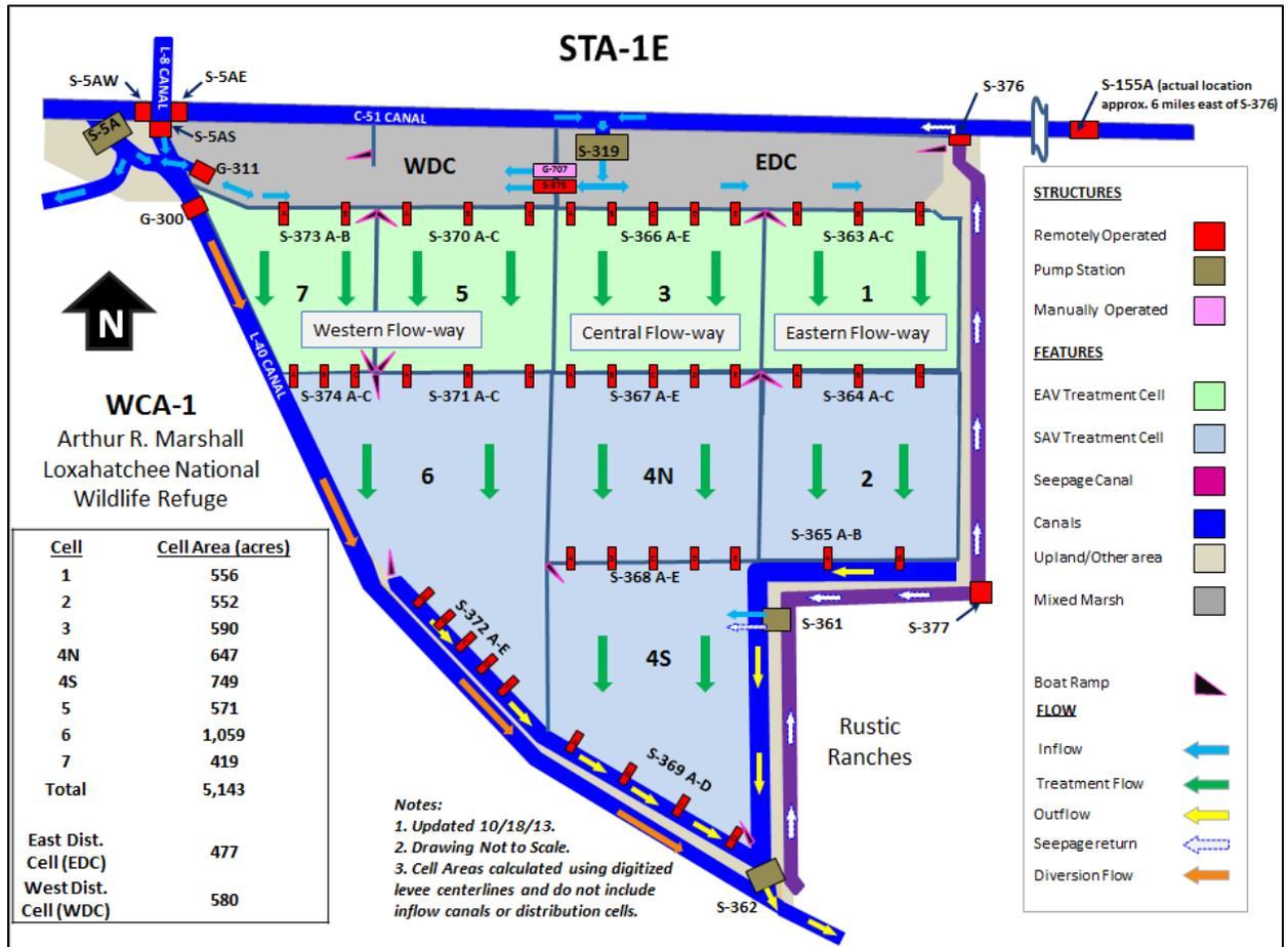
Figure 1. STA-1E Schematic\*
