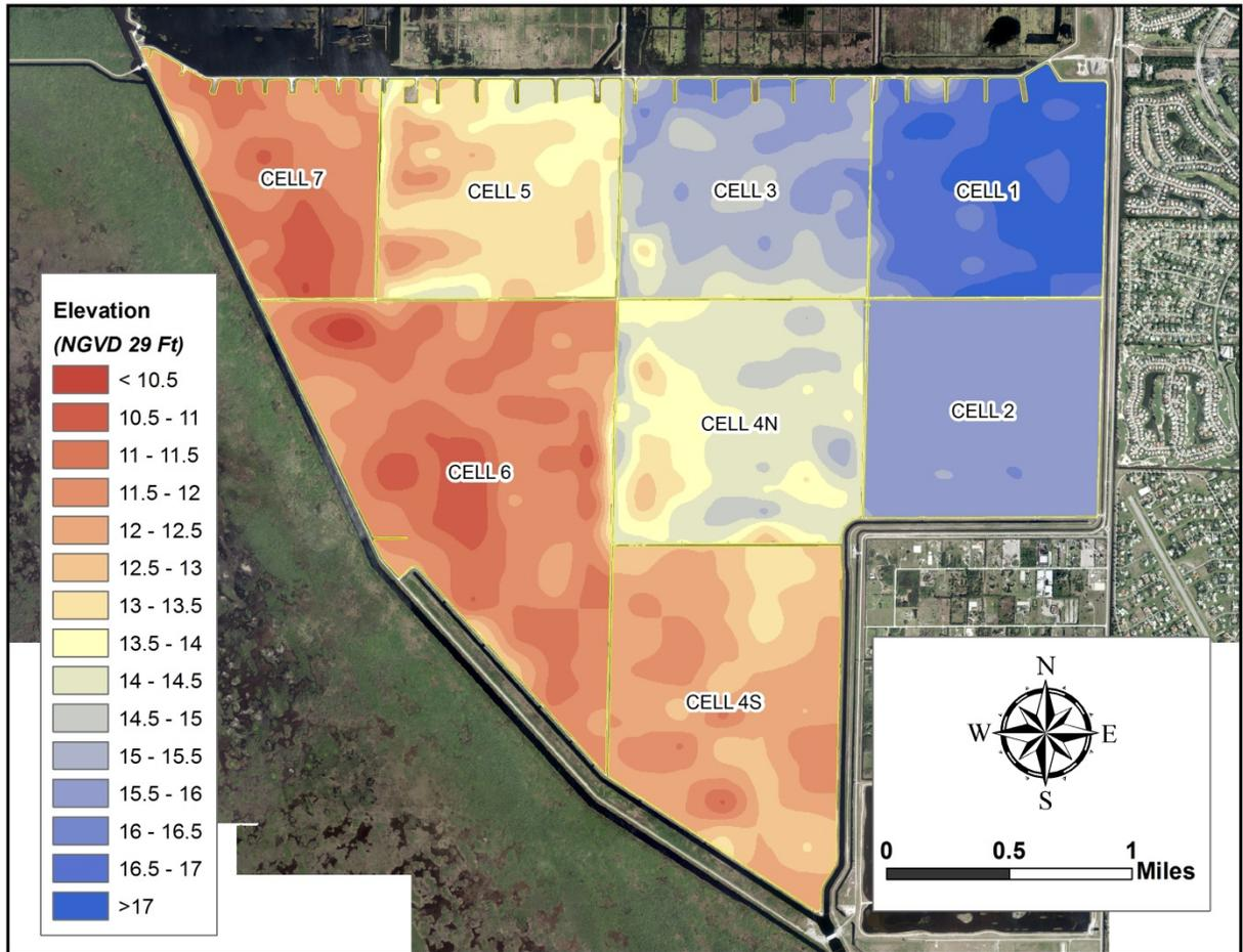
**Figure 6. STA-1E DEM based on 2005 and 2014 Topographic Survey Data\***
