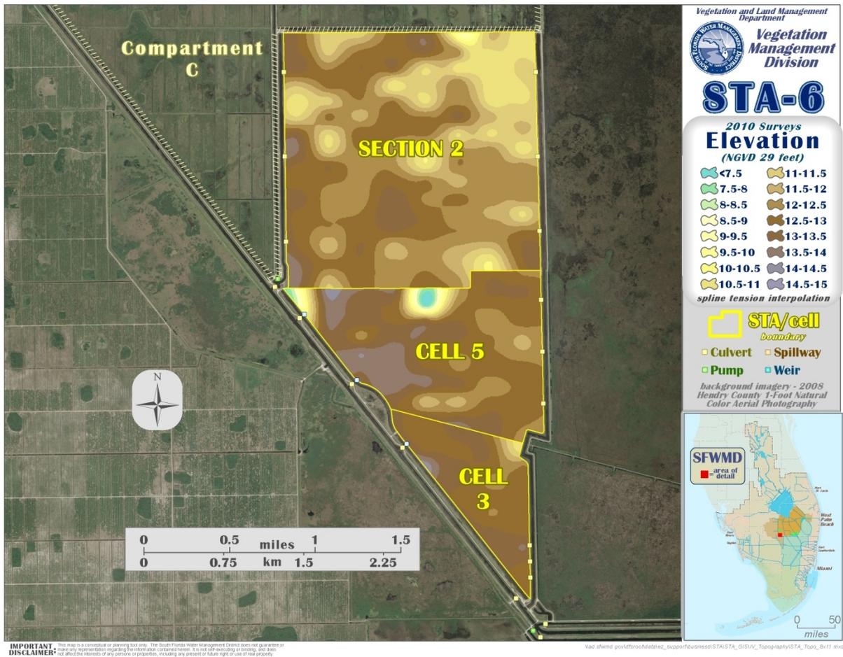
**Figure 11. STA-6 DEM based on 2010 Topographic Survey Data**
