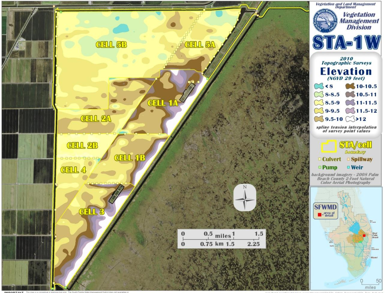
**Figure 7. STA-1W DEM based on 2010 Topographic Survey Data**
