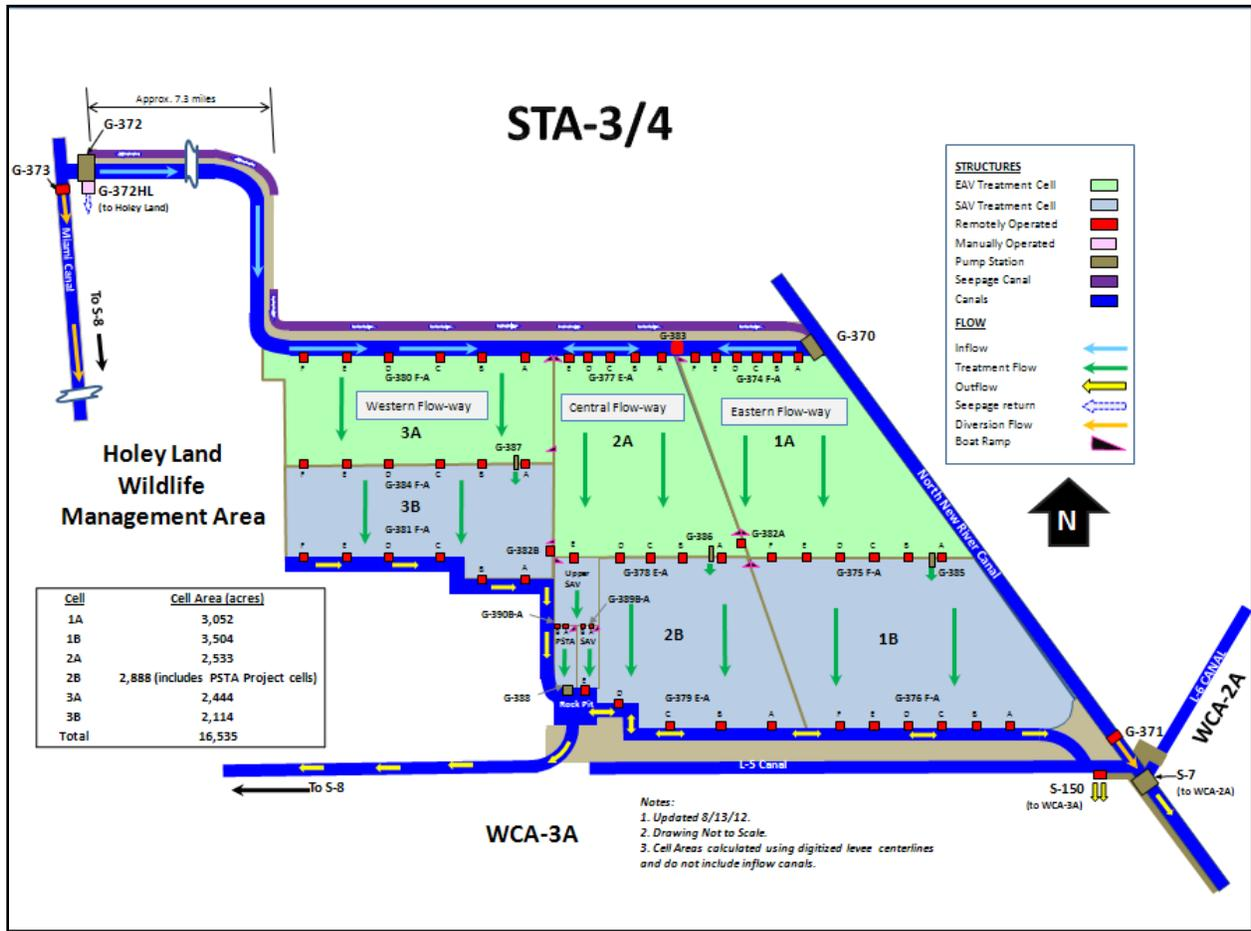
**Figure 4. STA-3/4 Schematic**
