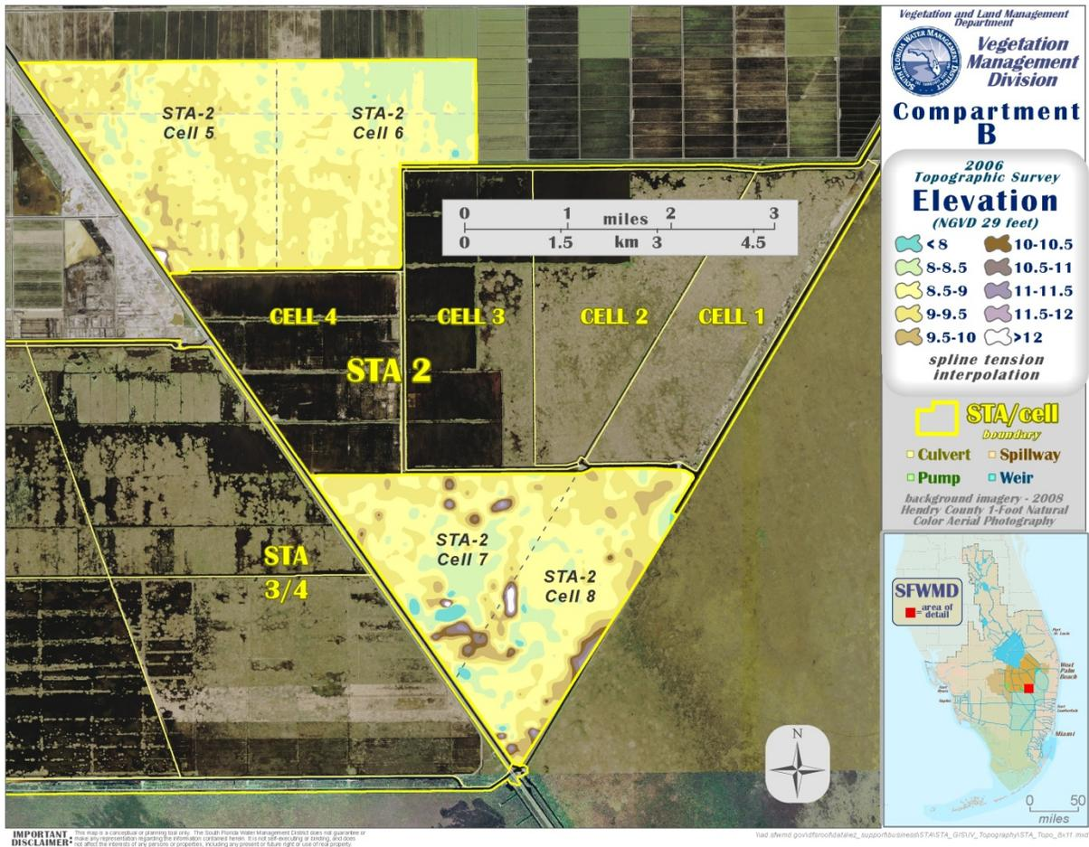
**Figure 12. Compartment B\* DEM based on 2006 Topographic Survey Data**
