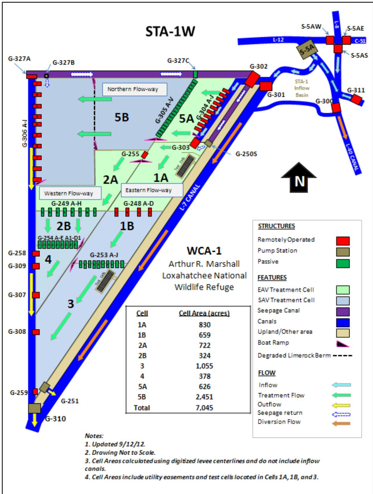
Figure 2. STA-1W Schematic
