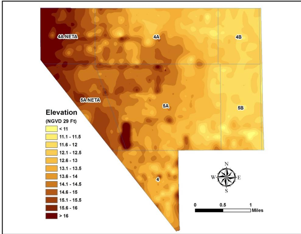
**Figure 13. Compartment C\* DEM based on 2006 Topographic Survey Data
