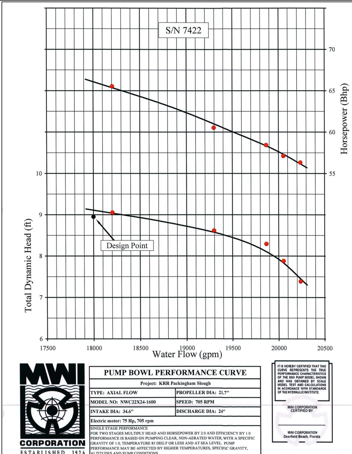
Figure 4. Pump Performance Curve for Pump Station G700
