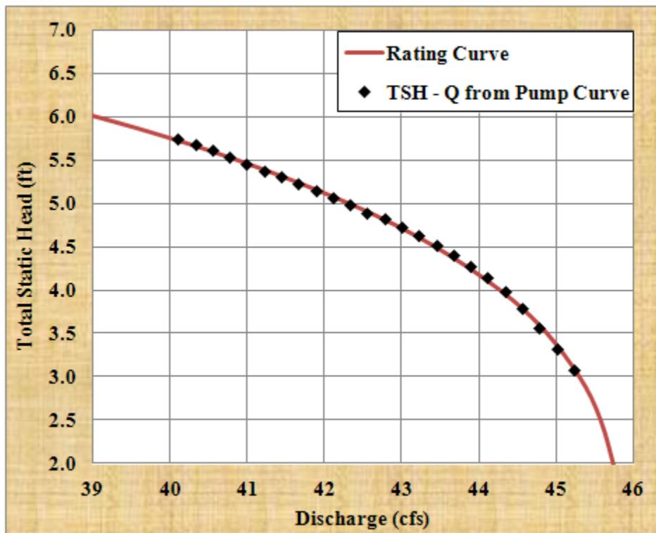
**Figure 5. Flow Rating Curve for Pump Station G700**
