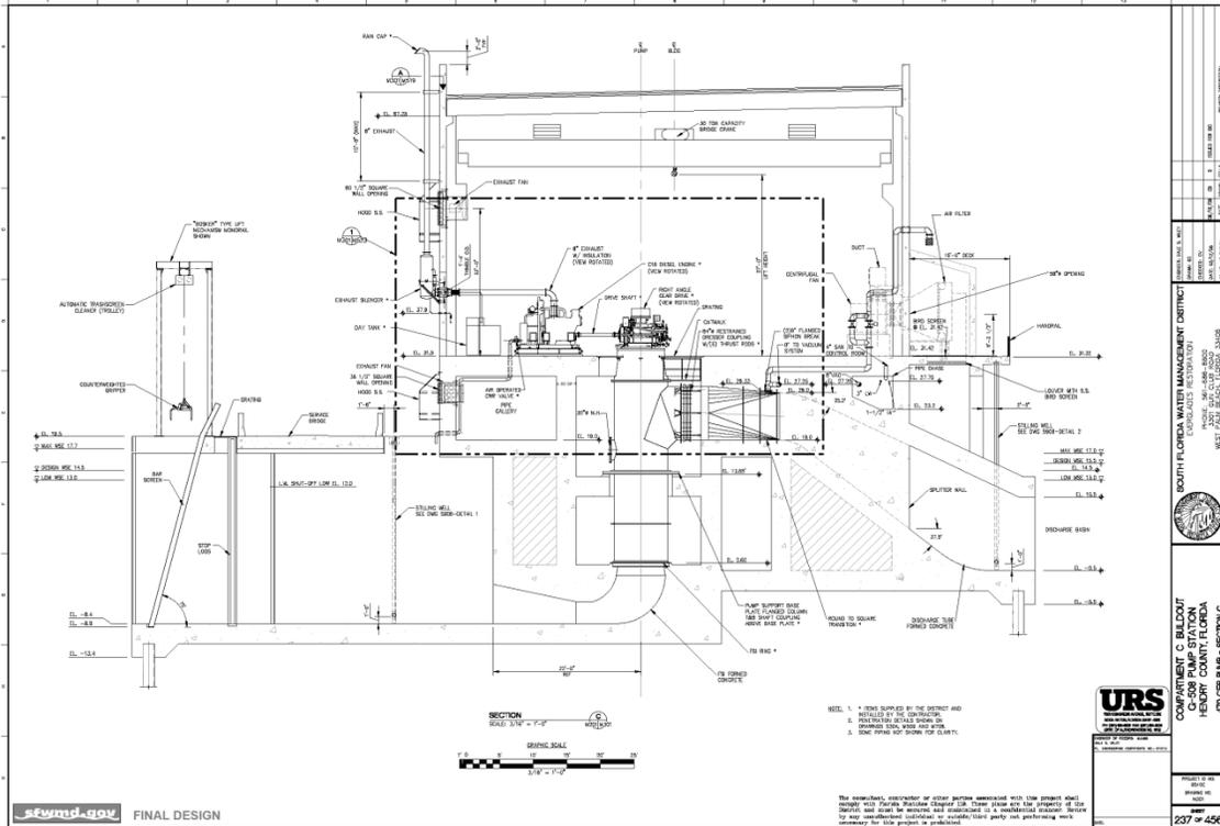
Figure 3a. Profile view of G508 main inflow pump – 470 cfs
