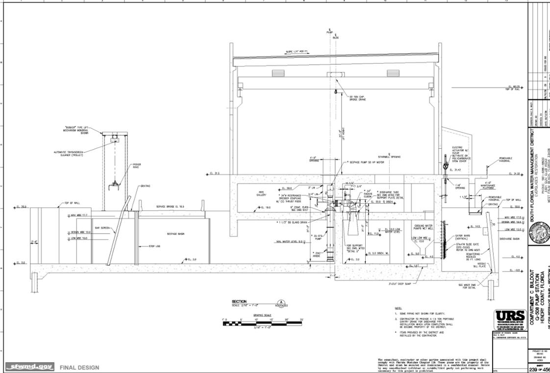
Figure 3c. Profile view of G508 seepage pump – 25 cfs
