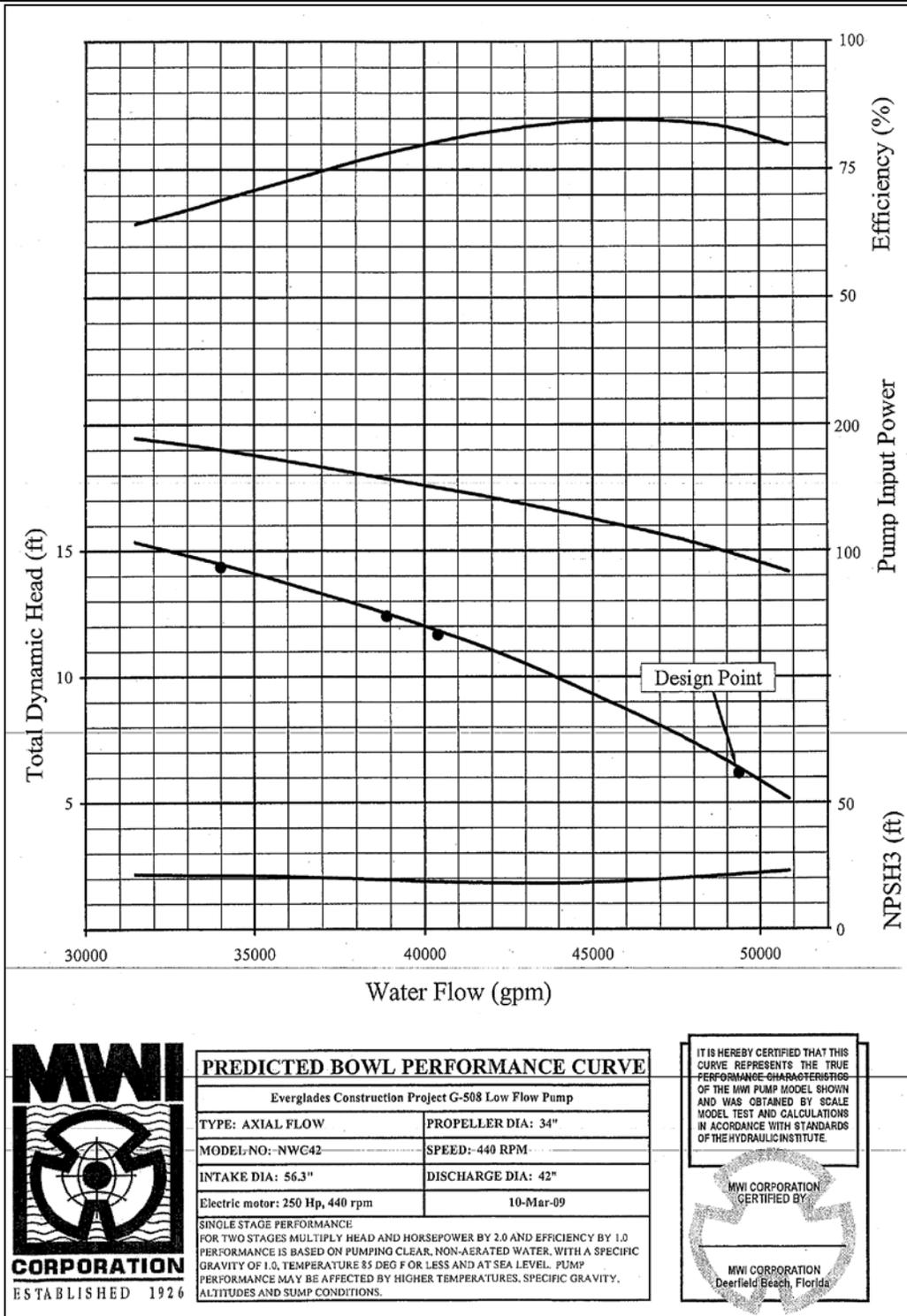
Figure 5. Pump performance curve for G508 electric low inflow pump of 110 cfs
