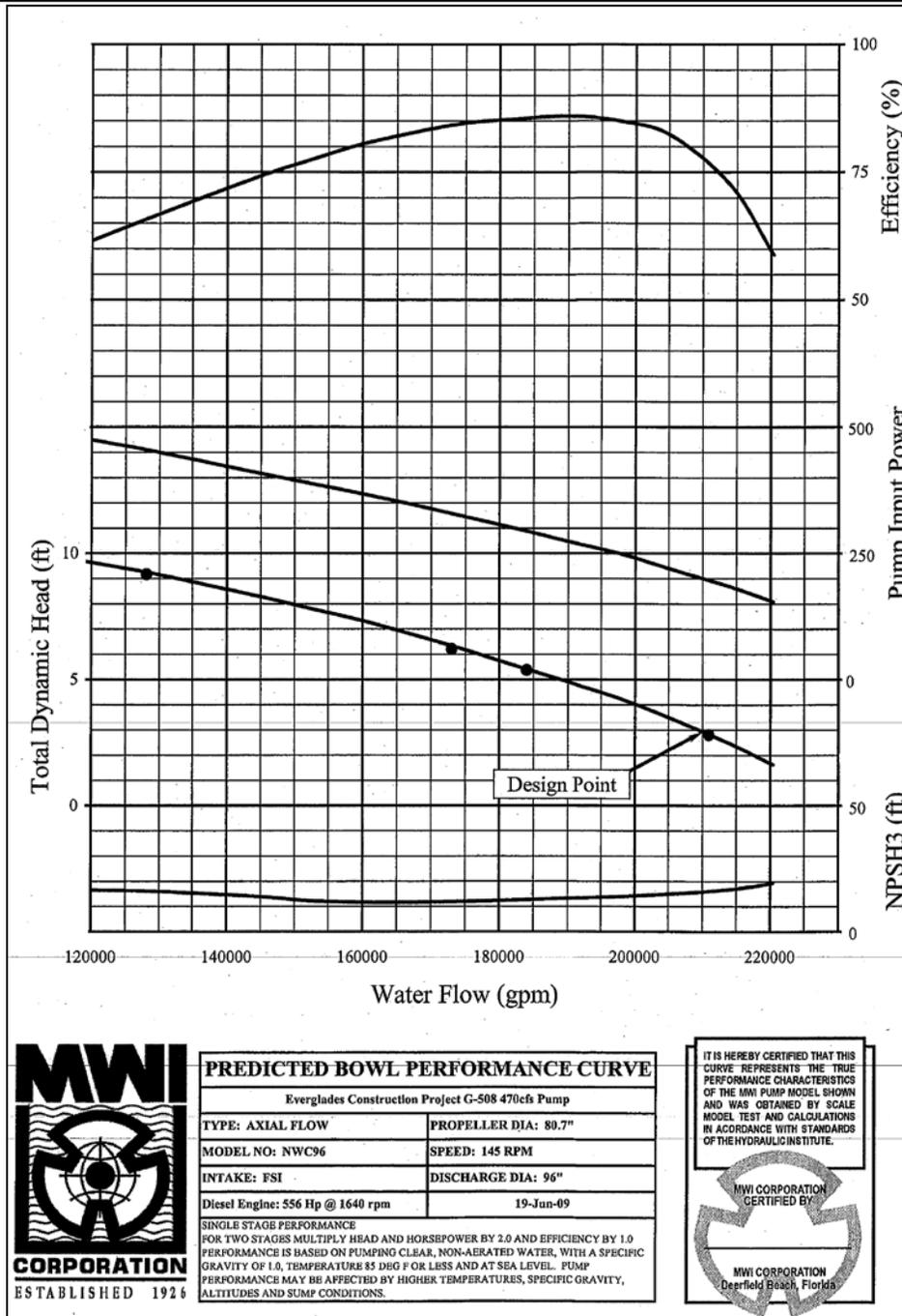
Figure 4. Pump performance curve for G508 diesel main inflow pump of 470 cfs
