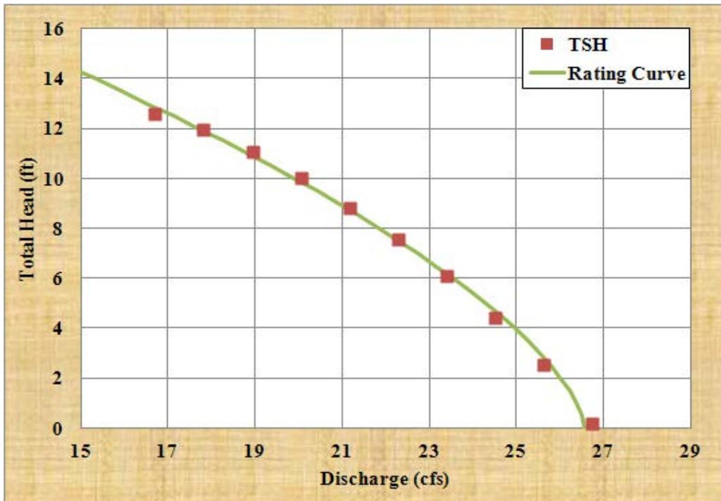
Figure 9. Flow rating curve for G508 electric seepage pump
