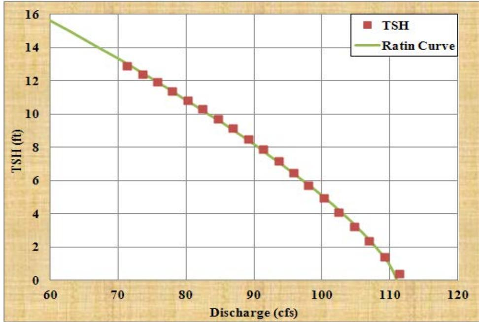
Figure 8. Flow rating curve for G508 electric low inflow pump
