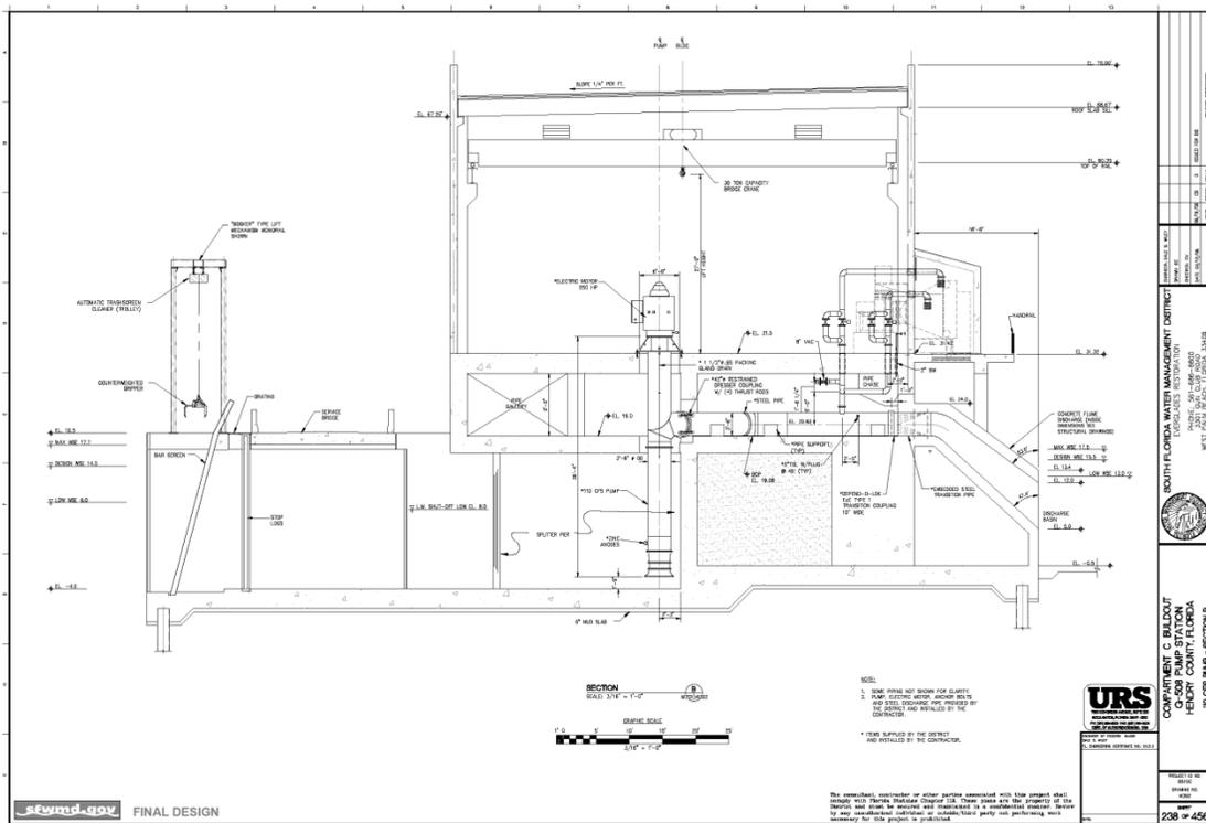
Figure 3b. Profile view of G508 low inflow pump – 110 cfs
