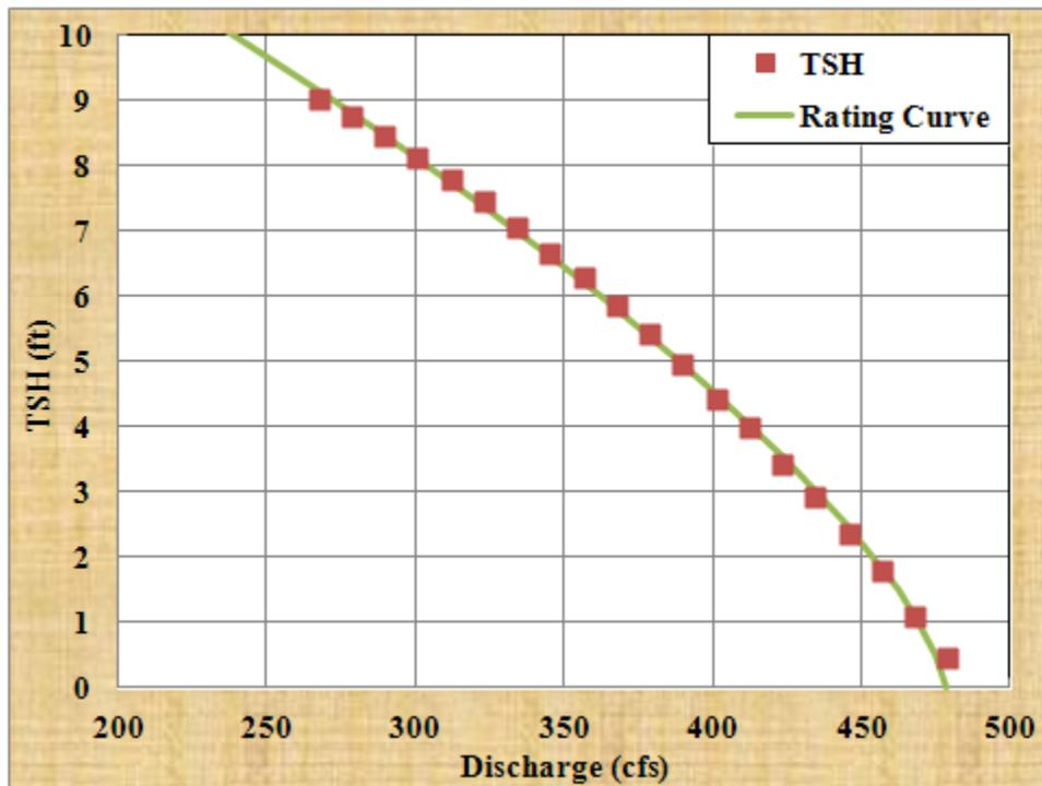
**Figure 7.** Flow rating curve for G508 diesel main inflow pump
