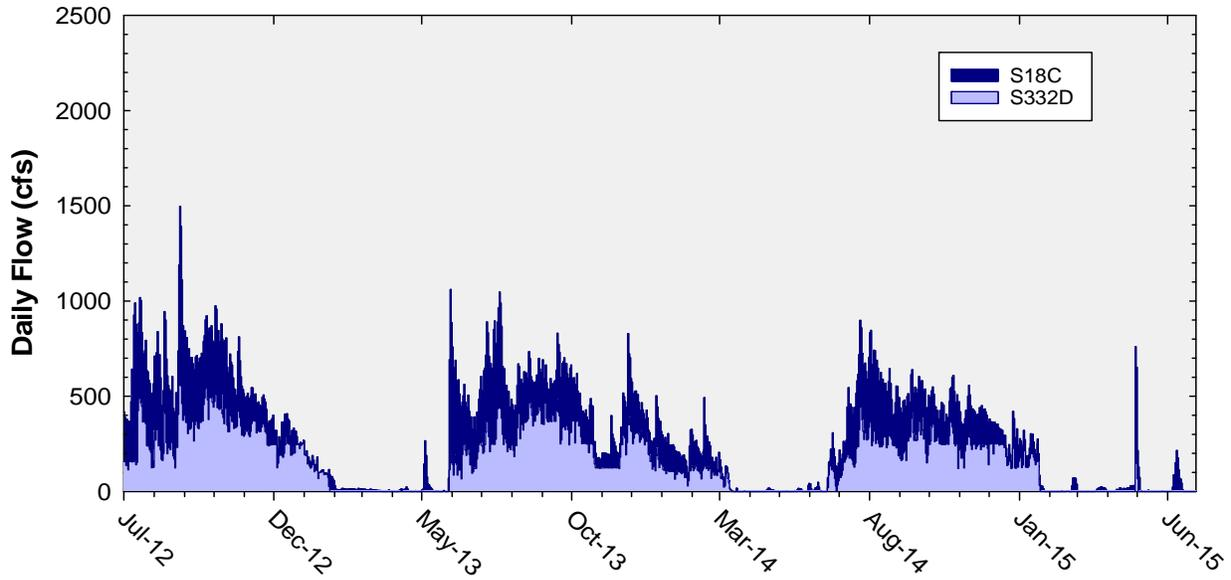
**Figure 7.** Daily flows measured in cubic feet per second (cfs) into ENP as a stacked sum of Taylor Slough (structure S332D) and Coastal Basins (structure S18C).
