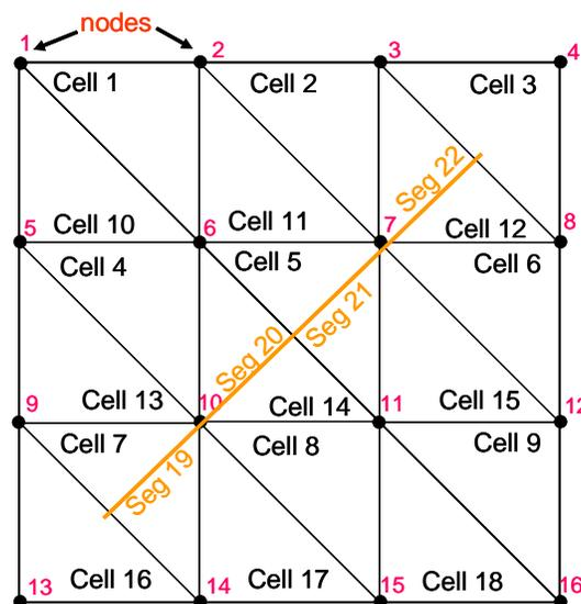
Figure 1.2 Standard 3x3 mesh and four-segment canal for benchmarks
