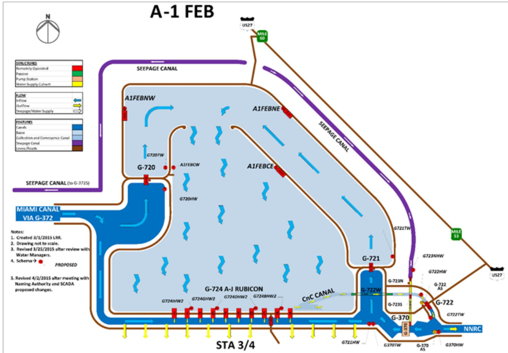
Figure B-7. A-1 Flow Equalization Basin (FEB) schematic showing configurations of basin, canals, flow direction, and locations of flow structures.
