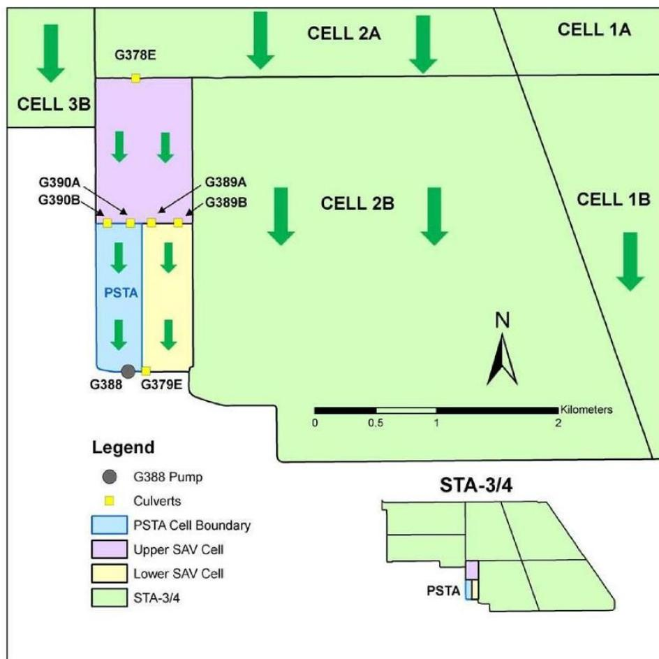
Figure A-1. Schematic of the PSTA project in the western portion of Cell 2B of STA-3/4.
