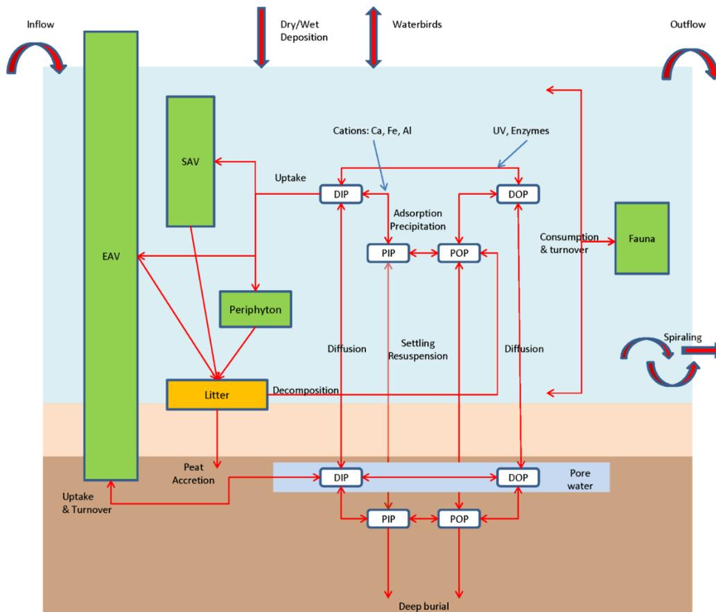
Figure 3-1. Schematic of chemical, physical, and biological processes that can influence changes in P concentrations between the soil and water column.
