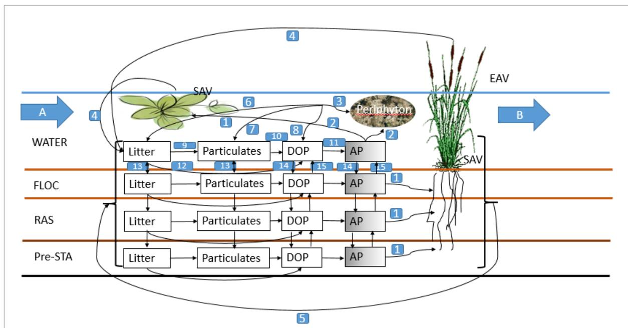
Figure 3-4. Conceptual model with state variables and fluxes to be incorporated into a numerical framework. The figure depicts a length segment within an STA cell. The state variables are operating in four domains: water, floc, recently accreted soil (RAS), and pre-STA soil.
