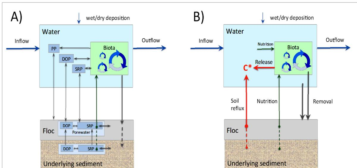
Figure 3-3. Aggregated (A) and highly aggregated (B) conceptual diagrams of P cycling in STA systems. Lowest achievable TP concentrations from the STAs ( $C^*$ ) likely are limited by internal loading from soil (e.g., diffusive fluxes, storages; indicated in red) and biotic sources (e.g., SAV biomass turnover, phytoplankton production; indicated in green). The soil matrix is shown partitioned into upper and lower layers.
