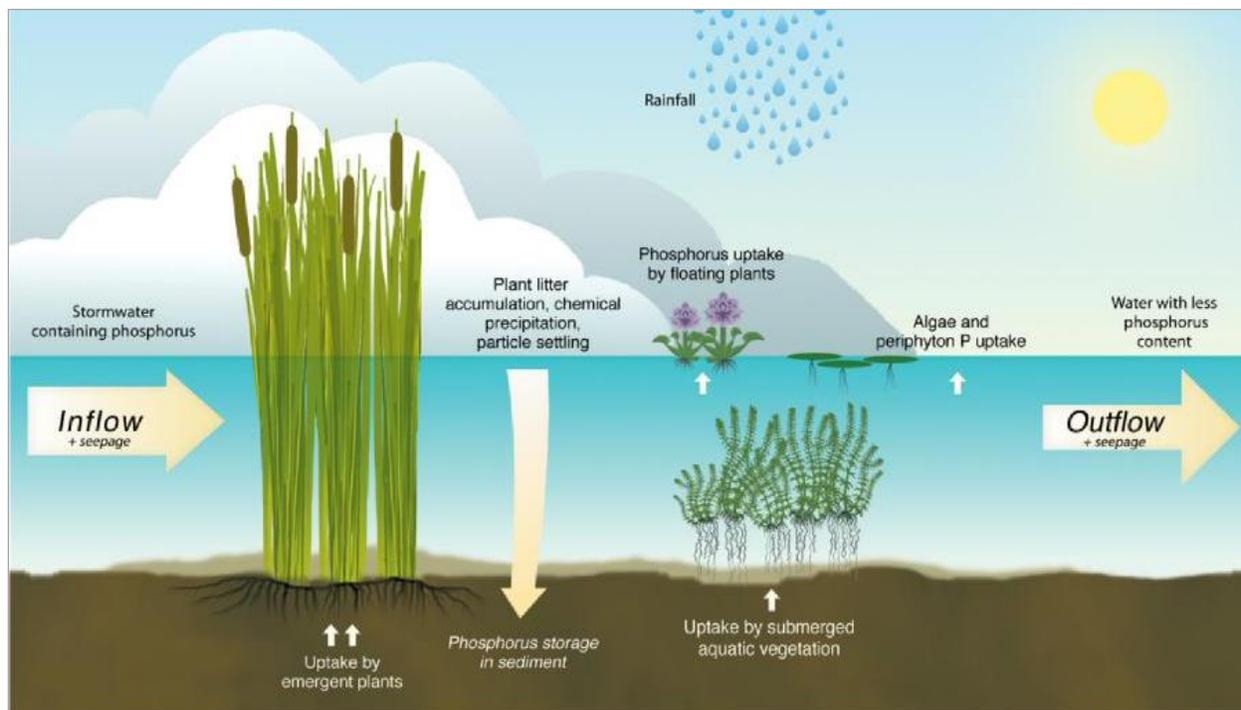
Figure 2-2. Schematic of phosphorus (P) retention process and mechanisms in the STAs.
