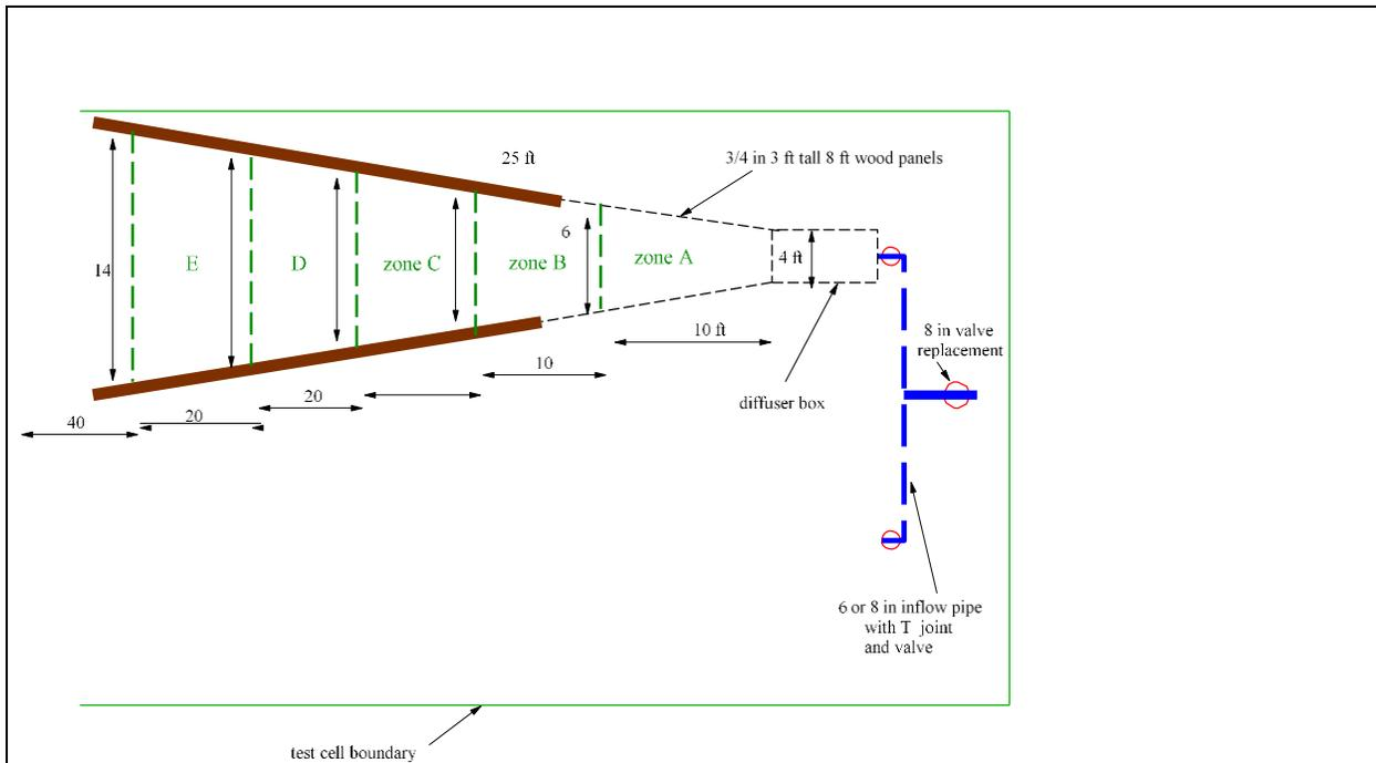
Figure A-2. Schematic of V-shaped treatment channel to be used in the Sustainable Landscape and Treatment in a Stormwater Treatment Area study.
