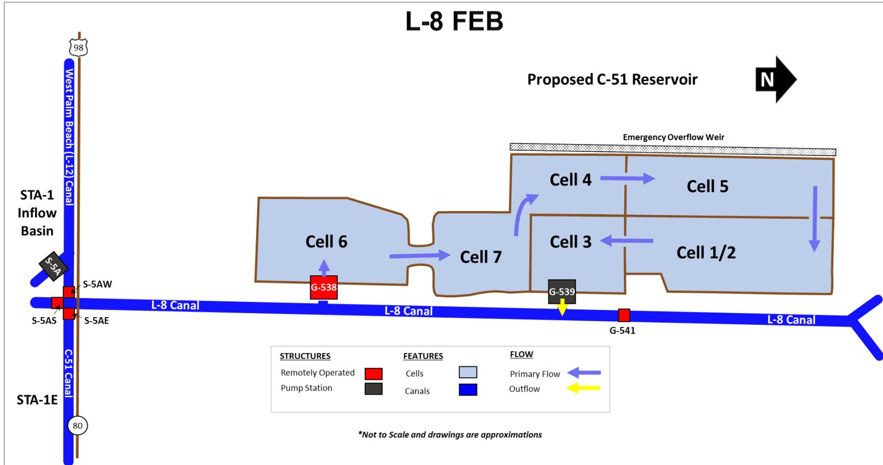
Figure B-6. L-8 Flow Equalization Basin (FEB) schematic showing configurations of cells, flow direction, and locations of flow structures.
