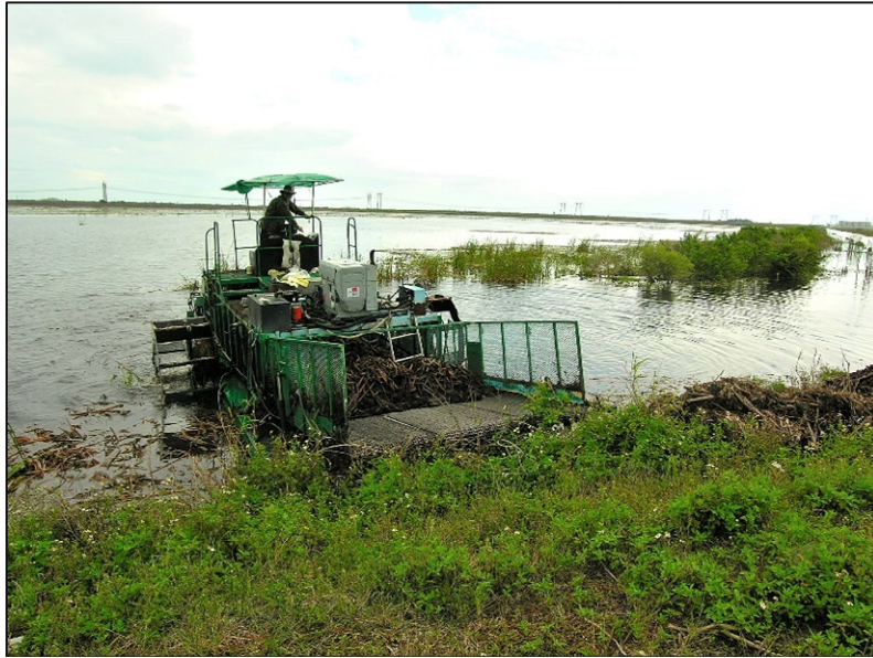
Figure 7. Decaying vegetation harvesting in STA-1W Cell 3 on July 1, 2008.
