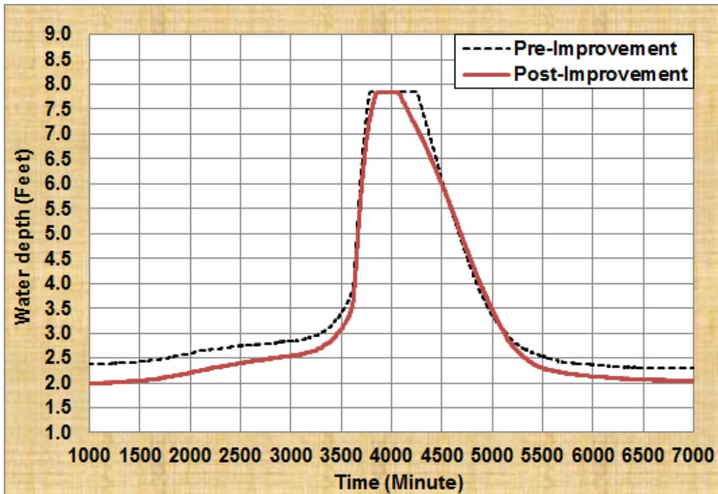
Figure 19d. Water Depth in C-Imp1-1E for Pre- and Post-Improvements
