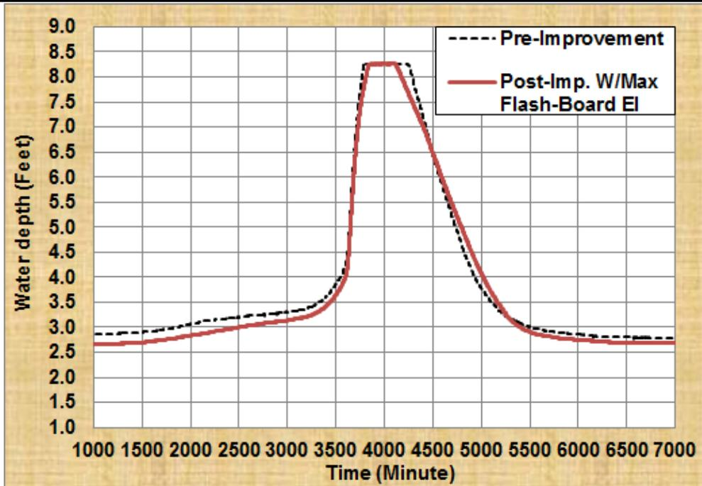
Figure 25c. Water Depth in C-Imp1S-2 for Pre-Improvement and Post-Improvement with Maximum Flash-board Elevation for the 25-year, 3-Day Design Storm
