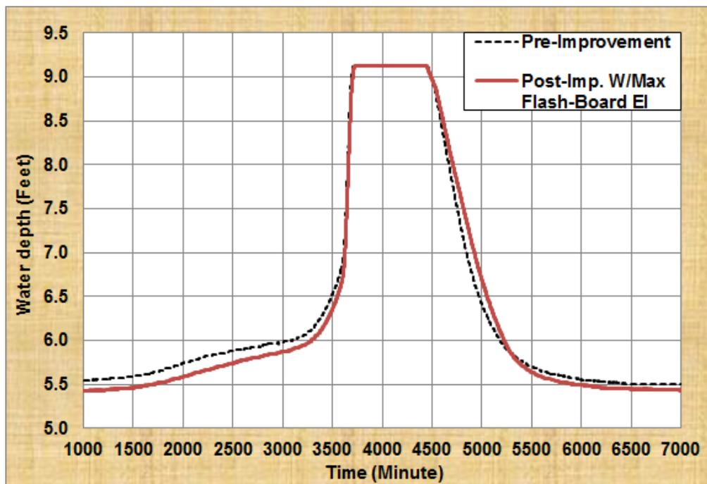
Figure 25f. Water Depth in C-Imp1S-Store for Pre-Improvement and Post-Improvement with Maximum Flash-board Elevation for the 25-year, 3-Day Design Storm
