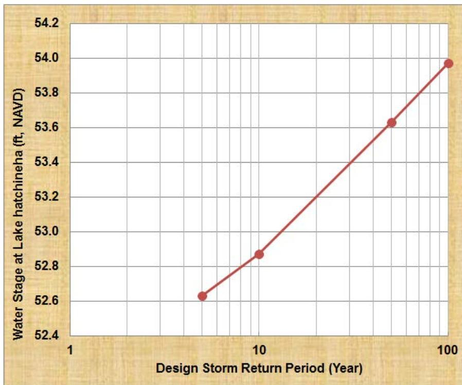
**Figure 12** Stages at Lake Hatchineha Corresponding to Design Storm Frequencies
