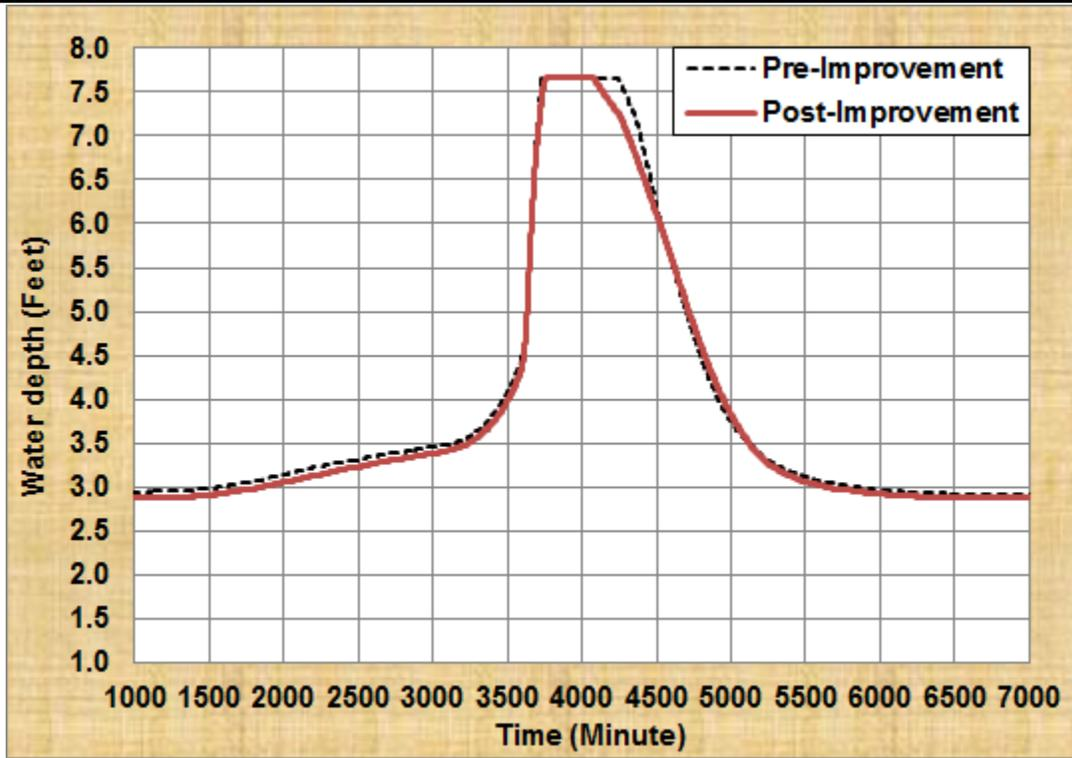
Figure 19a. Water Depth in C67 for Pre- and Post-Improvements
