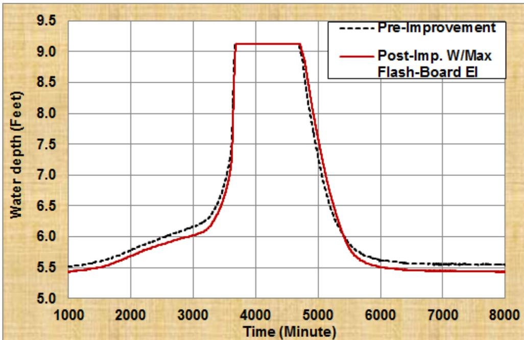
Figure 26f. Water Depth in C-Imp1S-Store for Pre-Improvement and Post-Improvement with Maximum Flash-board Elevation for the 100-year, 3-Day Design Storm
