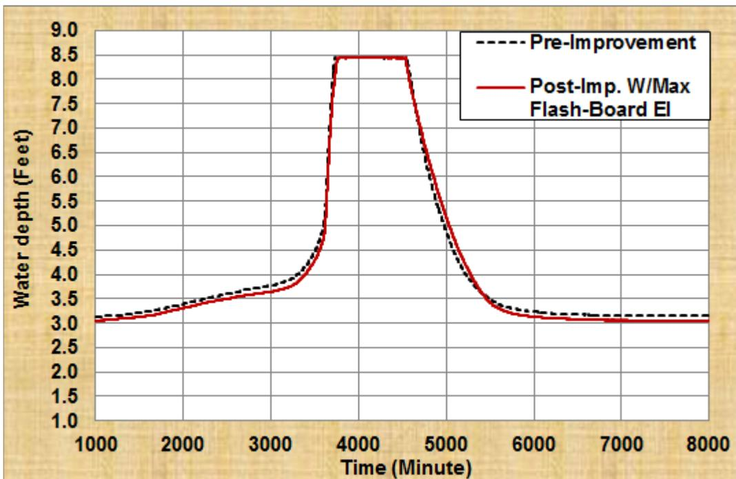
Figure 26b. Water Depth in C-Imp1SN for Pre-Improvement and Post-Improvement with Maximum Flash-board Elevation for the 100-year, 3-Day Design Storm
