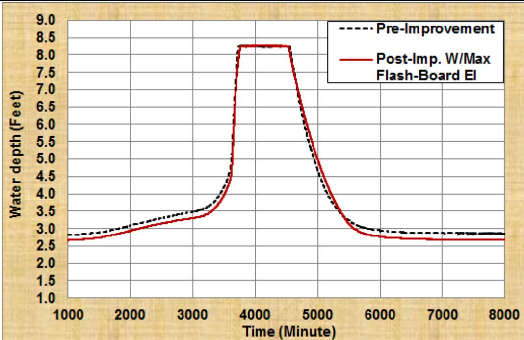
Figure 26c. Water Depth in C-Imp1S-2 for Pre-Improvement and Post-Improvement with Maximum Flash-board Elevation for the 100-year, 3-Day Design Storm
