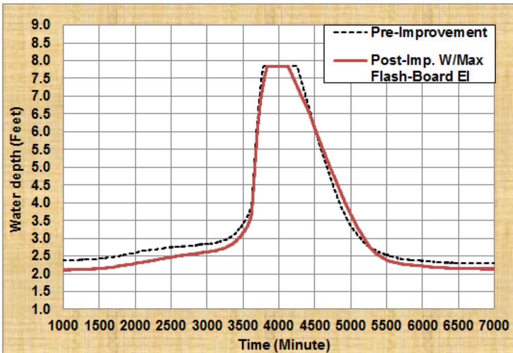
Figure 25d. Water Depth in C-Imp1-1E for Pre-Improvement and Post-Improvement with Maximum Flash-board Elevation for the 25-year, 3-Day Design Storm
