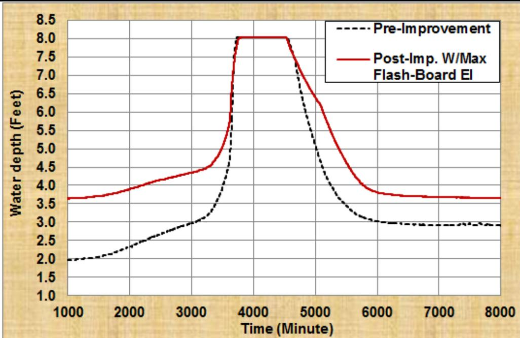
Figure 26e. Water Depth in C-Imp1-E for Pre-Improvement and Post-Improvement with Maximum Flash-board Elevation for the 100-year, 3-Day Design Storm
