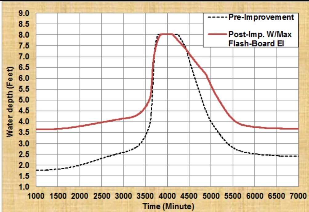
Figure 25e. Water Depth in C-Imp1-E for Pre-Improvement and Post-Improvement with Maximum Flash-board Elevation for the 25-year, 3-Day Design Storm
