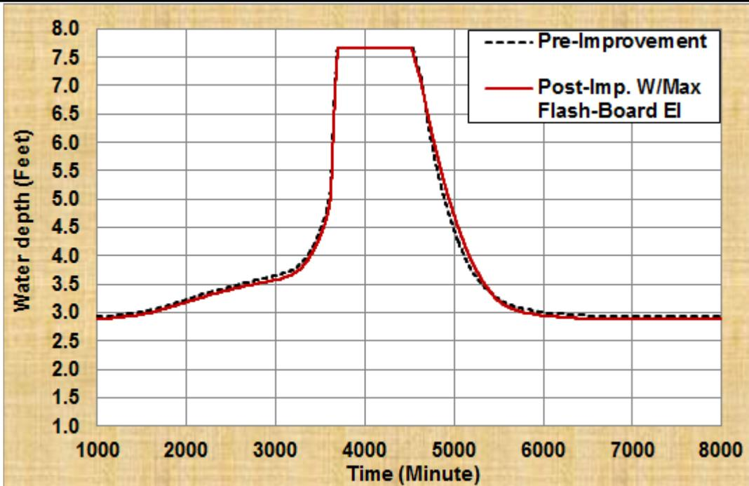
Figure 26a. Water Depth in C67 for Pre-Improvement and Post-Improvement with Maximum Flash-board Elevation for the 100-year, 3-Day Design Storm
