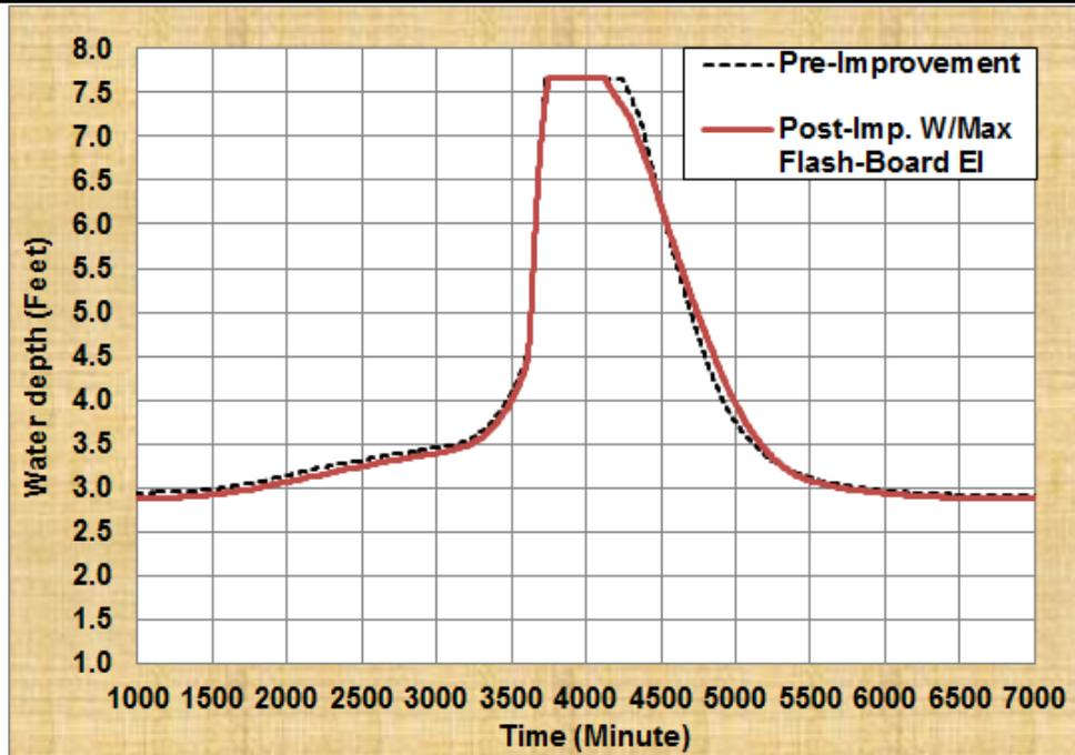
**Figure 25a.** Water Depth in C67 for Pre-Improvement and Post-Improvement with Maximum Flashboard Elevation for the 25-year, 3-Day Design Storm
