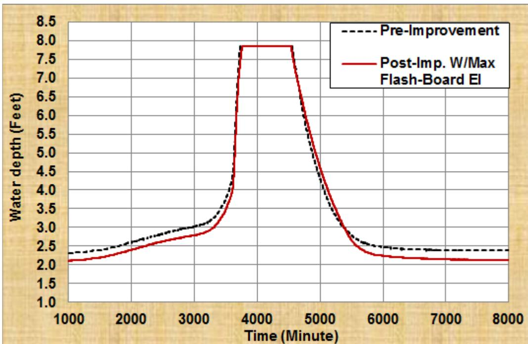
Figure 26d. Water Depth in C-Imp1-1E for Pre-Improvement and Post-Improvement with Maximum Flash-board Elevation for the 100-year, 3-Day Design Storm
