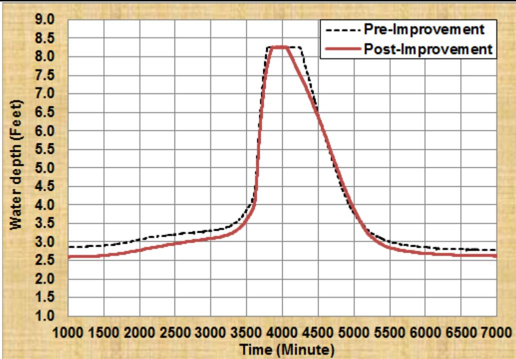
Figure 19c. Water Depth in C-Imp1S-2 for Pre- and Post-Improvements
