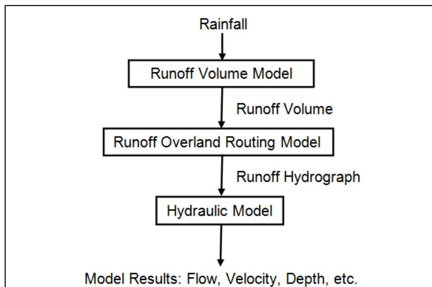
**Figure 2.** Schematic of the SWMM Hydrological and Hydraulic Model
