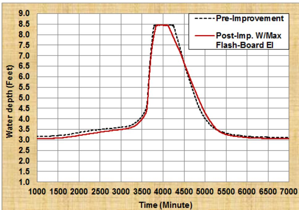
**Figure 25b.** Water Depth in C-Imp1SN for Pre-Improvement and Post-Improvement with Maximum Flash-board Elevation for the 25-year, 3-Day Design Storm
