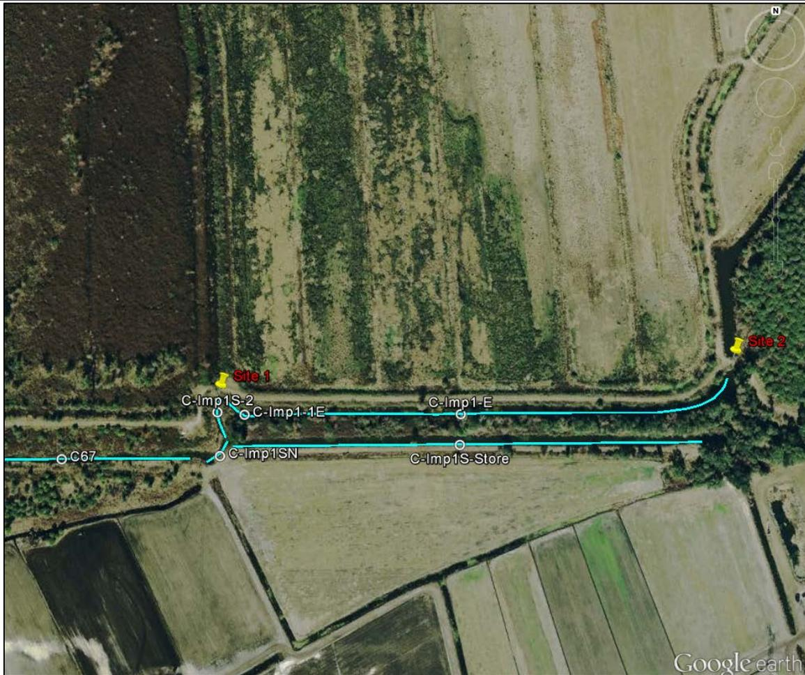
**Figure 18.** SWMM Conduits Representing the Canal Segments between Site 1 & Site 2
