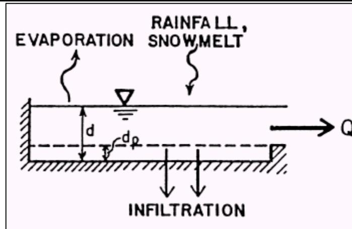
**Figure 3.** Schematic of the SWMM Surface Runoff Routing Model
