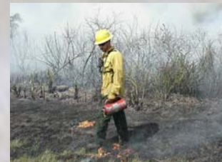
Tools such as this drip torch are used to ignite the brush
