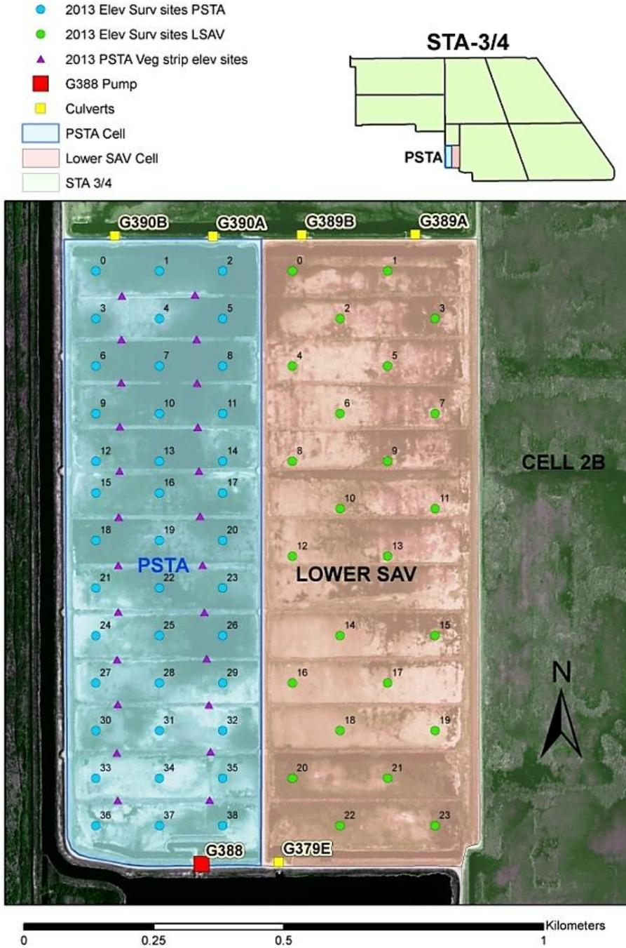
Figure C-1. Map of the STA-3/4 PSTA Project showing elevation survey points measured within the PSTA and LSAV cells in August 2013.
