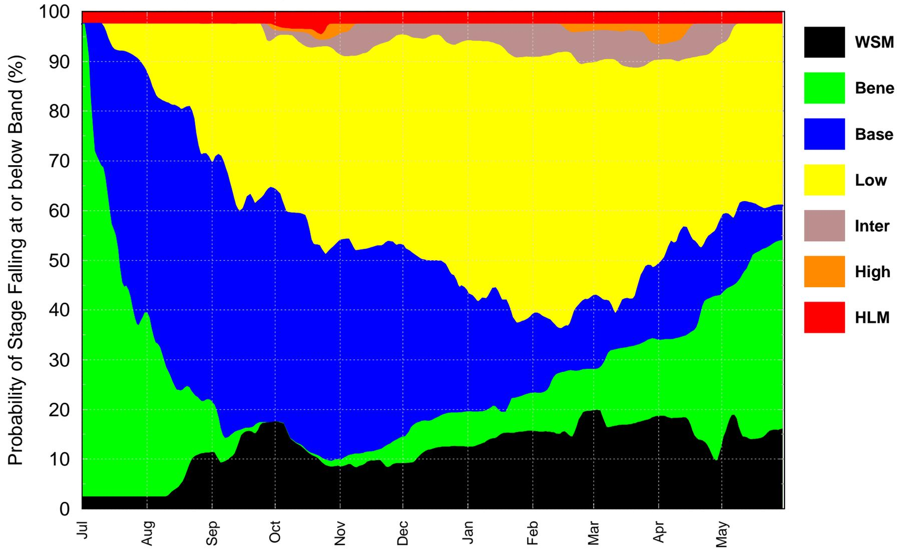
The width for each band gives the probability of stage falling in that band, as defined by the operational schedules.
