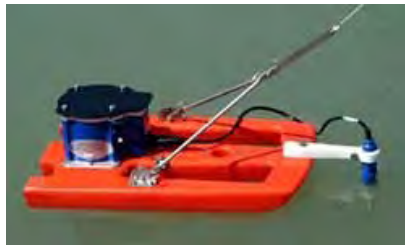
Figure 5-4. StreamPro 2400-KHz Acoustic Doppler Current Profiler (ADCP).
