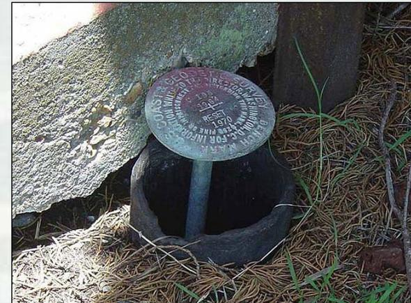
Deep-driven rod mark, sometimes with cap, most often without. Datum point is the tip of the rod, with the name stamped on the aluminum collar/cover.
