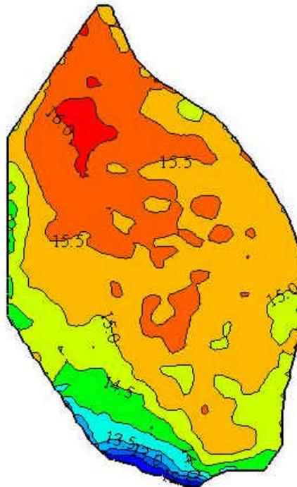
**Figure 10.** Bathymetric Contours for the Loxahatchee Refuge (ft NGVD29)
