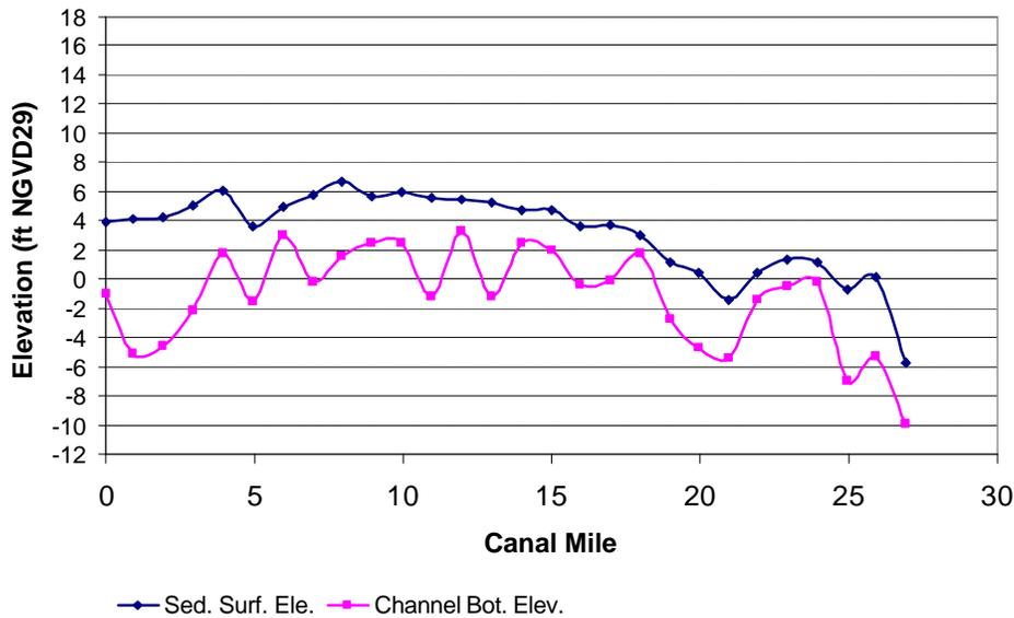
**Figure 15.** Thalweg Profiles for the Sediment Surface Elevation and Channel Bottom Elevation for the Eastern Canal (L-40) (adapted from Meselhe et al., 2005)
