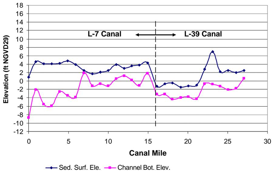
**Figure 14.** Thalweg Profiles for the Sediment Surface Elevation and Channel Bottom Elevation for the Western Canals (L-7 and L-39) (adapted from Meselhe et al., 2005)
