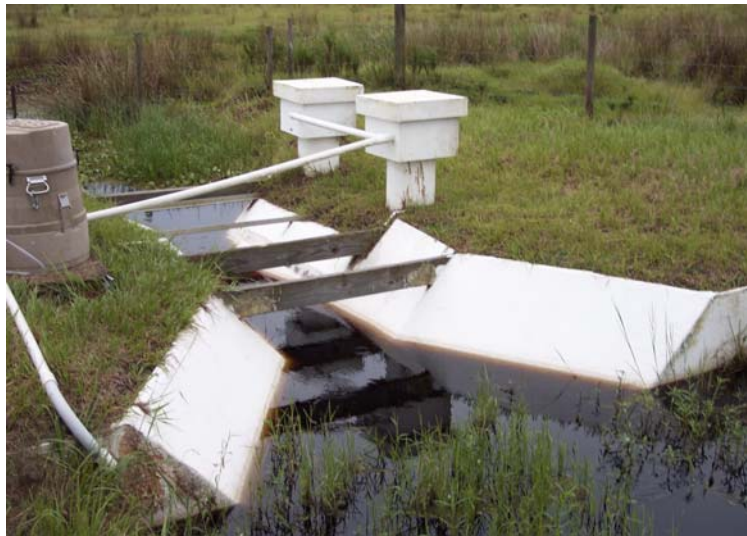
Figure 2.4. Photo of a flume used to collect surface runoff from an experimental pasture.
