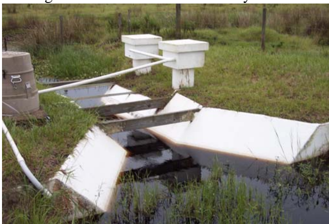
Figure 4. Photo of flume structure showing 1) two stilling wells (top center) containing shaft encoders to monitor water levels in the flume; and 2) an ISCO automatic water sampler (left) that collects samples just upstream of the flume.
