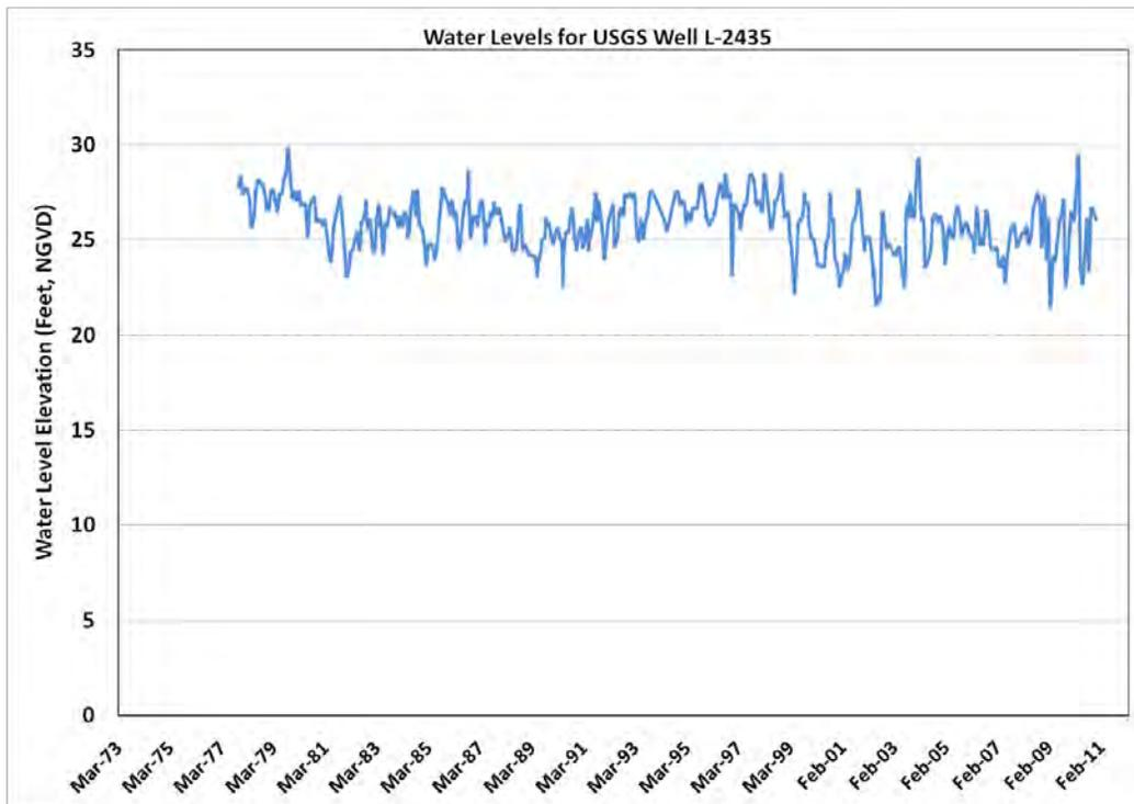
**Figure 13.** Water levels in an Upper Floridan monitor well at a location and depth typical of PWS withdrawals in Lee County.
