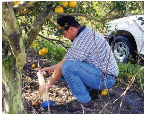
Technician Collecting Discharge Volume from Microirrigation Spray Jet Emitter
