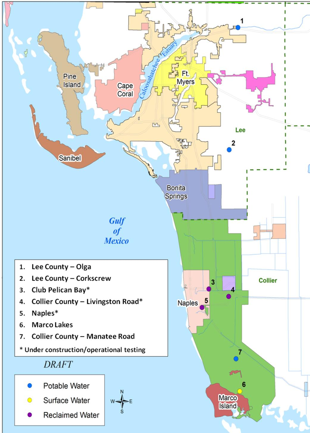
**Figure D-4.** LWC utility aquifer storage and recovery (ASR) systems.
