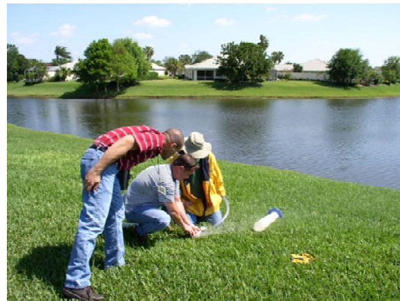
Technician Testing Sprinkler Head for Flow and Pressure
