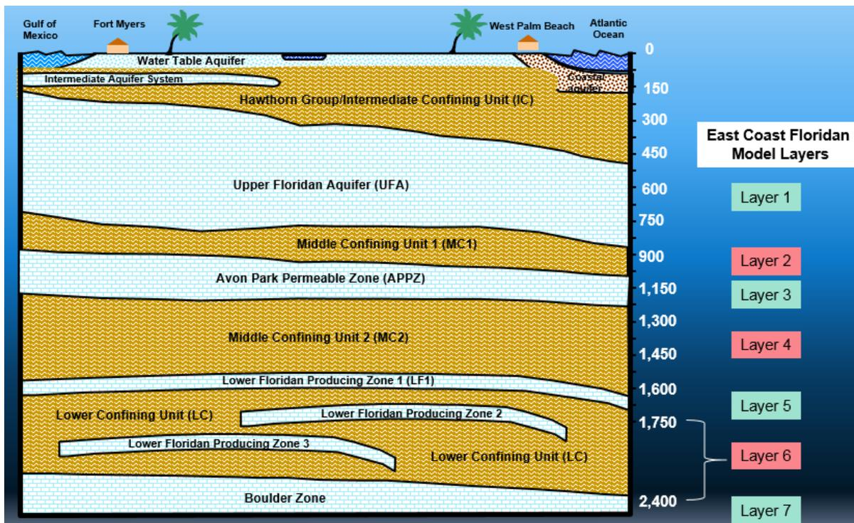
Figure 2. The seven layers of the East Coast Floridan Model shown with a generalized cross-section of the aquifer systems in South Florida.
