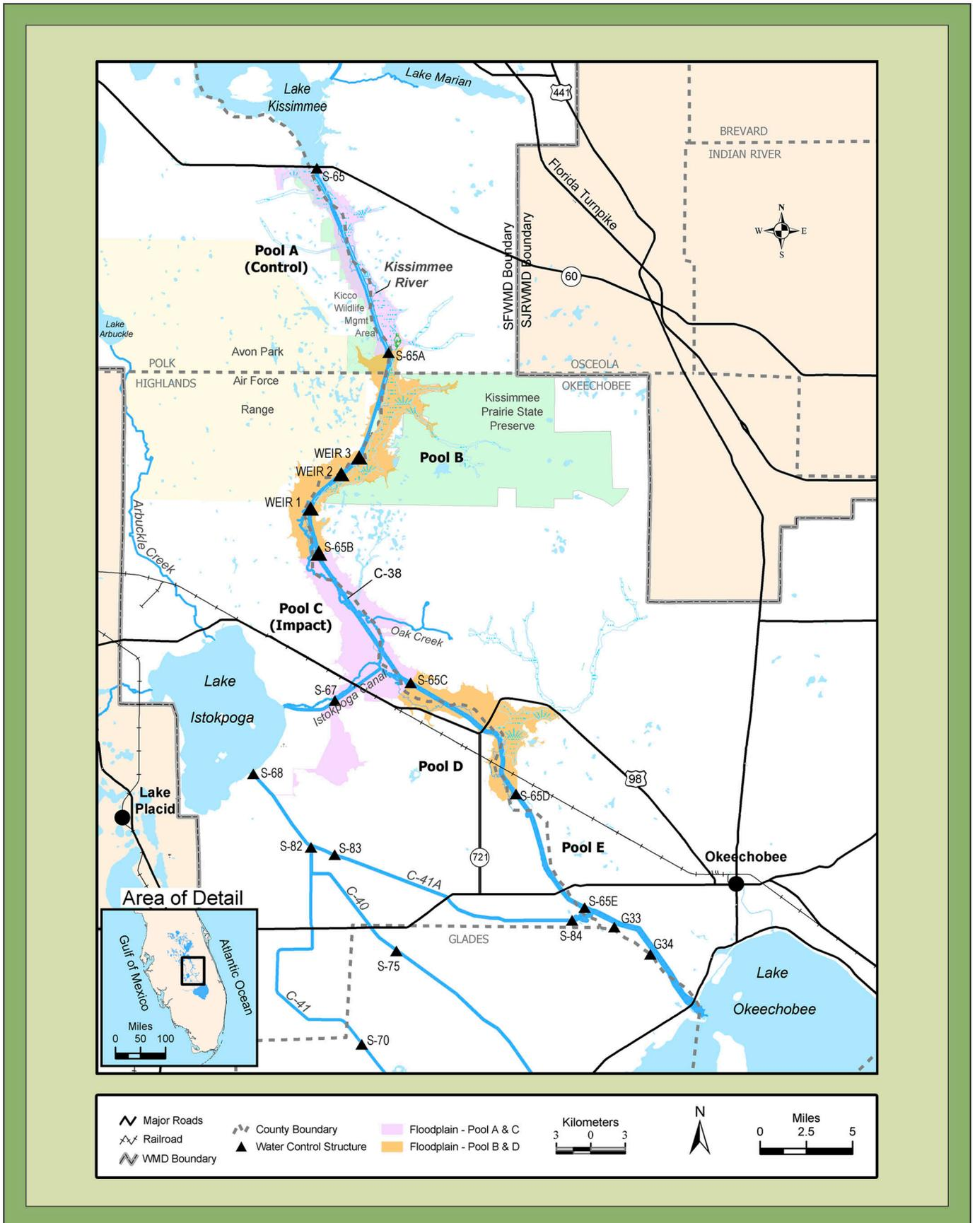
**Figure 1.** Location of the Kissimmee River in Florida. The C-38 canal cuts through the floodplain and intercepts the meandering river channel. The channelized system includes the floodplain, remnant river channels and the C-38 canal. The canal is divided into a series of five impounded pools (Pools A-E) by six water control structures (S-65 to S-65E). The Upper Chain of Lakes through Lake Kissimmee provides water to the Kissimmee River, which discharges into Lake Okeechobee.
