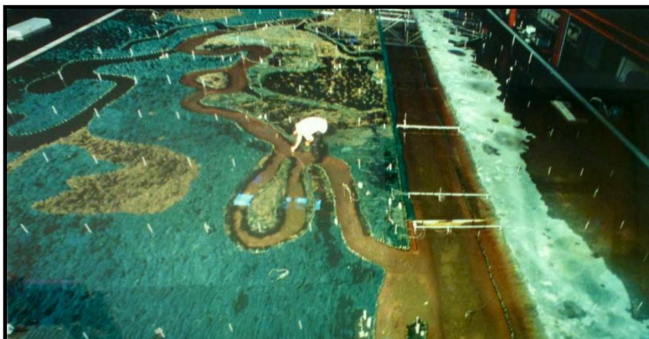
The planning of the restoration project was aided by the construction of a large scale-model of the river in a huge tank in a lab at Univ. of California, Berkley.
