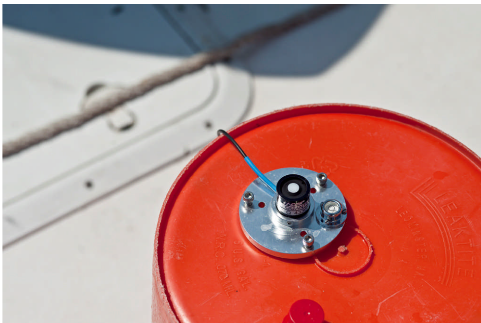
Figure 5.2-2. Licor LI-190 Sensor Used to Measure Ambient Light at the Surface Simultaneously with Underwater Measurements to Calculate Light Attenuation with Depth.
