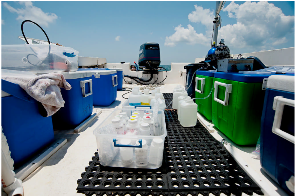
Figure 5.2-6. A Peristaltic Pump (on Top of Green Coolers) Used to Collect Porewater for Nutrient and Tracer Suite Analysis.
