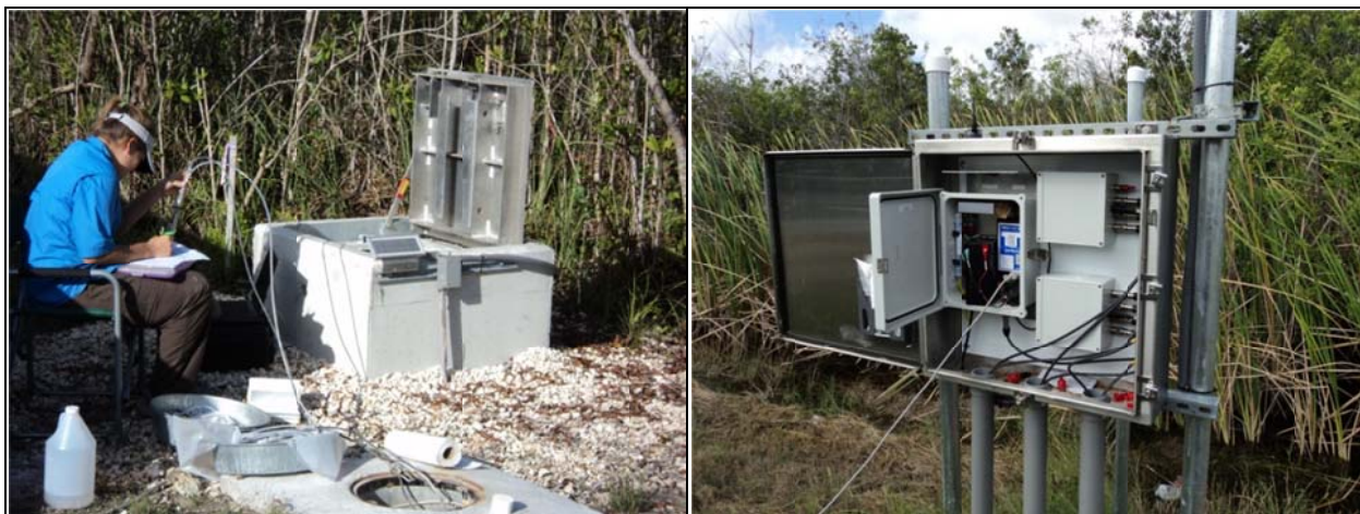
Figure 2-1. Automated Groundwater Station.
