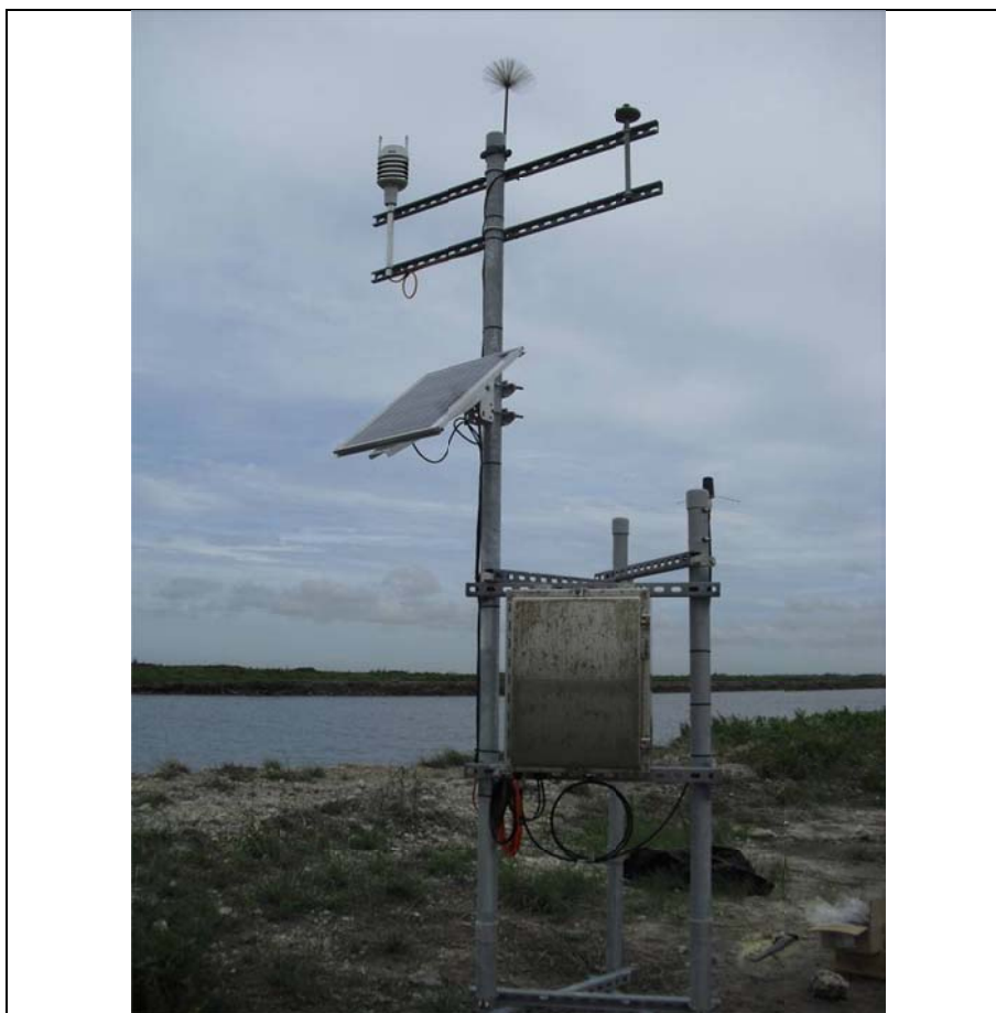
Figure 2-80. Meteorological Station Showing Vaisala WST520 Weather Transmitter, a Static Electricity Dissipater (Bristle Brush at Highest Point of Structure) and the LI-190SA Quantum Sensor. The solar panel is located between the instrumentation and the Campbell datalogger (housed within the stainless steel box). Data are recorded in the CR-1000 logger at 15-minute intervals and uploaded daily via telemetry.
