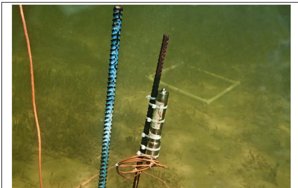
Figure 4-7. A ThermoWorks TCTemp 1000 thermocouple datalogger inserted to 30 cm in the substrate to measure in-situ porewater temperature. A quarter-meter quadrat used to estimate SAV coverage is visible in the background.
