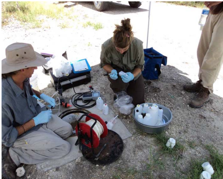
Figure 3-1. Groundwater Sampling Setup Using Peristaltic Pump, Flow Through Cell and Dedicated Well Tubing.
