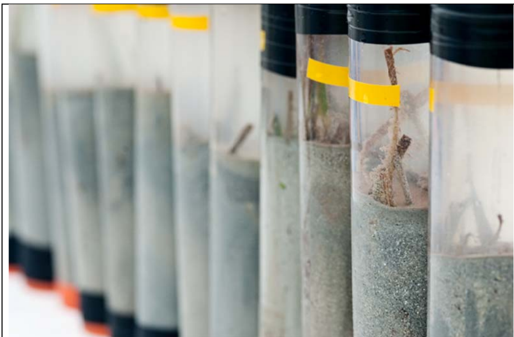
Figure 4-9. Soil cores capped and ready for transport to the lab for processing.
