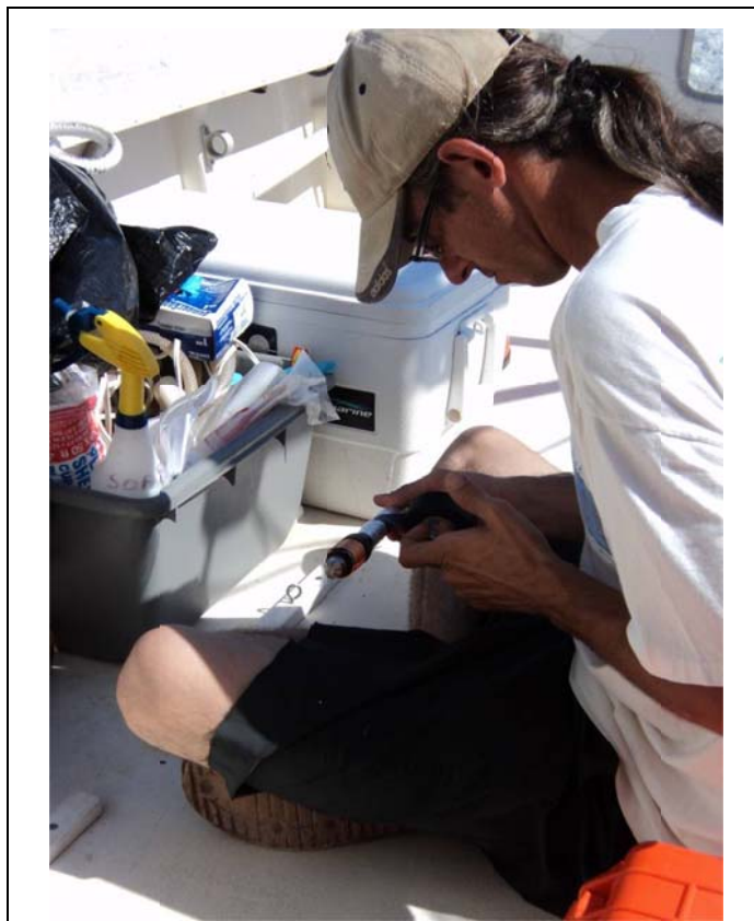
Figure 2-16. Preparing AquaTROLL® 100 for deployment in Biscayne Bay. The sensors within the probe are protected by a Copper Gard (shield of wound copper fitting over probe end).
