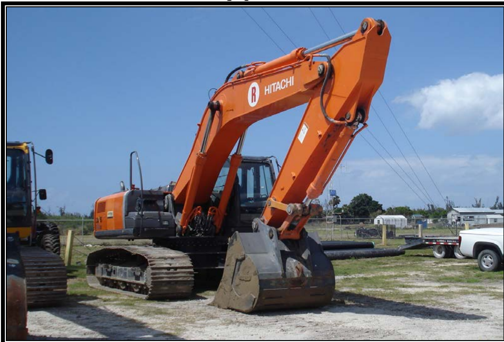
District Construction Equipment: Excavator / Trackhoe
