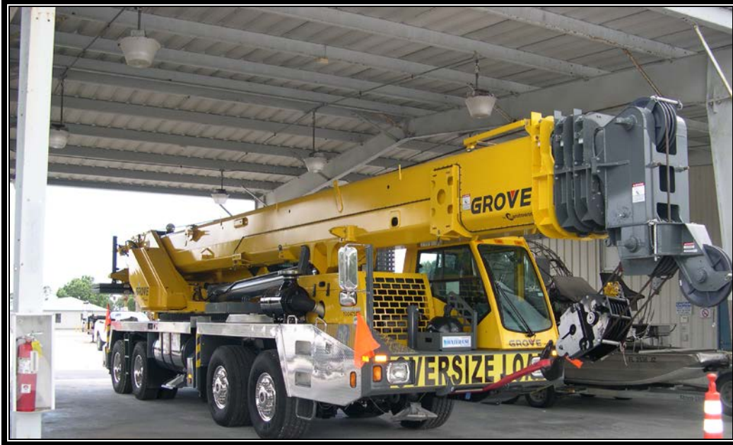
District Construction Equipment: 80 Ton Hydraulic Crane
