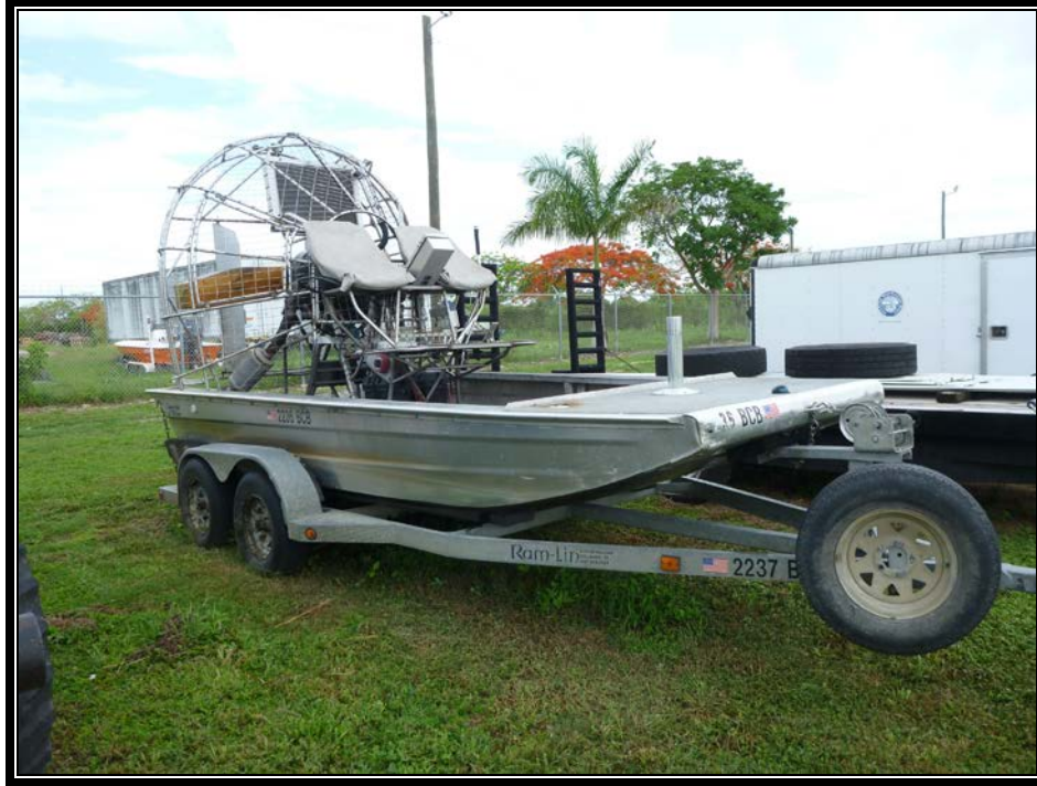
District Airboat with Vehicle Engine
