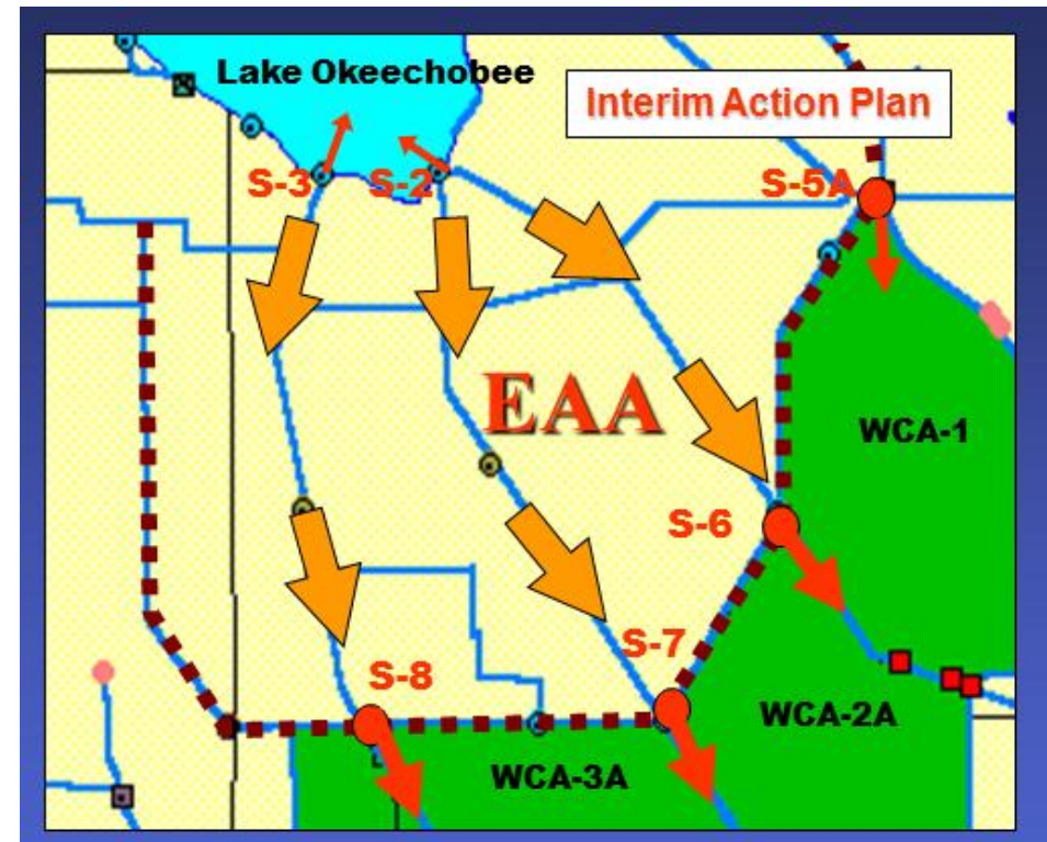
Figure A-2. EAA flow patterns under the Interim Action Plan (IAP). [Note: Following IAP implementation in the early 1980s, most of the EAA runoff was directed to the WCAs in efforts to reduce nutrient impacts to Lake Okeechobee. EAA runoff discharged to the WCAs increased by about 190,000 ac-ft. Flood control operation of S-2 and S-3 occurs only when southern capacity is not sufficient.]
