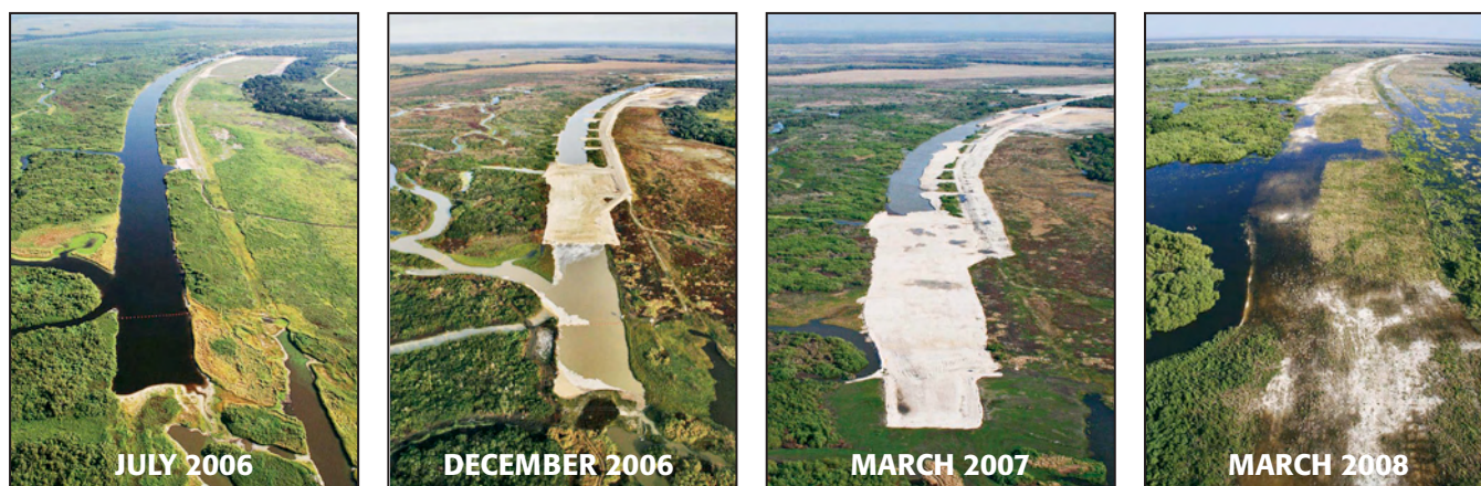
STAGES OF PHASE IVA CONSTRUCTION (JULY 2006–MARCH 2007) FOLLOWED BY PARTIAL REESTABLISHMENT OF WETLAND VEGETATION (MARCH 2008) ON A BACKFILLED SECTION OF THE KISSIMMEE RIVER FLOODPLAIN
