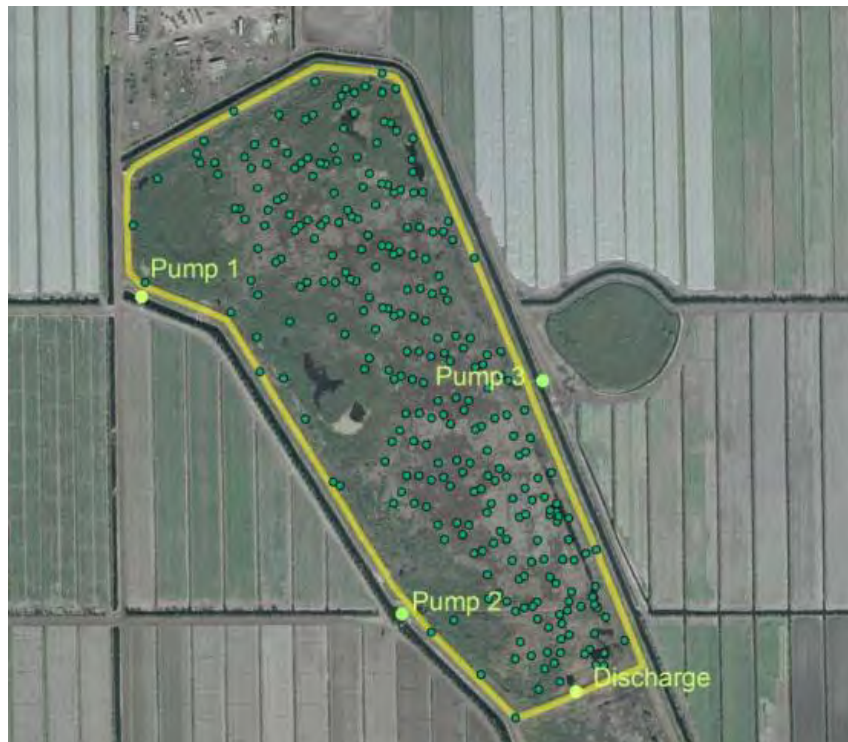
Figure 7. Location of topographic survey data points (green circles).
