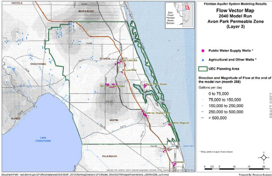
Figure 16. APPZ flow vectors in the final month of the 2040 simulation.
