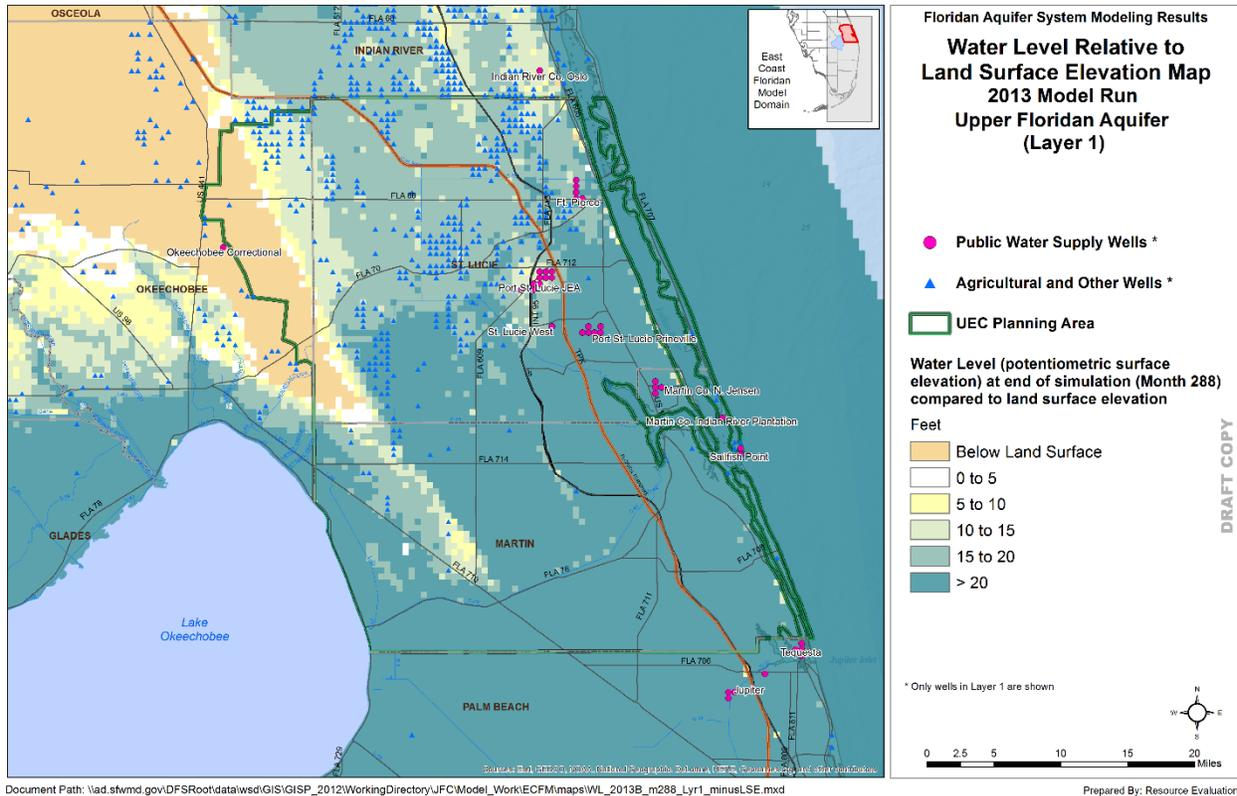
Figure 17. Potentiometric surface of the UFA relative to land surface at the end of the 2013 simulation.
