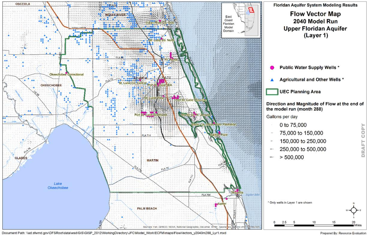
Figure 14. UFA flow vectors in the final month of the 2040 simulation.
