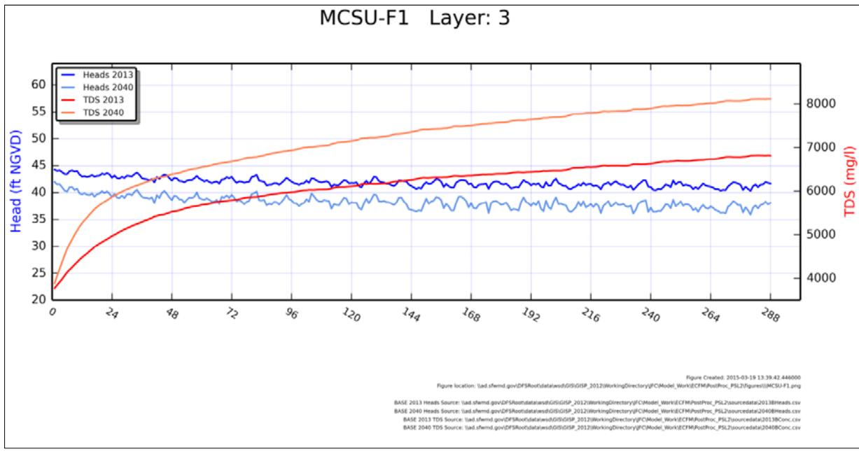
Figure 12. Change in water level and water quality for 2013 and 2040 in the APPZ at the MCSU-F1 monitoring well in Martin County.
