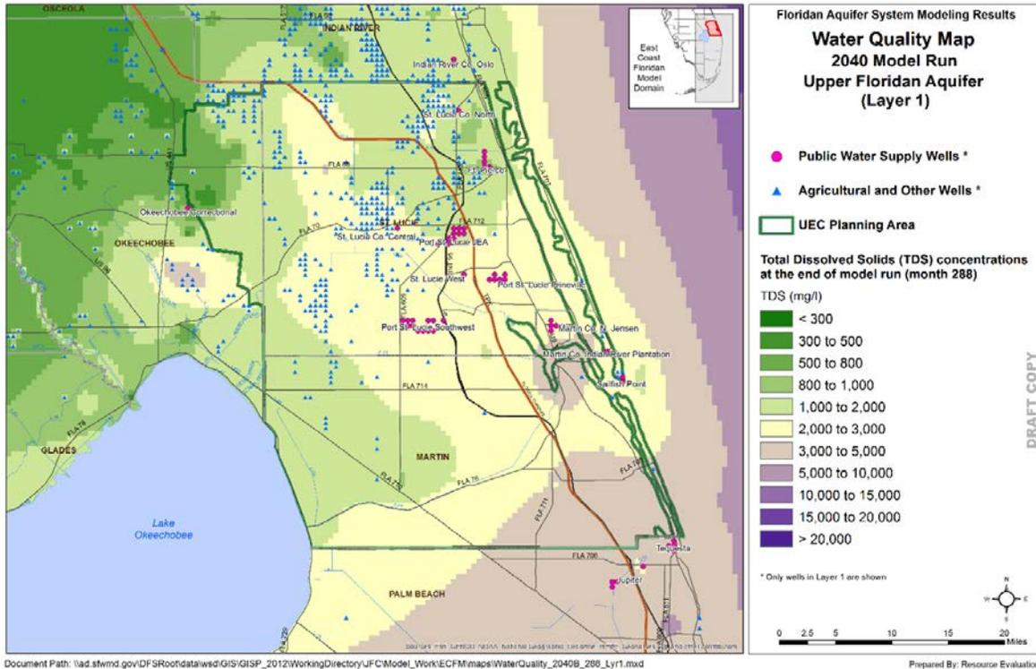
Figure 7. Change in water quality between the initial condition and the end of the 2040 simulation (month 288) in the UFA (Layer 1).
