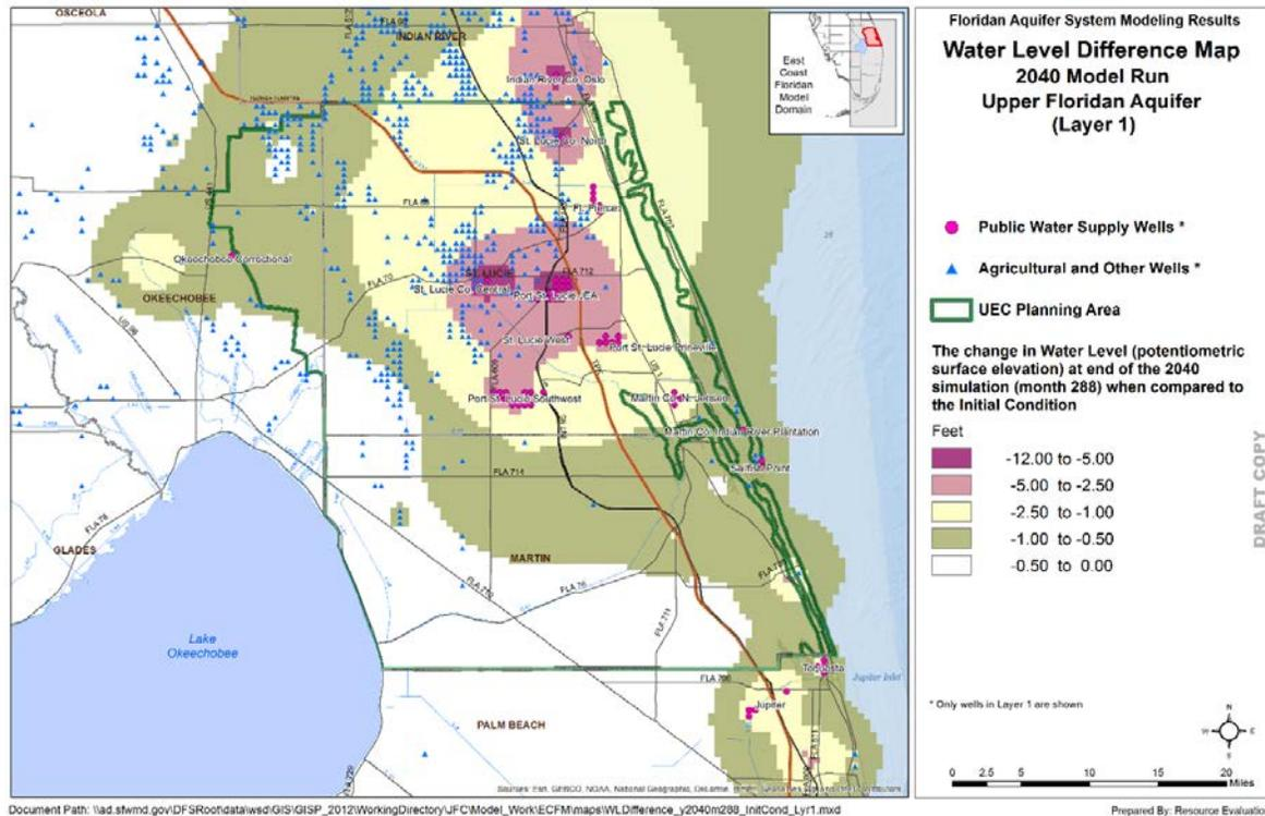
Figure 3. Change in water levels between the initial condition and of the end of the 2040 simulation (month 288) in the UFA (Layer 1).
