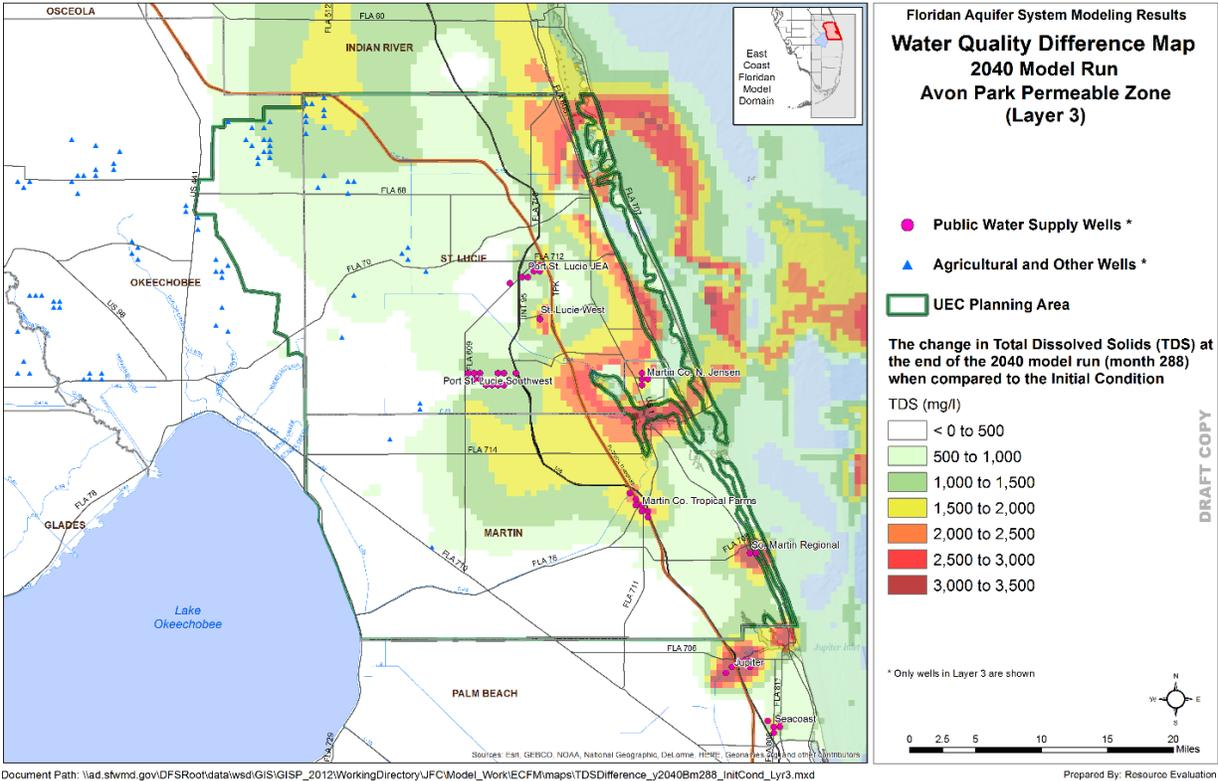
Figure 11. Change in water quality in the APPZ from the initial condition to the end of the 2040 simulation.
