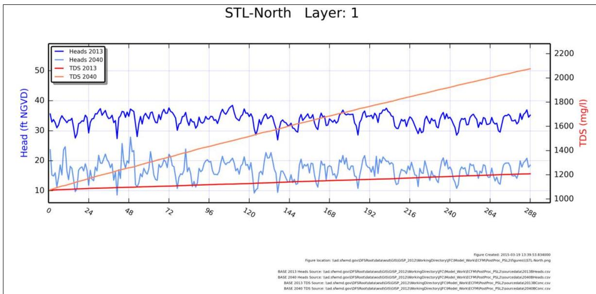
Figure 4. Results of 2013 and 2040 simulation head and TDS differences in the UFA at the proposed St. Lucie County Utilities North wellfield.
