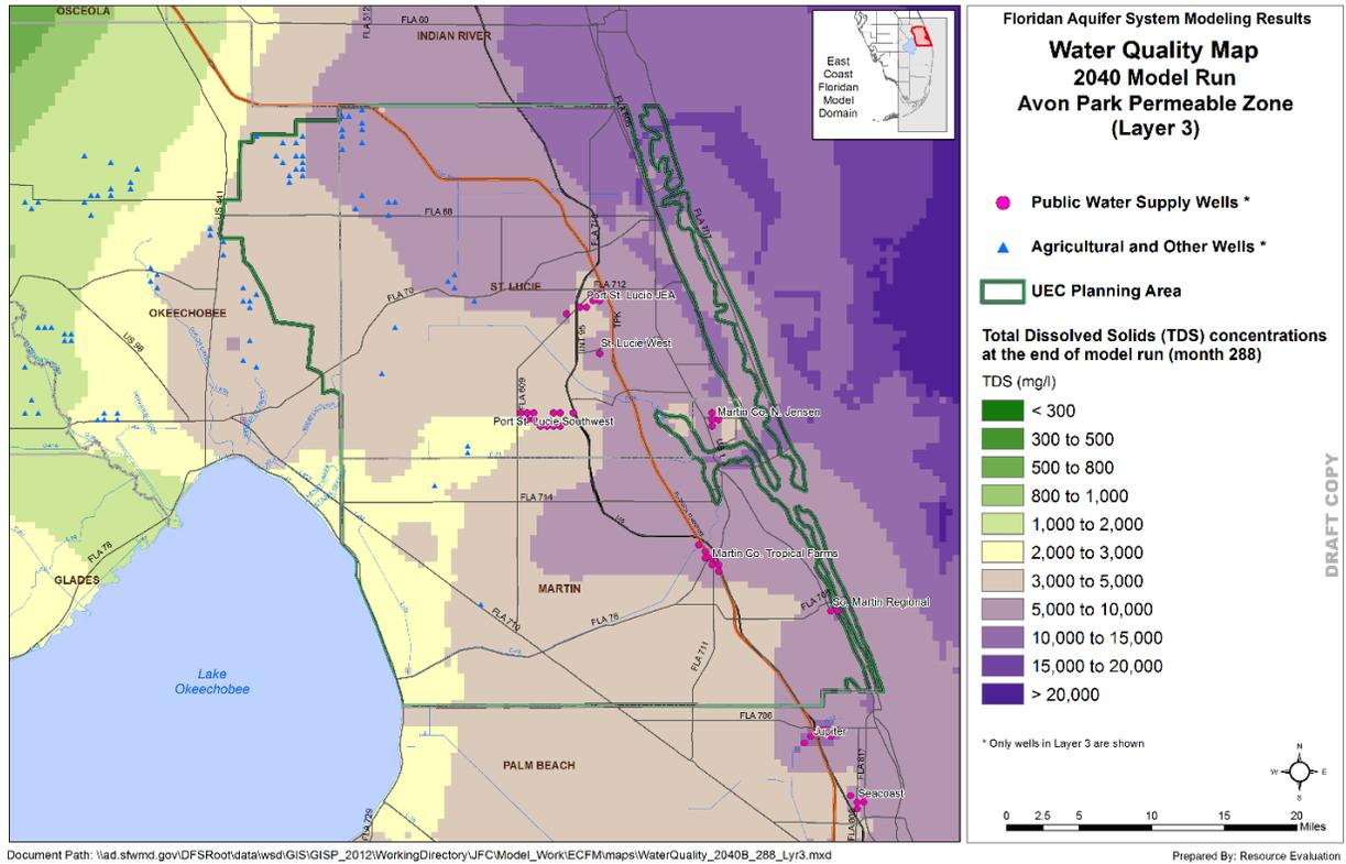
Figure 10. Water quality conditions in the APPZ at the end of the 2040 simulation.
