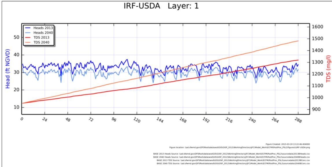
**Figure 9.** Results of the 2013 and 2040 simulated changes in water quality in Indian River County at Well IRF-USDA.
