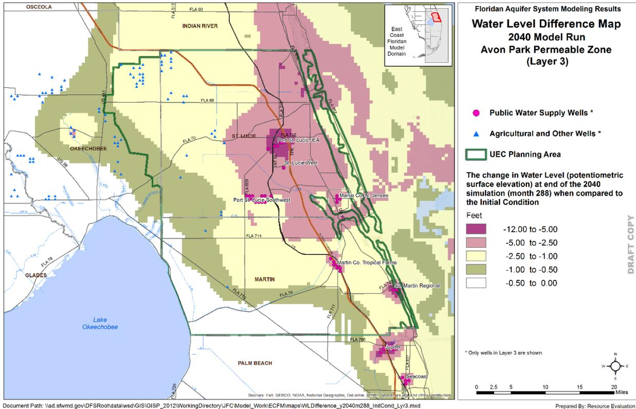
Figure 6. Water level change between the initial condition and the end of the 2040 simulation (month 288) in the APPZ (Layer 3).
