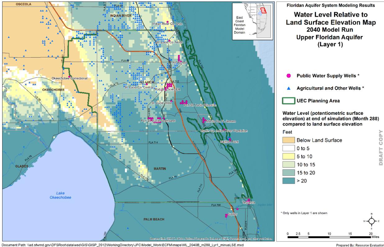
Figure 18. Potentiometric surface of the UFA relative to land surface at the end of the 2040 simulation.
