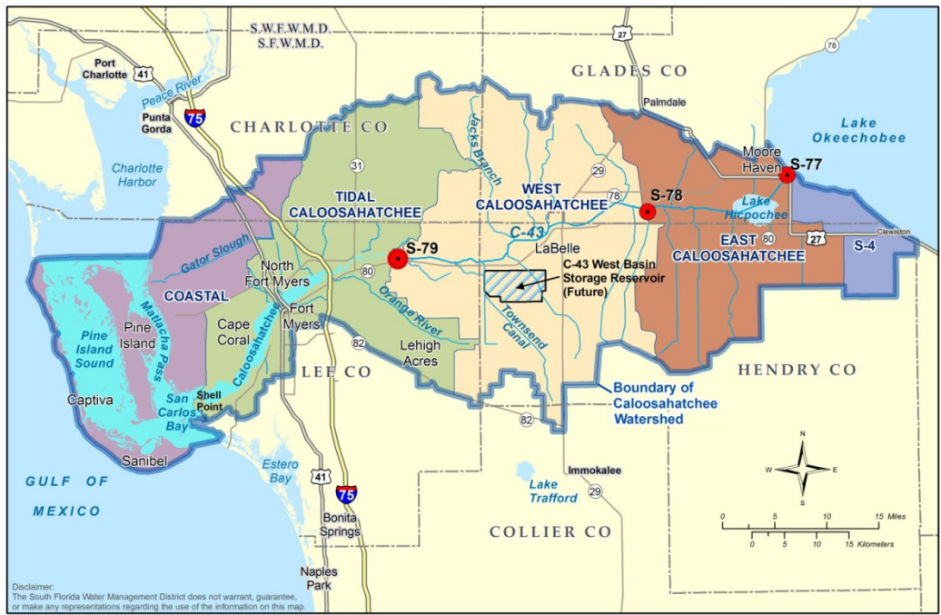
Figure 3-1. Caloosahatchee River, C-43 Canal, and watershed showing major basins, water management structures, and location of the C-43 Reservoir.
