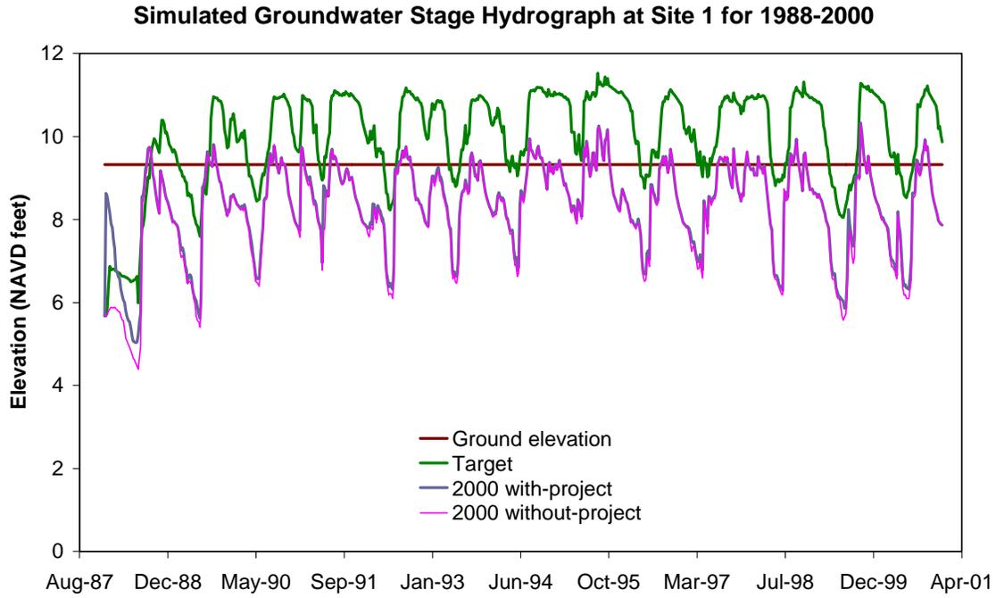
Figure A-2. Simulated groundwater stage hydrograph at Site 1 for 1988 to 2000
