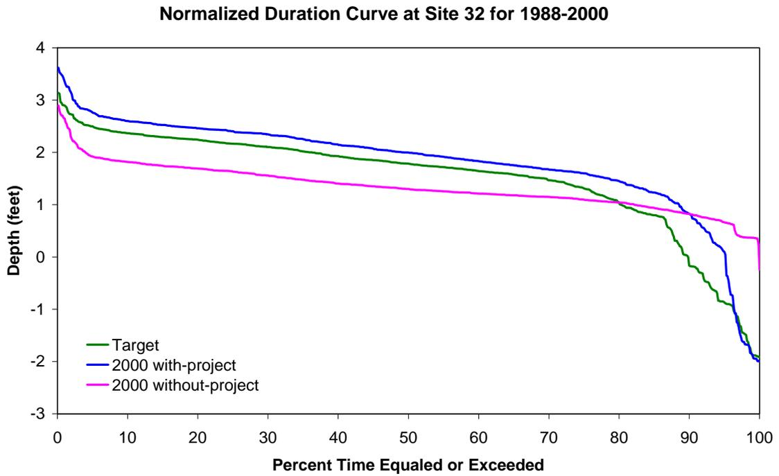
Figure A-65. Normalized duration curve at Site 32 for 1988 to 2000
