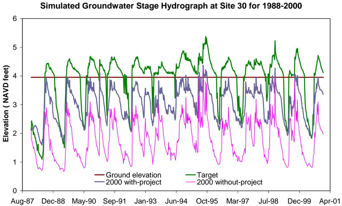
Figure A-31. Simulated groundwater stage hydrograph at Site 30 for 1988 to 2000
