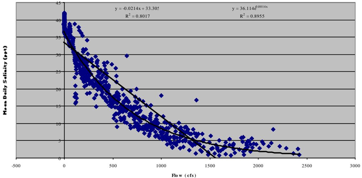
Figure 34. Relationship between flow and salinity above the fixed weir at Port of the Islands on the Faka Union Canal 2000 to 2002
