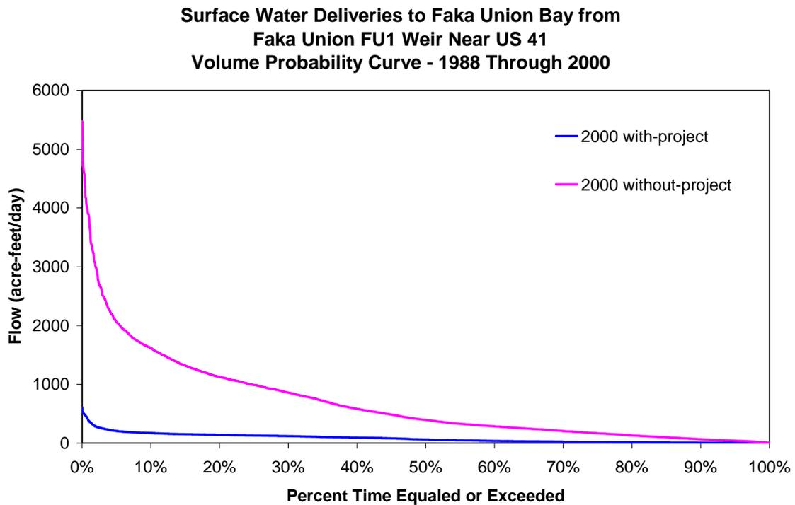
Figure 66. Volume probability curve for surface water inflow from the FU1 weir on Faka Union Canal for the entire period of record (1988 - 2000)
