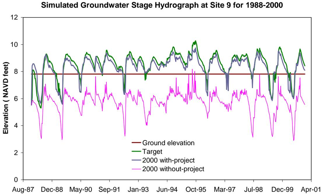
Figure A-10. Simulated groundwater stage hydrograph at Site 9 for 1988 to 2000
