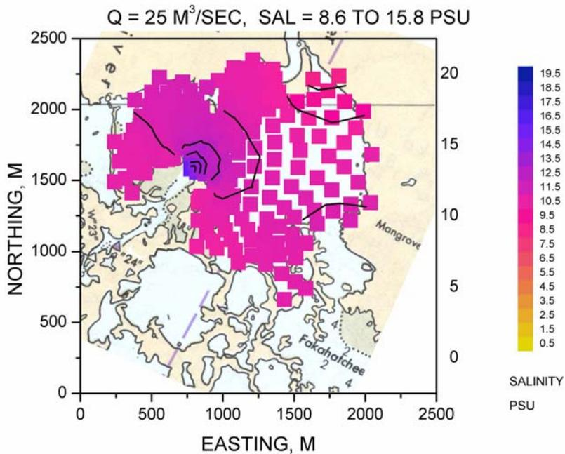
Figure 21. Model-computed salinity field for freshwater inflow of 25 m<sup>3</sup>/s
