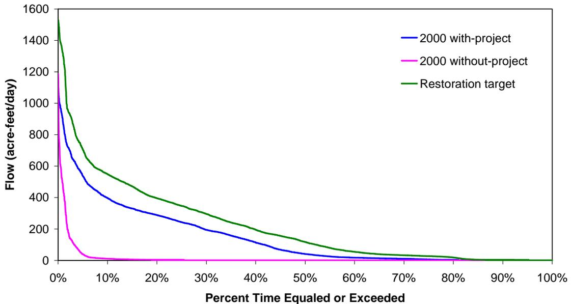
Figure 60. Volume probability curve for surface water inflow along the Merritt Canal flowway near US 41 for the entire period of record (1988 – 2000)
