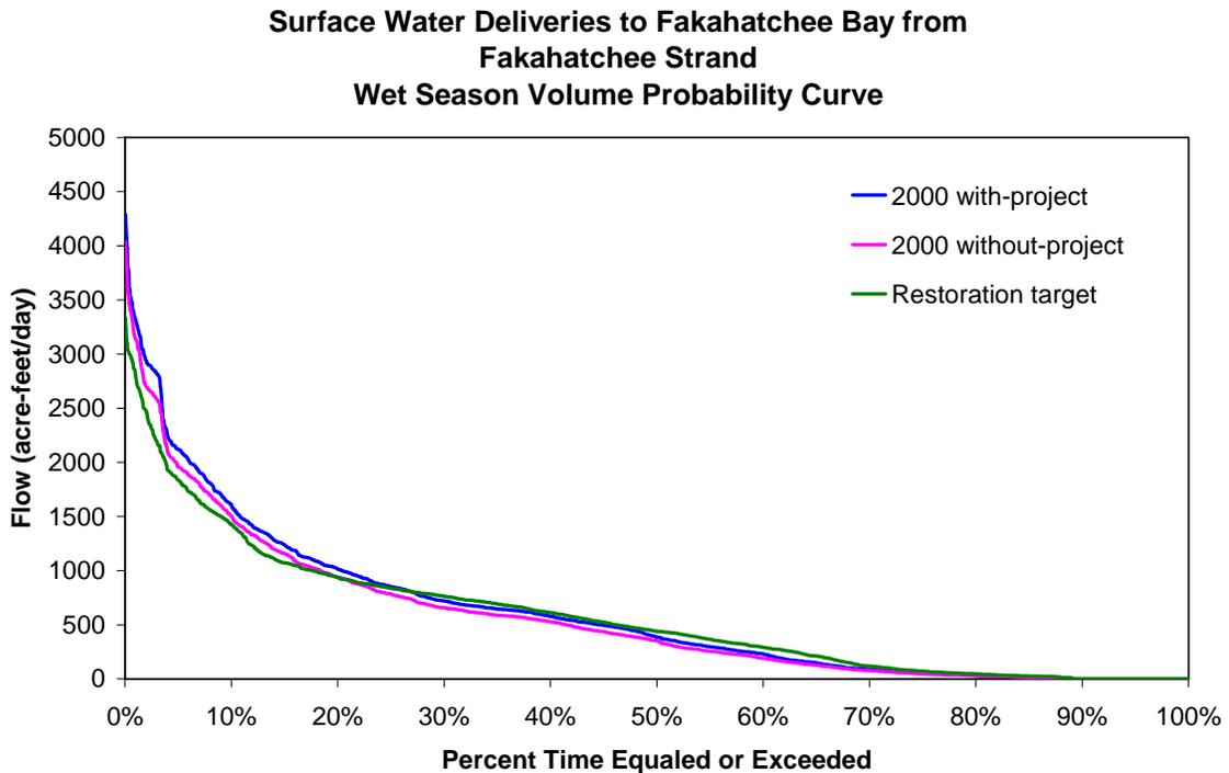
Figure 64. Volume probability curve for surface water inflow from Fakahatchee Strand for the wet season for the period of record (1988 - 2000)
