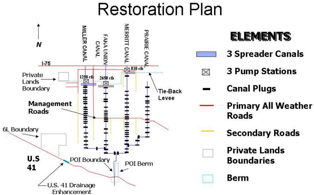
Figure 4. Construction features of the Picayune Strand Restoration Project
