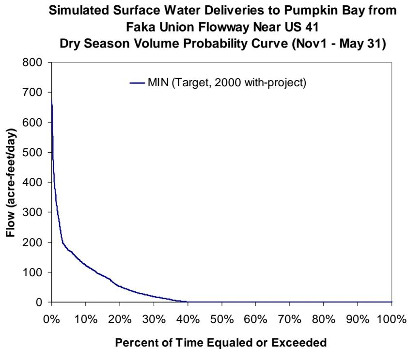
Figure 83. Volume probability curve for surface water inflow along the Faka Union Canal flowway to be reserved for the dry seasons during the period of record (1988 - 2000)
