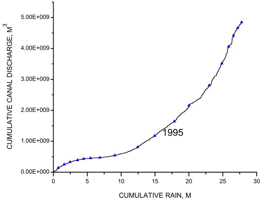
Figure 17. Mass balance of cumulative rain versus cumulative Faka Union Canal discharge 1985 to 2002
