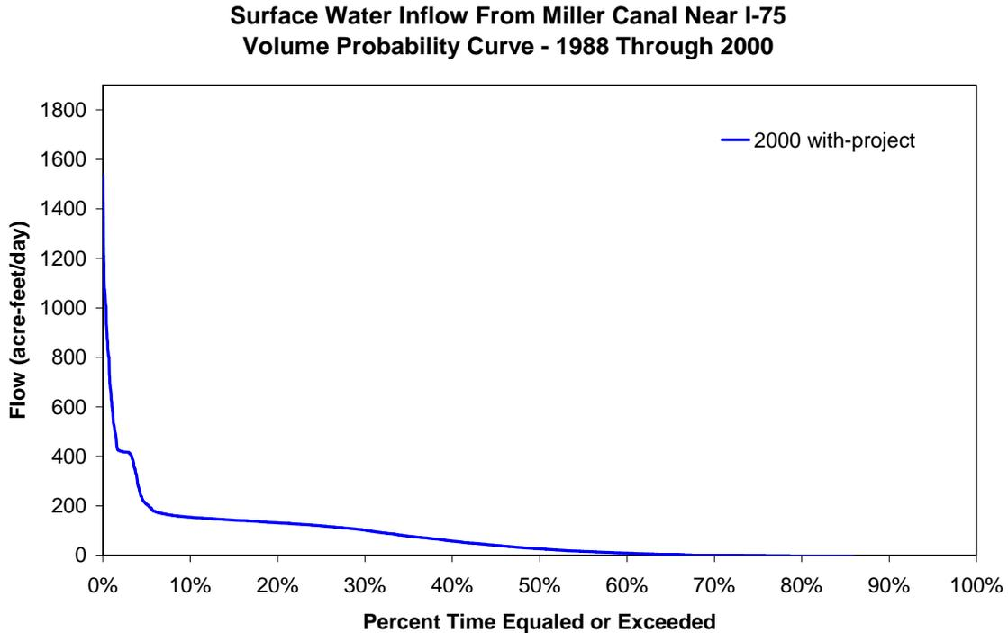
Figure 69. Volume probability curve of surface water deliveries into Picayune Strand Restoration Area from the Miller Canal to be reserved
