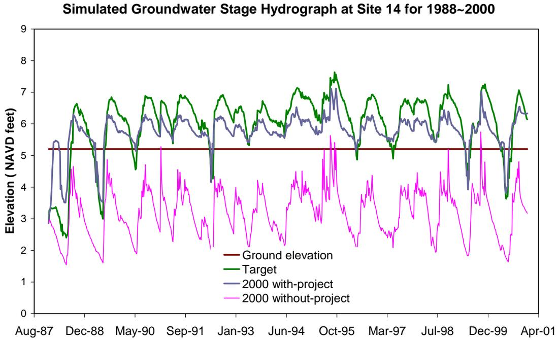
Figure A-15. Simulated groundwater stage hydrograph at Site 14 for 1988 to 2000
