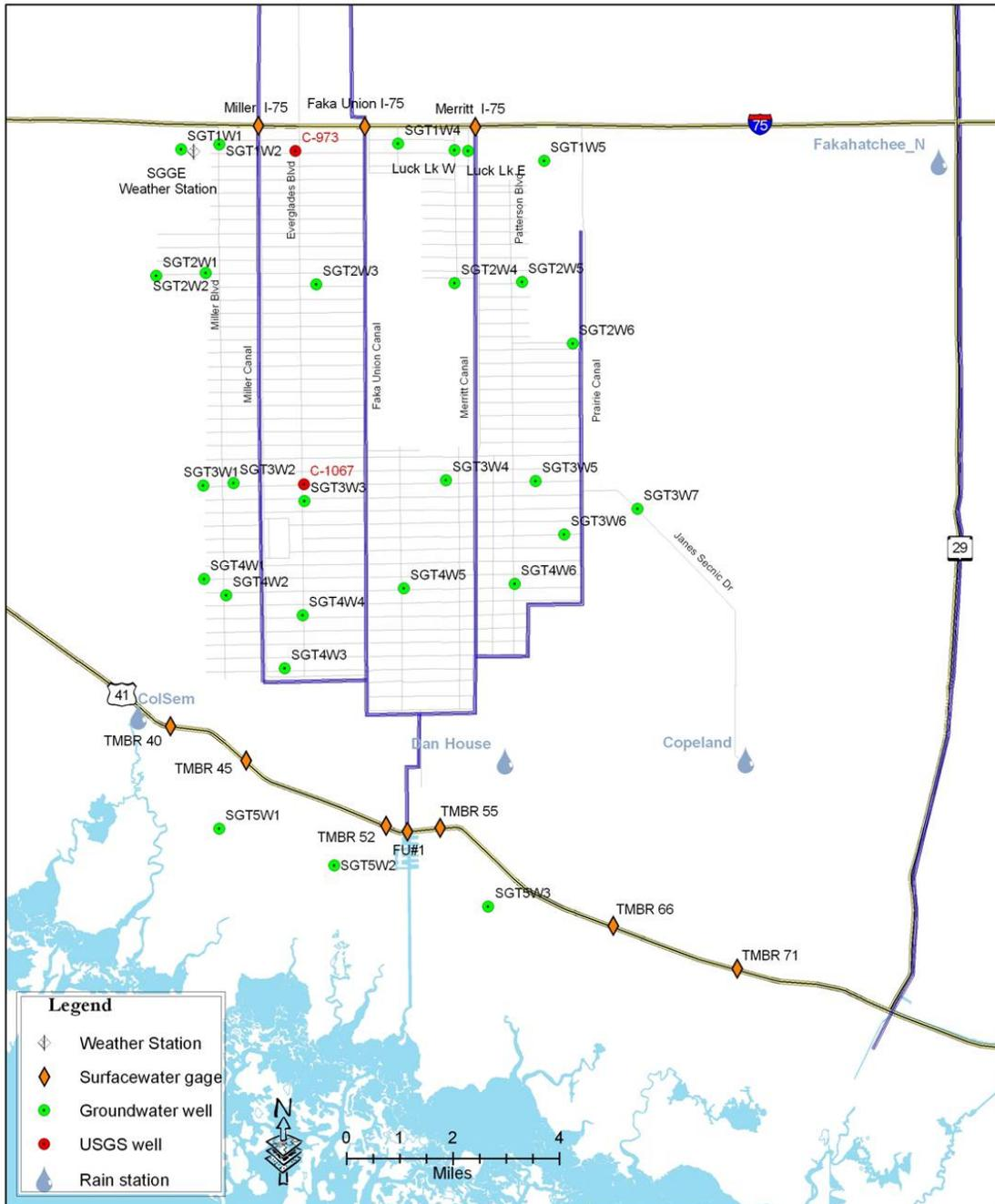
Figure 32. Picayune Strand Restoration Project hydrologic monitoring sites
