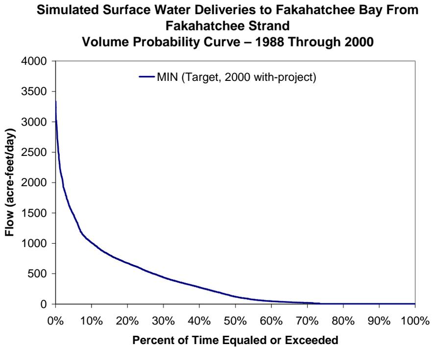
Figure 87. Volume probability curve for surface water inflow from Fakahatchee Strand to be reserved for the period of record (1988 - 2000)
