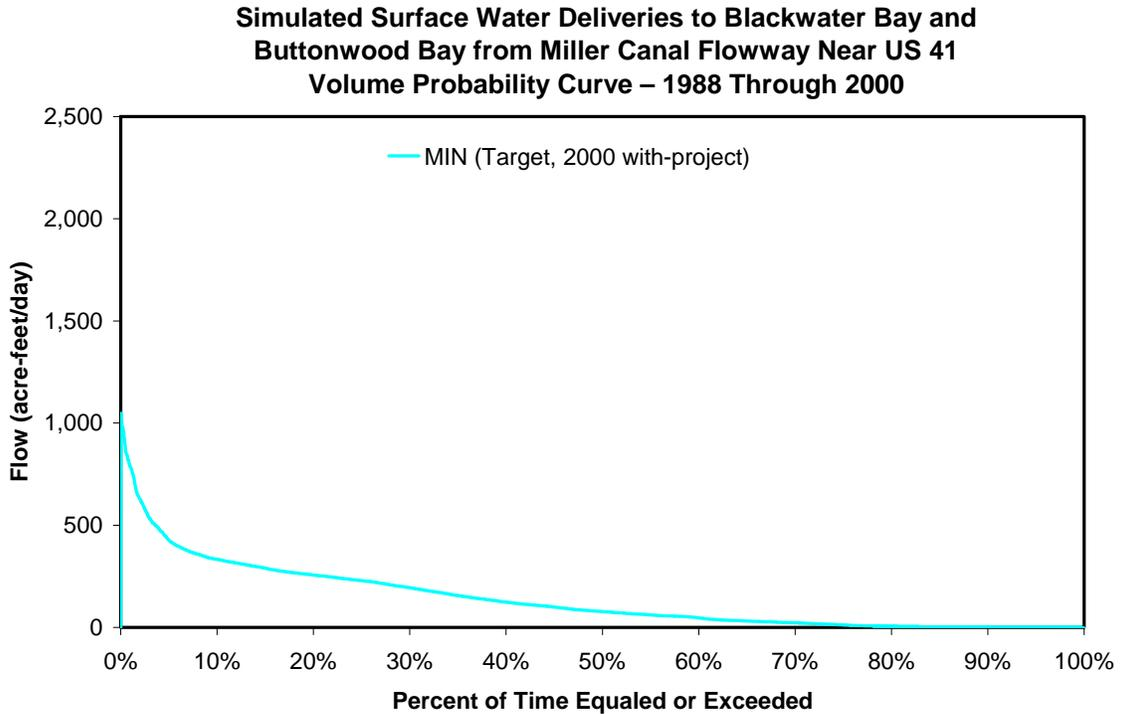
Figure 78. Volume probability curve for surface water inflow along the Miller Canal flowway to be reserved for the period of record (1988 - 2000)
