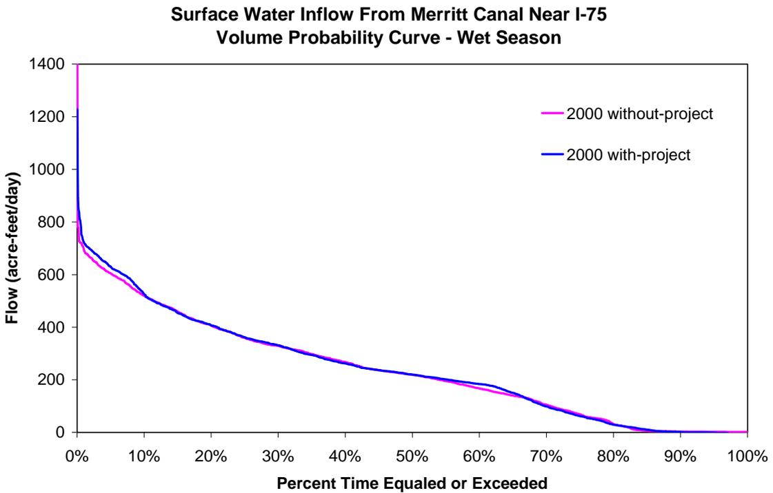
Figure 52. Volume probability curve for surface water deliveries into Picayune Strand Restoration Area from the Merritt Canal for the wet seasons during the period of record (1988 - 2000)
