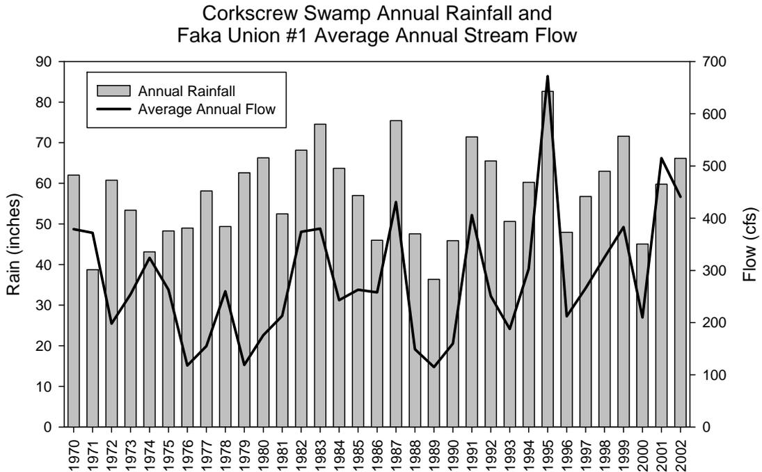
Figure 36. Annual variability of rainfall versus stream flow in the Faka Union Canal watershed
