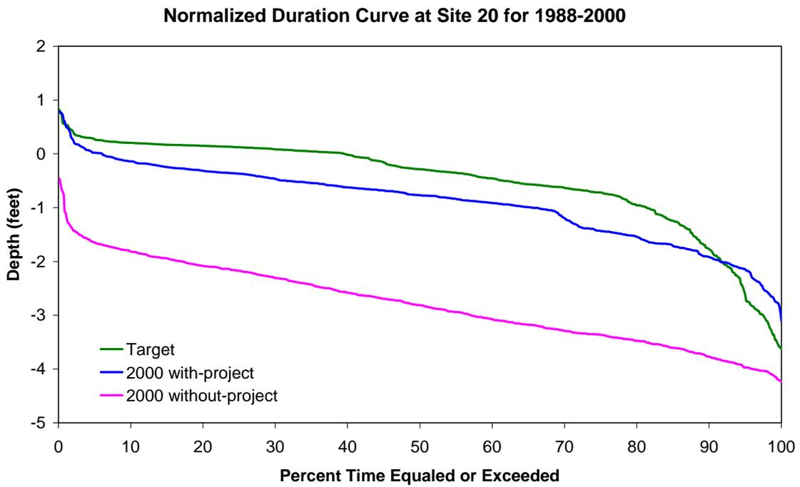
Figure A-53. Normalized duration curve at Site 20 for 1988 to 2000
