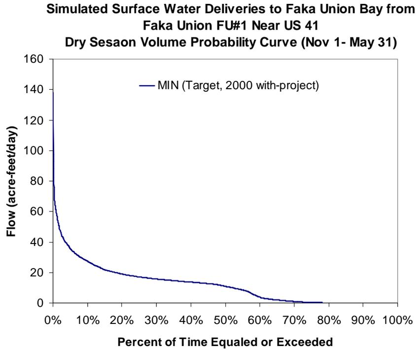
Figure 92. Volume probability curve for surface water inflow from from the FU1 weir on Faka Union Canal to be reserved for the dry seasons during the period of record (1988 - 2000)
