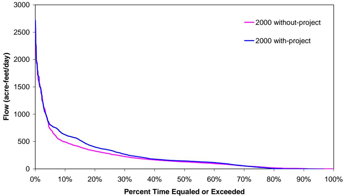
Figure 49. Volume probability curve for surface water deliveries into Picayune Strand Restoration Area from the Faka Union Canal for the wet seasons during the period of record (1988 - 2000)
