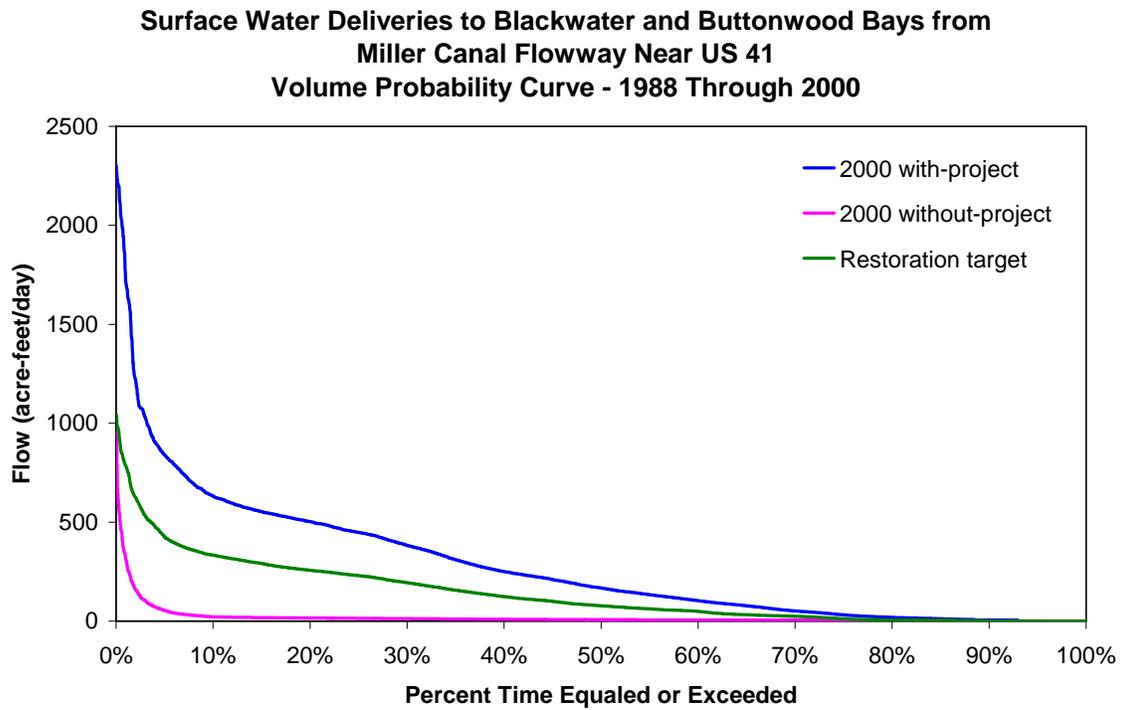
Figure 54. Volume probability curve for surface water inflow along the Miller Canal flowway near US 41 for the entire period of record (1988 - 2000)
