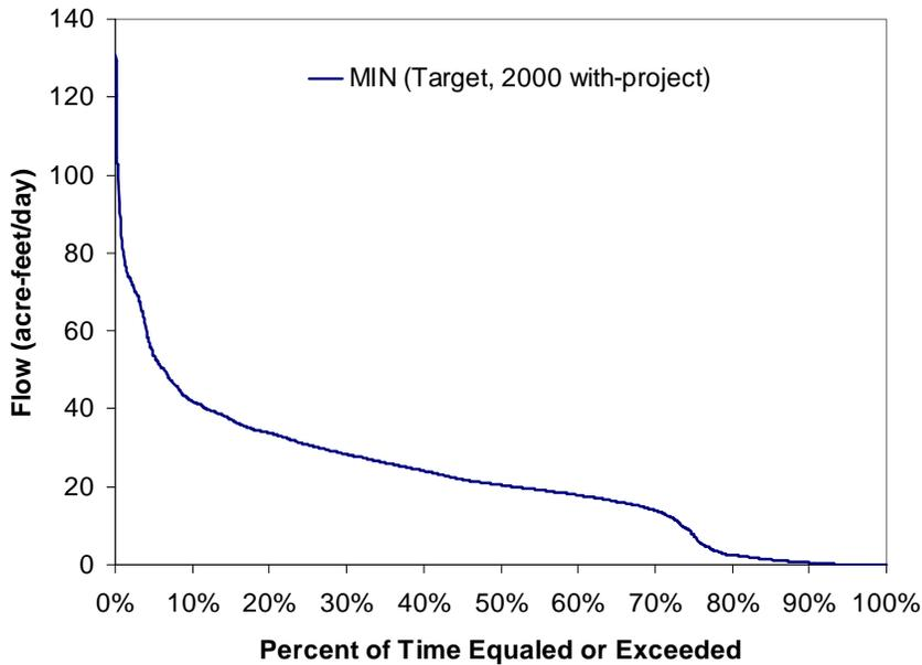
Figure 91. Volume probability curve for surface water inflow from from the FU1 weir on Faka Union Canal to be reserved for the wet seasons during the period of record (1988 - 2000)
