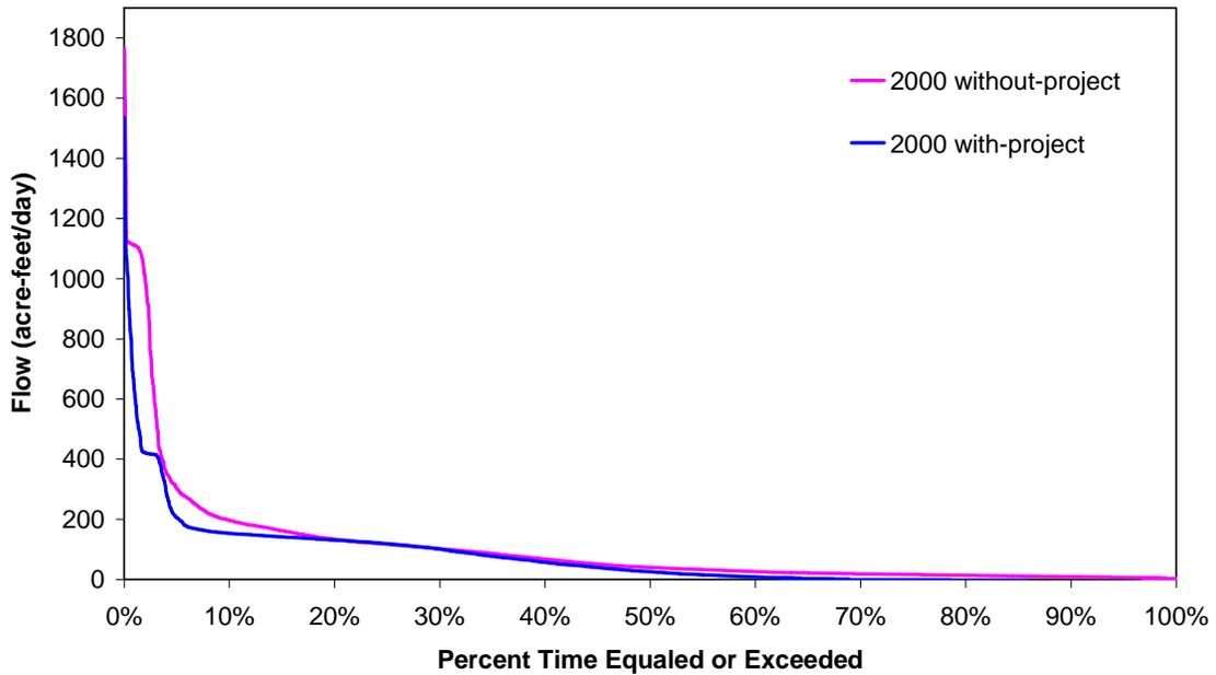
Figure 45. Volume probability curve for surface water deliveries into Picayune Strand Restoration Area from the Miller Canal for the entire period of record (1988 - 2000)
