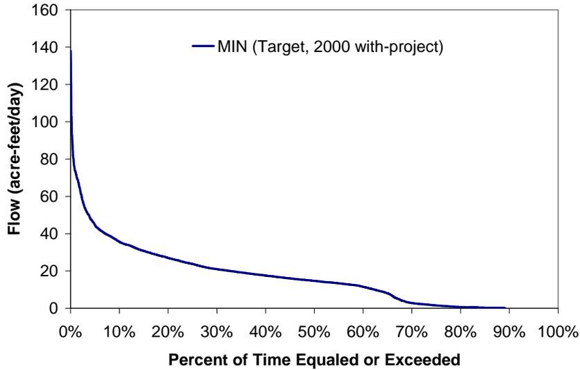
Figure 90. Volume probability curve for surface water inflow from from the FU1 weir on Faka Union Canal to be reserved for the period of record (1988 - 2000)
