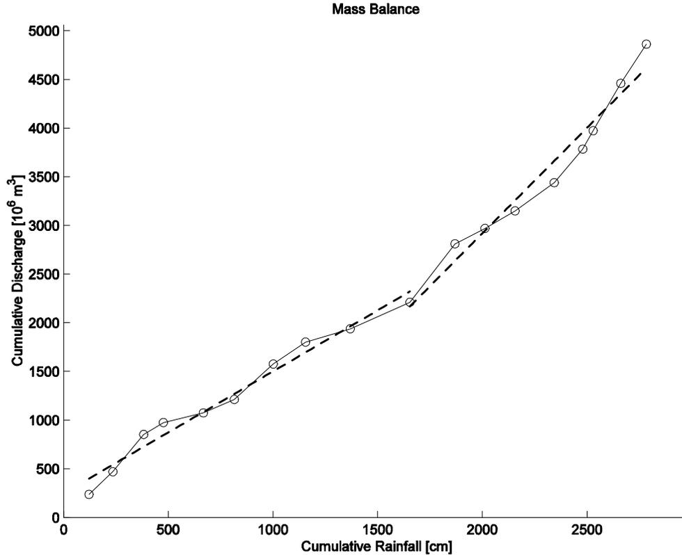
Figure 19. Mass balance curve with the tendency of the data, after fitting a straight line,  $y = ax + b$ , indicated by the dashed line in the figure
