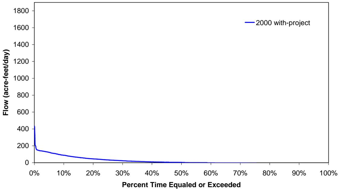
Figure 71. Volume probability curve for surface water deliveries into Picayune Strand Restoration Area from the Miller Canal to be reserved for the dry seasons
