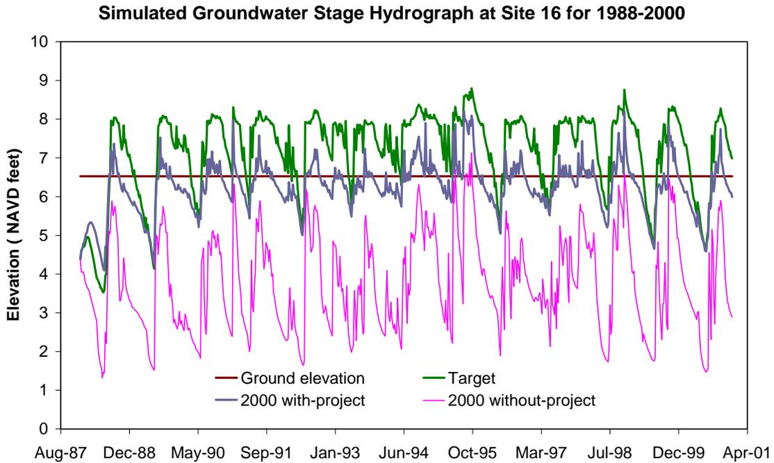
Figure A-17. Simulated groundwater stage hydrograph at Site 16 for 1988 to 2000
