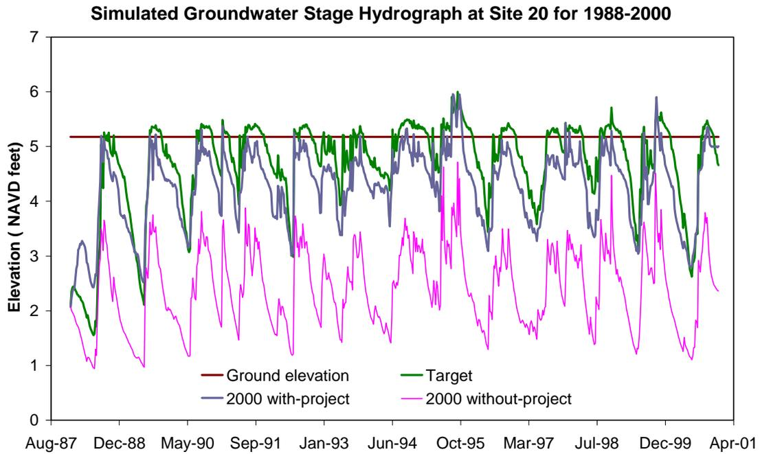
Figure A-21. Simulated groundwater stage hydrograph at Site 20 for 1988 to 2000
