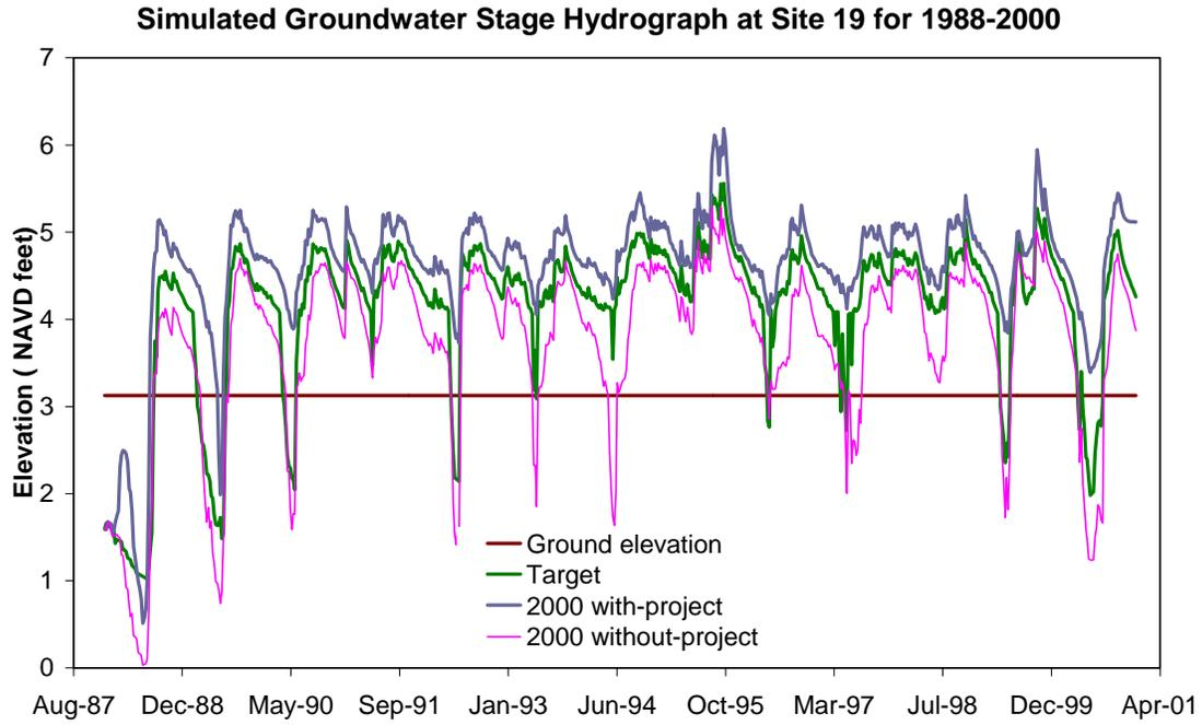
Figure A-20. Simulated groundwater stage hydrograph at Site 19 for 1988 to 2000
