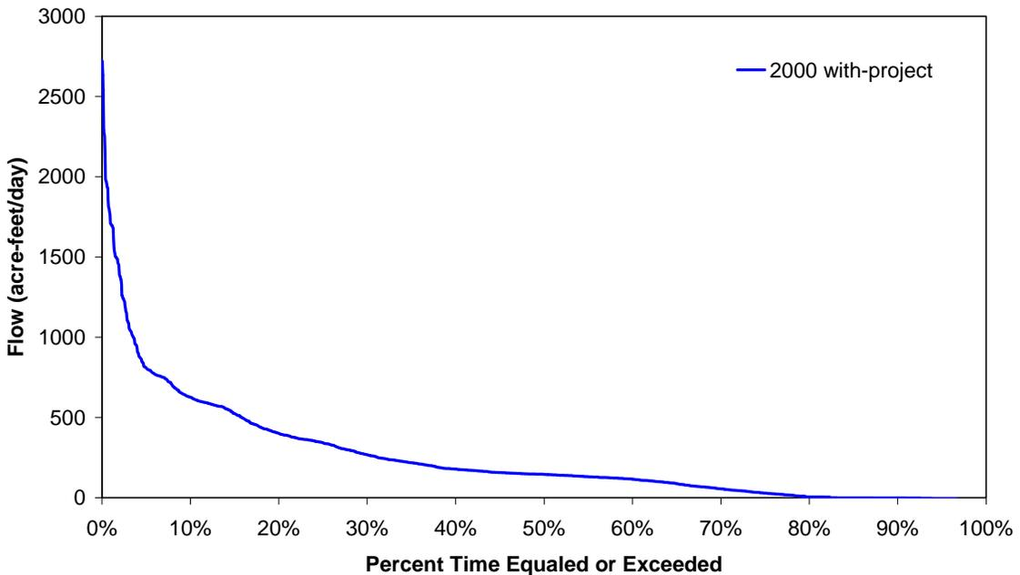
Figure 73. Volume probability curve for surface water deliveries into Picayune Strand Restoration Area from the Faka Union Canal to be reserved for the wet seasons
