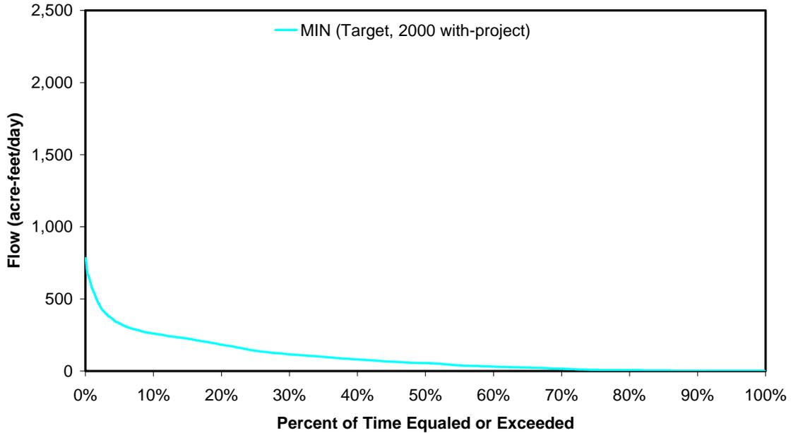
Figure 80. Volume probability curve for surface water inflow along the Miller Canal flowway to be reserved for the dry seasons during the period of record (1988 - 2000)
