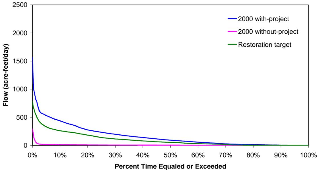
Figure 56. Volume probability curve for surface water inflow along the Miller Canal flowway near US 41 for the dry season during the period of record (1988 - 2000)
