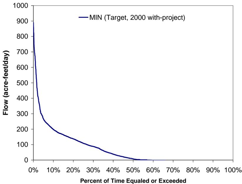
Figure 81. Volume probability curve for surface water inflow along the Faka Union Canal flowway to be reserved for the period of record (1988 - 2000)
