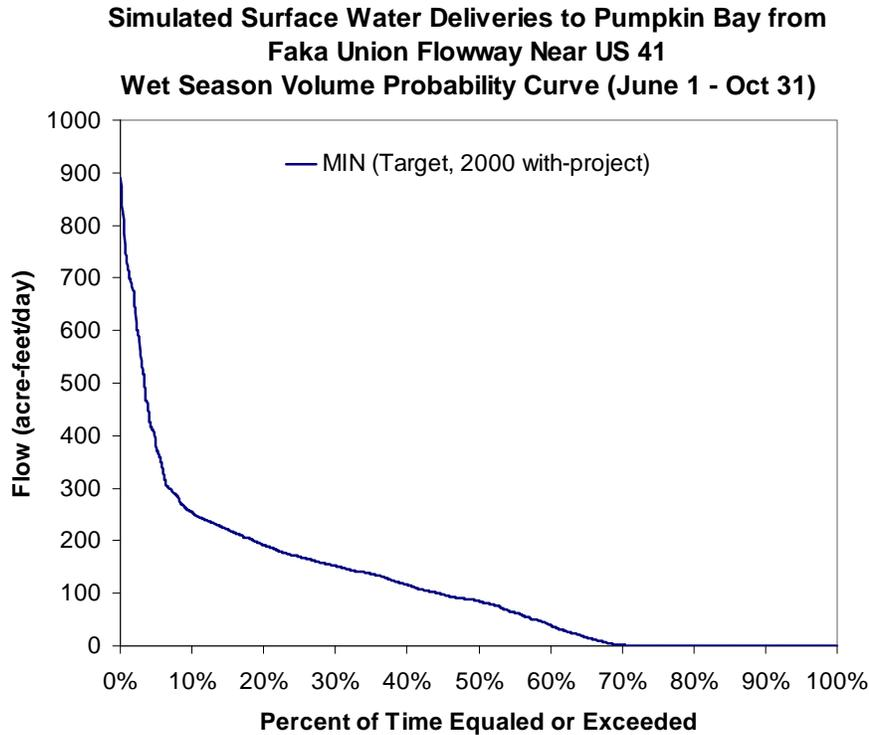
Figure 82. Volume probability curve for surface water inflow along the Faka Union Canal flowway to be reserved for the wet seasons during the period of record (1988 - 2000)
