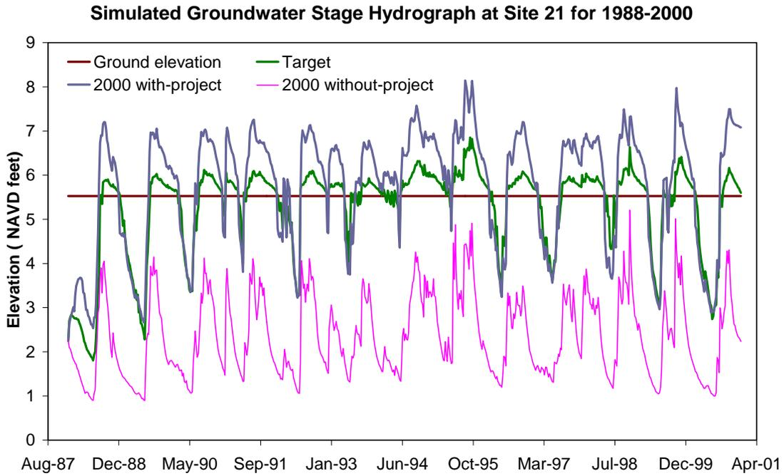
Figure A-22. Simulated groundwater stage hydrograph at Site 21 for 1988 to 2000
