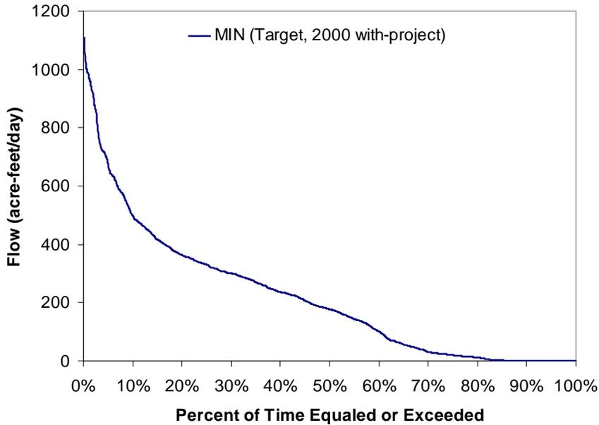
Figure 85. Volume probability curve for surface water inflow along the Merritt Canal flowway to be reserved for the wet seasons during the period of record (1988 - 2000)
