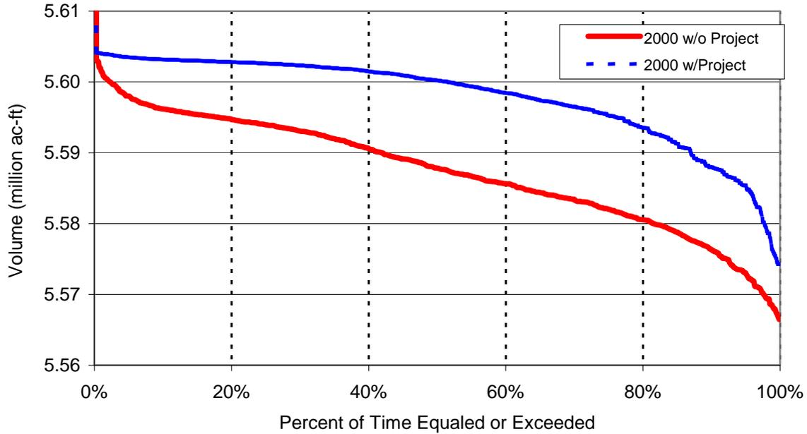
Figure 44. Groundwater storage volume probability 1988-2000
