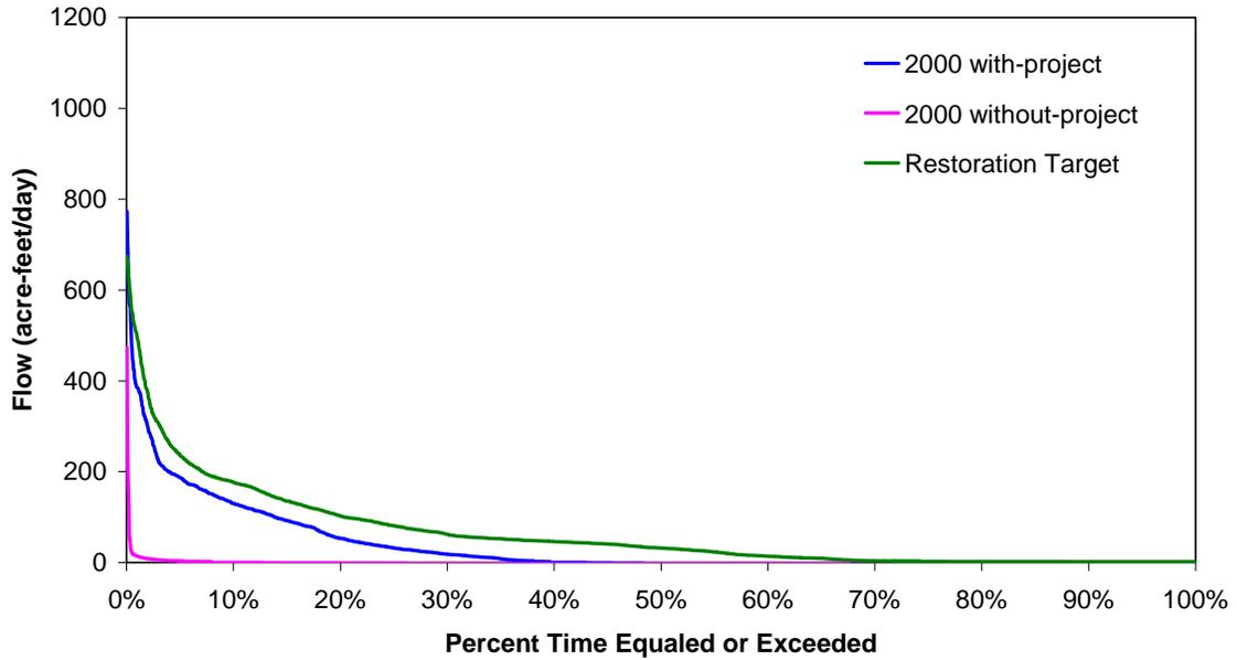
Figure 59. Volume probability curve for surface water inflow along the Faka Union Canal flowway near US 41 for the dry season during the period of record (1988 - 2000)
