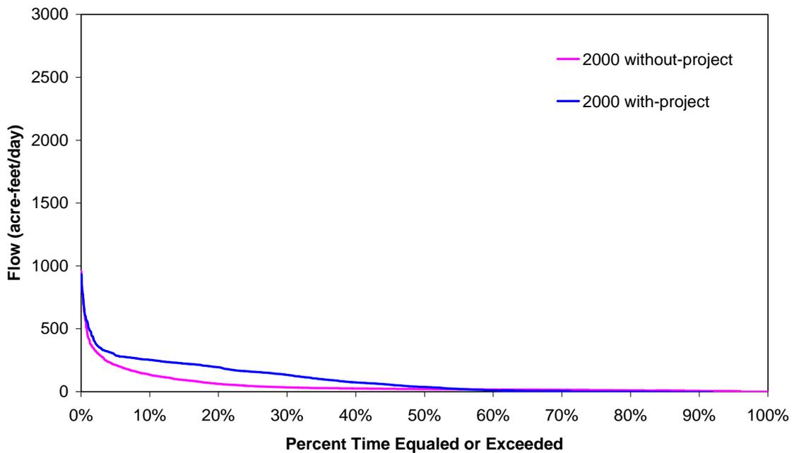
Figure 50. Volume probability curve for surface water deliveries into Picayune Strand Restoration Area from the Faka Union Canal for the dry seasons during the period of record (1988 - 2000)
