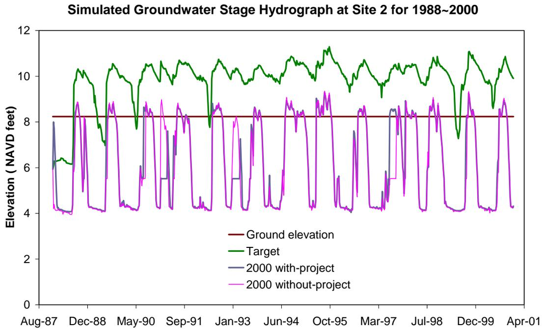
Figure A-3. Simulated groundwater stage hydrograph at Site 2 for 1988 to 2000
