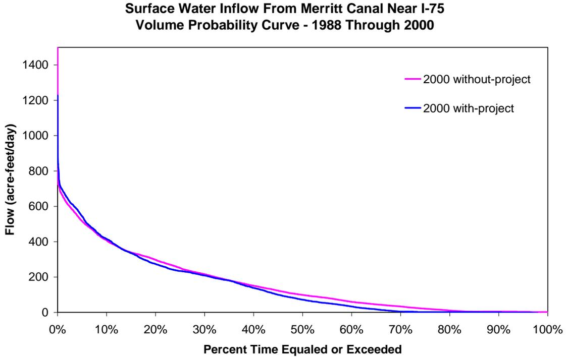
Figure 51. Volume probability curve for surface water deliveries into Picayune Strand Restoration Area from the Merritt Canal for the entire period of record (1988 - 2000)
