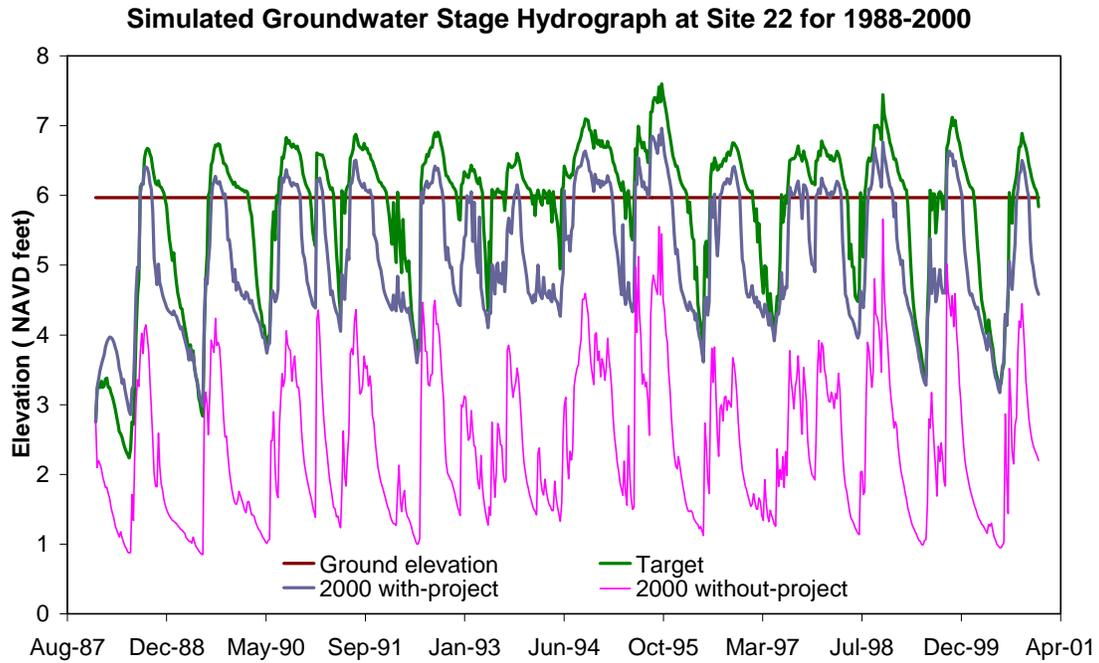
Figure A-23. Simulated groundwater stage hydrograph at Site 22 for 1988 to 2000
