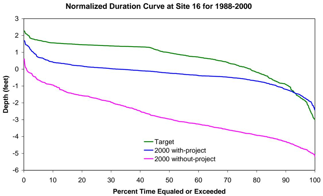
Figure A-49. Normalized duration curve at Site 16 for 1988 to 2000
