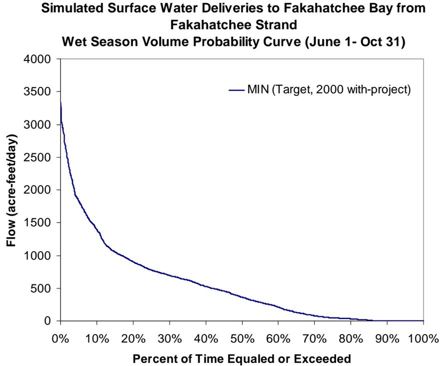
Figure 88. Volume probability curve for surface water inflow from Fakahatchee Strand to be reserved for the wet seasons during the period of record (1988 - 2000)
