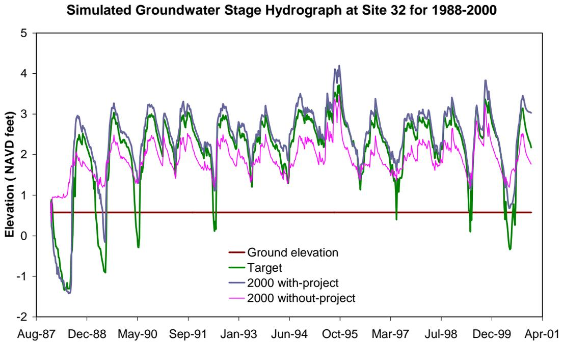
Figure A-33. Simulated groundwater stage hydrograph at Site 32 for 1988 to 2000
