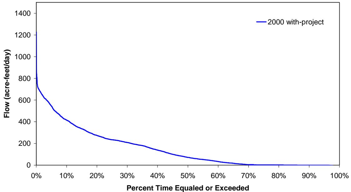
Figure 75. Volume probability curve of surface water deliveries into Picayune Strand Restoration Area from the Merritt Canal to be reserved
