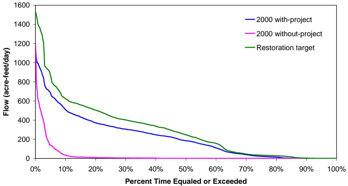
Figure 61. Volume probability curve for surface water inflow along the Merritt Canal flowway near US 41 for the wet season for the period of record (1988 -2000)
