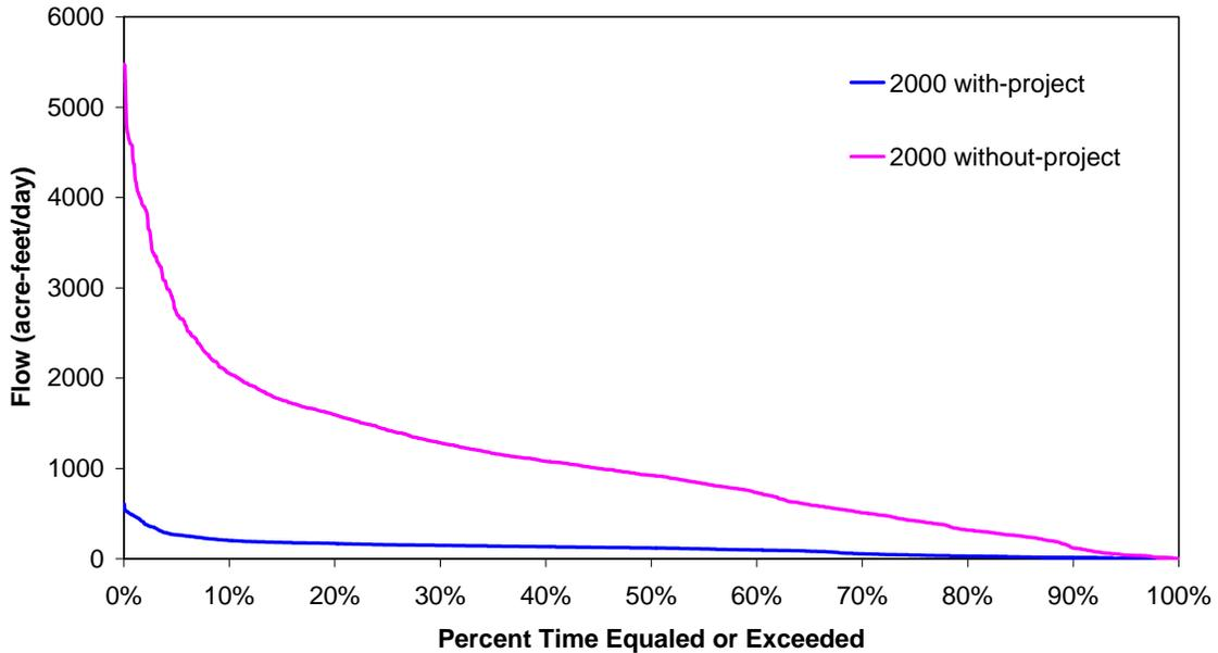
Figure 67. Volume probability curve for surface water inflow from the FU1 weir on Faka Union Canal for the wet season during the period of record (1988 - 2000)
