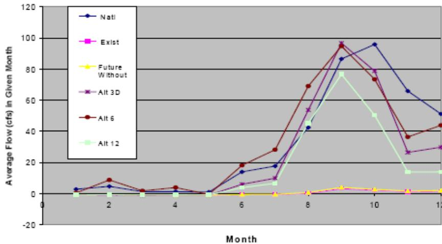
Figure 23. Total monthly water flows into Pumpkin Bay predicted by the various modeled alternatives
