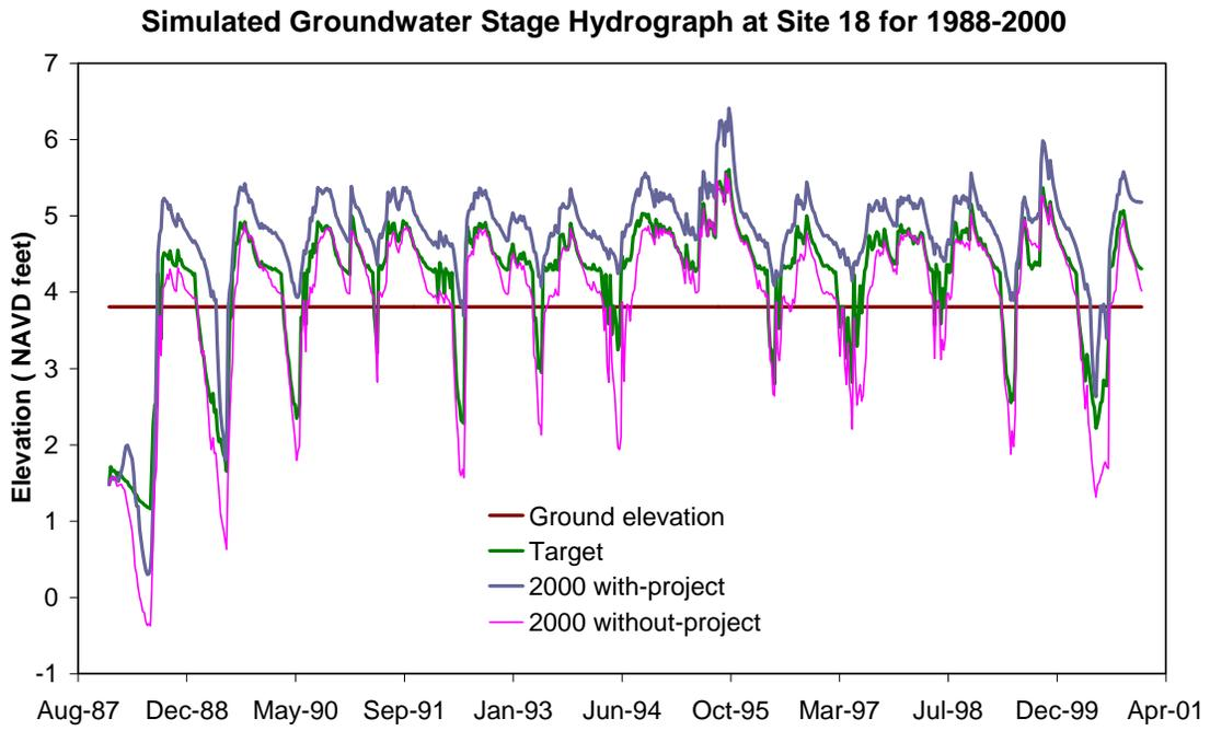
Figure A-19. Simulated groundwater stage hydrograph at Site 18 for 1988 to 2000
