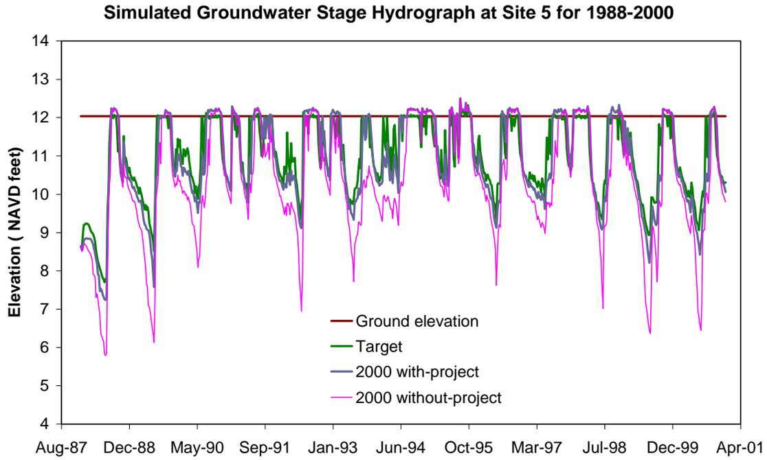
Figure A-6. Simulated groundwater stage hydrograph at Site 5 for 1988 to 2000
