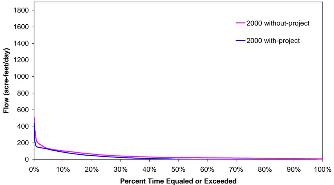
Figure 47. Volume probability curve for surface water deliveries into Picayune Strand Restoration Area from the Miller Canal for the dry seasons during the period of record (1988 - 2000)
