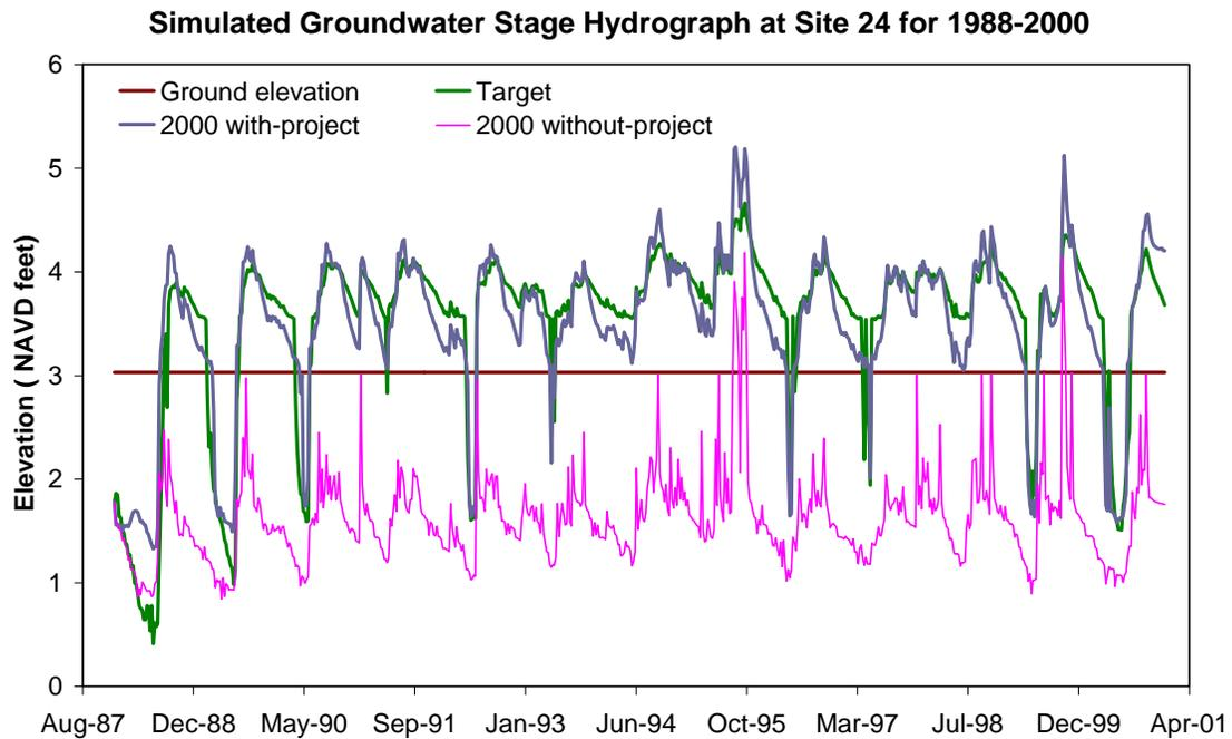
Figure A-25. Simulated groundwater stage hydrograph at Site 24 for 1988 to 2000
