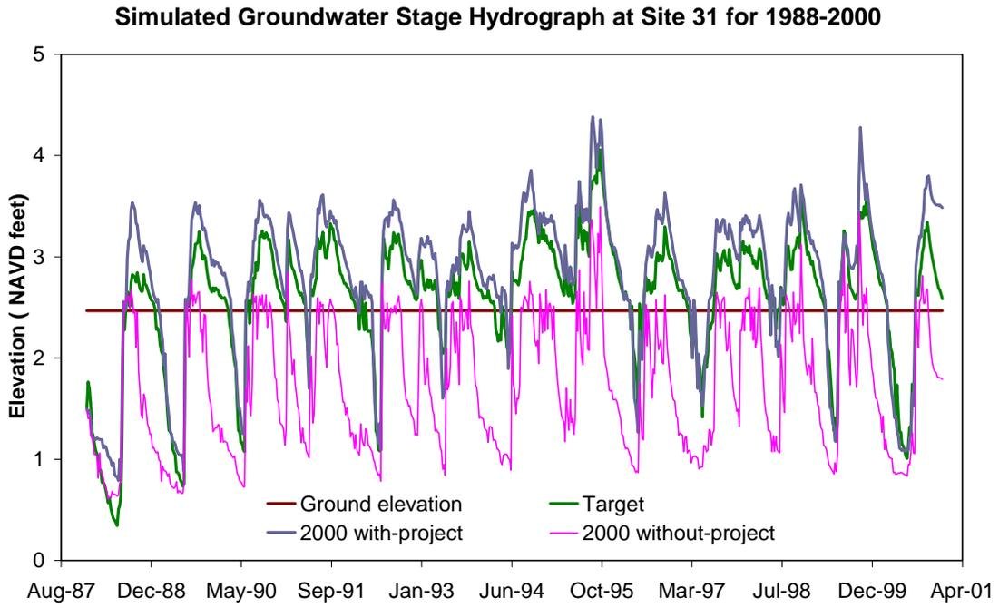
Figure A-32. Simulated groundwater stage hydrograph at Site 31 for 1988 to 2000
