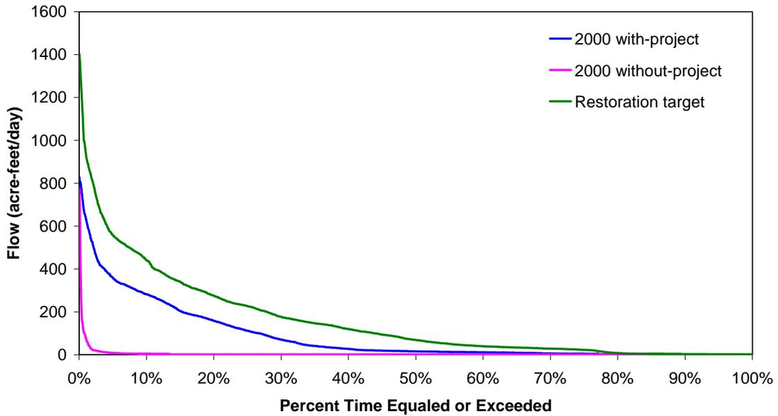
Figure 62. Volume probability curve for surface water inflow along the Merritt Canal flowway near US 41 for the dry season during the period of record (1988 - 2000)
