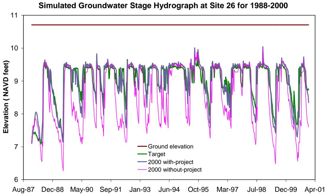
Figure A-27. Simulated groundwater stage hydrograph at Site 26 for 1988 to 2000
