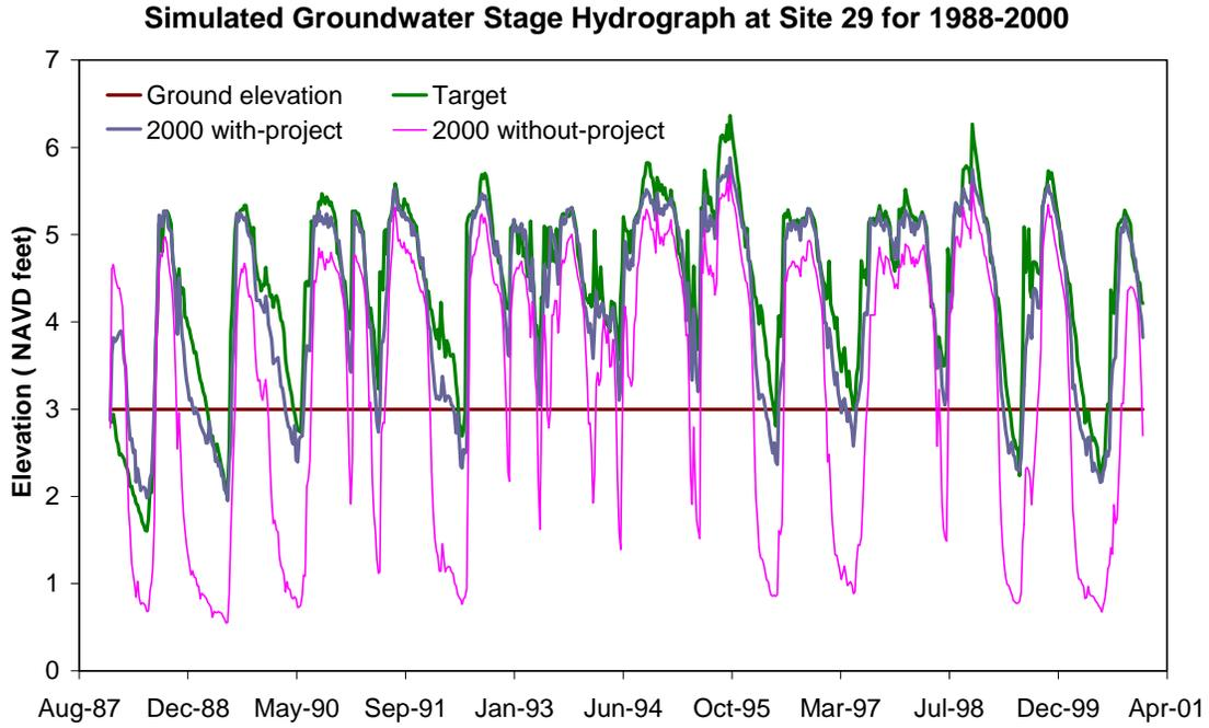
Figure A-30. Simulated groundwater stage hydrograph at Site 29 for 1988 to 2000
