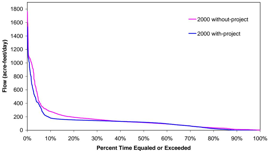
Figure 46. Volume probability curve for surface water deliveries into Picayune Strand Restoration Area from the Miller Canal for the wet seasons during the period of record (1988 - 2000)
