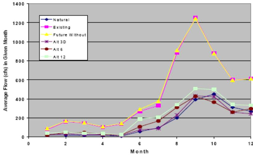
Figure 22. Total monthly water flows into Faka Union Bay predicted by the various modeled alternatives
