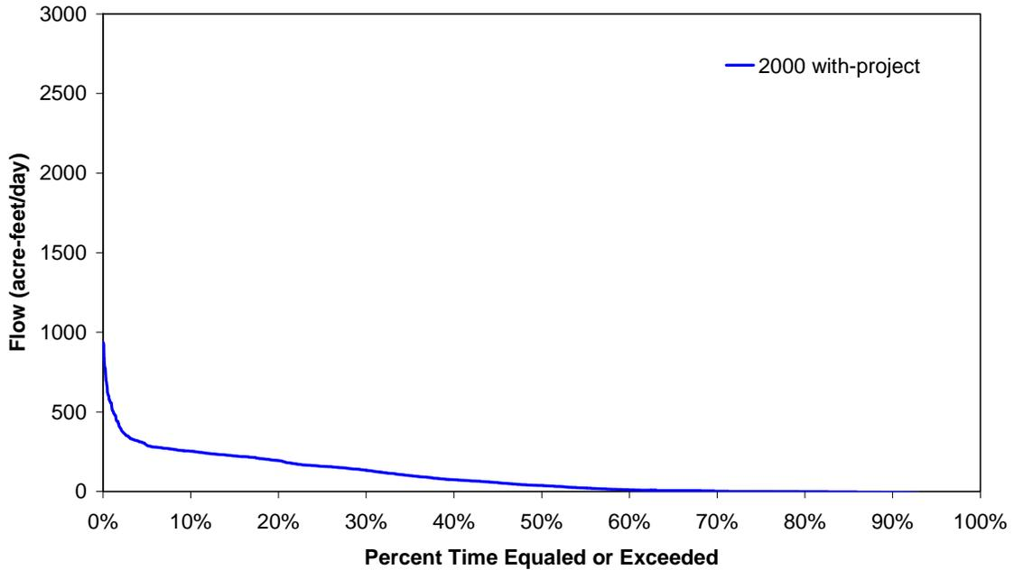
Figure 74. Volume probability curve for surface water deliveries into Picayune Strand Restoration Area from the Faka Union Canal to be reserved for the dry seasons
