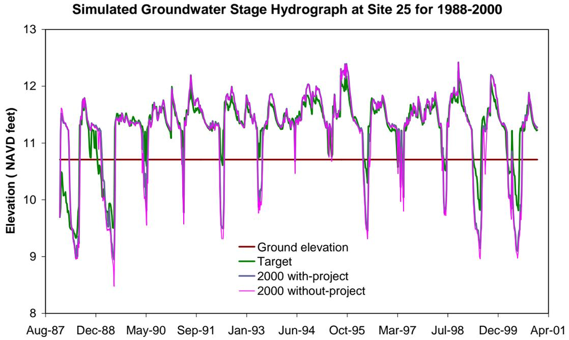
Figure A-26. Simulated groundwater stage hydrograph at Site 25 for 1988 to 2000
