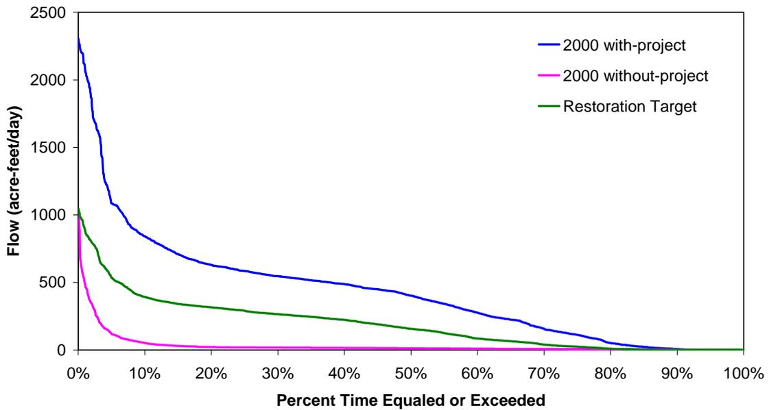
Figure 55. Volume probability curve for surface water inflow along the Miller Canal flowway near US 41 for the wet season for the period of record (1988 - 2000)
