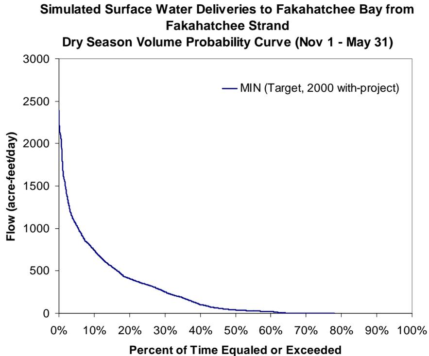
Figure 89. Volume probability curve for surface water inflow from Fakahatchee Strand to be reserved for the dry seasons during the period of record (1988- 2000)
