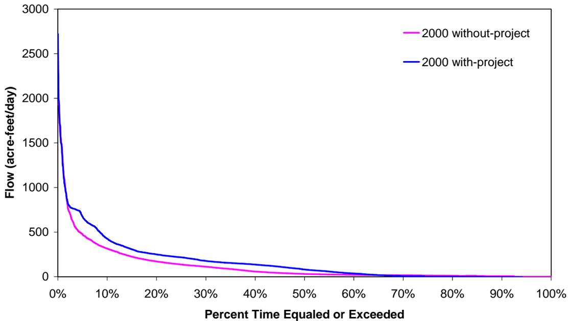
Figure 48. Volume probability curve for surface water deliveries into Picayune Strand Restoration Area from the Faka Union Canal for the entire period of record (1988 - 2000)
