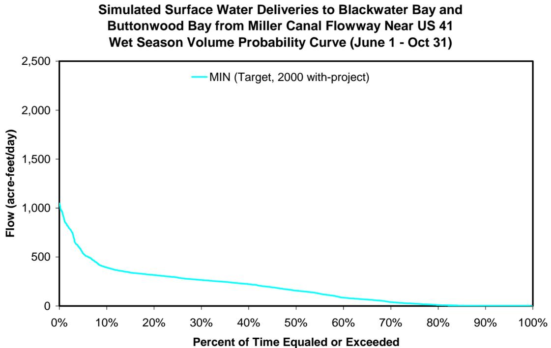
Figure 79. Volume probability curve for surface water inflow along the Miller Canal flowway to be reserved for the wet seasons during the period of record (1988 - 2000)
