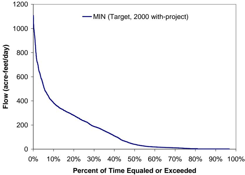
Figure 84. Volume probability curve for surface water inflow along the Merritt Canal flowway to be reserved for the period of record (1988 - 2000)
