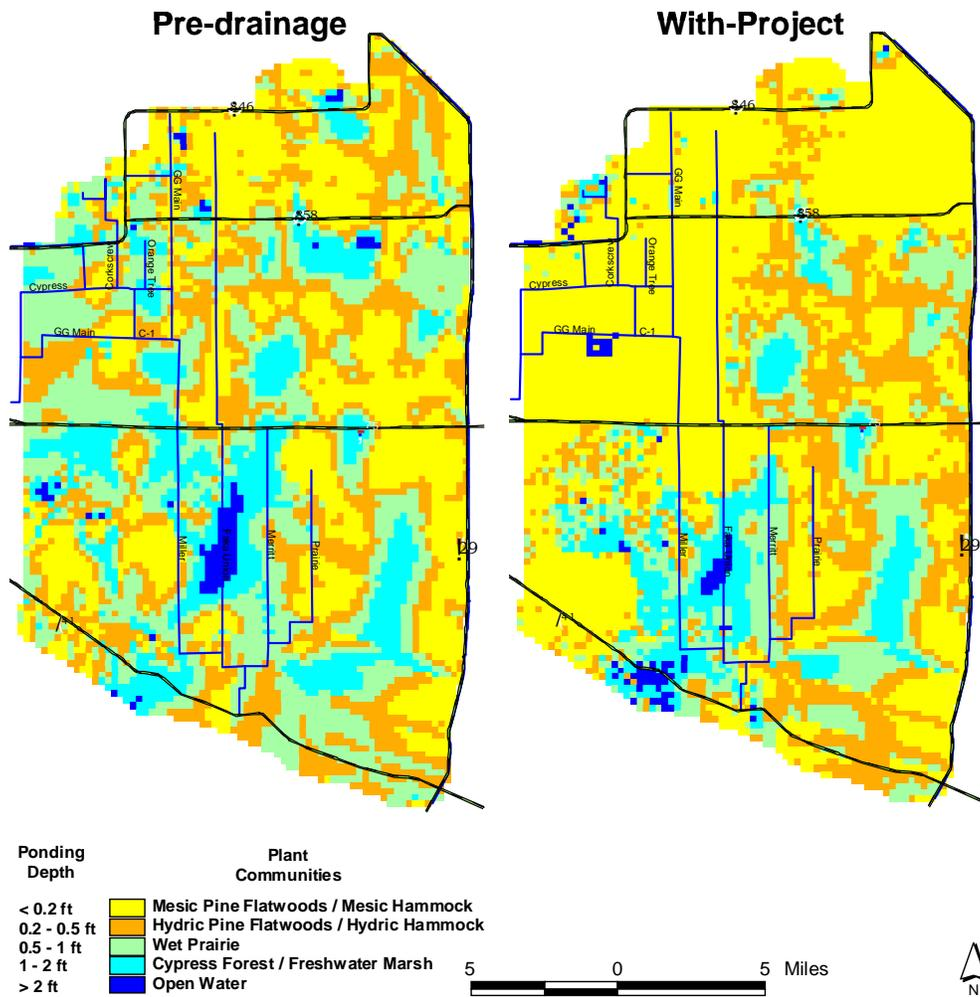
Figure 29. Pre-drainage and 2000 with-project average wet season water depths and corresponding plant community types
