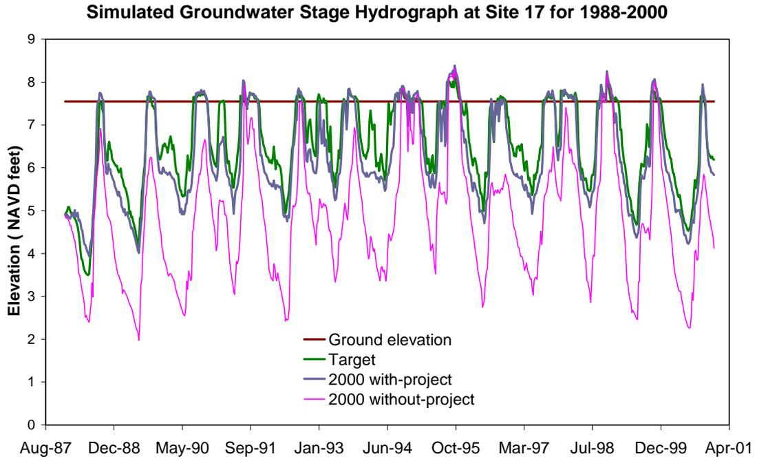
Figure A-18. Simulated groundwater stage hydrograph at Site 17 for 1988 to 2000
