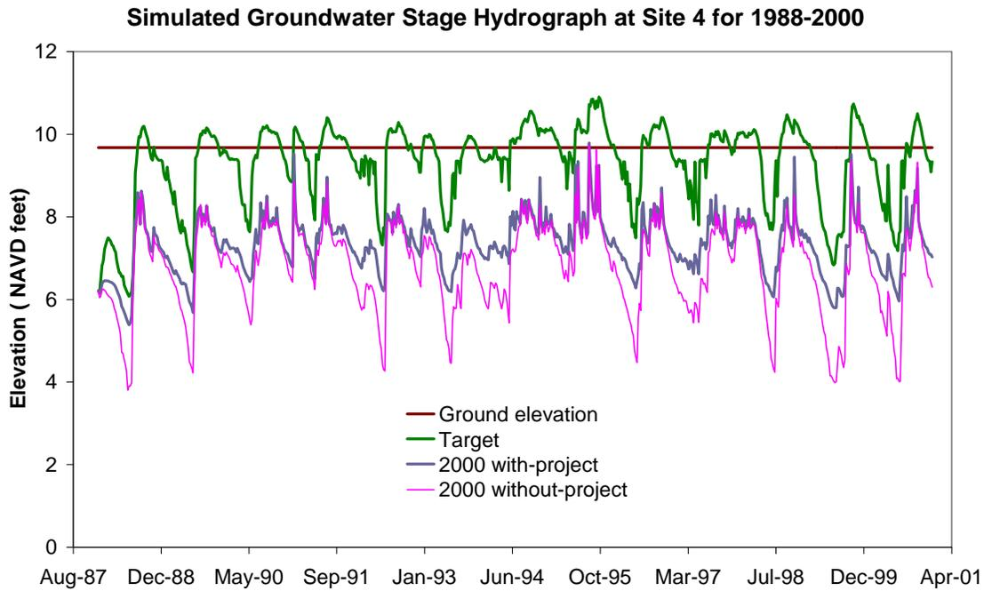
Figure A-5. Simulated groundwater stage hydrograph at Site 4 for 1988 to 2000
