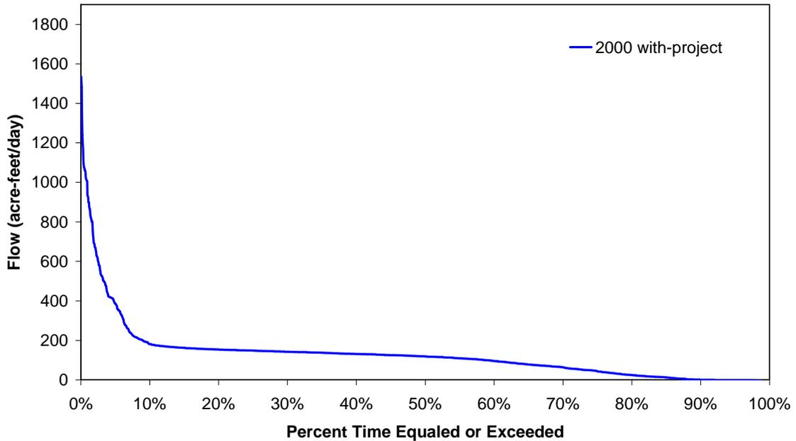
Figure 70. Volume probability curve for surface water deliveries into Picayune Strand Restoration Area from the Miller Canal to be reserved for the wet seasons
