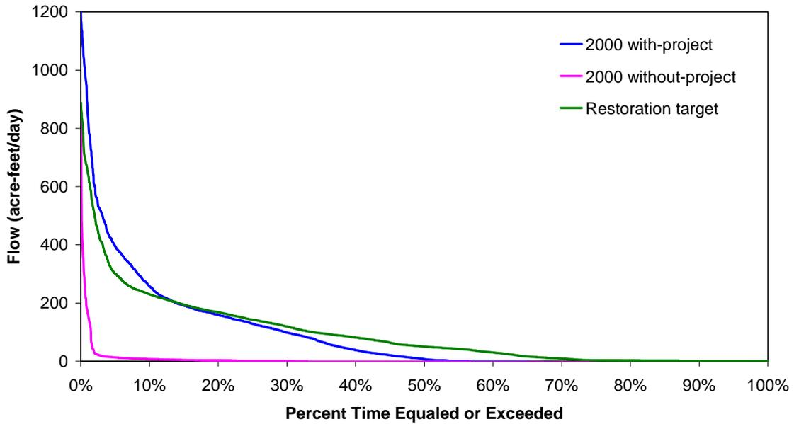
Figure 57. Volume probability curve for surface water inflow along the Faka Union Canal flowway near US 41 for the entire period of record (1988 - 2000)
