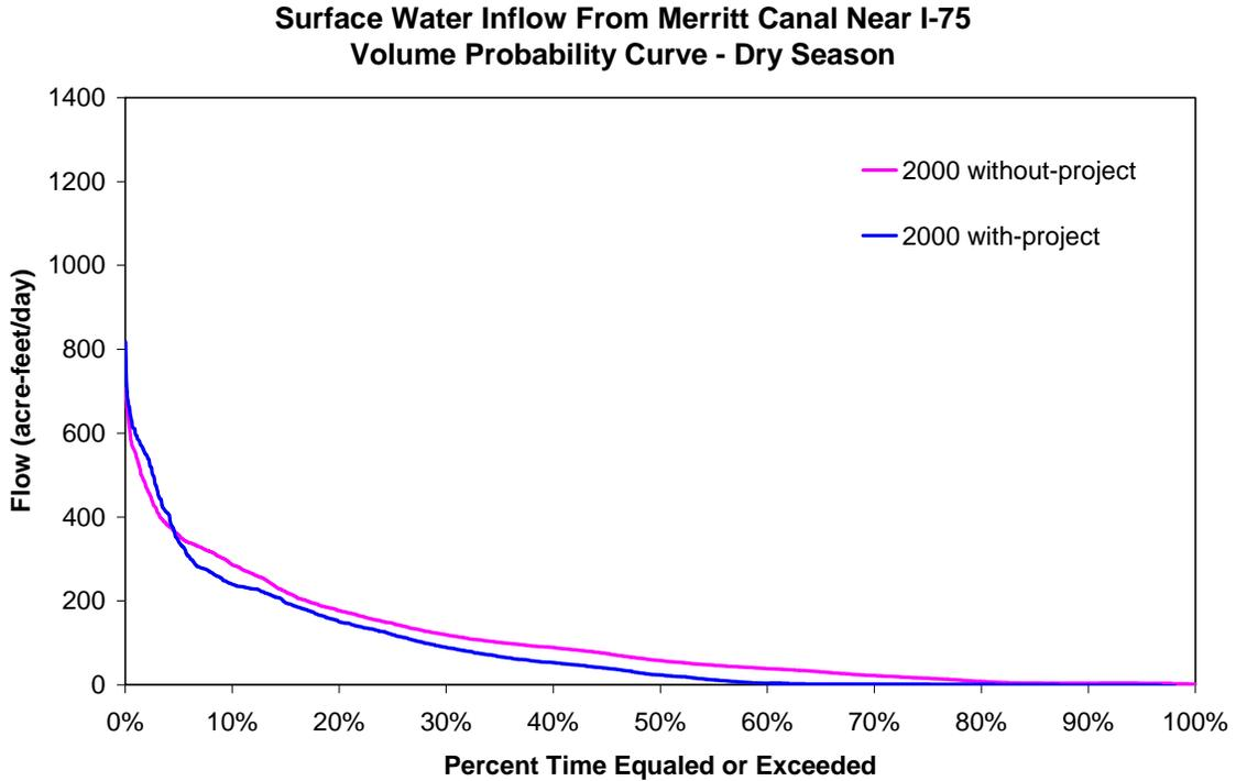
Figure 53. Volume probability curve for surface water deliveries into Picayune Strand Restoration Area from the Merritt Canal for the dry seasons during the period of record (1988 -2000)
