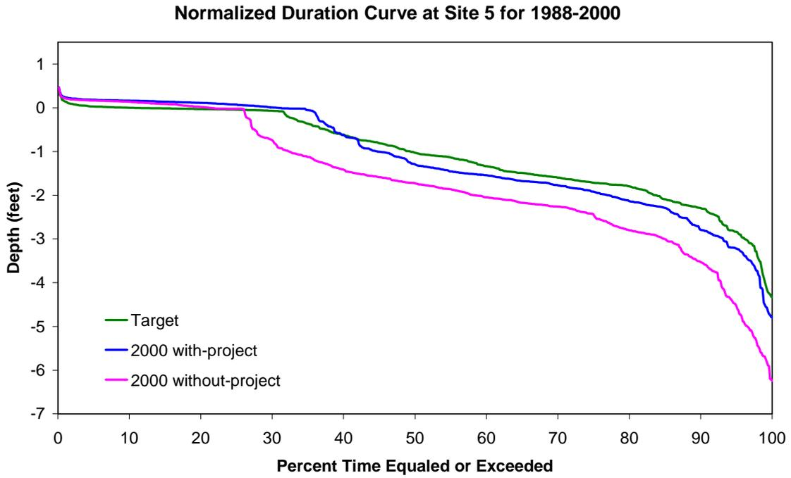
Figure A-38. Normalized duration curve at Site 5 for 1988 to 2000
