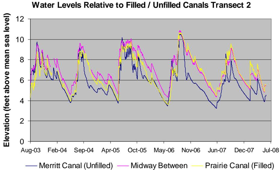
Figure 30. Transect 2 water levels near filled (SWT2W4) and unfilled (SWT2W6) canals
