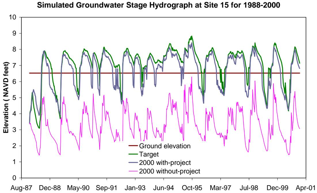
Figure A-16. Simulated groundwater stage hydrograph at Site 15 for 1988 to 2000
