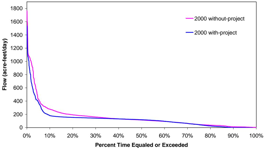
Figure 46. Volume probability curve for surface water deliveries into Picayune Strand Restoration Area from the Miller Canal for the wet seasons during the period of record (1988 - 2000)
