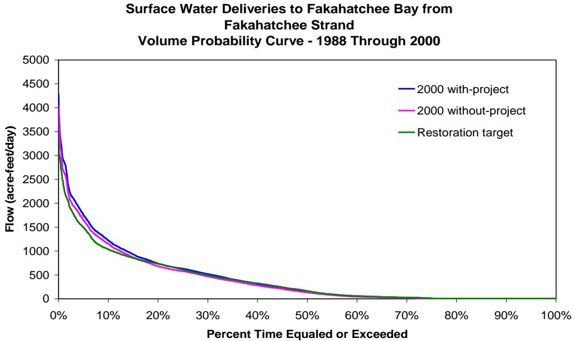
Figure 63. Volume probability curve for surface water inflow from Fakahatchee Strand for the entire period of record (1988 - 2000)
