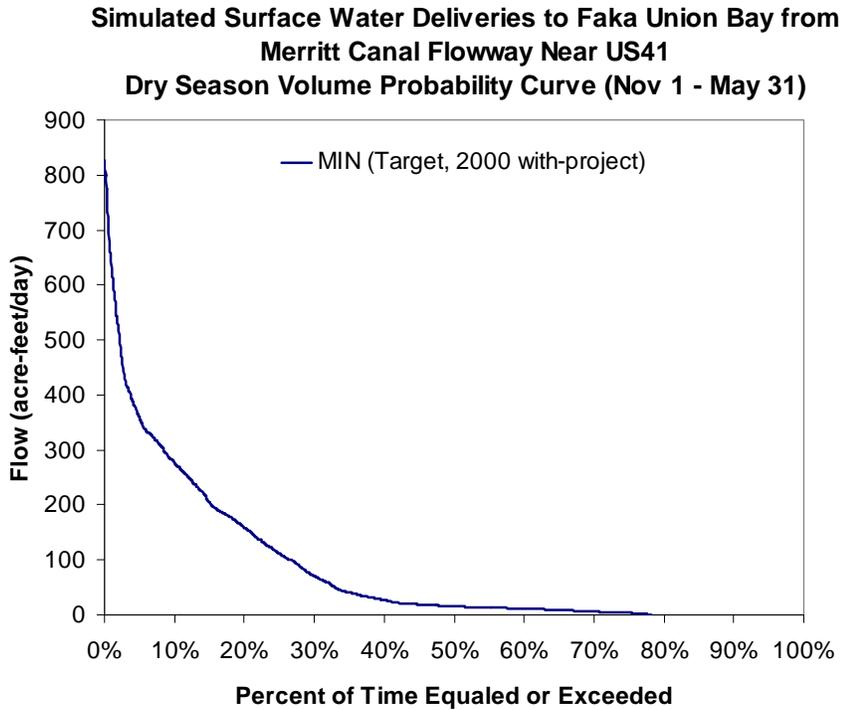
Figure 86. Volume probability curve for surface water inflow along the Merritt Canal flowway to be reserved for the dry seasons during the period of record (1988 - 2000)
