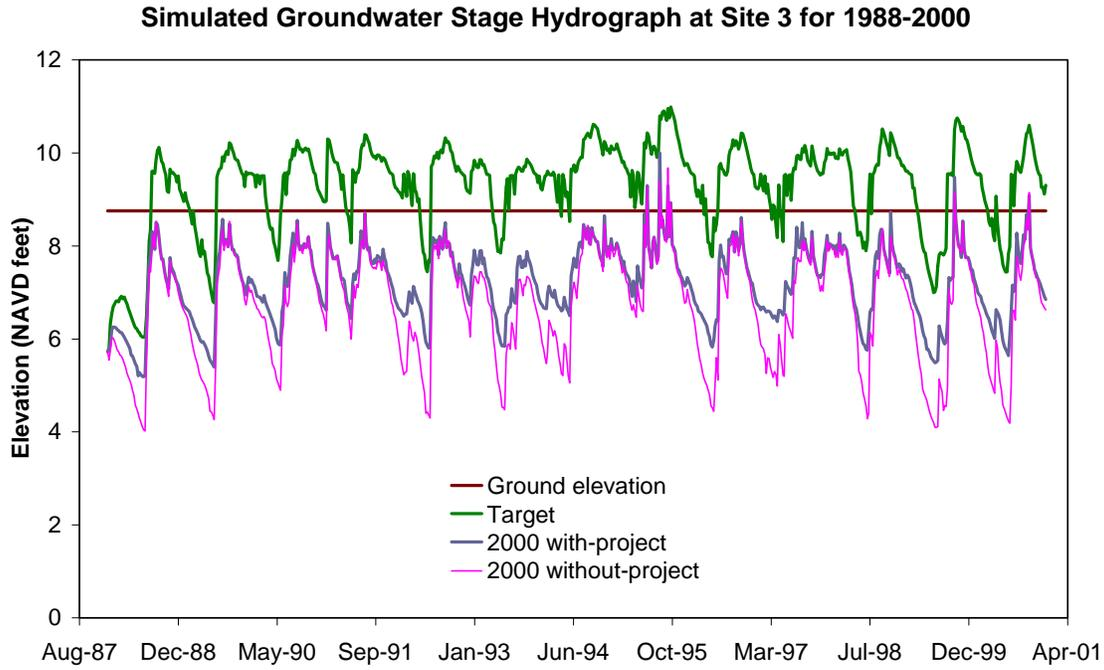
Figure A-4. Simulated groundwater stage hydrograph at Site 3 for 1988 to 2000
