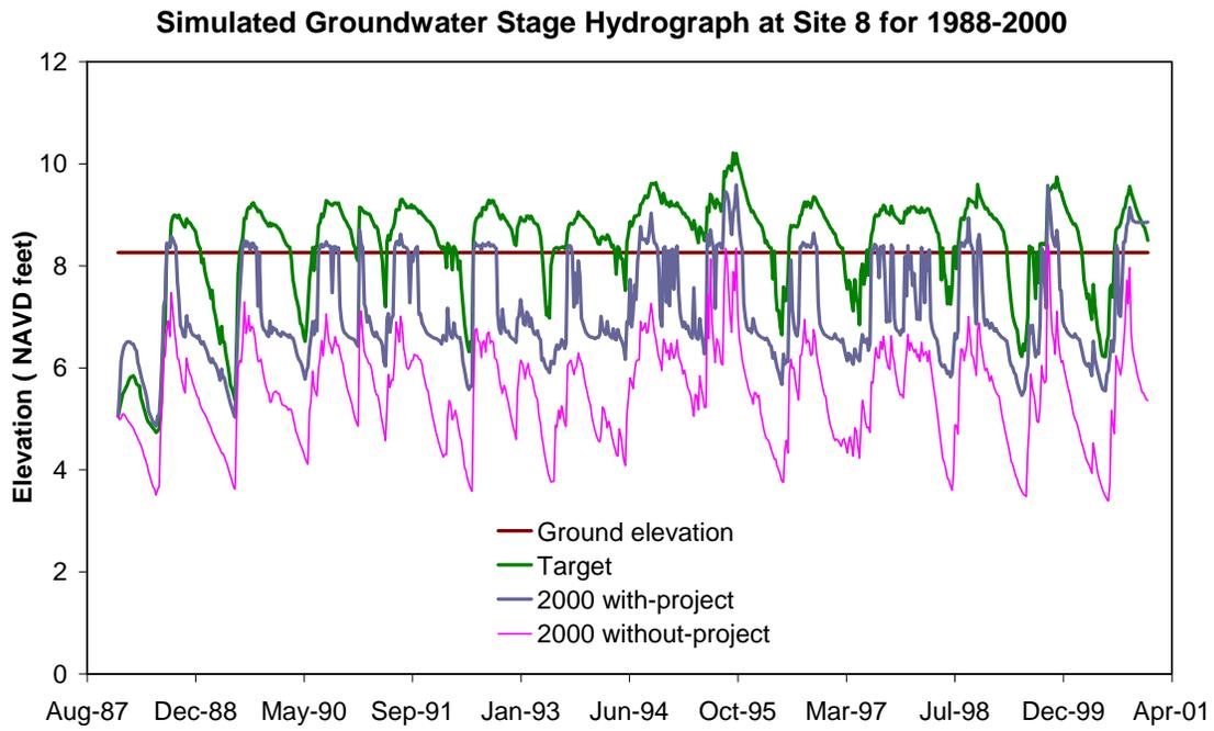
Figure A-9. Simulated groundwater stage hydrograph at Site 8 for 1988 to 2000
