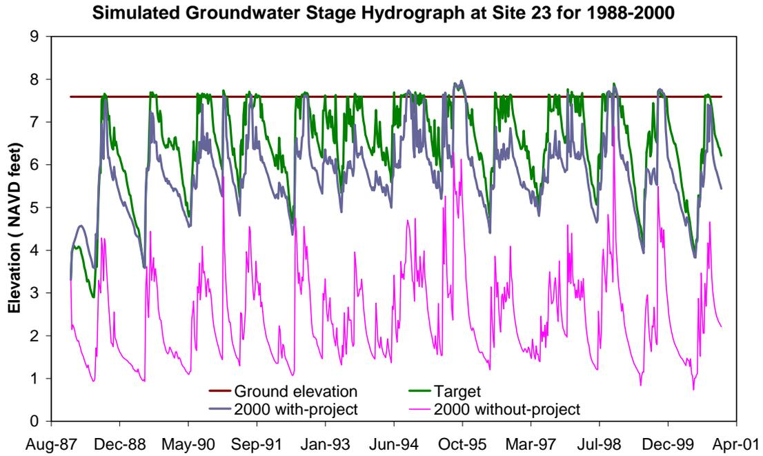
Figure A-24. Simulated groundwater stage hydrograph at Site 23 for 1988 to 2000
