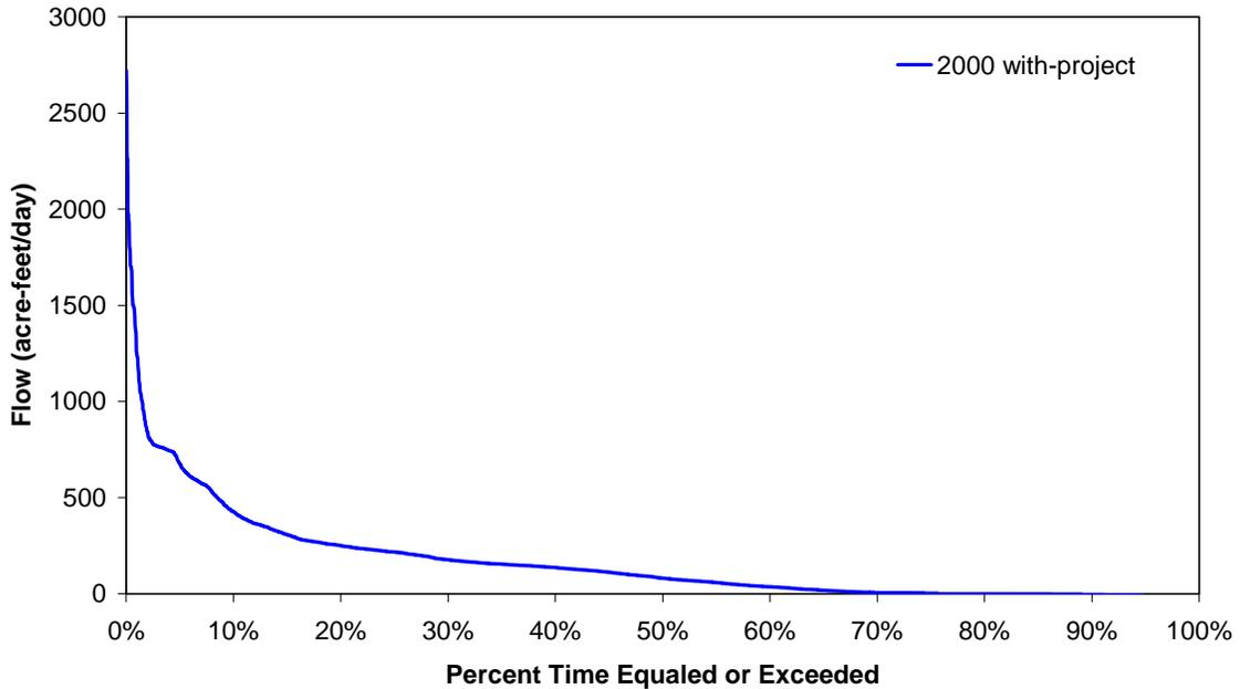
Figure 72. Volume probability curve of surface water deliveries into Picayune Strand Restoration Area from the Faka Union Canal to be reserved
