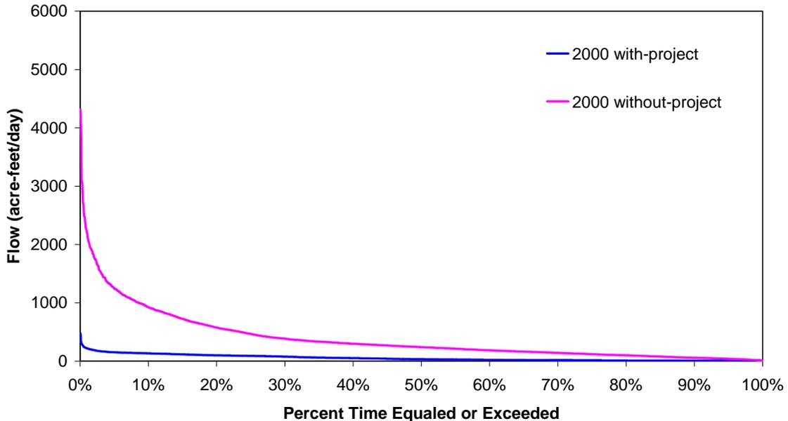
Figure 68. Volume probability curve for surface water inflow from the FU1 weir on Faka Union Canal for the dry season during the period of record (1988- 2000)
