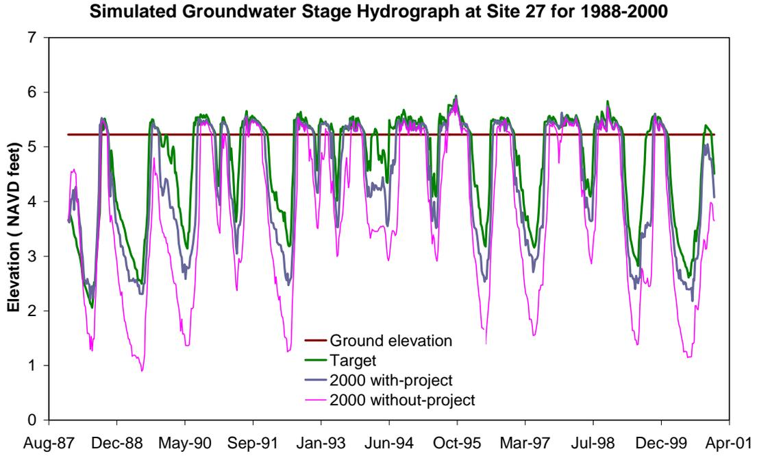
Figure A-28. Simulated groundwater stage hydrograph at Site 27 for 1988 to 2000
