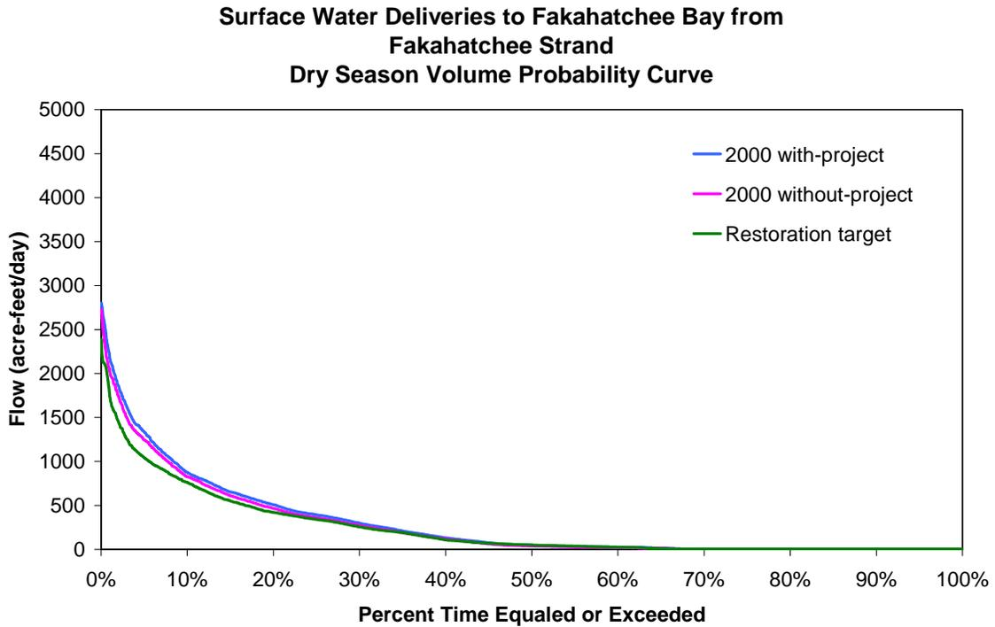
Figure 65. Volume probability curve for surface water inflow from Fakahatchee Strand for the dry season during the period of record (1988 - 2000)
