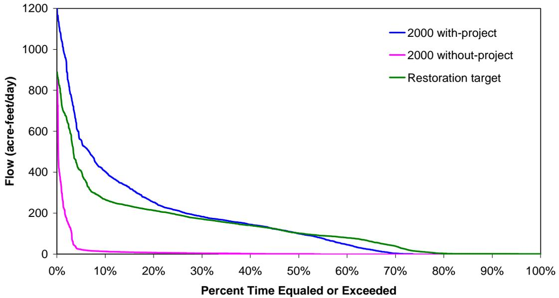
Figure 58. Volume probability curve for surface water inflow along the Faka Union Canal flowway near US 41 for the wet season for the period of record (1988 - 2000)
