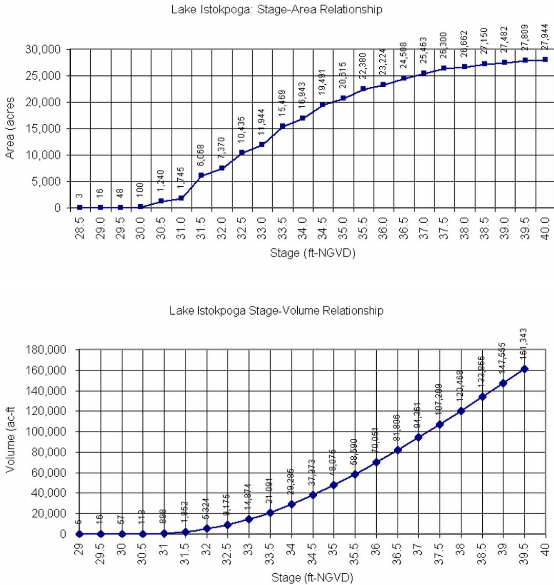
**Figure 14.** Stage vs. Area and Stage vs. Volume for Lake Istokpoga (Source: derived from bathymetry developed by ReMetrix 2003).
