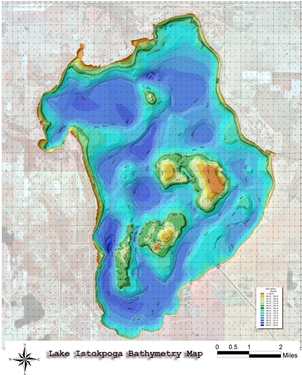
Figure 13. Lake Istokpoga Bathymetric Map (Source: ReMetrix 2003).
