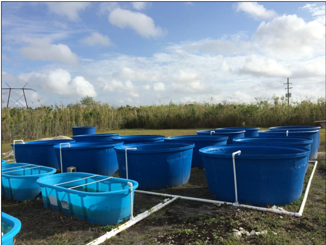
Figure 1. Mesocosms were established at a range of water depths to explore the effects of operating conditions on P removal effectiveness and biological community response. The shorter tanks (to the lower left) were plumbed 4 in-series at water depths of 23 or 46 cm. The larger mesocosms were plumbed 2 in-series and were also established at 46 cm before transitioning to 69 cm or 92 cm water depths.
