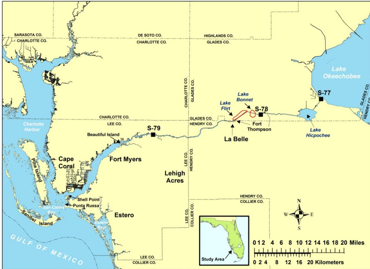
**Figure 3-2.** Caloosahatchee River showing water control structures, connection to Lake Okeechobee, and historical headwaters at Lake Flirt and Lake Bonnet.
