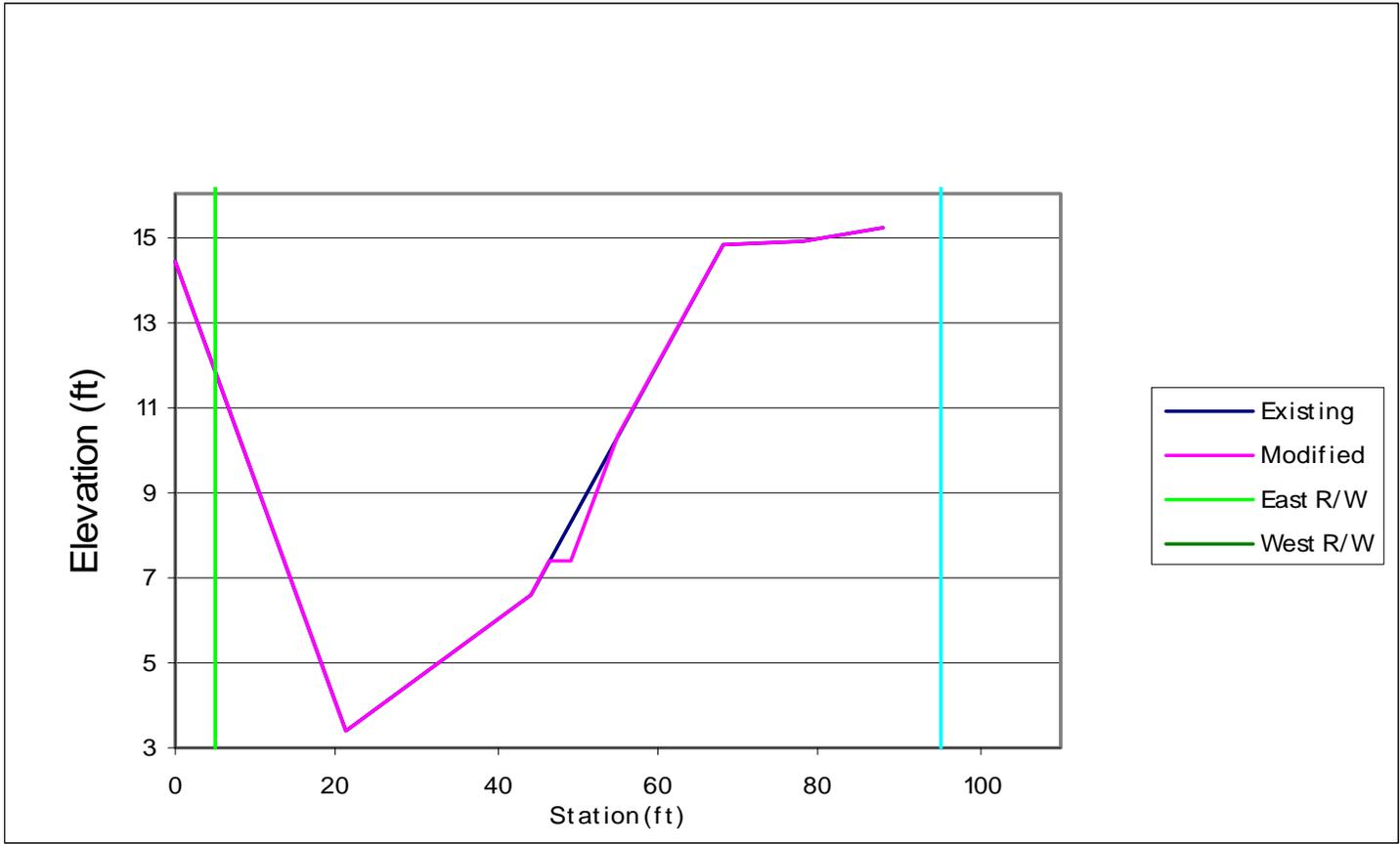
Figure B-8. Corkscrew Canal cross section just downstream of 37th avenue.
