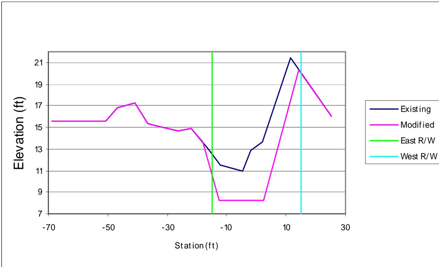
Figure B-1. Corkscrew Canal cross section upstream of 47<sup>th</sup> avenue.
