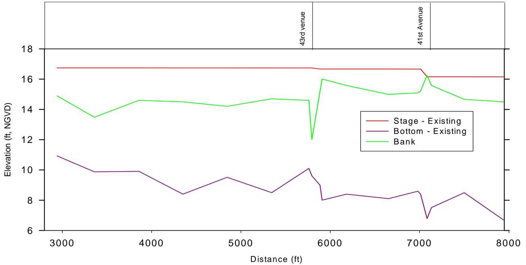
Figure 17a. Corkscrew Canal simulated water surface profile for existing condition.
