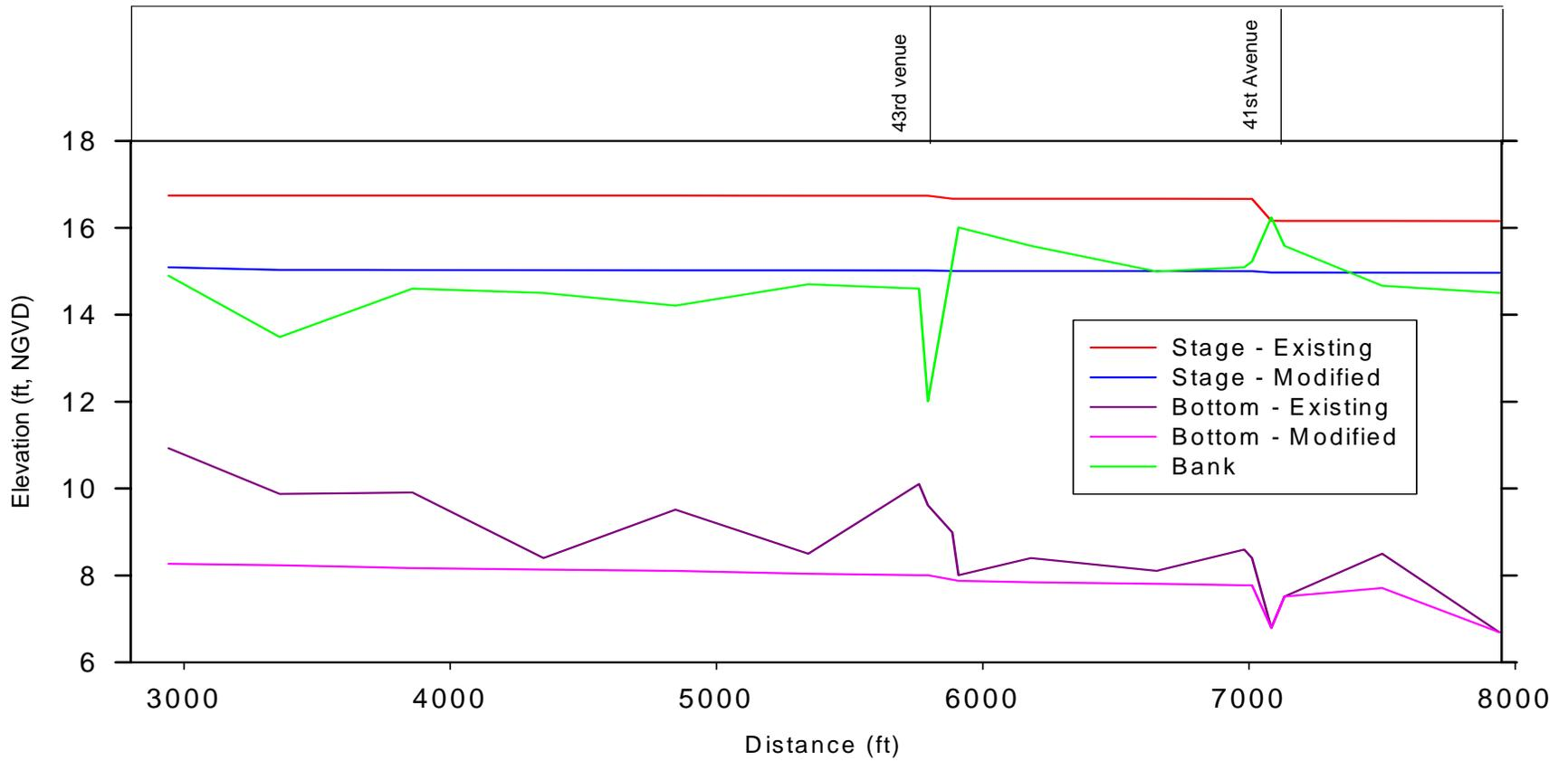
Figure 21a. Corkscrew Canal simulated water surface profiles.
