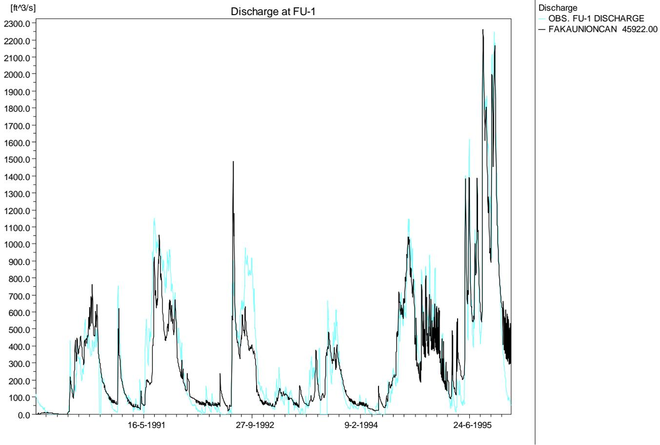
Figure A-5. Simulated and observed river flows in Faka Union Canal at weir FU-1 (chainage 45992) in cfs from 1990-95.
