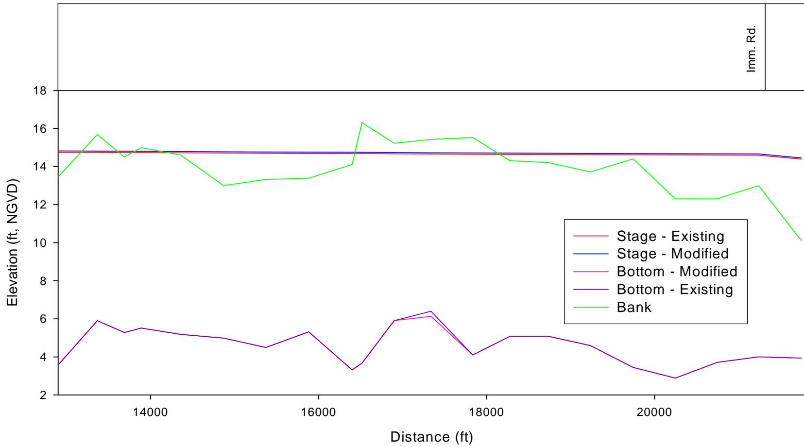
Figure 21c. Corkscrew Canal simulated water surface profiles.
