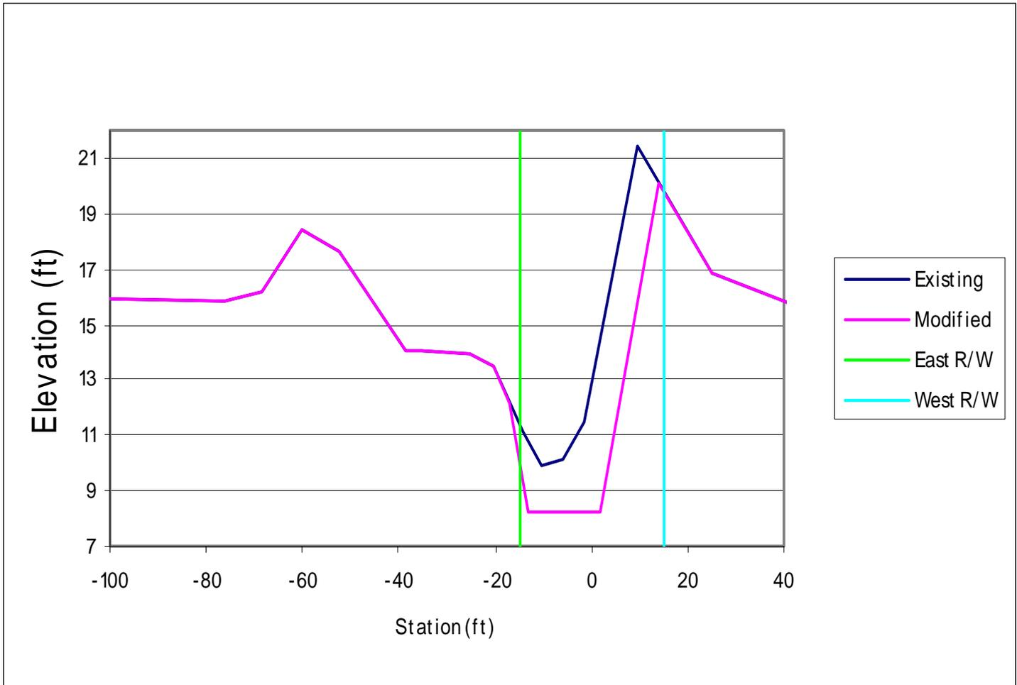
Figure B-2. Corkscrew Canal cross section between 47<sup>th</sup> and 45<sup>th</sup> avenues.
