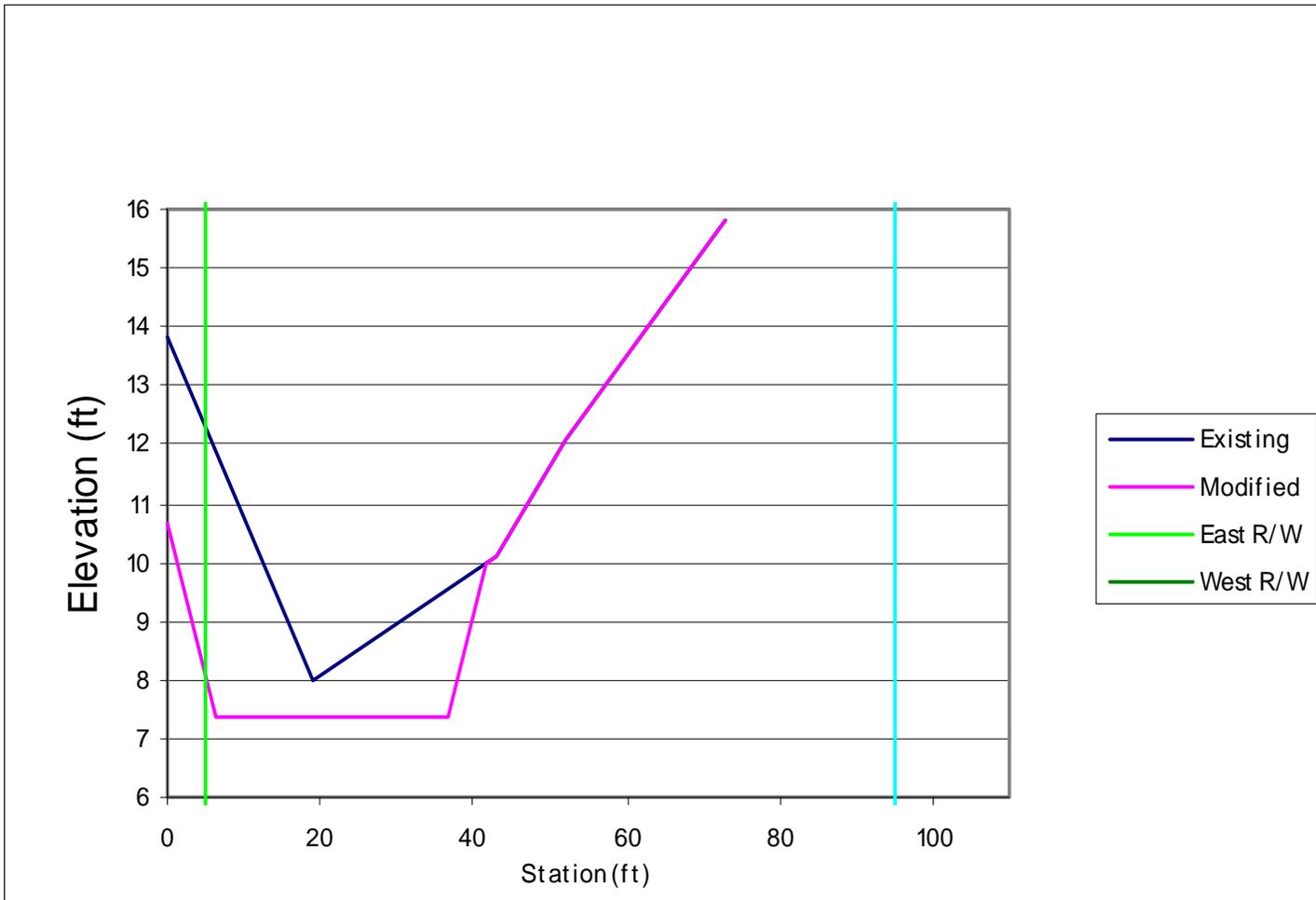
Figure B-7. Corkscrew Canal cross section just upstream of 37th avenue.
