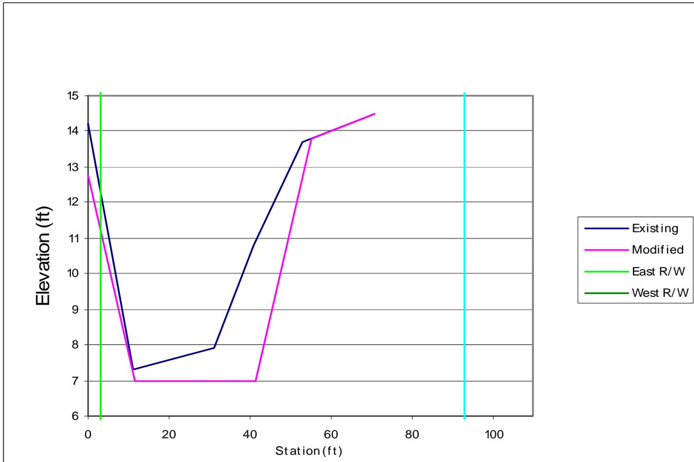
Figure B-11. Corkscrew Canal cross section just upstream of 33rd avenue.
