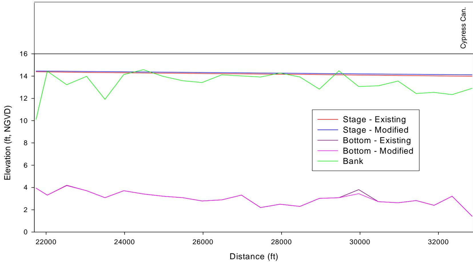
Figure 21d. Corkscrew Canal simulated water surface profiles.
