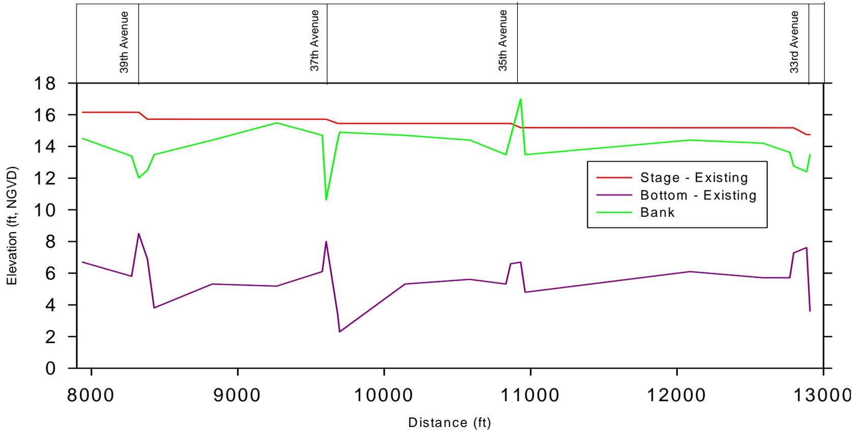
Figure 17b. Corkscrew Canal simulated water surface profile for existing condition.
