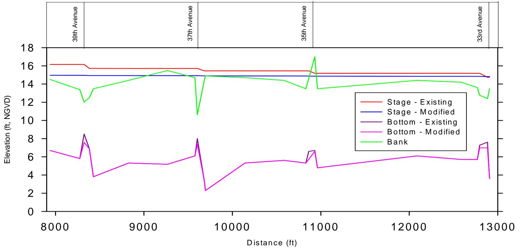
Figure 21b. Corkscrew Canal simulated water surface profiles.
