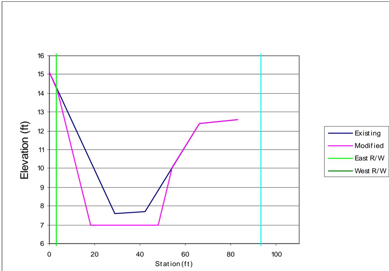
Figure 18c. A typical Corkscrew Canal section just downstream of 33<sup>rd</sup> Avenue.
