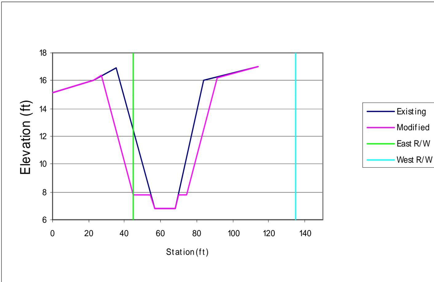
Figure B-4. Corkscrew Canal cross section just downstream of 41<sup>st</sup> avenue.
