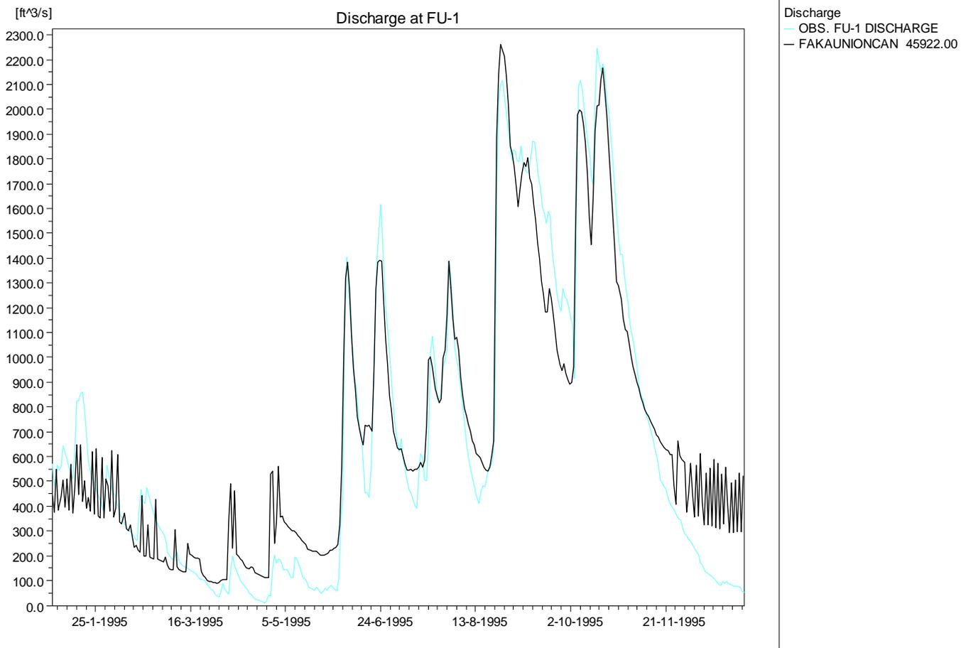
Figure A-6. Simulated and observed river flows in Faka Union Canal at weir FU-1 (chainage 45992) in 1995.
