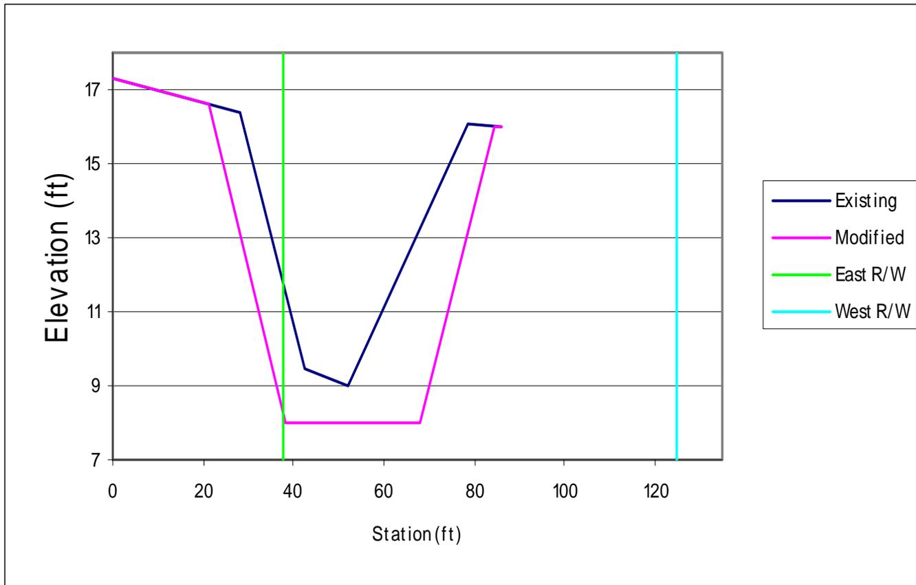
Figure 18b. A typical Corkscrew Canal section just downstream of 43<sup>rd</sup> Avenue.
