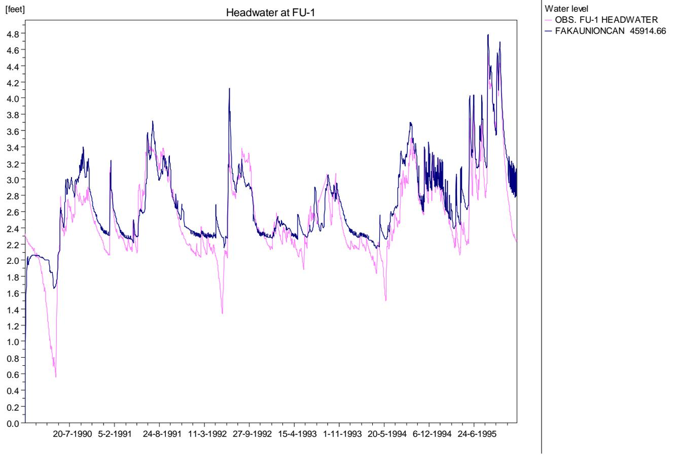
Figure A-4. Simulated and observed headwater in Faka Union Canal at weir FU-1 (chainage 45992) in cfs from 1990-95.
