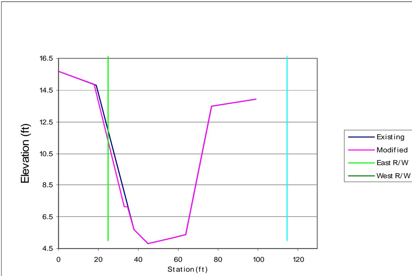
Figure B-10. Corkscrew Canal cross section just downstream of 35th avenue.
