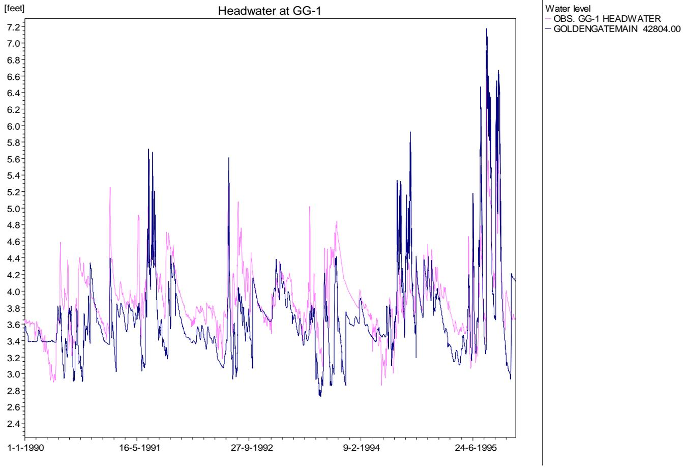
Figure A-3. Simulated and observed headwater in Golden Gate Main Canal at weir GG-1 (chainage 42804) in cfs from 1990-95.
