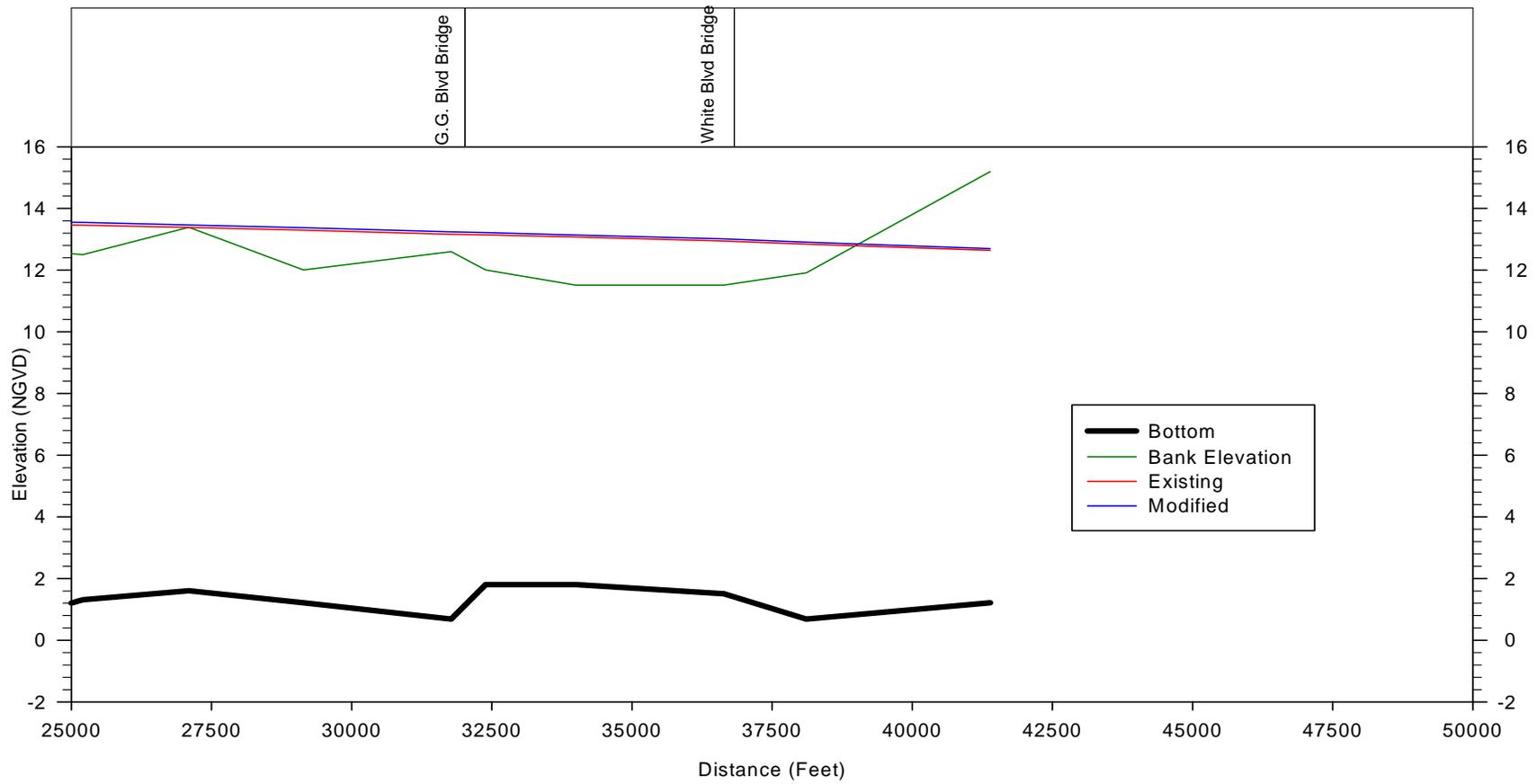
Figure 23b. Cypress Canal simulated water surface profiles
