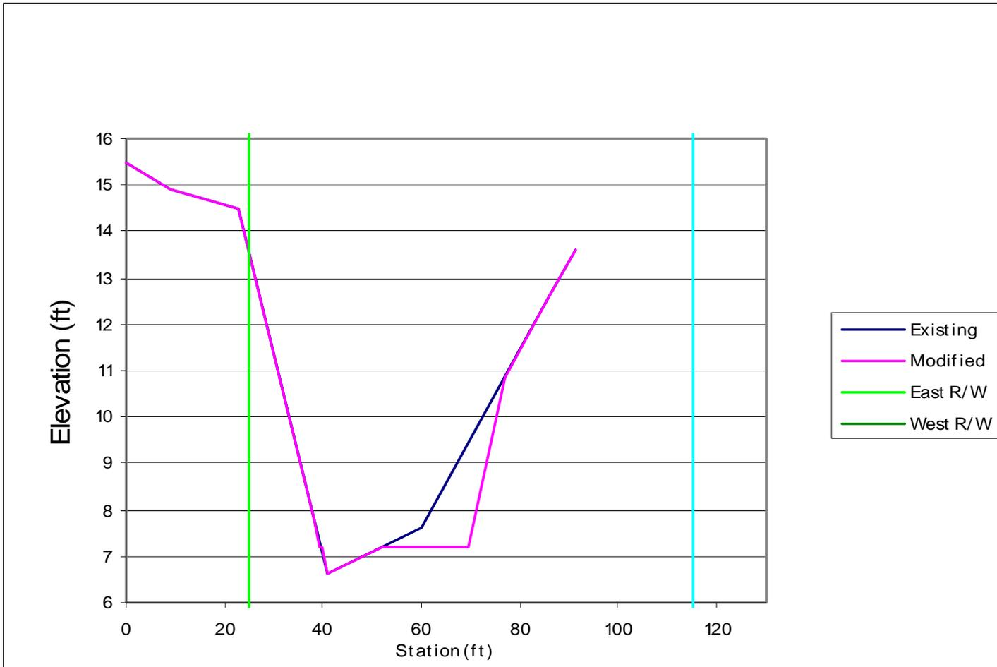
Figure B-9. Corkscrew Canal cross section just upstream of 35th avenue.
