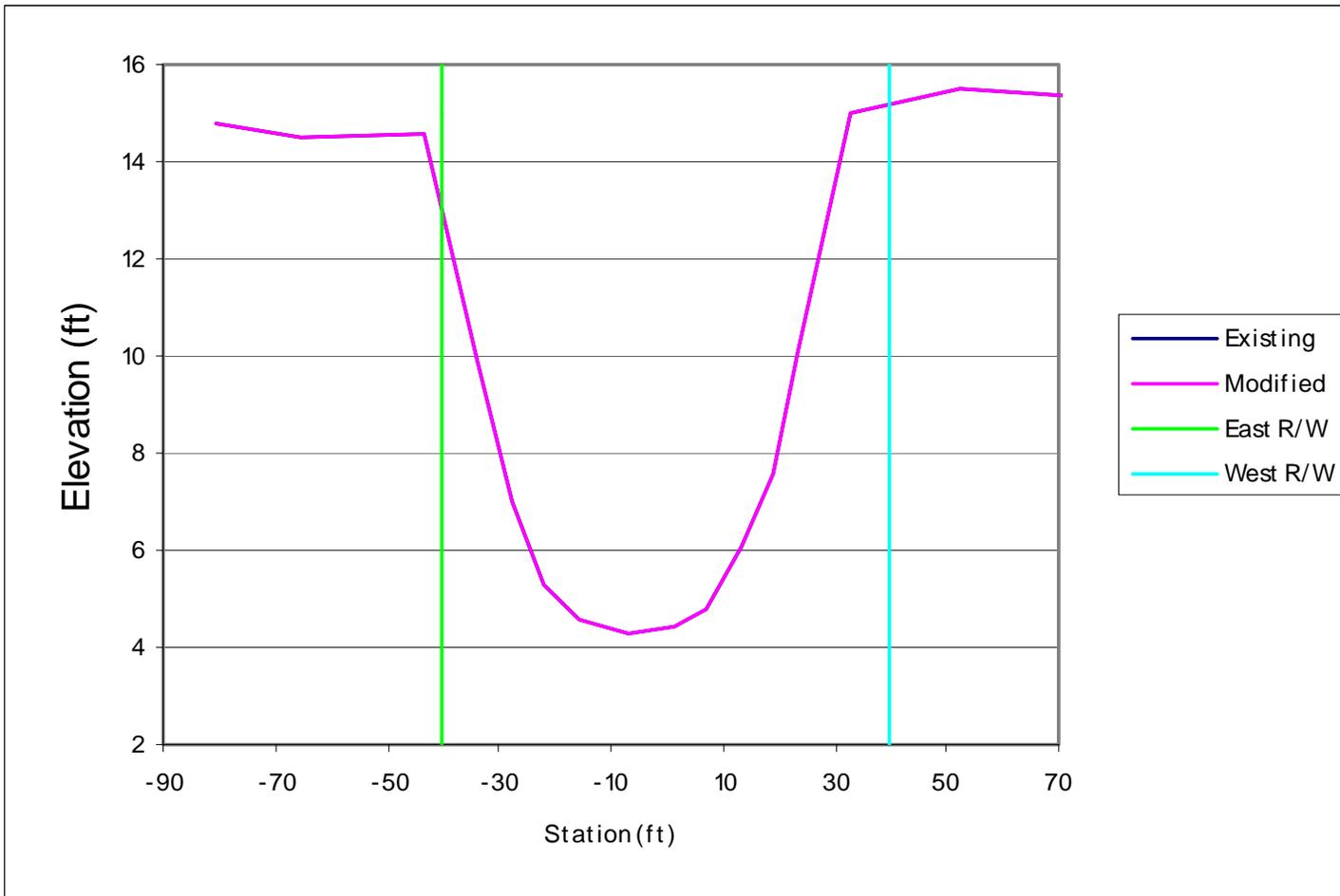
Figure B-12. Corkscrew Canal cross section just upstream of Immokalee Road.
