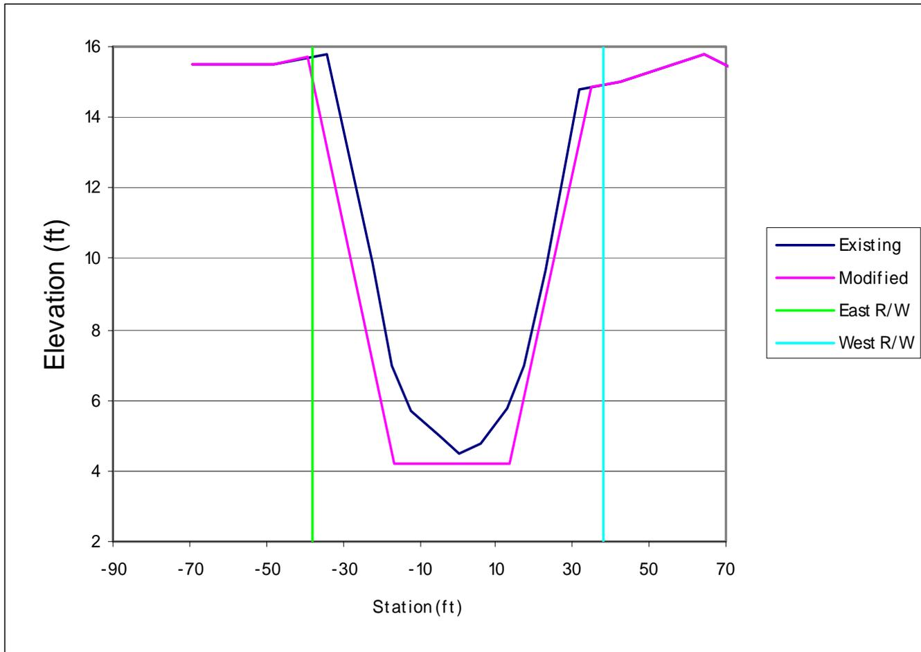
Figure 18d. A typical Corkscrew Canal section just downstream of 33<sup>rd</sup> Avenue.
