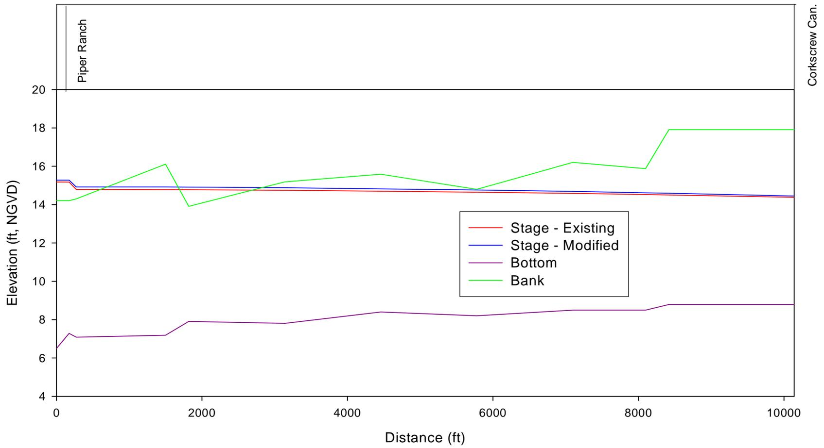
Figure 22. Cocohatchee (East) Canal simulated water surface profiles.
