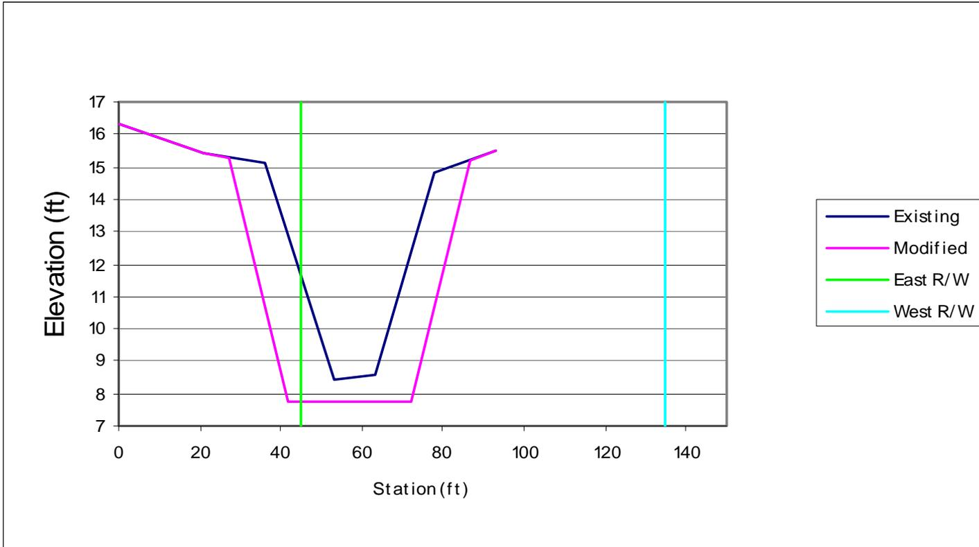
Figure B-3. Corkscrew Canal cross section just upstream of 41<sup>st</sup> avenue.
