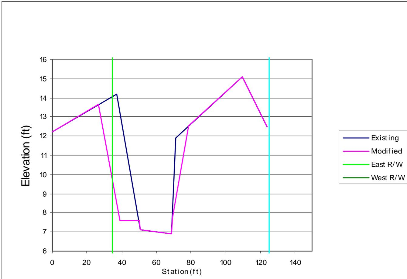
Figure 18f. A typical cross section just upstream of Cypress Canal.
