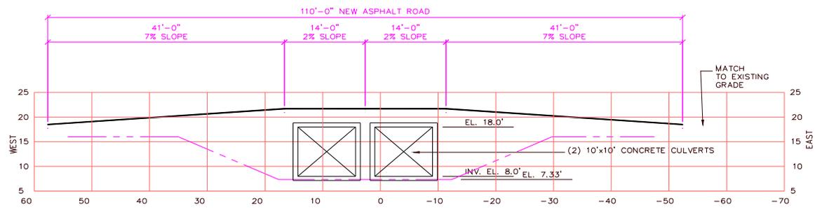
Figure C-1. Gated box culvert at 43<sup>rd</sup> Avenue.
