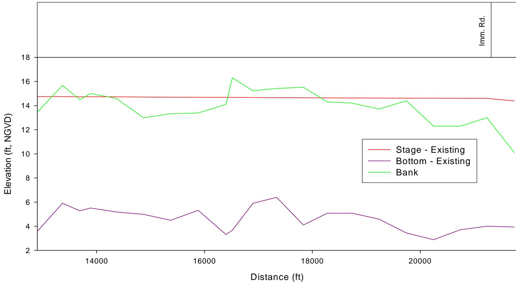
Figure 17c. Corkscrew Canal simulated water surface profile for existing condition.
