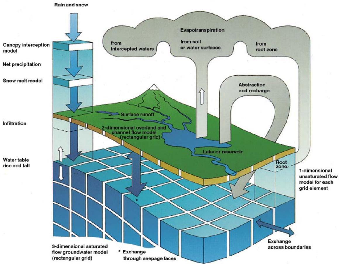
Figure 3. A general configuration of an interactive groundwater-surface water model.
