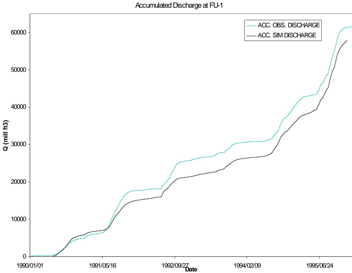
Figure A-7. Accumulated simulated and observed flow in Faka Union Canal at FU-1 in mill. cubic feet from 1990-95.
