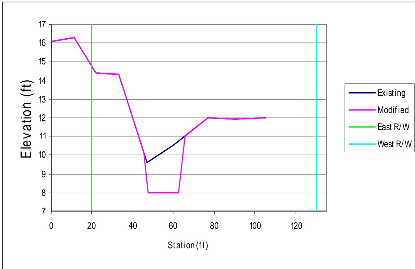
Figure 18a. A typical Corkscrew Canal section upstream of 43<sup>rd</sup> Avenue.
