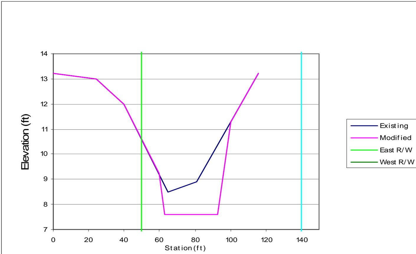
Figure B-5. Corkscrew Canal cross section just upstream of 39th avenue.
