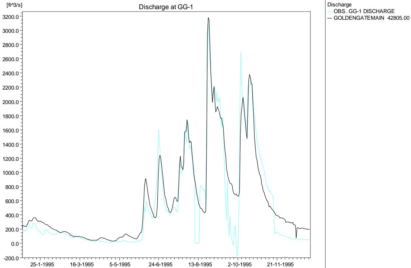
Figure A-1. Simulated and observed stream flows in Golden Gate Canal at weir GG-1 (chainage 42805) in 1995.
