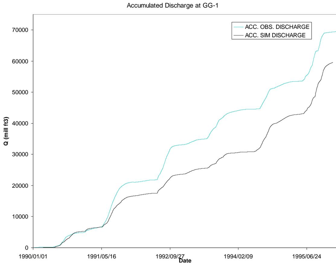
Figure A-2. Accumulated simulated and observed flow in Golden Gate Main Canal at GG-1 in mill. cubic feet from 1990-95.
