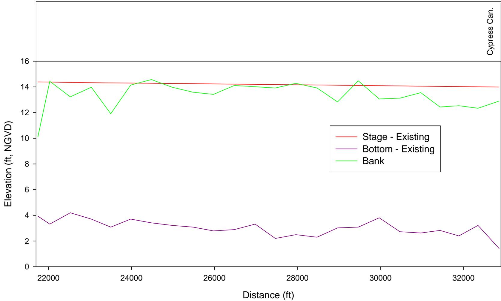
Figure 17d. Corkscrew Canal simulated water surface profile for existing condition.
