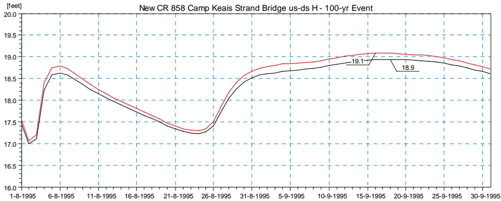
**Figure 4.21 Simulated Stage Results for Scenario 1 Upstream (red) and Downstream (black) of the Proposed Bridge on CR-858 at Camp Keais Strand (Location 1) for the 100-year Design Event.**
