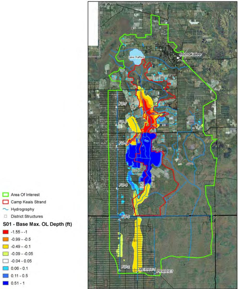
**Figure 4.36 Simulated Differences Between Existing Conditions (Scenario 0) and Scenario 1 Maximum Overland Water Depths During the 100-year Design Event.**
