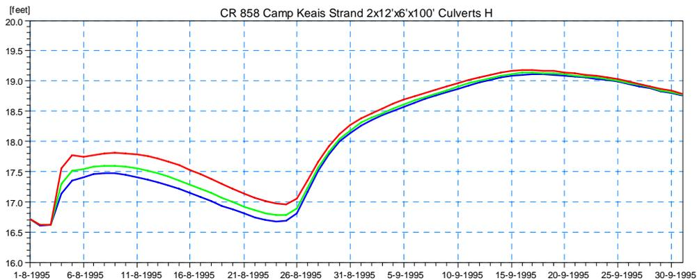
**Figure 4.57 Simulated Stage Results for Scenario 3 Upstream of the Proposed Culvert on CR-858 at Camp Keais Strand (Location 2) for the 5-year (blue), 25-year (green), and 100-year (red) Design Event.**
