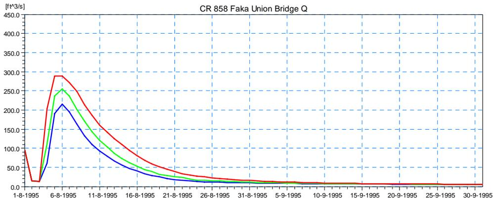
**Figure 4.29 Simulated Discharge Results for Scenario 1 at the Proposed Modified Bridge on CR-858 at Faka Union Canal (Location 3) for the 5-year (blue), 25-year (green), and 100-year (red) Design Event.**
