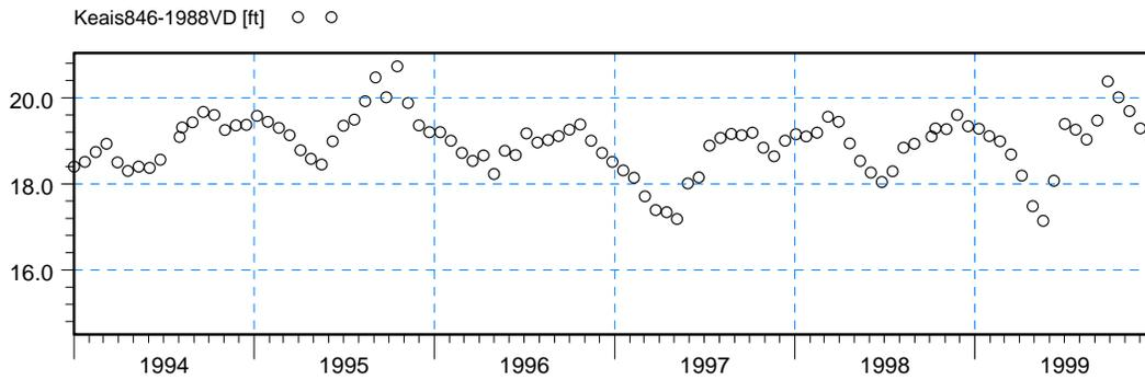
**Figure 2.6 Observed Stages at the Tailwater Side (South) of the Bridge on Camp Keais Strand at CR 846 (ft NAVD 1988).**
