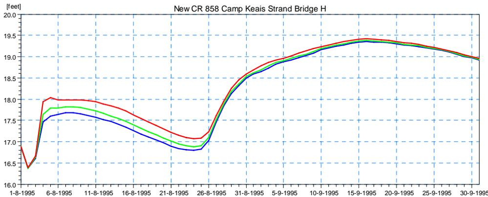
**Figure 4.54 Simulated Stage Results for Scenario 3 Upstream of the Proposed Bridge on CR-858 at Camp Keais Strand (Location 1) for the 5-year (blue), 25-year (green), and 100-year (red) Design Event.**
