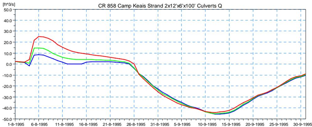
**Figure 4.42 Simulated Discharge Results for Scenario 2 at the Proposed Culvert on CR-858 at Camp Keais Strand (Location 2) for the 5-year (blue), 25-year (green), and 100-year (red) Design Event.**
