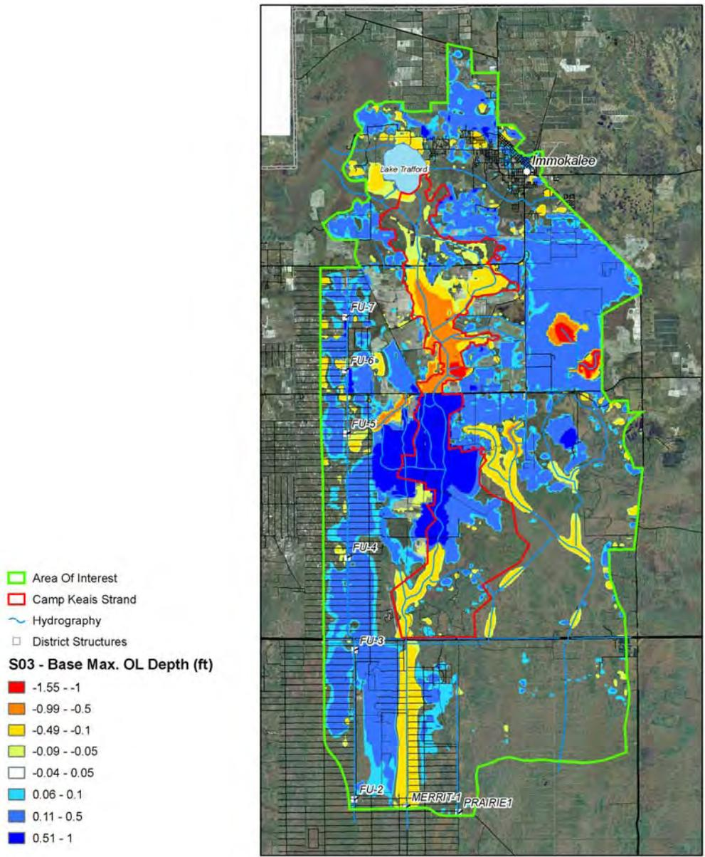
**Figure 4.68 Simulated Differences between Existing Conditions (Scenario 0) and Scenario 3 Maximum Overland Water Depths During the 100-year Design Event.**
