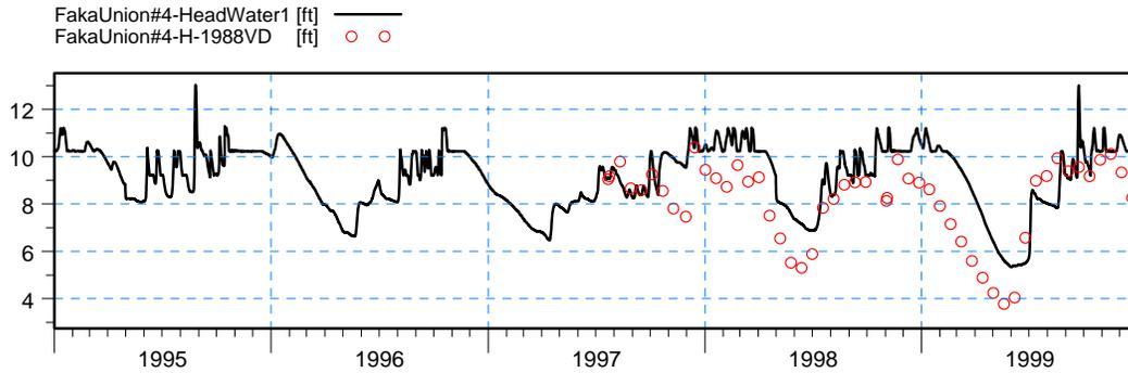
**Figure 3.10 Simulated and Observed Results at the Faka Union Canal Number 4 Headwater Gage.**
