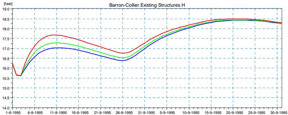
**Figure 4.34 Simulated Stage Results for Scenario 1 Upstream of the Existing Barron-Collier Structure in Camp Keais Strand (Location 5) for the 5-year (blue), 25-year (green), and 100-year (red) Design Event.**
