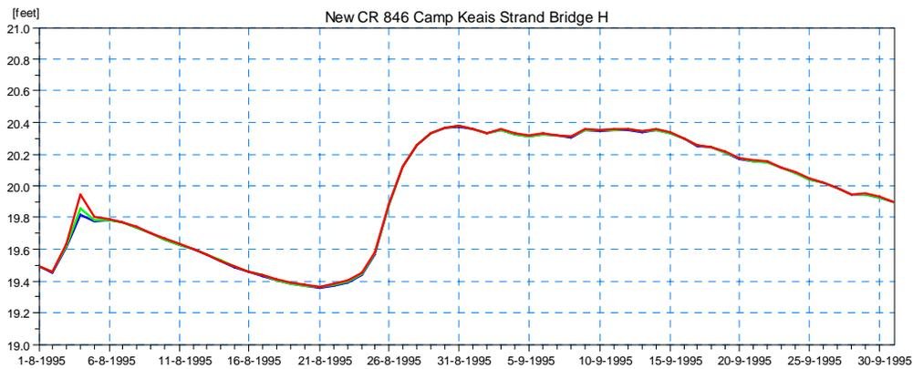
**Figure 4.63 Simulated Stage Results for Scenario 3 Upstream of the Proposed Modified Bridge on CR-846 at Camp Keais Strand (Location 4) for the 5-year (blue), 25-year (green), and 100-year (red) Design Event.**
