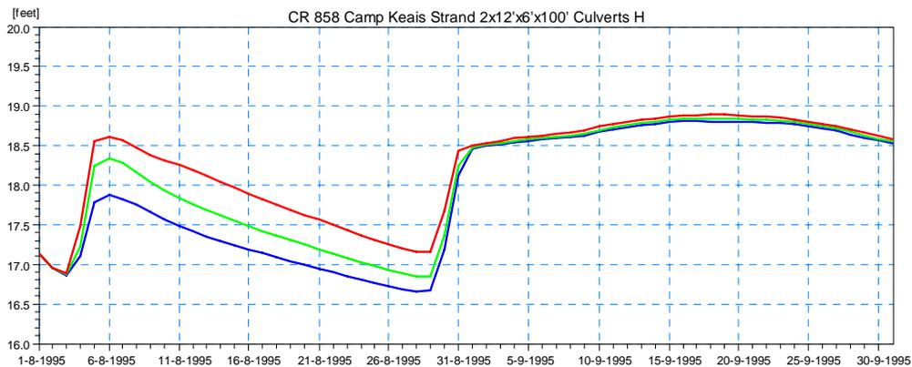
**Figure 4.25 Simulated Stage Results for Scenario 1 Upstream of the Proposed Culvert on CR-858 at Camp Keais Strand (Location 2) for the 5-year (blue), 25-year (green), and 100-year (red) Design Event.**
