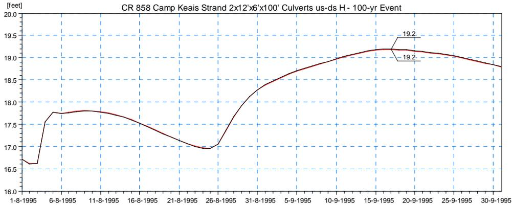
**Figure 4.56 Simulated Stage Results for Scenario 3 Upstream (red) and Downstream (black) of the Proposed Culvert on CR-858 at Camp Keais Strand (Location 2) for the 100-year Design Event.**
