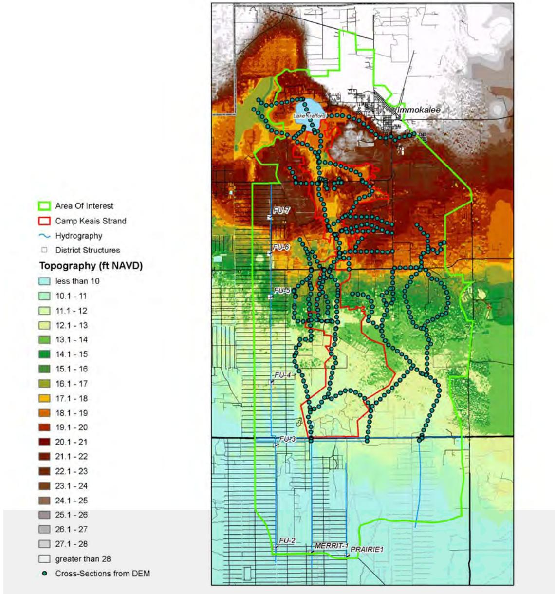
**Figure 2.20** Digital elevation model for the Camp Keais Strand Area developed from the best available topographic area for the data (ft NAVD). The locations for cross-sections extracted from the digital elevation model are also shown. The digital elevation model has a maximum horizontal resolution of 100 ft.
