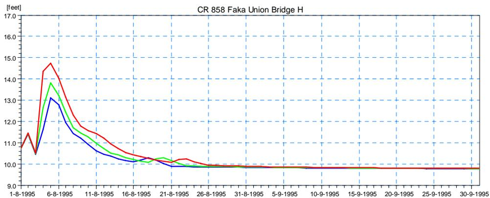
**Figure 4.60 Simulated Stage Results for Scenario 3 Upstream of the Proposed Modified Bridge on CR-858 at Faka Union Canal (Location 3) for the 5-year (blue), 25-year (green), and 100-year (red) Design Event.**
