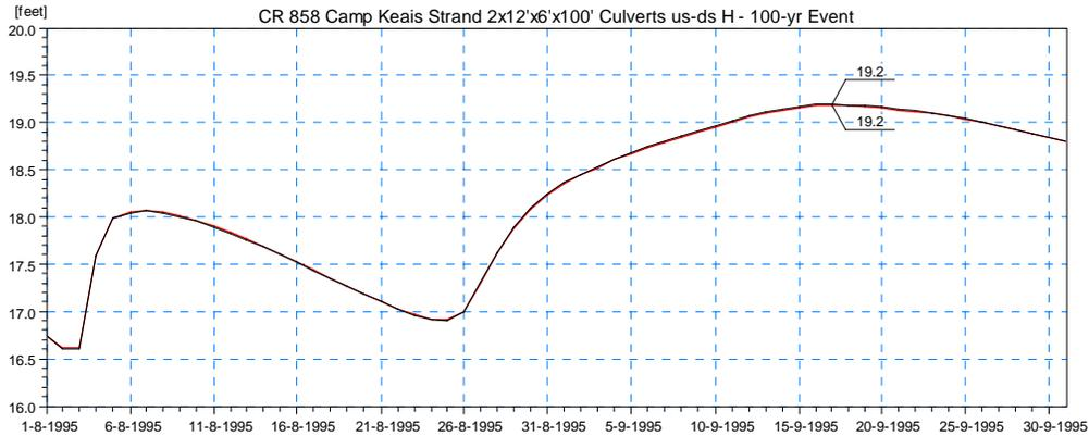
**Figure 4.40 Simulated Stage Results for Scenario 2 Upstream (red) and Downstream (Black) of the Proposed Culvert on CR-858 at Camp Keais Strand (Location 2) for the 100-year Design Event.**
