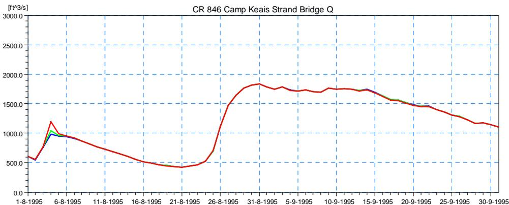
**Figure 4.32 Simulated Discharge Results for Scenario 1 at the Existing Bridge on CR-846 at Camp Keais Strand (Location 4) for the 5-year (blue), 25-year (green), and 100-year (red) Design Event.**
