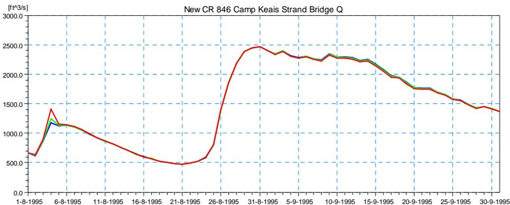
**Figure 4.64 Simulated Discharge Results for Scenario 3 at the Proposed Modified Bridge on CR-846 at Camp Keais Strand (Location 4) for the 5-year (blue), 25-year (green), and 100-year (red) Design Event.**
