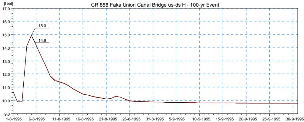
**Figure 4.43 Simulated Stage Results for Scenario 2 Upstream (red) and Downstream (black) of the Proposed Modified Bridge on CR-858 at Faka Union Canal (Location 3) for the 100-year Design Event.**
