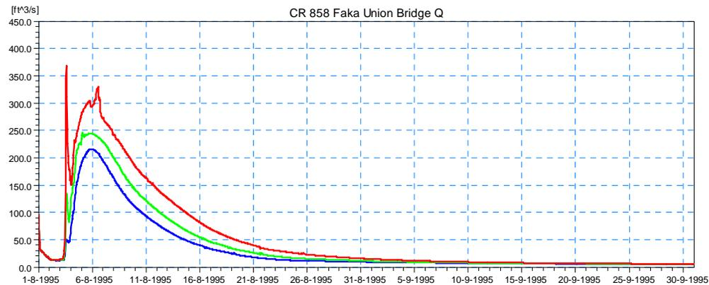
**Figure 4.14 Simulated discharge results for existing conditions (Scenario 0) at the existing bridge on CR-858 at Faka Union Canal (location 3) for the 5-year (blue), 25-year (green), and 100-year (red) design event.**
