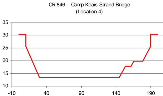
**Figure 4.4** Geometry of the New Bridge on CR-846 at Camp Keais Strand (Location 4).
