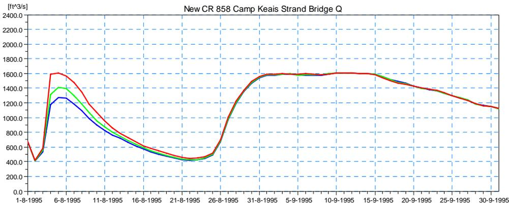
**Figure 4.23 Simulated Discharge Results for Scenario 1 at the Proposed Bridge on CR-858 at Camp Keais Strand (Location 1) for the 5-year (blue), 25-year (green), and 100-year (red) Design Event.**
