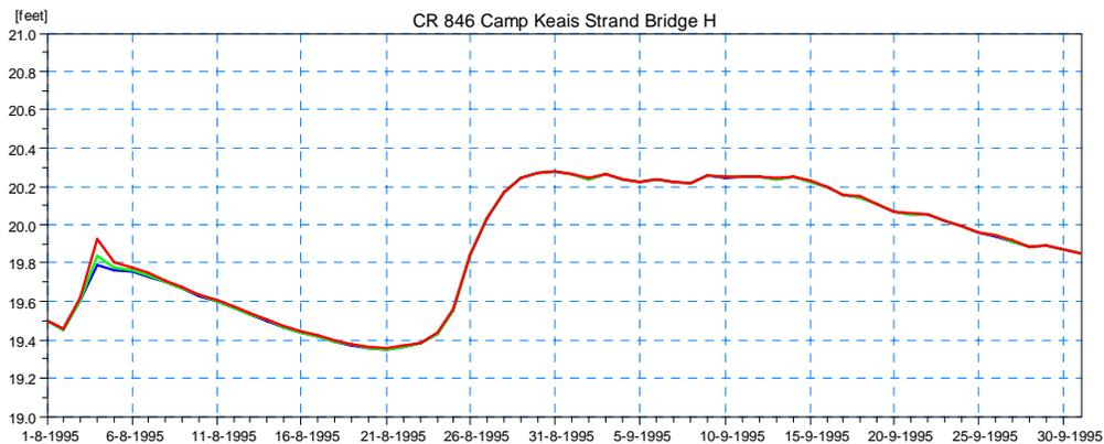
**Figure 4.31 Simulated Stage Results for Scenario 1 Upstream of the Existing Bridge on CR-846 at Camp Keais Strand (Location 4) for the 5-year (blue), 25-year (green), and 100-year (red) Design Event.**
