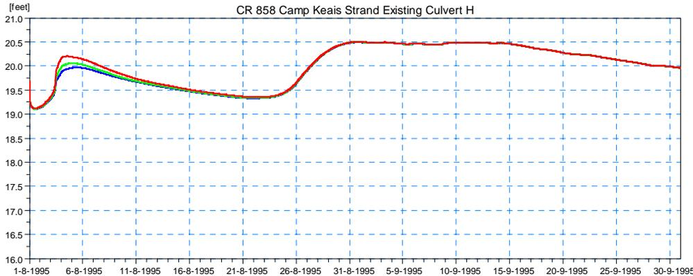
**Figure 4.7 Simulated Stage Results for Existing Conditions (Scenario 0) Upstream of the Existing Culvert on CR-858 at Camp Keais Strand (Location 1) for the 5-year (blue), 25-year (green), and 100-year (red) Design Event.**
