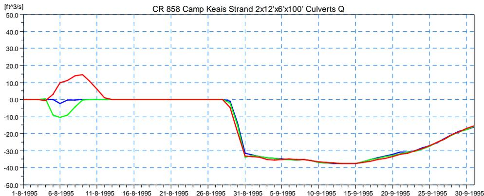
**Figure 4.26 Simulated Discharge Results for Scenario 1 at the Proposed Culvert on CR-858 at Camp Keais Strand (Location 2) for the 5-year (blue), 25-year (green), and 100-year (red) Design Event.**
