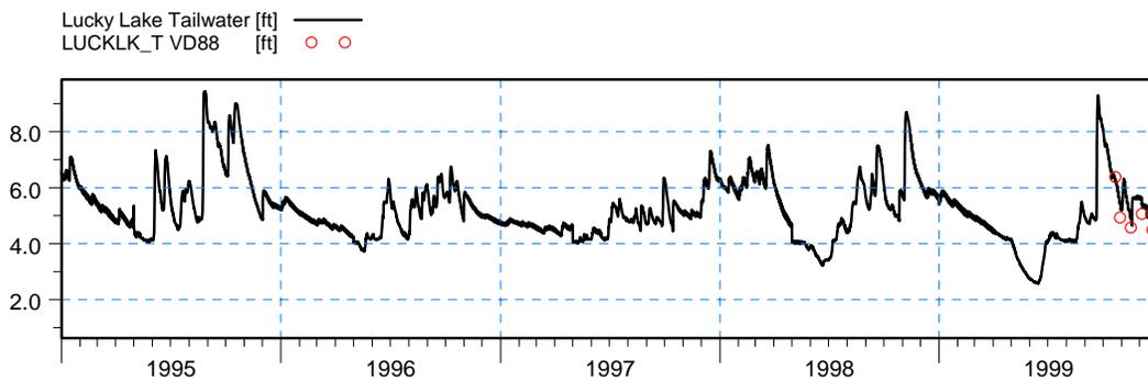
**Figure 3.15 Simulated and Observed Results at the Luck Lake Weir Tailwater Gage.**
