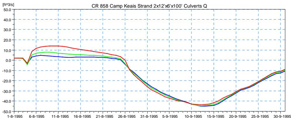
**Figure 4.58 Simulated Discharge Results for Scenario 3 at the Proposed Culvert on CR-858 at Camp Keais Strand (Location 2) for the 5-year (blue), 25-year (green), and 100-year (red) Design Event.**
