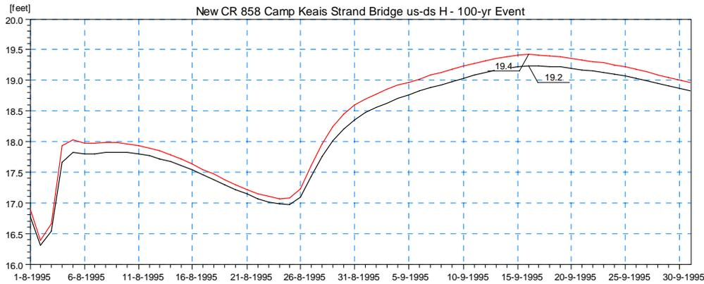
**Figure 4.53 Simulated Stage Results for Scenario 3 Upstream (red) and Downstream (black) of the Proposed Bridge on CR-858 at Camp Keais Strand (Location 1) for the 100-year Design Event.**
