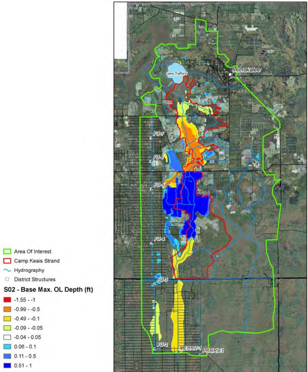
**Figure 4.52 Simulated Differences Between Existing Conditions (Scenario 0) and Scenario 2 Maximum Overland Water Depths During the 100-year Design Event.**
