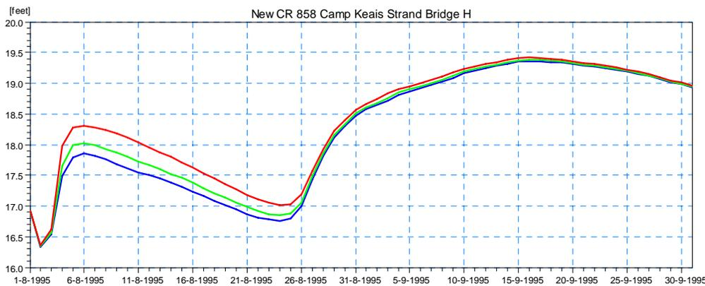
**Figure 4.38 Simulated Stage Results for Scenario 2 Upstream of the Proposed Bridge on CR-858 at Camp Keais Strand (Location 1) for the 5-year (blue), 25-year (green), and 100-year (red) Design Event.**
