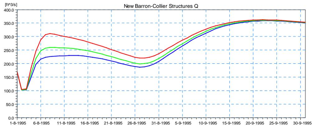
**Figure 4.51 Simulated Discharge Results for Scenario 2 at the Proposed Modified Barron-Collier Structure in Camp Keais Strand (Location 6) for the 5-year (blue), 25-year (green), and 100-year (red) Design Event.**
