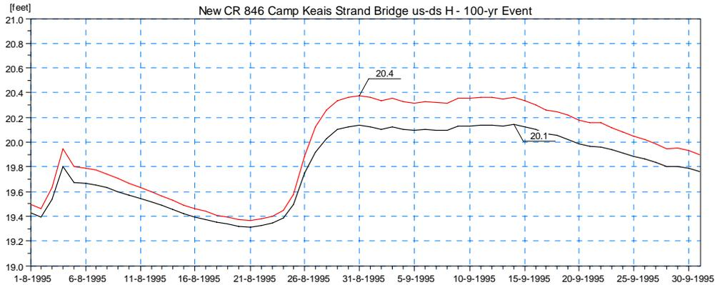
**Figure 4.62 Simulated Stage Results for Scenario 3 Upstream (red) and Downstream (black) of the Proposed Modified Bridge on CR-846 at Camp Keais Strand (Location 4) for the 100-year Design Event.**
