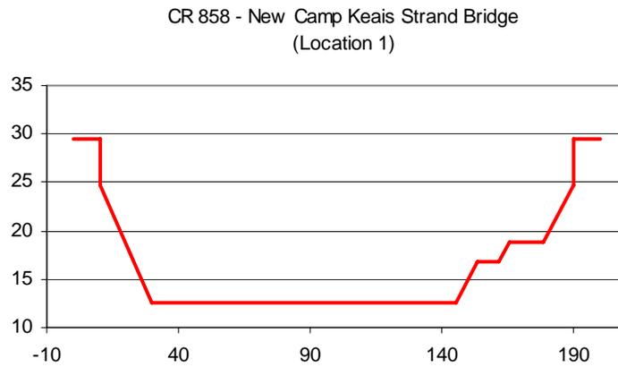
**Figure 4.2** Geometry of the New Bridge on CR-858 at Camp Keais Strand (Location 1).
