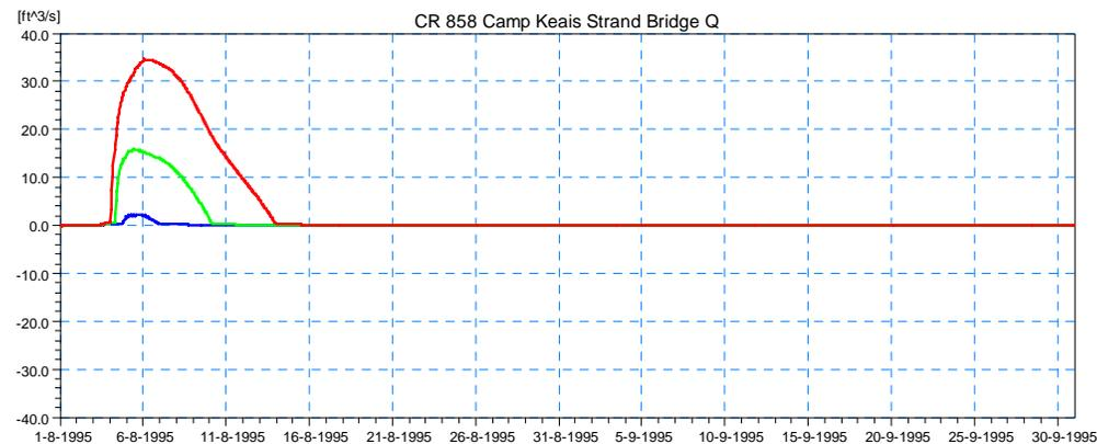
**Figure 4.11 Simulated Discharge Results for Existing Conditions (Scenario 0) at the Existing Bridge on CR-858 at Camp Keais Strand (Location 2) for the 5-year (blue), 25-year (green), and 100-year (red) Design Event.**
