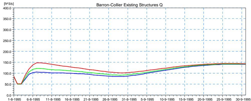
**Figure 4.35 Simulated Discharge Results for Scenario 1 at the Existing Barron-Collier Structure in Camp Keais Strand (Location 6) for the 5-year (blue), 25-year (green), and 100-year (red) Design Event.**
