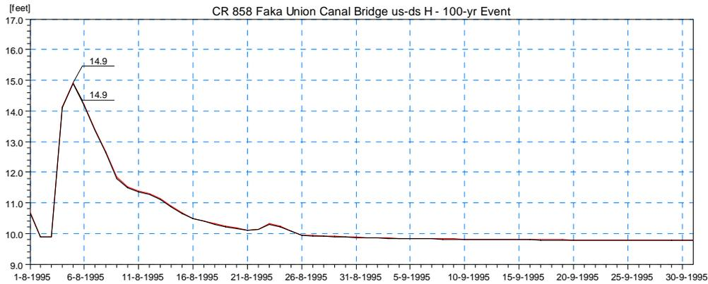
**Figure 4.27 Simulated Stage Results for Scenario 1 Upstream (red) and Downstream (black) of the Proposed Modified Bridge on CR-858 at Faka Union Canal (Location 3) for the 100-year Design Event.**
