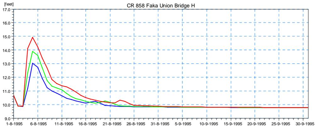
**Figure 4.28 Simulated Stage Results for Scenario 1 Upstream of the Proposed Modified Bridge on CR-858 at Faka Union Canal (Location 3) for the 5-year (blue), 25-year (green), and 100-year (red) Design Event.**
