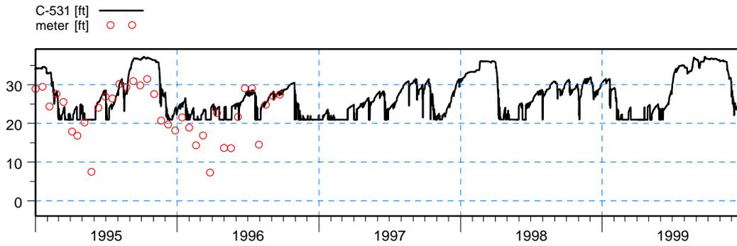
**Figure 3.17 Simulated and Observed Results at the Groundwater Observation Well C-531.**
