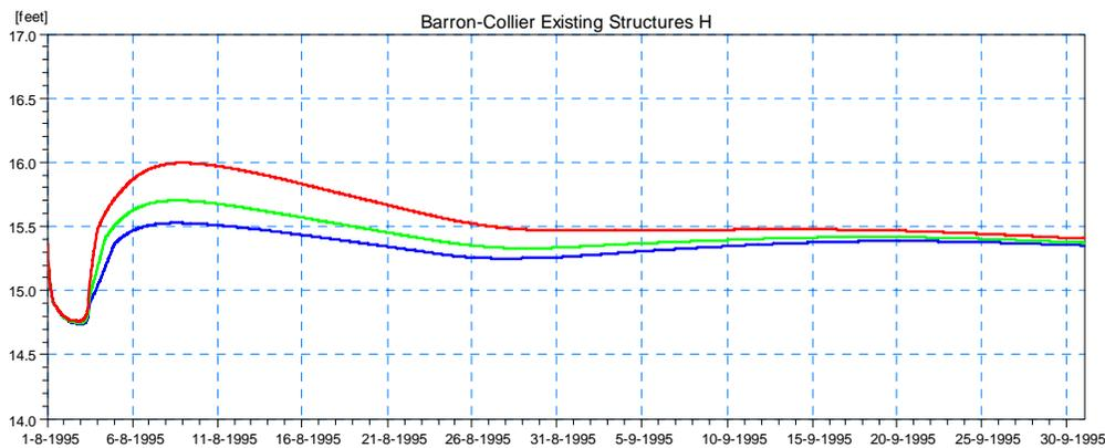
**Figure 4.19 Simulated Stage Results for Existing Conditions (Scenario 0) Upstream of the Existing Barron-Collier Structure in Camp Keais Strand (Location 5) for the 5-year (blue), 25-year (green), and 100-year (red) Design Event.**
