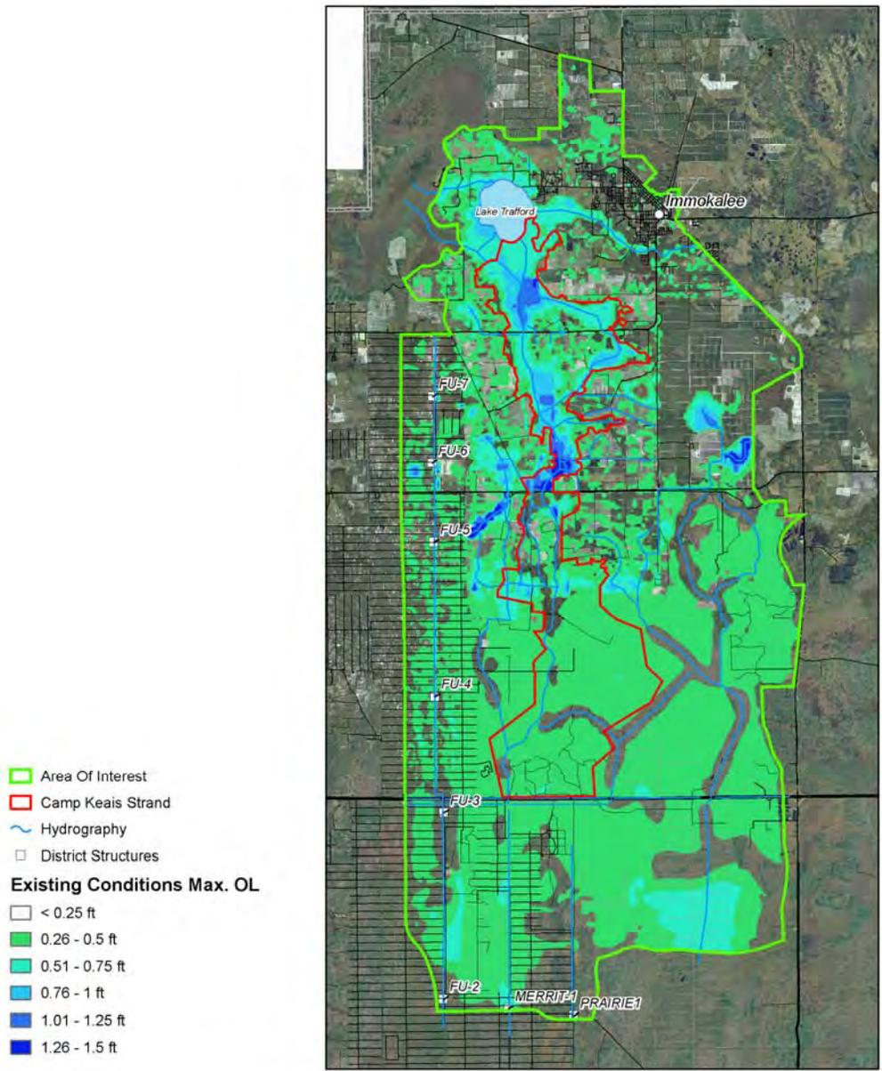
**Figure 3.22 Simulated Maximum Overland Water Depths for the Calibrated Model with the 5-day 100-year Design Event.**
