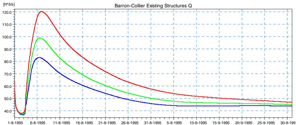
**Figure 4.20 Simulated Discharge results for Existing Conditions (Scenario 0) at the Existing Barron-Collier Structure in Camp Keais Strand (Location 6) for the 5-year (blue), 25-year (green), and 100-year (red) Design Event.**
