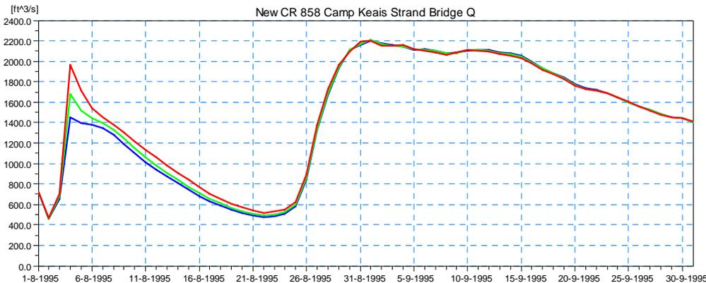
**Figure 4.55 Simulated Discharge Results for Scenario 3 at the Proposed Bridge on CR-858 at Camp Keais Strand (Location 1) for the 5-year (blue), 25-year (green), and 100-year (red) Design Event.**
