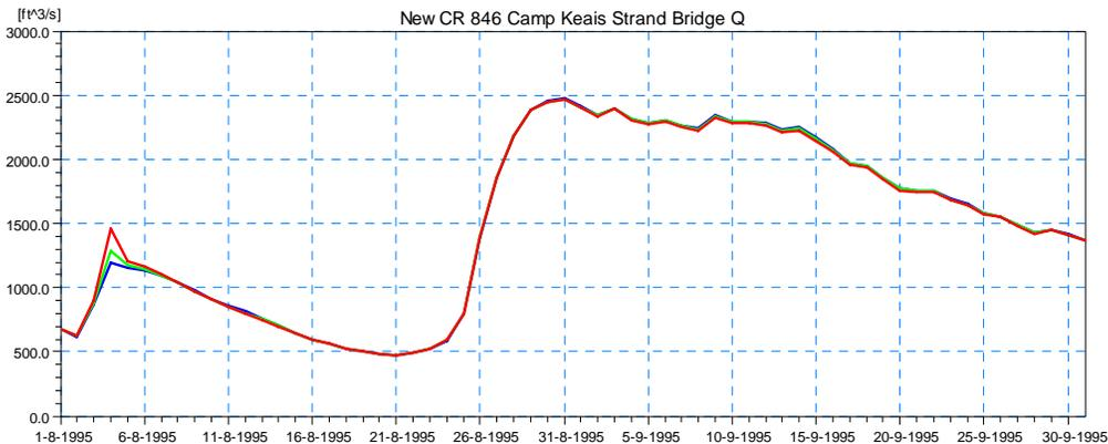
**Figure 4.48 Simulated Discharge Results for Scenario 2 at the Proposed Modified Bridge on CR-846 at Camp Keais Strand (Location 4) for the 5-year (blue), 25-year (green), and 100-year (red) Design Event.**
