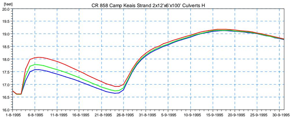
**Figure 4.41 Simulated Stage Results for Scenario 2 Upstream of the Proposed Culvert on CR-858 at Camp Keais Strand (Location 2) for the 5-year (blue), 25-year (green), and 100-year (red) Design Event.**
