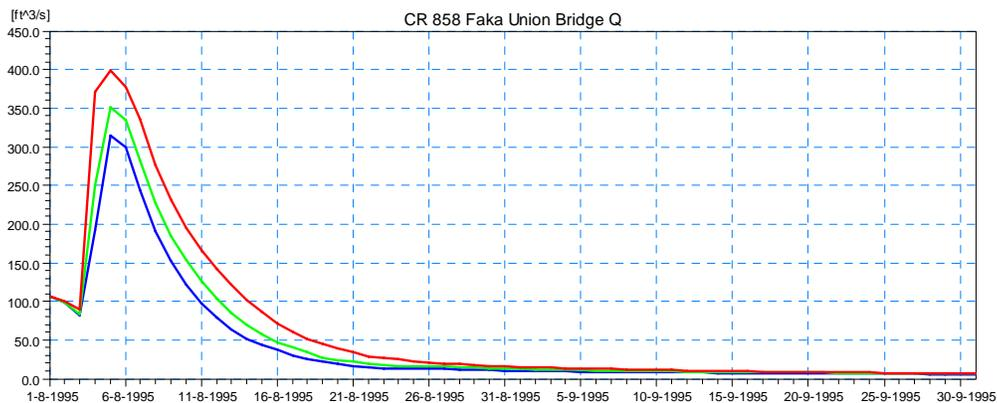
**Figure 4.61 Simulated Discharge Results for Scenario 3 at the Proposed Modified Bridge on CR-858 at Faka Union Canal (Location 3) for the 5-year (blue), 25-year (green), and 100-year (red) Design Event.**
