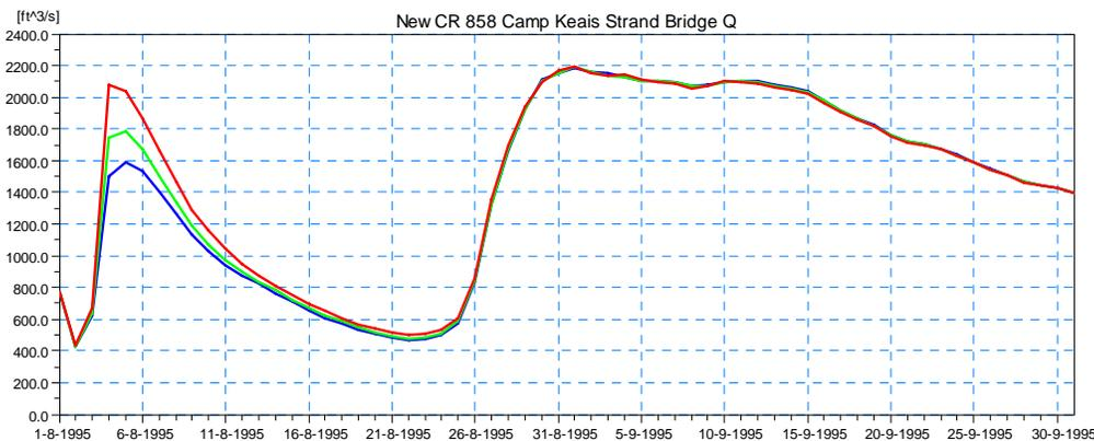
**Figure 4.39 Simulated Discharge Results for Scenario 2 at the Proposed Bridge on CR-858 at Camp Keais Strand (Location 1) for the 5-year (blue), 25-year (green), and 100-year (red) Design Event.**
