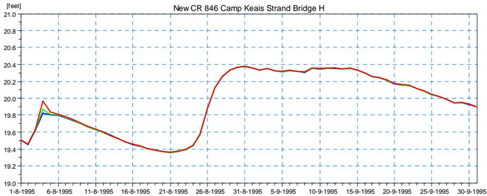
**Figure 4.47 Simulated Stage Results for Scenario 2 Upstream of the Proposed Modified Bridge on CR-846 at Camp Keais Strand (Location 4) for the 5-year (blue), 25-year (green), and 100-year (red) Design Event.**
