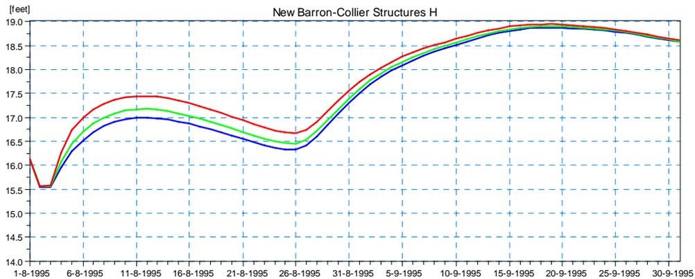
**Figure 4.66 Simulated Stage Results for Scenario 3 Upstream of the Proposed Modified Barron-Collier Structure in Camp Keais Strand (Location 5) for the 5-year (blue), 25-year (green), and 100-year (red) Design Event.**
