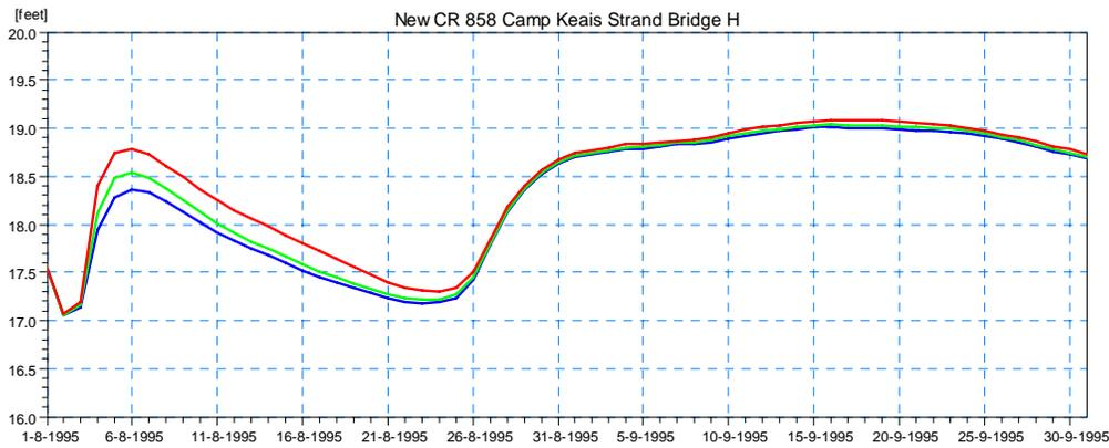
**Figure 4.22 Simulated Stage Results for Scenario 1 Upstream of the Proposed Bridge on CR-858 at Camp Keais Strand (Location 1) for the 5-year (blue), 25-year (green), and 100-year (red) Design Event.**
