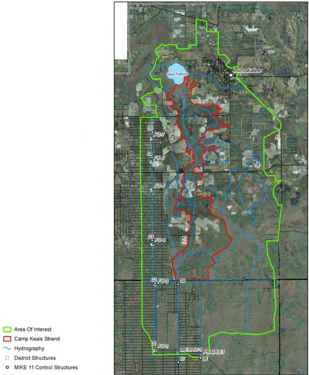
**Figure 3.4 Control Structures Simulated in the Camp Keais Strand MIKE 11 Model.**
