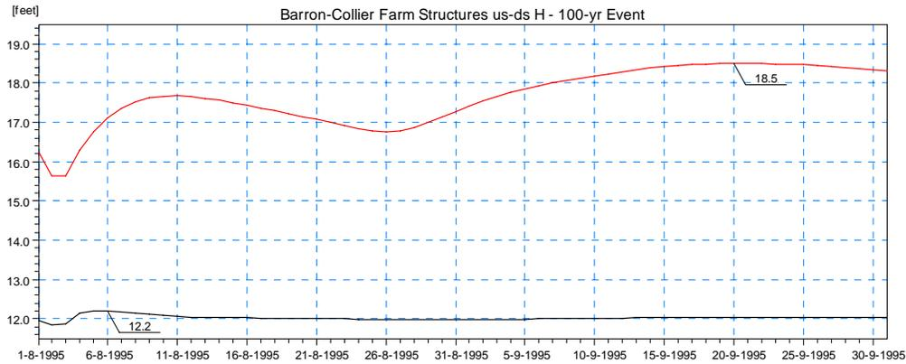
**Figure 4.33 Simulated Stage Results for Scenario 1 Upstream (red) and Downstream (black) of the Existing Barron-Collier Structures in Camp Keais Strand (Locations 5 and 6) for the 100-year Design Event.**
