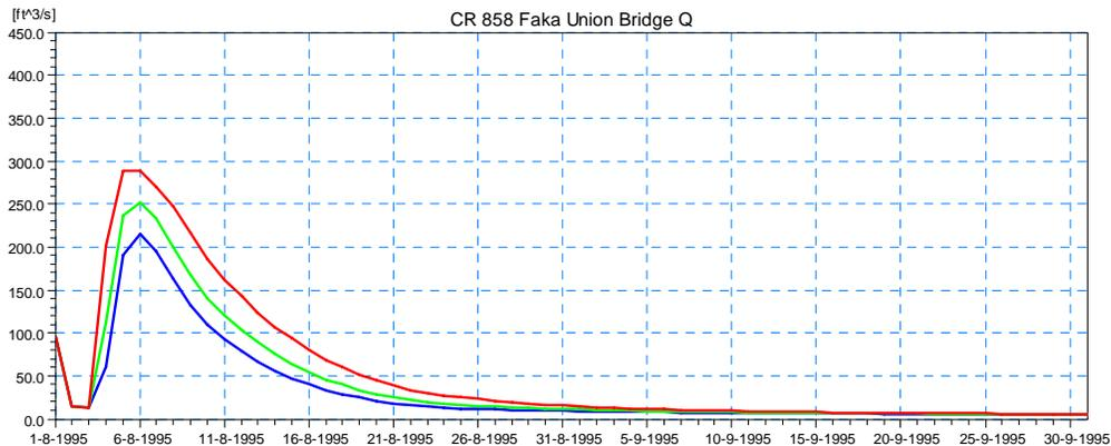
**Figure 4.45 Simulated Discharge Results for Scenario 2 at the Proposed Modified Bridge on CR-858 at Faka Union Canal (Location 3) for the 5-year (blue), 25-year (green), and 100-year (red) Design Event.**
