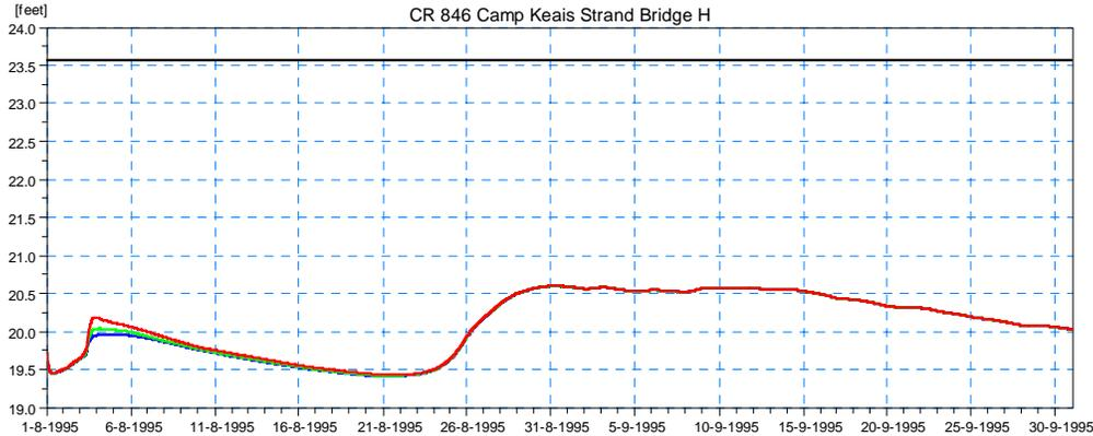
**Figure 4.16** Simulated Stage Results for Existing Conditions (Scenario 0) Upstream of the Existing Bridge on CR-846 at Camp Keais Strand (Location 4) for the 5-year (blue), 25-year (green), and 100-year (red) Design Event.
