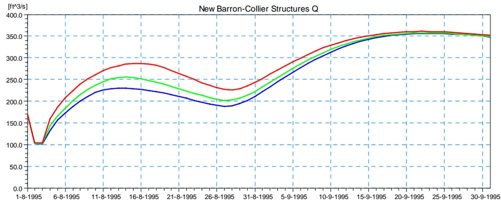
**Figure 4.67 Simulated Discharge Results for Scenario 3 at the Proposed Modified Barron-Collier Structure in Camp Keais Strand (Location 6) for the 5-year (blue), 25-year (green), and 100-year (red) Design Event.**
