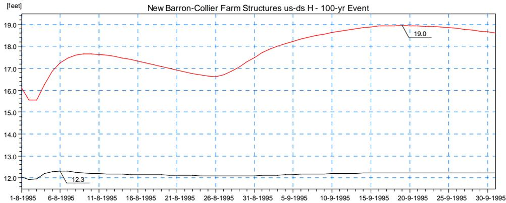
**Figure 4.49 Simulated Stage Results for Scenario 2 Upstream (red) and Downstream (black) of the Proposed Modified Barron-Collier Structures in Camp Keais Strand (Locations 5 and 6) for the 100-year Design Event.**
