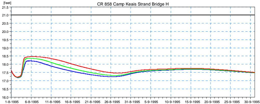
**Figure 4.10 Simulated Stage Results for Existing Conditions (Scenario 0) Upstream of the Existing Bridge on CR-858 at Camp Keais Strand (Location 2) for the 5-year (blue), 25-year (green), and 100-year (red) Design Event.**
