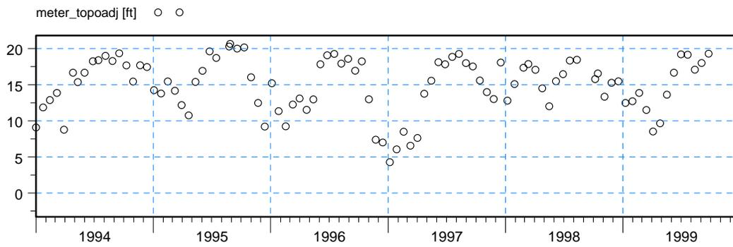
**Figure 2.17** Observed Groundwater Levels at C-1079 (ft NAVD 1988).
