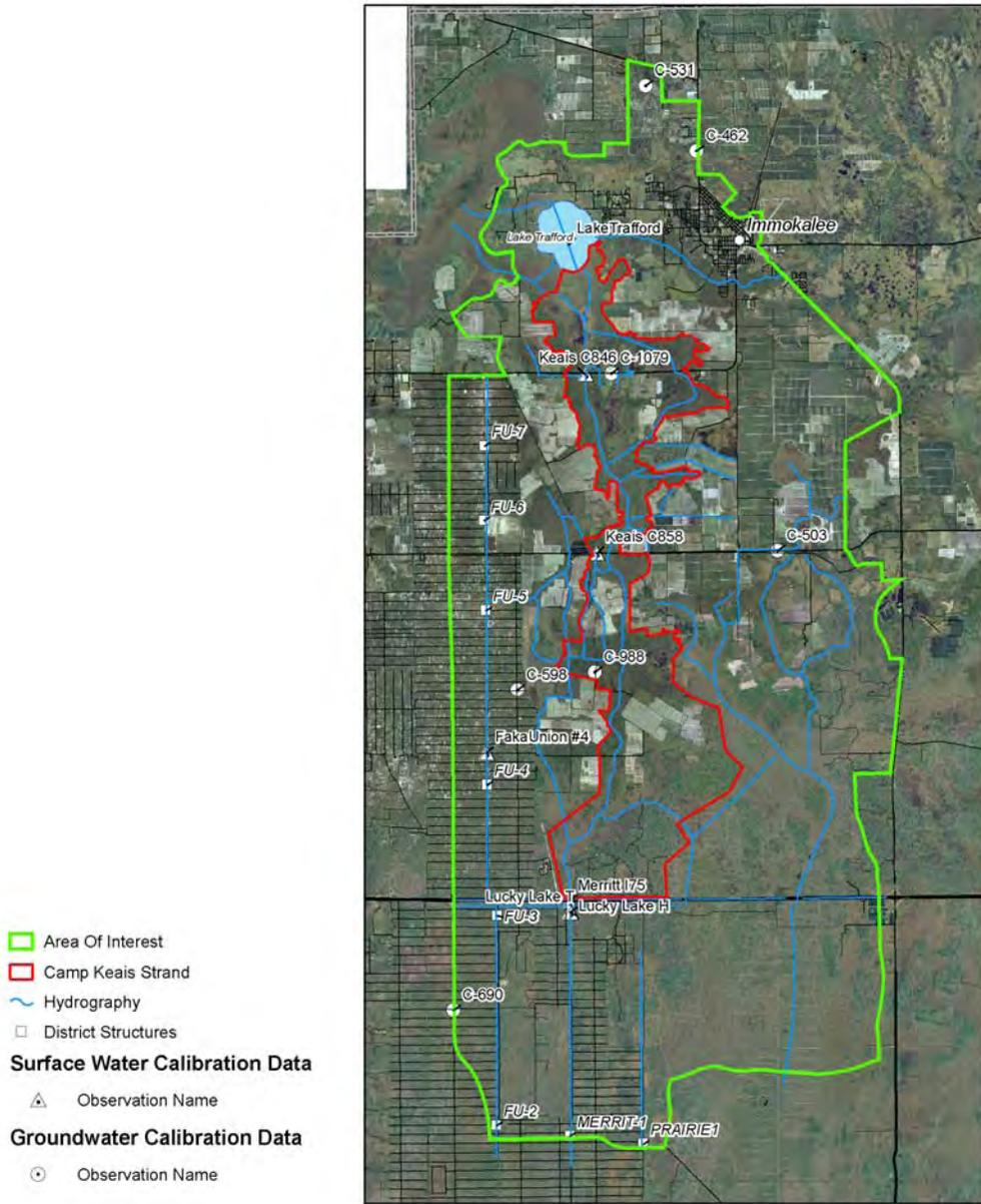
**Figure 2.4 Location of Surface Water Gages and Groundwater Observation Wells in the Vicinity of Camp Keais Strand.**
