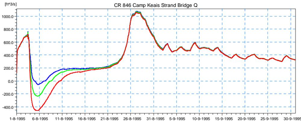
**Figure 4.17** Simulated Discharge Results for Existing Conditions (Scenario 0) at the Existing Bridge on CR-846 at Camp Keais Strand (Location 4) for the 5-year (blue), 25-year (green), and 100-year (red) Design Event.
