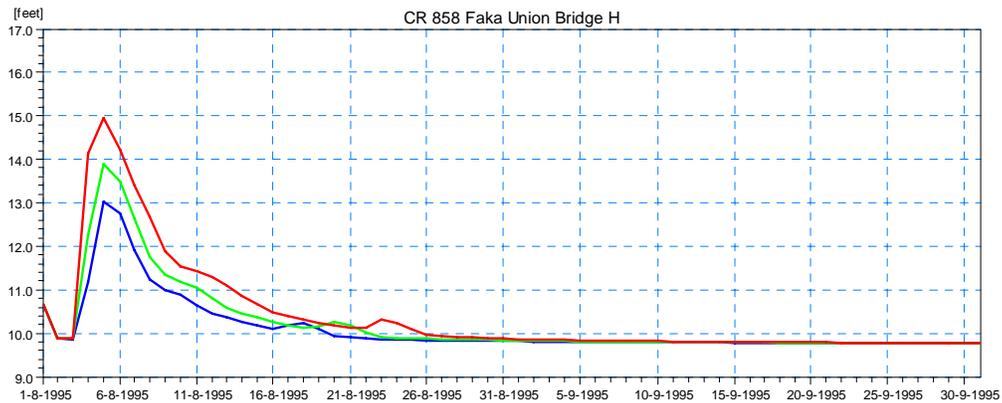
**Figure 4.44 Simulated Stage Results for Scenario 2 Upstream of the Proposed Modified Bridge on CR-858 at Faka Union Canal (Location 3) for the 5-year (blue), 25-year (green), and 100-year (red) Design Event.**
