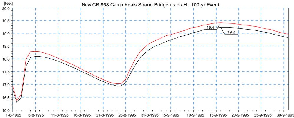
**Figure 4.37 Simulated Stage Results for Scenario 2 Upstream (red) and Downstream (black) of the Proposed Bridge on CR-858 at Camp Keais Strand (Location 1) for the 100-year Design Event.**
