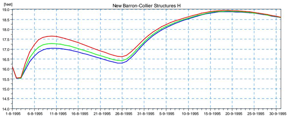
**Figure 4.50 Simulated Stage Results for Scenario 2 Upstream of the Proposed Modified Barron-Collier Structure in Camp Keais Strand (Location 5) for the 5-year (blue), 25-year (green), and 100-year (red) Design Event.**
