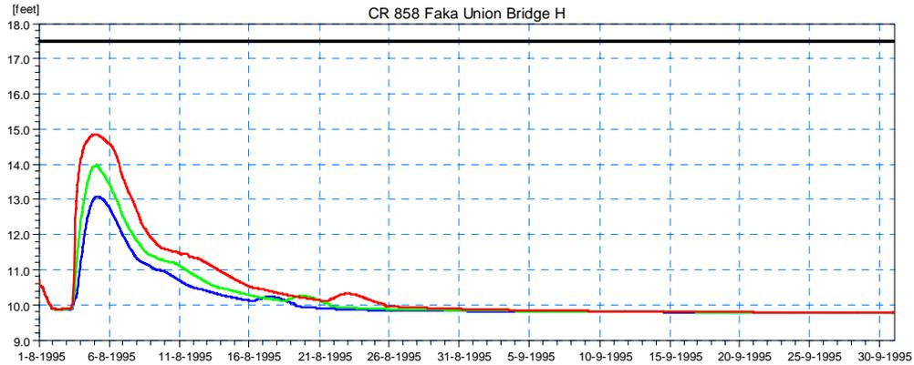
**Figure 4.13 Simulated Stage Results for Existing Conditions (Scenario 0) Upstream of the Existing Bridge on CR-858 at Faka Union Canal (Location 3) for the 5-year (blue), 25-year (green), and 100-year (red) Design Event.**
