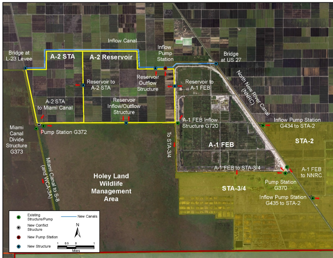
Figure 3.2. C240A Schematic Diagram Provided by EAASR Project Team
