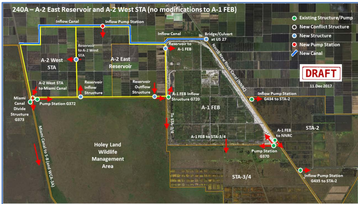
Figure 3.6. Example R240 Schematic Diagram Provided by EAASR Project Team
